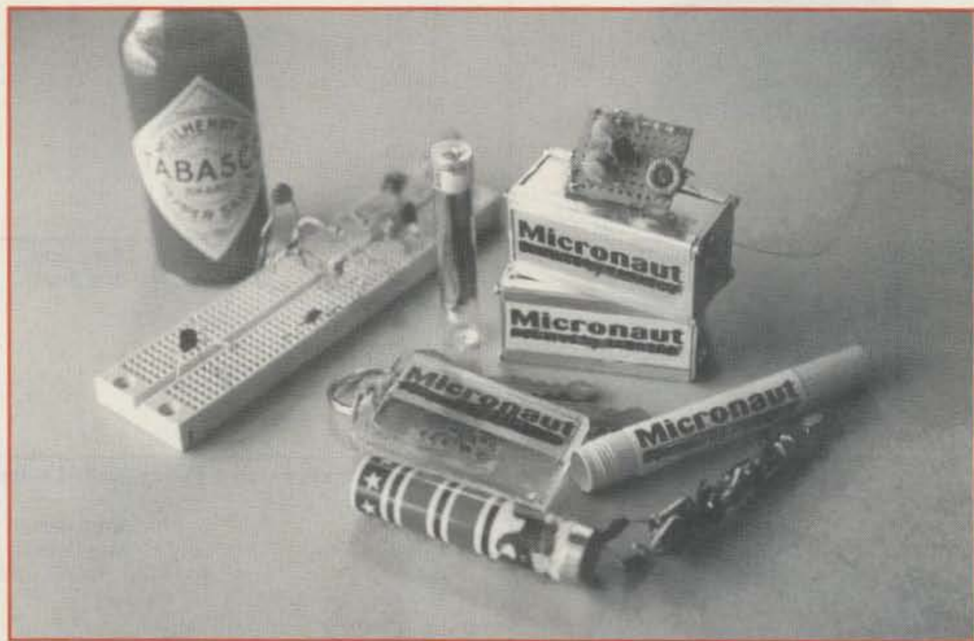
Fig. 2— Photo of my prototype Micronauts and a homemade hot-sauce battery. Circuits were first made by plugging leads of exact components into a white Radio Shack "building block," then moving those parts to perfboard, etc. Note chip components visible through clear keyfob. Pardon poor lighting in the photo; Paco was coaching the photo session.
