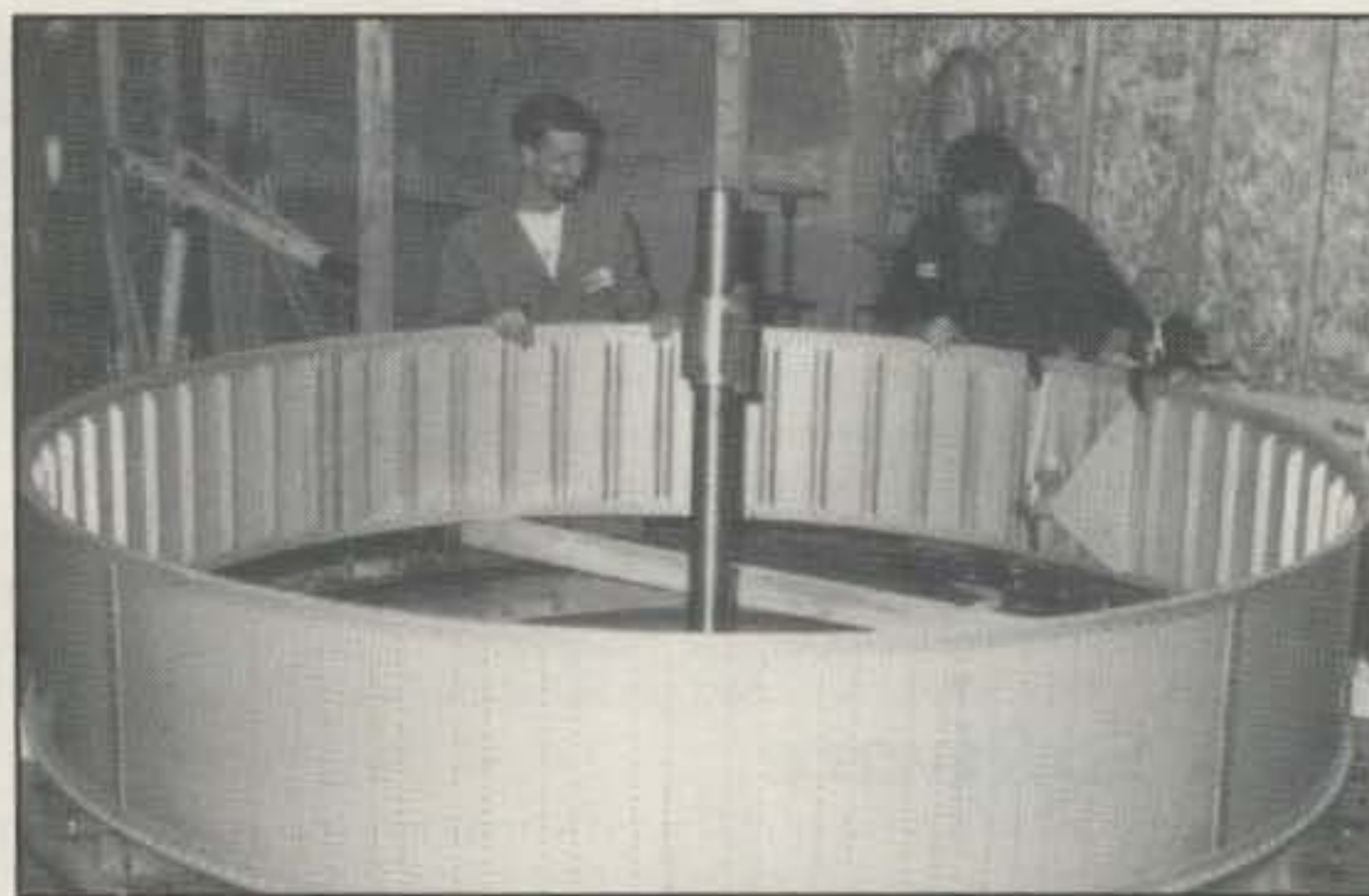
Here students Gene Hansen (left) and Richard Vanderford (right) inspect the completed flight model Phase 3D Specific Bearing Structure (SBS) in the Phase 3D lab at Weber State University in Ogden, Utah. The SBS will carry the Phase 3D satellite to orbit aboard its Ariane launch vehicle. (AMSAT-NA photo by Dick Jansson, WD4FAB)
