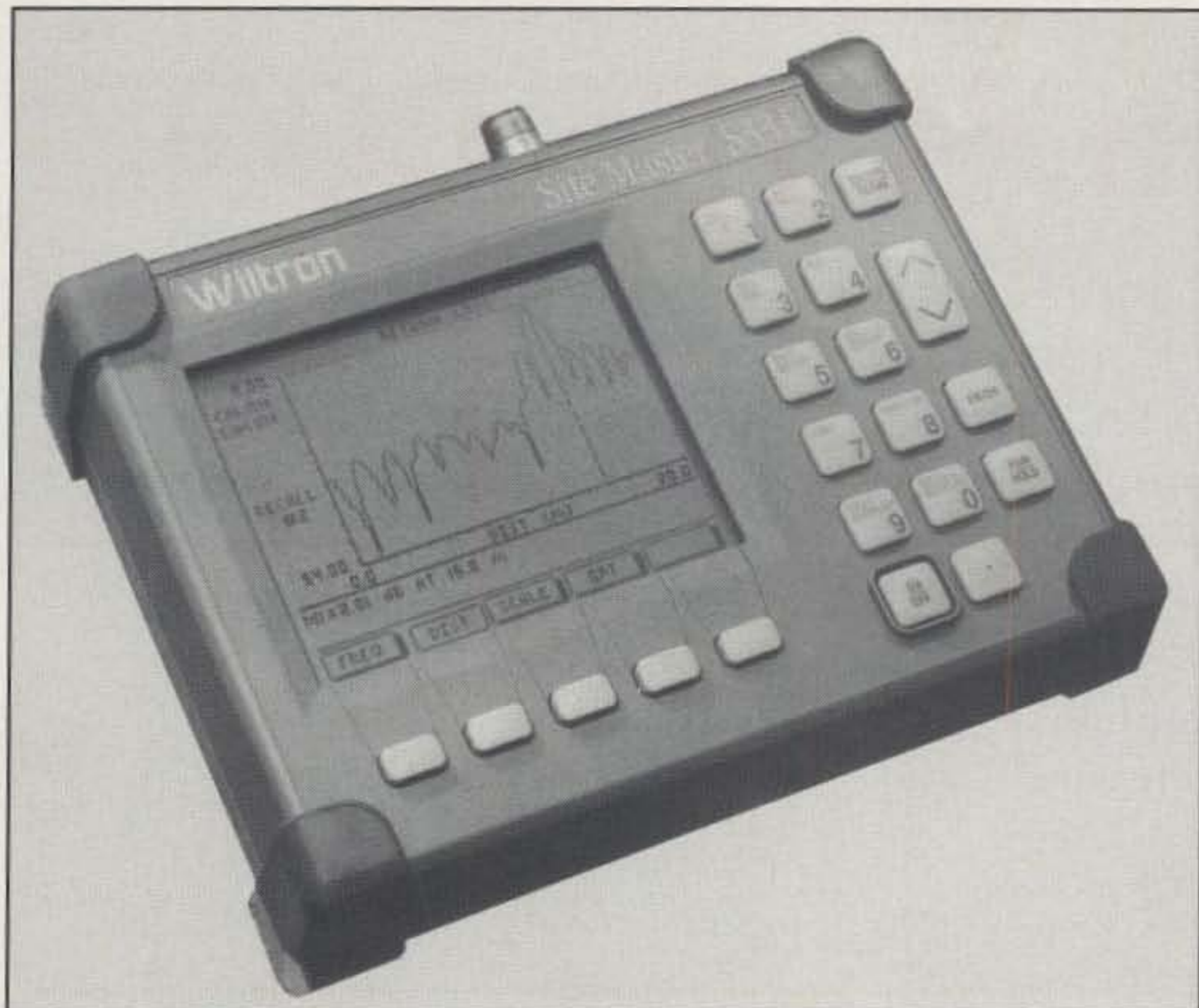
The Anritsu/Wiltron Site Master antenna analysis device.
