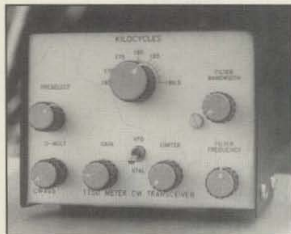
The Curry Communications CW495 1750 meter CW transceiver kit includes a receiver, pre-selector, RF Q-multiplier, noise limiter, and variable frequency and bandwidth filter. The transmitter is crystal controlled, but a variable frequency oscillator (VFO) also is available. The CW495 is shown installed in the optional cabinet. (Photo via Curry Communications.)
