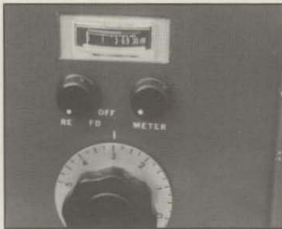
Photo 1—Photograph of an inexpensive tuning meter for use as an SWR indicator in a Murch antenna tuner.
