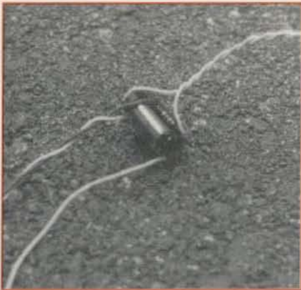
Photo 1— Reed relay mounted on "perf-board" provides building block for various interface applications.
