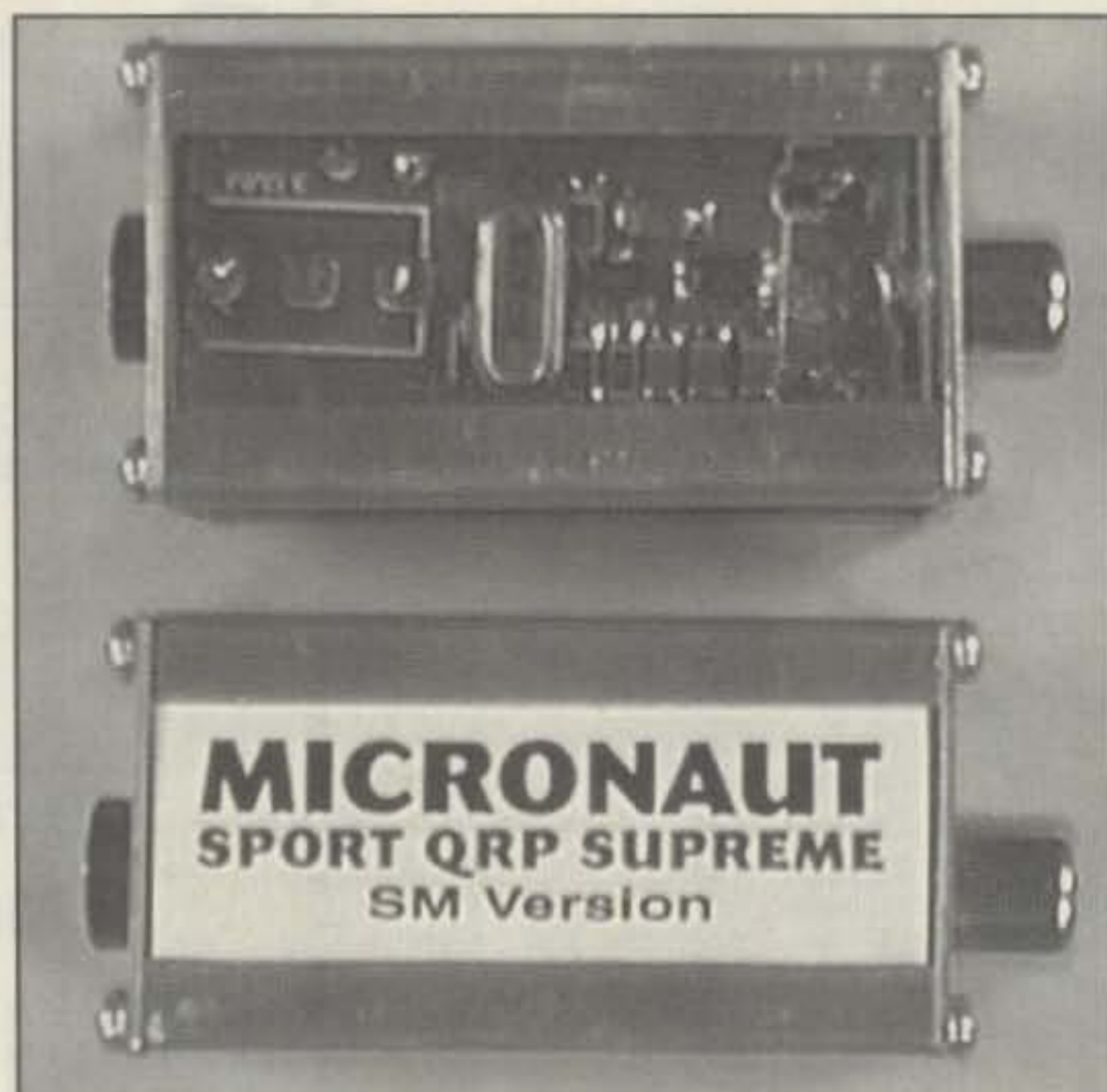
Fig. 5— Sescorm's miniature/surface-mount kit. This little delight is also supplied complete with all the pieces, and measures only 1.4 by .8 inch. (Photo by Sescorm, Inc.)
