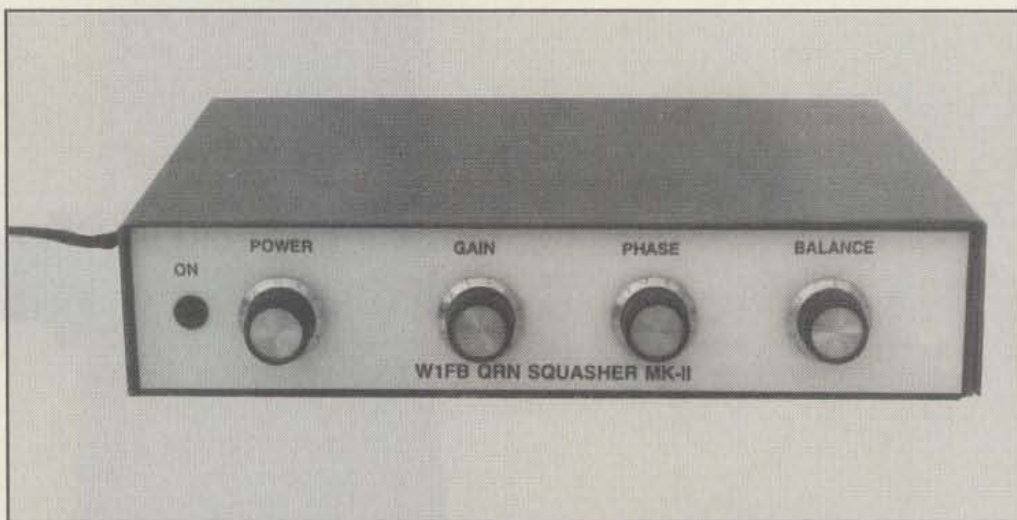
Front view of the completed unit. The front-panel design and lettering were done on a computer as described in the text.
