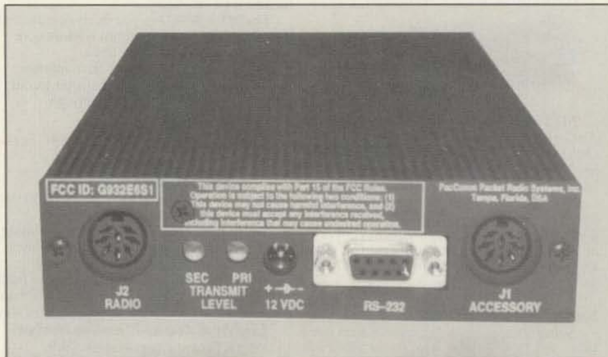
An RS-232 port is available on the rear of the unit. At the left is the radio socket.
