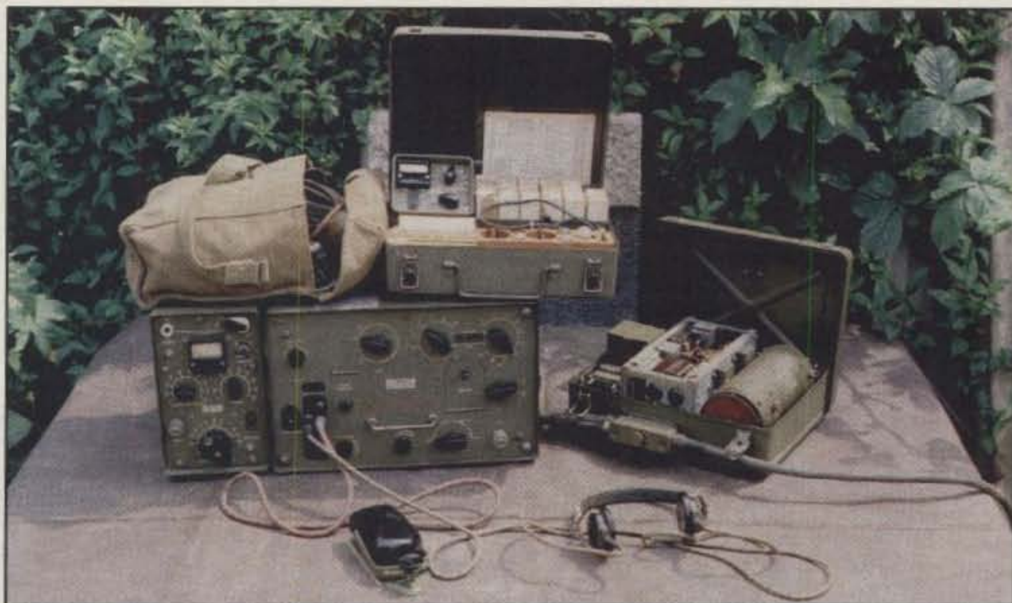
The RM-31a, with power supply on the right and spares box and headsets/mic satchel above. The ATU is on the left of the transceiver.
