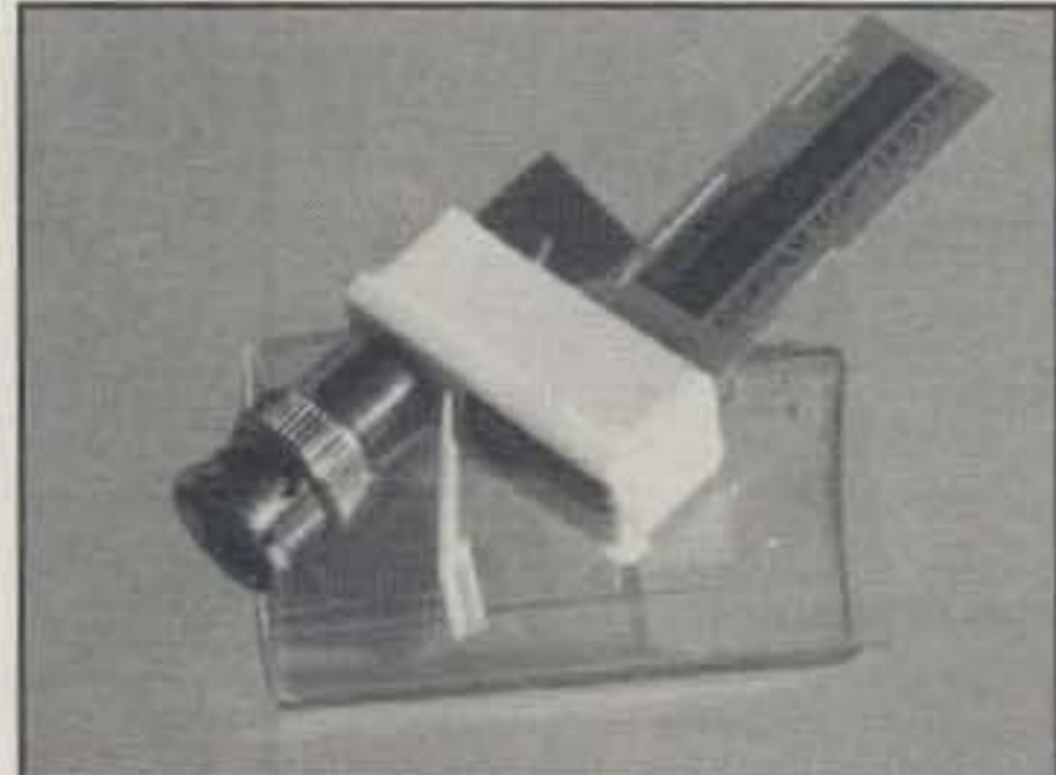
Front view of the battery tester strip and the associated container.
