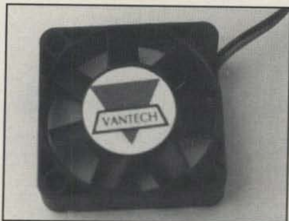
Photo 7— Ultra-small 12 volt DC fans such as those used on computer CPU chips are ideal for moving extra air to help internal cooling fans of transceivers that are squeezed into tight places.
