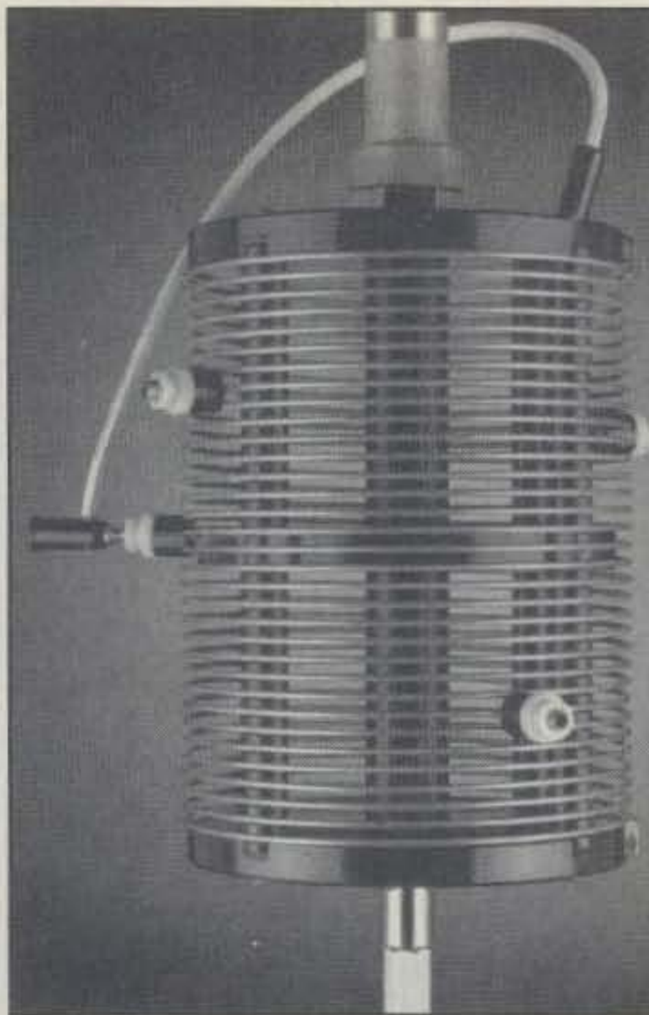
Photo 2— Close-up view of center loading coil in the Fortex Stealth antenna. The coil, taps, and all fittings are stainless steel. The item is 7 1/2 inches tall, 5 1/2 inches in diameter, and covers 80–15 meters. (Photo courtesy N4QB)
