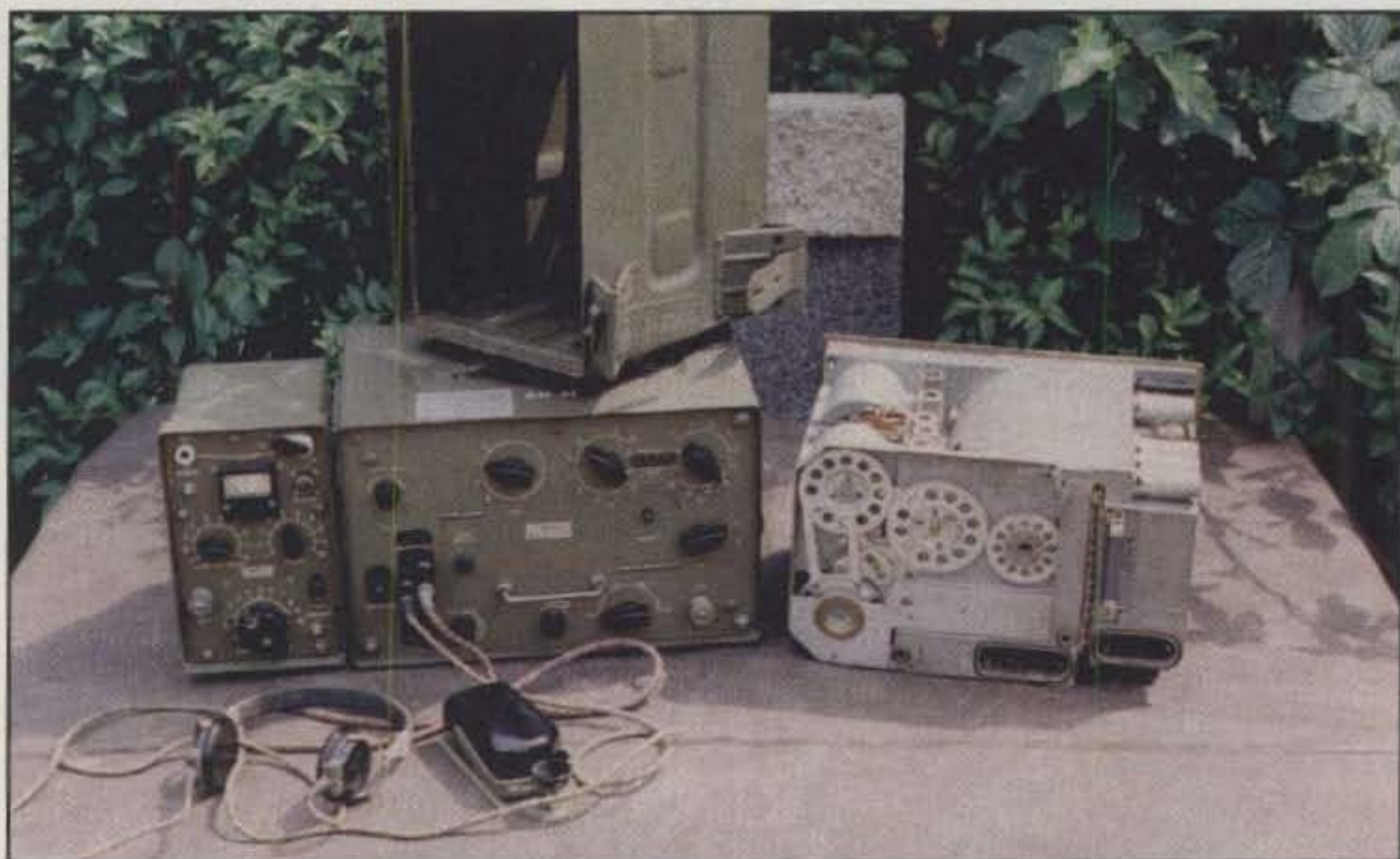
The RM-31a is shown on the left, with an internal view of the RM-31 on the right. Note the geared chain, which is operated during frequency selection.
