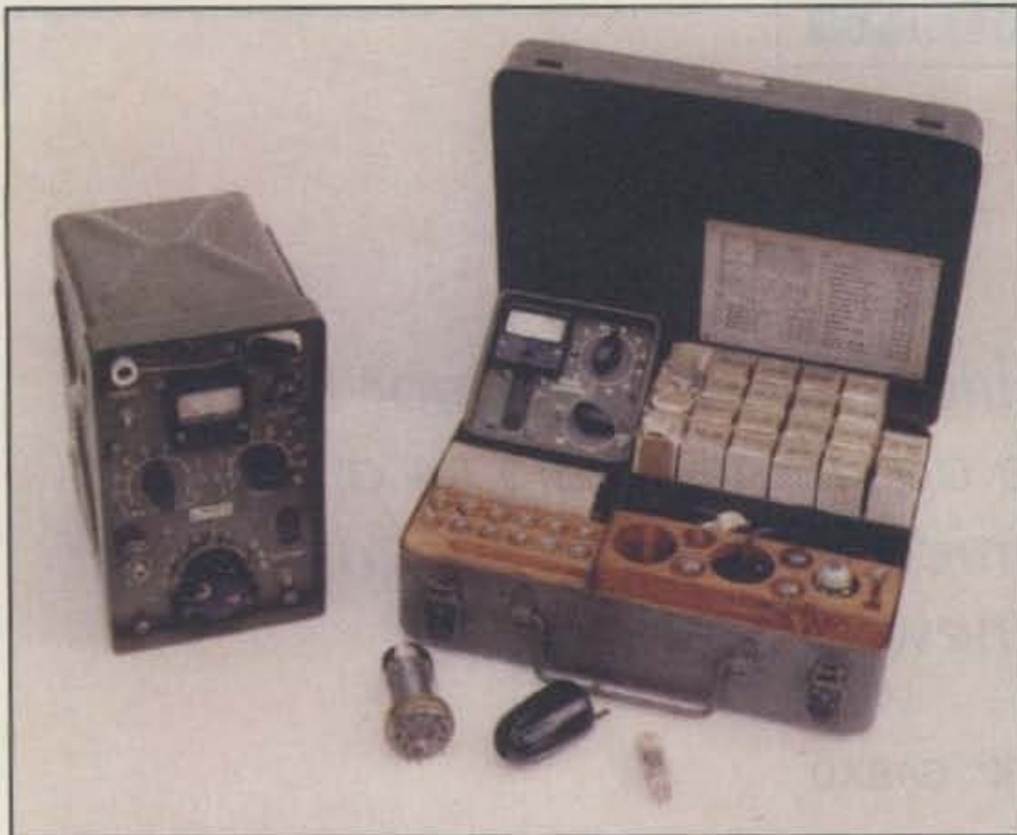
The RM-31 ATU and spares box. A spare amplifier tube can be seen at the front along with a dummy load device. ←
