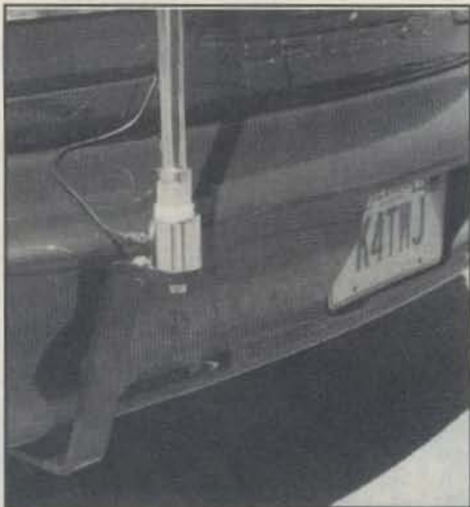
Photo 4—My custom Forex mount bolts to the car's underbody frame, contours around the bumper area, supports any size antenna, and solves an otherwise impossible problem.
