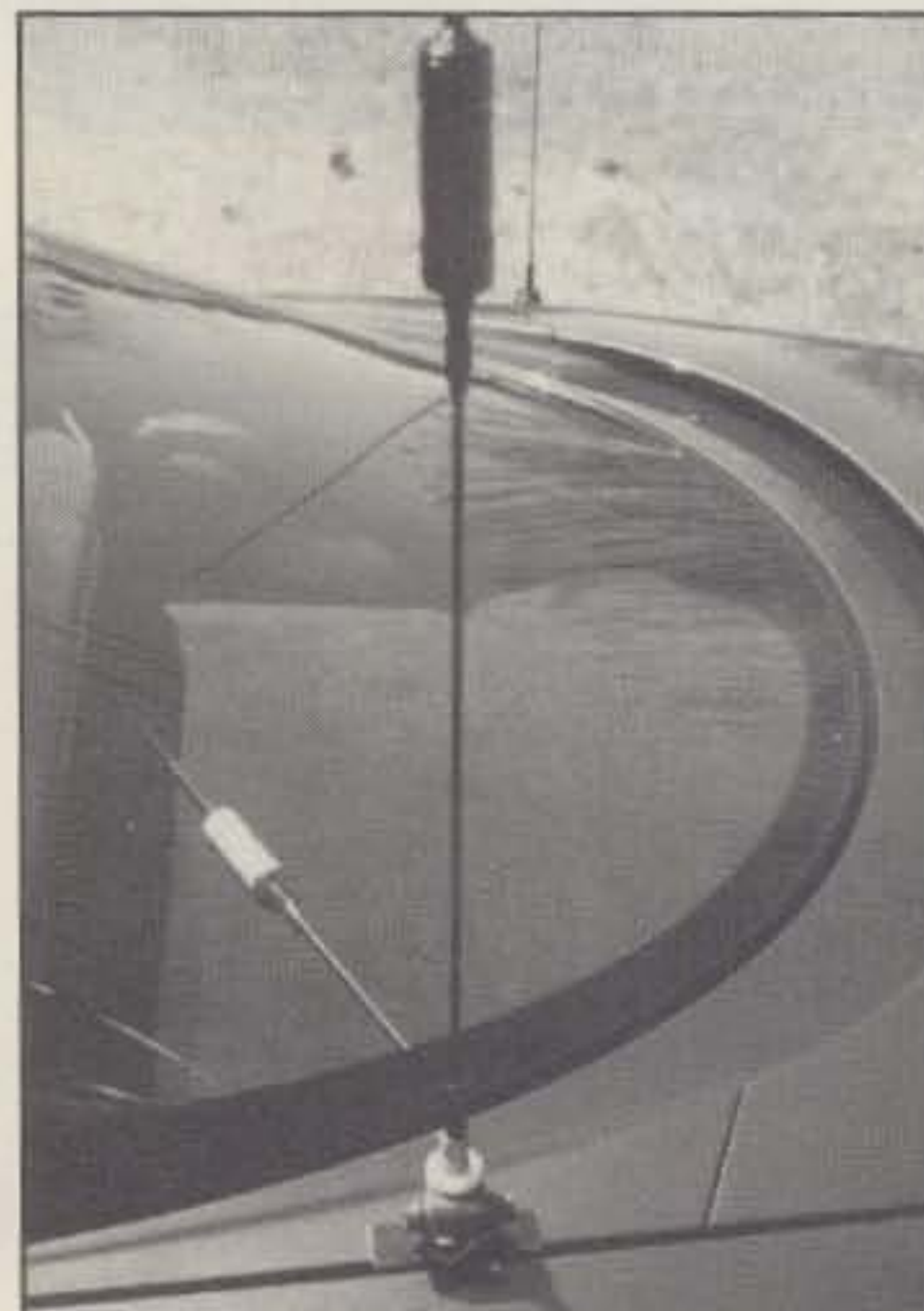
Photo 3— Here is a performance-improving idea everyone can use advantageously: Quick-strap a spare whip or resonator to a mount's ground connection, and use it to make a "one radial ground plane." As long as you are carrying them, you might as well put them to work in the rear window, right?
