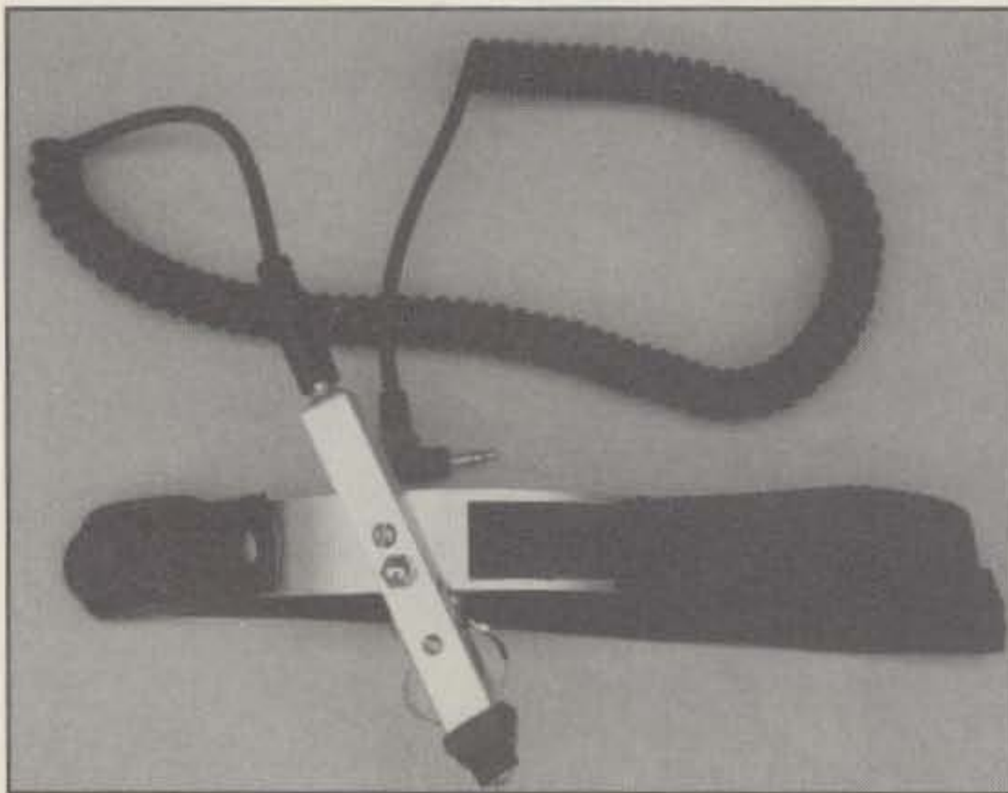
Photo 5— This clever new "Ne-Ke" was designed and is being made by Boyd Mason, N8VKA. It is a leg-strapped, smooth-handling iambic paddle, just the ticket for mobile CW.
