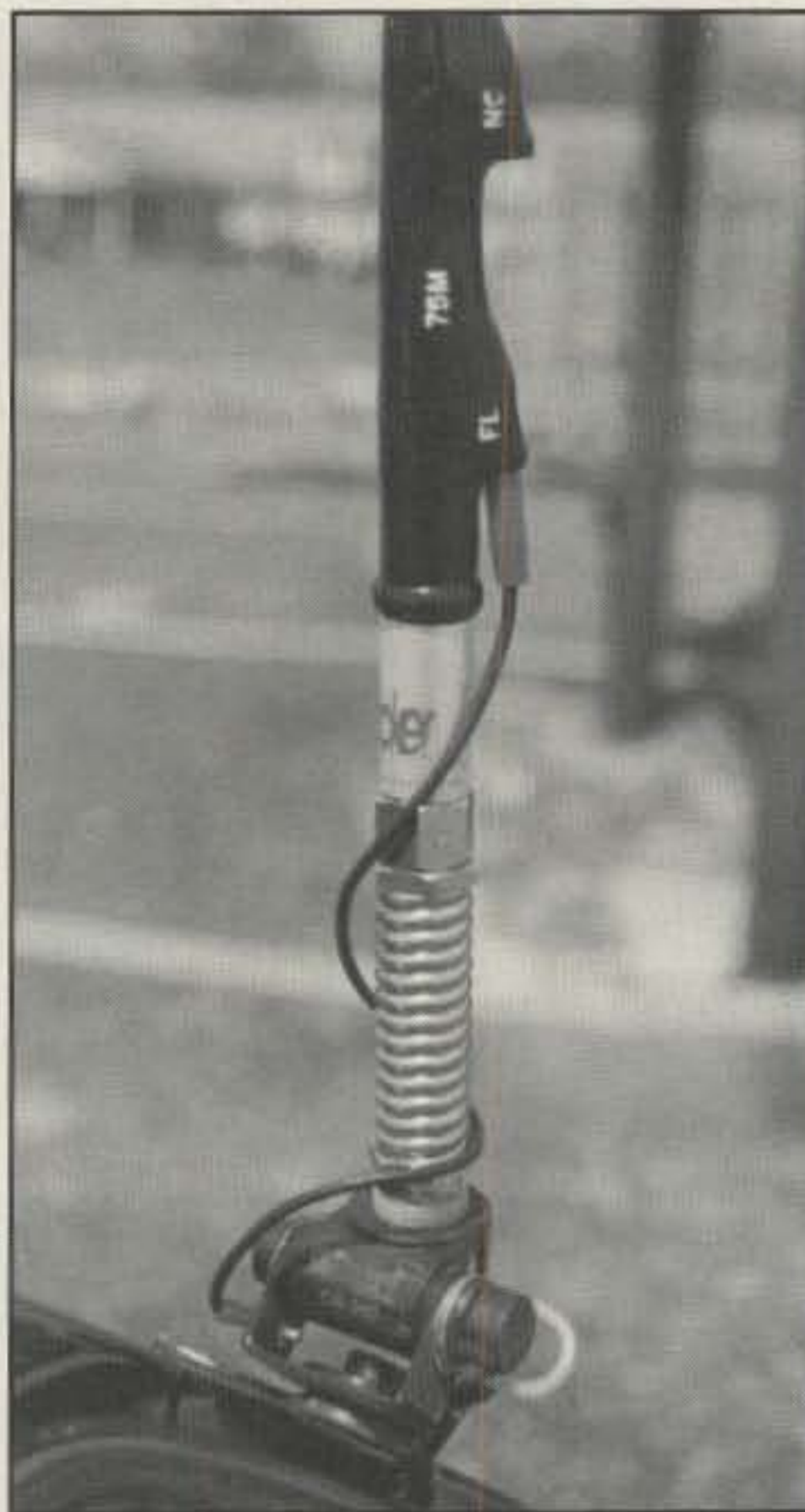
Photo 9— Outbacker's new OB-360 mount for the Perth Plus. It is supplied with spring and preassembled cable, and installs on a trunk or hatch lip in only a couple of minutes. (Photo by Don, WD4FSY.)
