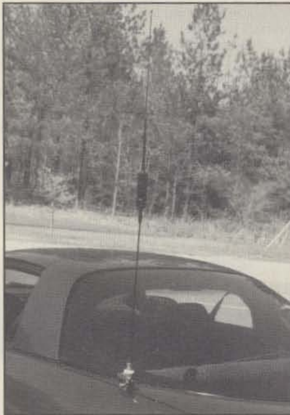
Photo 1— Trunk-lip or hatchback mounted antennas are popular because they are easy to install and they position the antenna over a metal ground. The concept works fine, provided the car's body is actually metal rather than non-conductive "composite material"!
