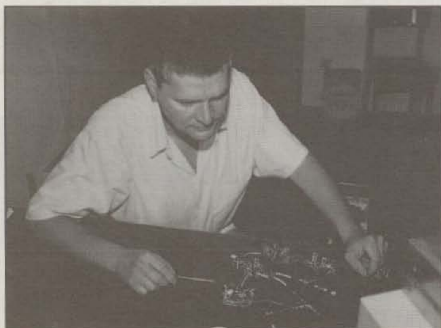
Photo E— Matjas Vidmar, S53MV, is shown experimenting with prototypes of the LEILA circuit for the Phase 3D satellite at his home workshop in Slovenia. A flight model of the LEILA now is slated to be carried aboard the satellite. It's designed to alert ground station operators who inadvertently run too much uplink power by superimposing a warning message on the "offending" station's downlink signal. (AMSAT-NA photo by Keith Baker, KB1SF)
