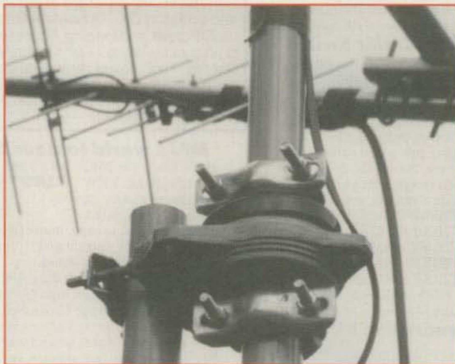
↑ This is a close-up view of the Phillips TB-105 support bearing. You will need two of these for this project.
