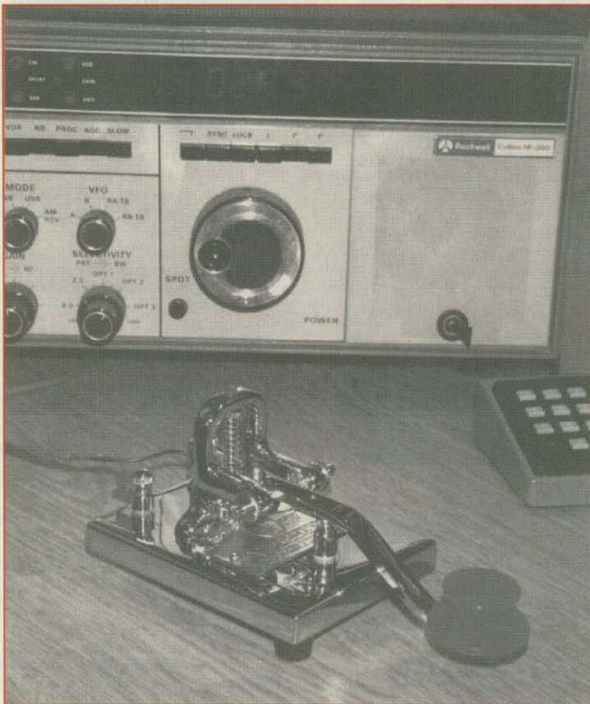
An old classic and a new one. Shown in this photo is the deluxe version of the new Vibroplex straight key.
