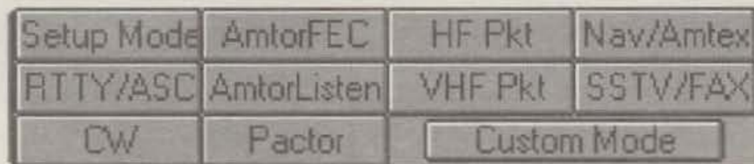
Fig. 4- The operating mode buttons are used to select the communications mode and to enter the "setup" mode.
