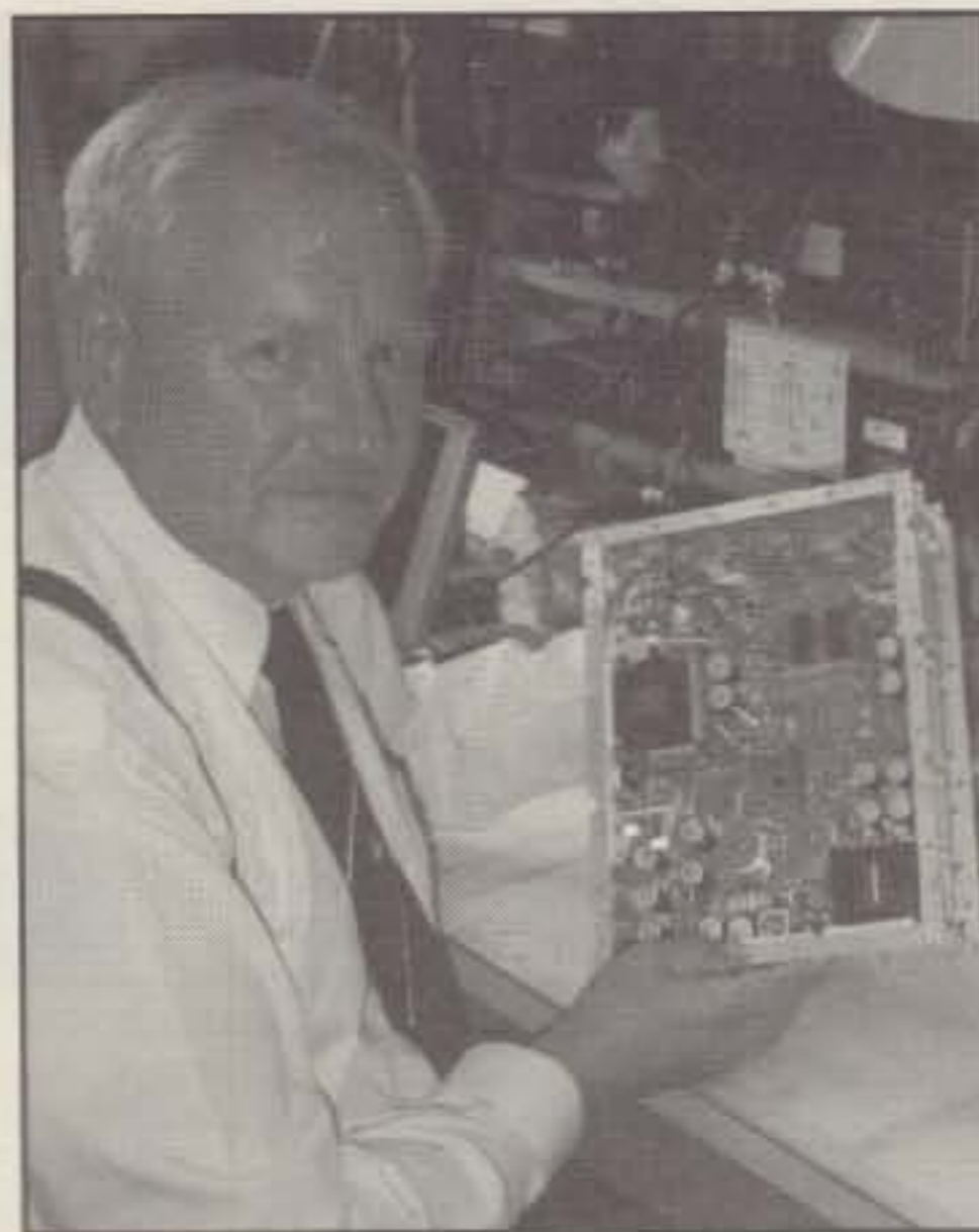
Dr. Andras (Bandi) Gschwindt, HA5WH, proudly displays Phase 3-D's Battery Charge Regulator (BCR) at the Marburg P3-D Lab. The BCR is a critical piece of Phase 3-D flight hardware that will control all the spacecraft's on-board power activity, such as regulating battery charging from the solar panels. The BCR was expertly built by bandi and his team at the Technical University of Budapest, Hungary.
