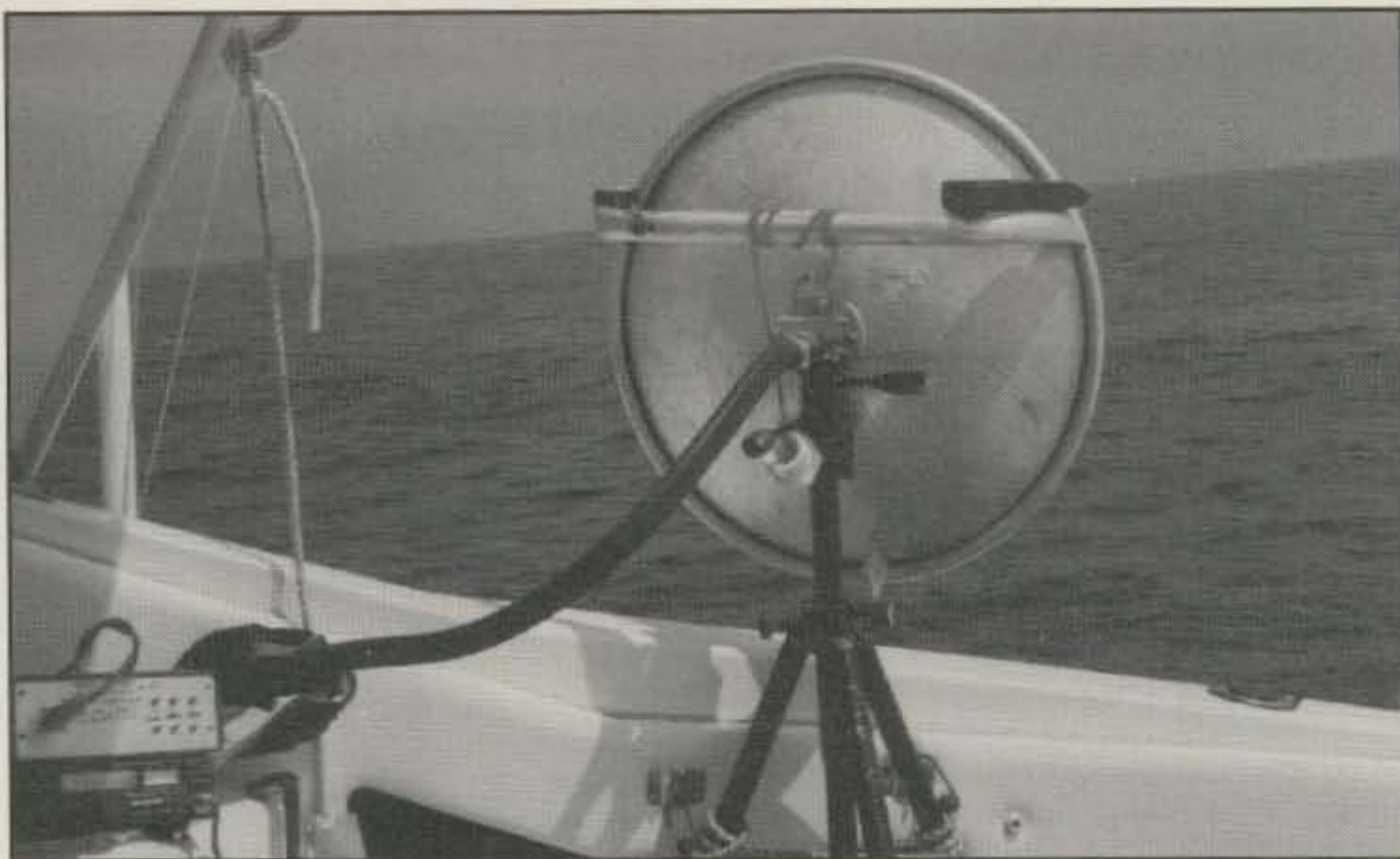
Gordon West, WB6NOA, used this 2 foot dish, hooked to the 100 mW transverter during the first weekend of the ARRL 10 GHz and above contest. (Photo courtesy WB6NOA.)
