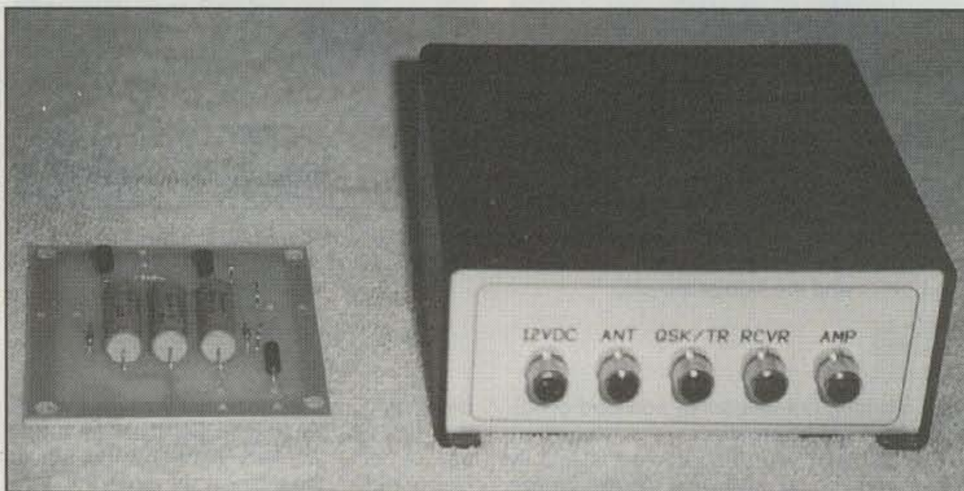
This view shows the completed board outside of a suitable cabinet. This is the rear of the cabinet showing the connecting jacks.
