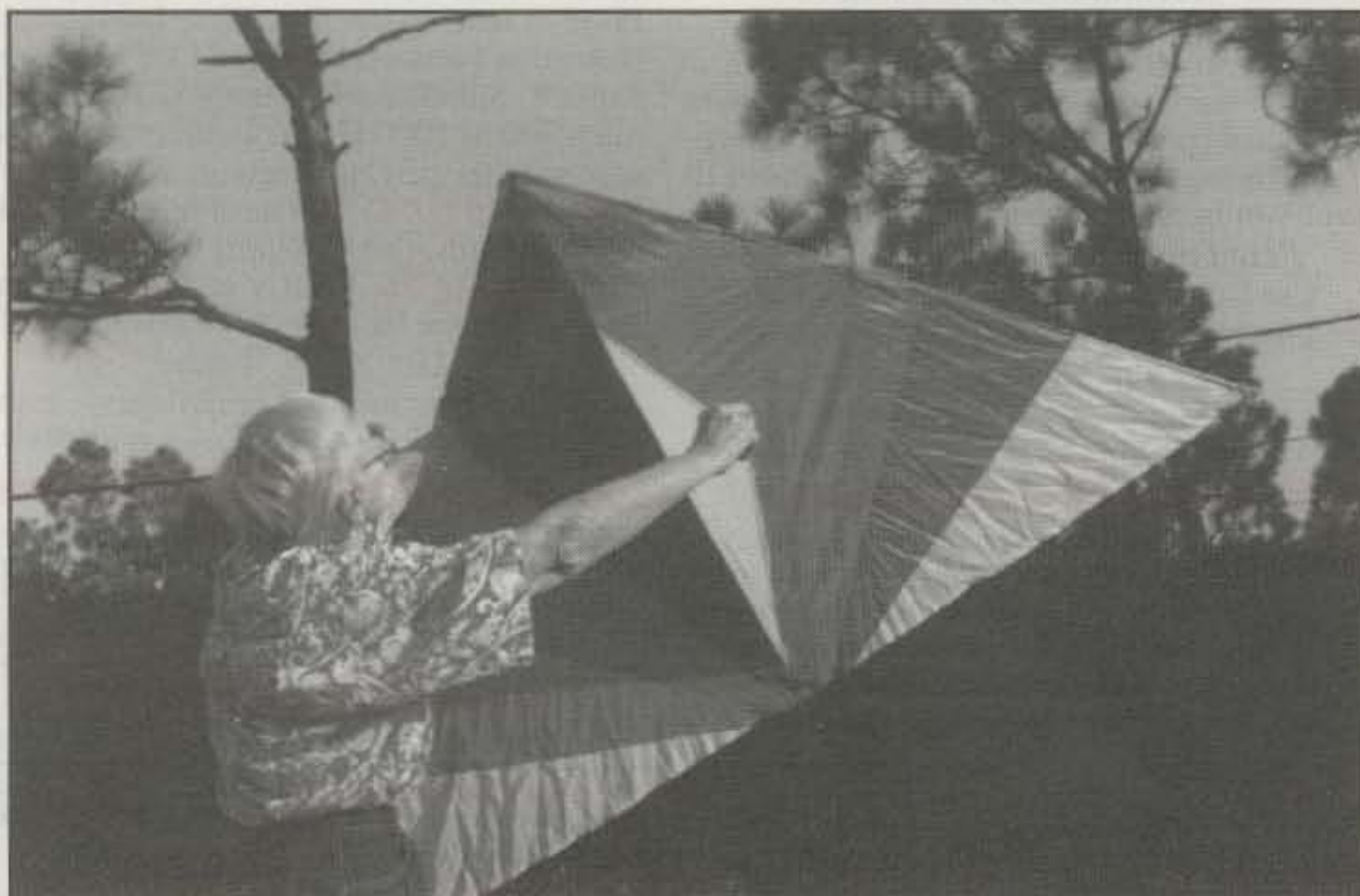
A delta wing kite. This one has a 6 foot wingspread and it can lift a couple of pounds into the air in a modest breeze.
