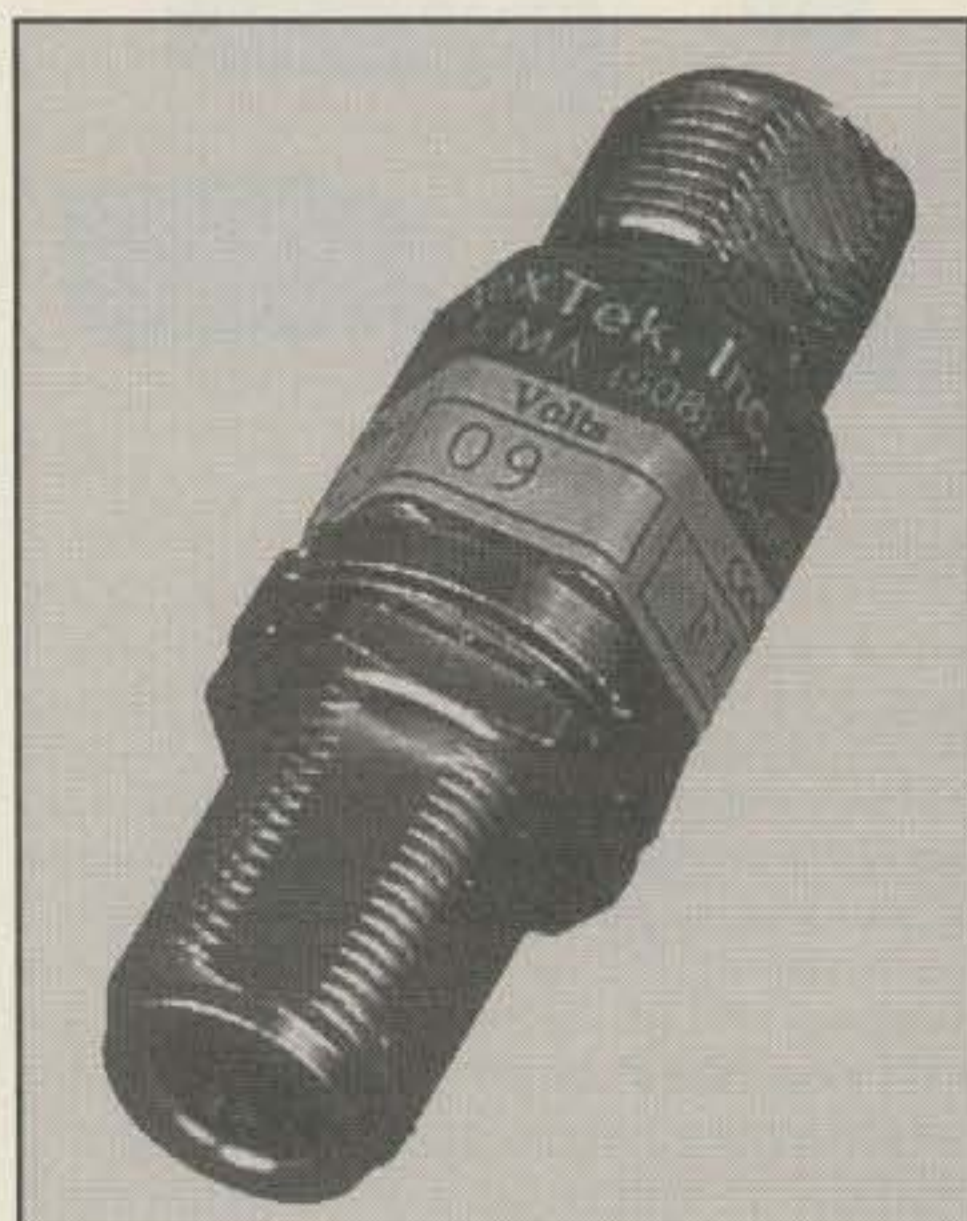
Gas discharge tubes (GDTs) sense voltage. When high voltages or spikes occur, the GDT clamps the transient to ground. This one is made by NexTek; it covers from DC to 2.5 GHz.
