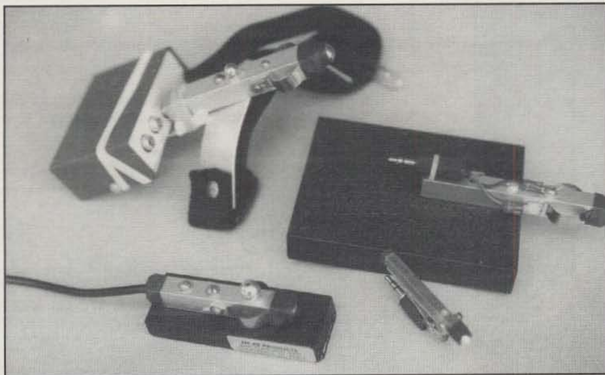
Photo 3— Ne Ke madness for sure! Top left: My leg-strapped Ne Ke is plugged into a self-contained Radio Adventure Company keyer for stand-alone use. Top right: The kit Ne Ke on a black wrinkle base. Left bottom: A black-base QRP Ne Ke positioned in line as discussed in photo 2. The final Ne Ke is a tie-tack paddle.
