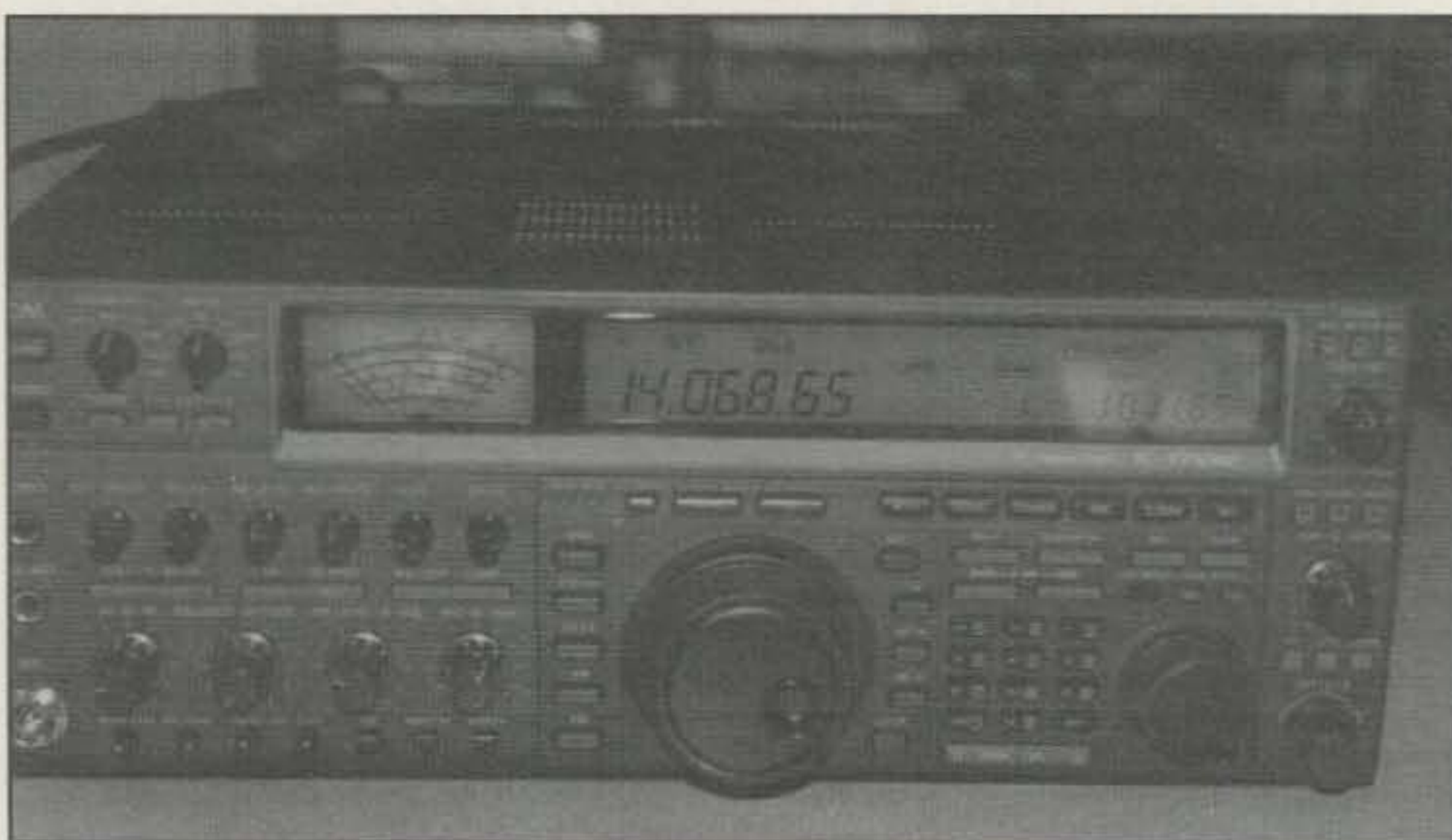
The IC-775DSP transceiver is a really nice box that puts out a 200 watt signal. The various mode switches are just to the left of the main tuning dial. The readout panel is clear and very easy to read.
