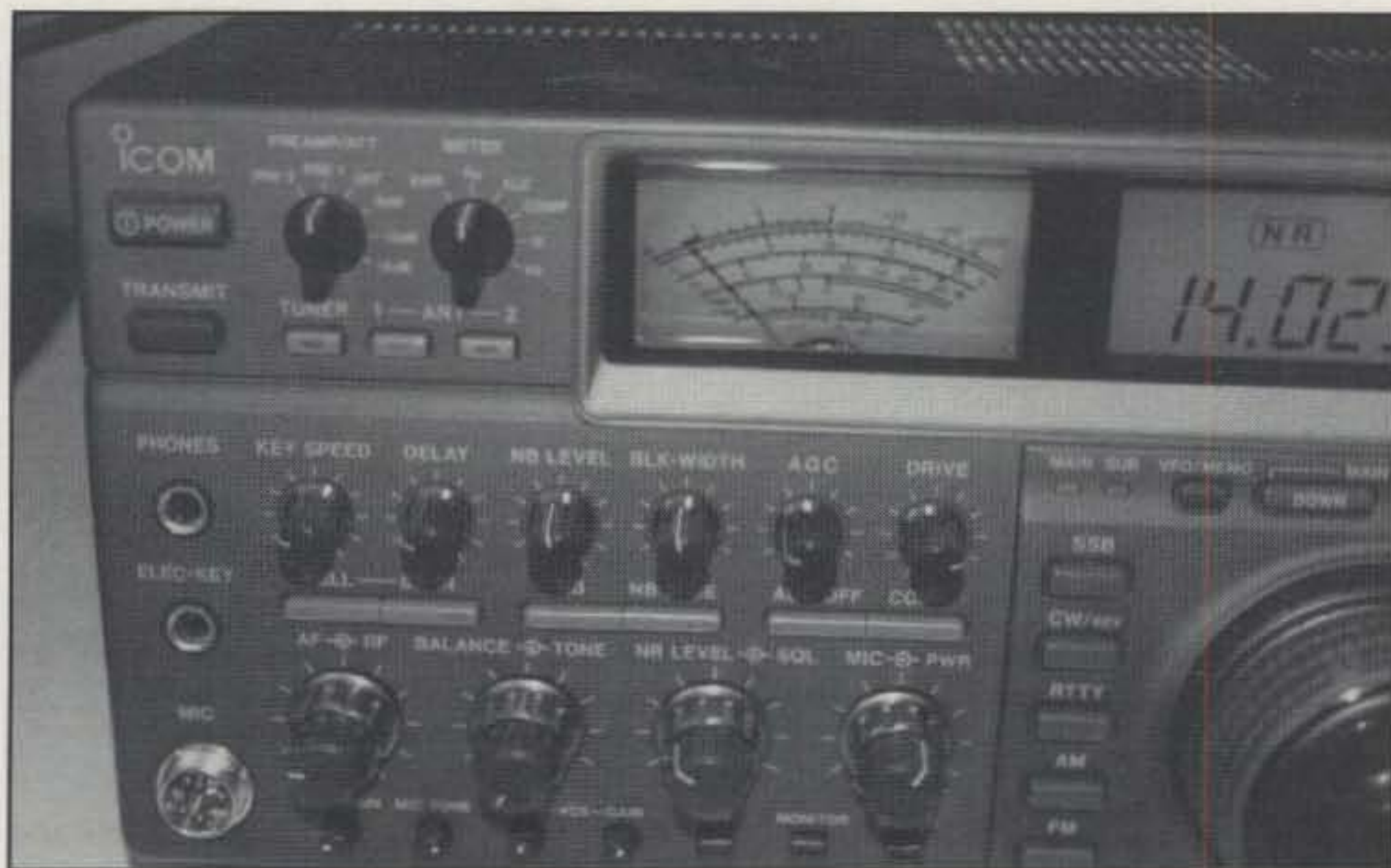
This is the left side of the front panel. There are lots of controls, and they take a little getting used to. At the upper left are the preamp controls and the meter reading switch. Below those are the tuner controls, one for either antenna input. Then there are the keyer controls, followed by noise blanker controls, then AGC and compressor controls. At the bottom left are the AF/RF, Balance/Tone, NR (noise reduction level), and Squelch, followed by Mic gain and PWR controls.
