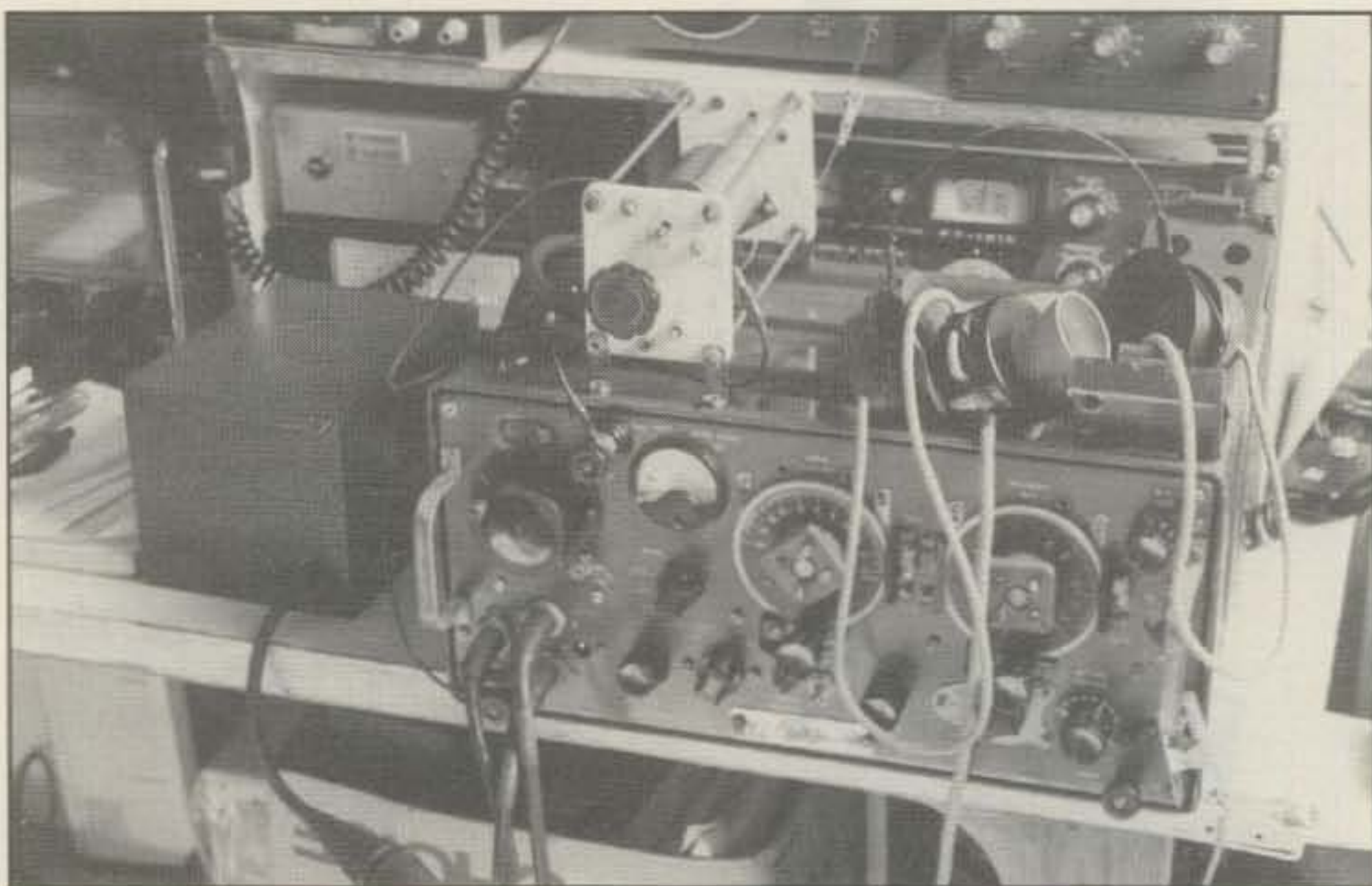
This is a front view of the wireless set No. 22. I typically use this on 80 meters for contacts up to 100 miles.
