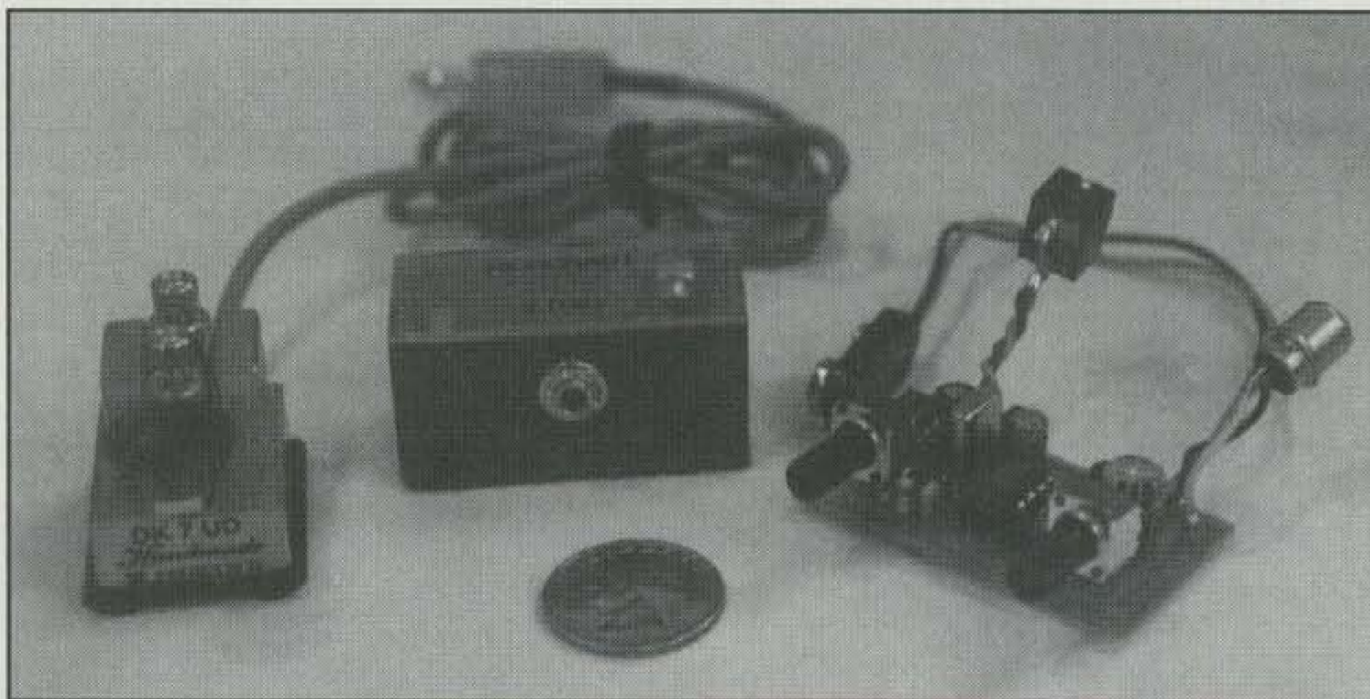
Photo 2— Carry a complete HF station in your shirt pocket? You bet! A couple of Micronauts do the trick. Shown here with a quarter for size reference is my Micronaut transmitter (middle) and K8IDN's mating receiver (right). The receiver's PC board is a fraction larger than the transmitter's board. Both items are available in easy-to-assemble kits. The miniature key, incidentally, was handmade by DK7UD and belongs to K8IDN.
