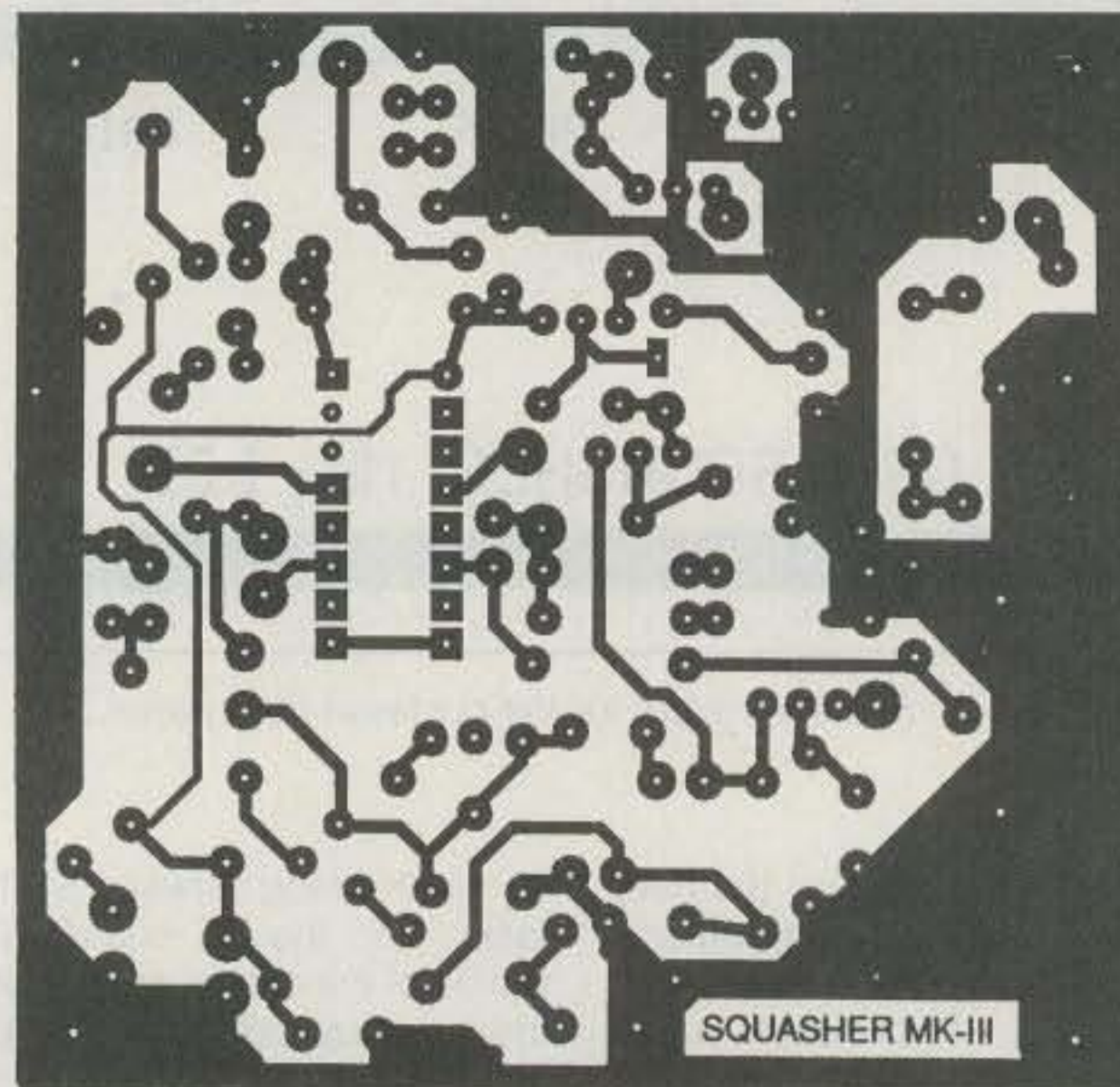
Fig. 7— Scale etching pattern for the MK-III Squasher as viewed from the etched side.
