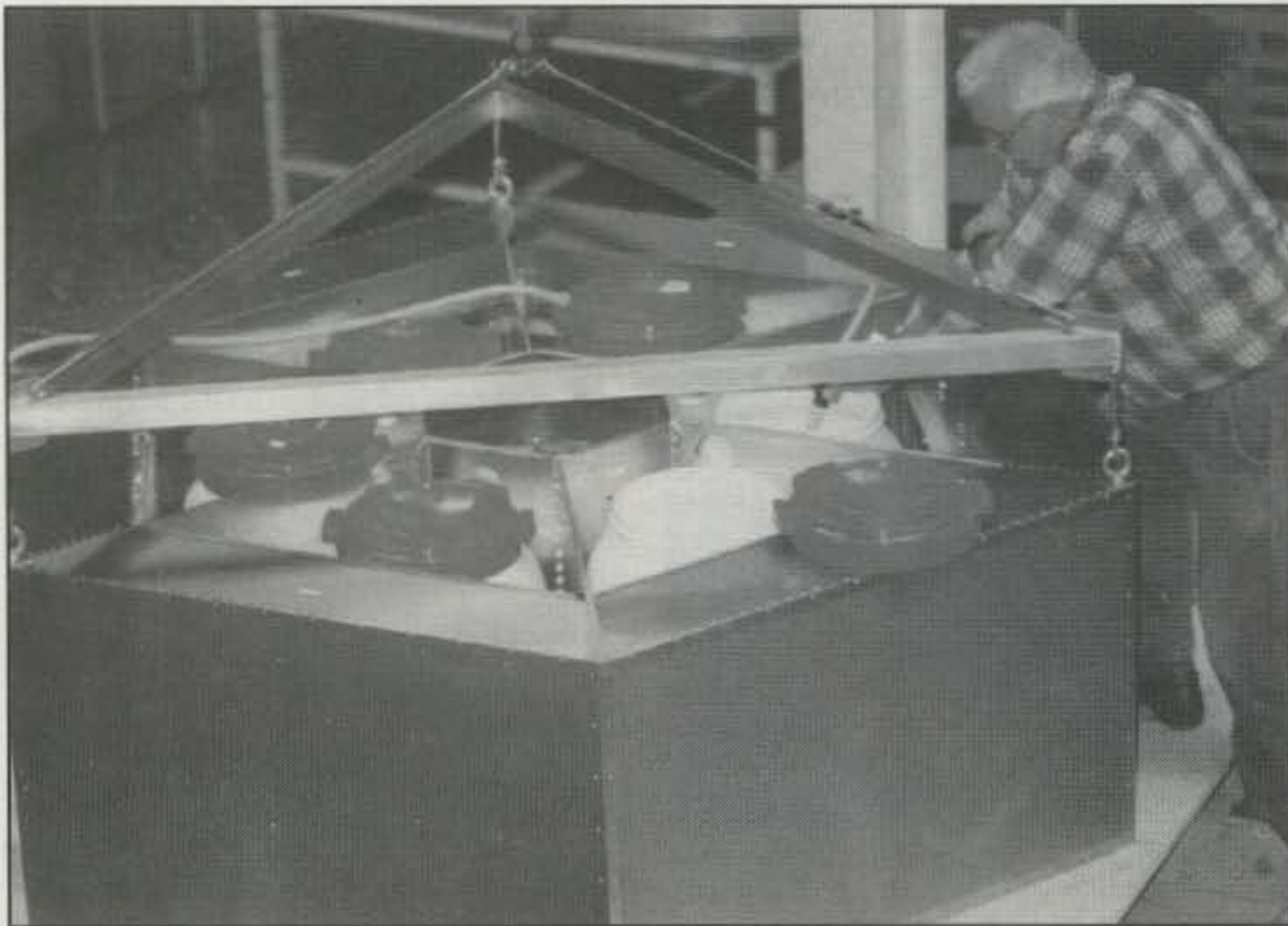
Here AMSAT-DL's Konrad Mueller, DG7FDQ, adds water to one of the "propellant tanks" of the Phase 3D engineering model. The photo was taken just prior to the first spacecraft dynamic tests of the AMSAT Phase 3D spaceframe and launch structure while mated with an Ariane 5 test stand. Konrad mounted plastic water jugs into the model to simulate propellant tanks. He also added wood blocks in the equipment bays to simulate electronic modules. The tests investigated how well the spacecraft and carrying structures will perform. (AMSAT-NA photo by Keith Baker, KB1SF)
