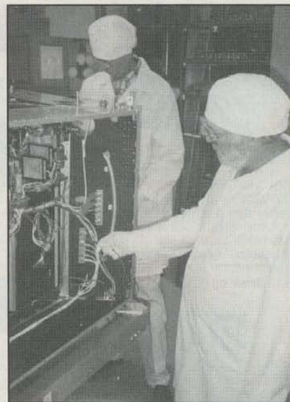
In a scene reminiscent of a hospital operating room at the Phase 3D International Satellite Integration Laboratory at Orlando, Florida, AMSAT Phase 3D Integration Laboratory Manager Lou McFadin, W5DID (right), and Stan Wood, WA4NFY, AMSAT-NA Assistant VP, Engineering (left), perform extensive continuity tests of the Phase 3D wiring harness. (AMSAT-NA photo by Keith Baker, KB1SF)
