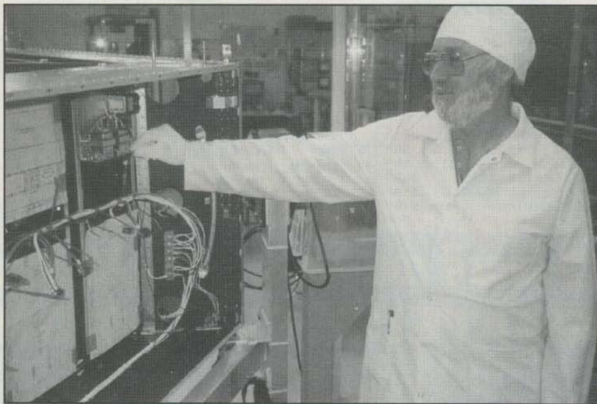
Here AMSAT Laboratory Manager Lou McFadin, W5DID, points out the satellite's VHF/UHF antenna relays in this photo taken at the Phase 3D Lab. The high-power, "space-rated" relays were provided by Dow-Key Corp. to switch receivers and transmitters between high-gain and omnidirectional VHF/UHF antennas on the spacecraft. The 2 meter transmitter position is located just below Lou's hand. (AMSAT-NA photo by Keith Baker, KB1SF)
