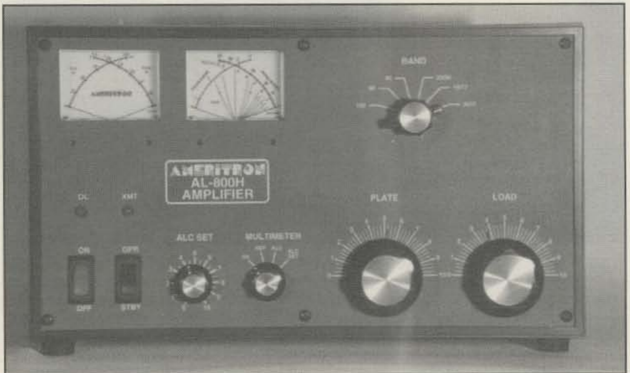
Front view of the Ameritron AL-800H linear amplifier.
