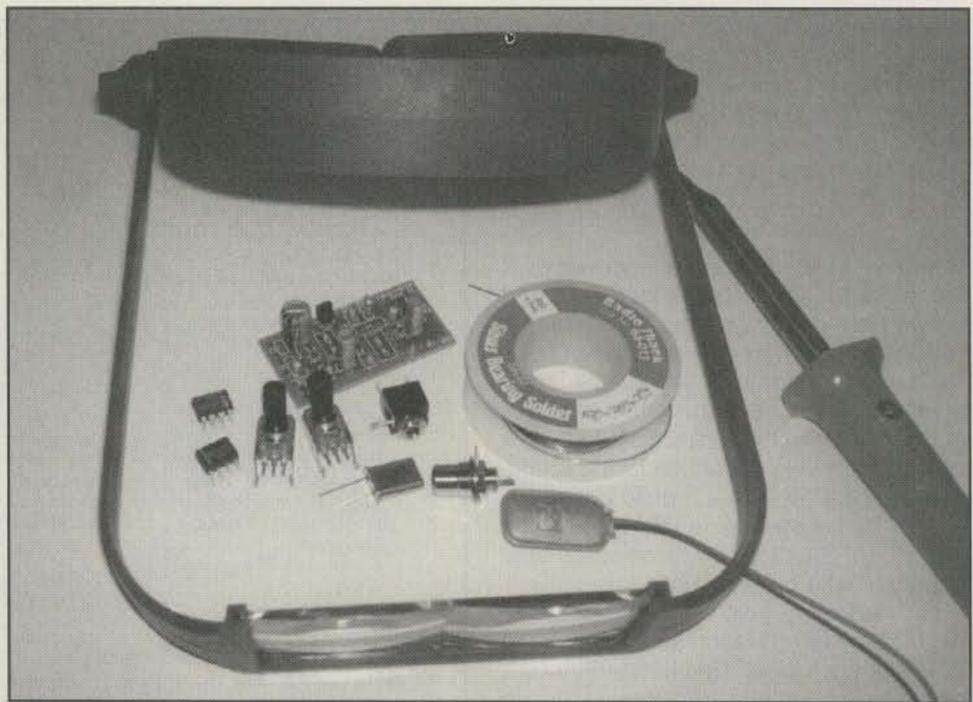
The MRX receiver is shown here midway through assembly. Magnifying goggles are great for turning fine work into relaxing enjoyment. A sharp-tipped iron and ultra-thin solder ensure accurate soldering without PC run "bridges."
