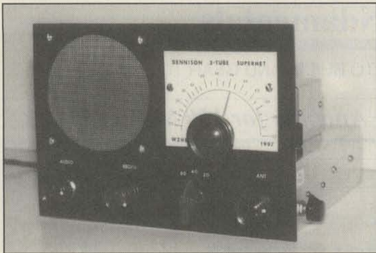
↑ Front view of W2HBE's slightly updated version of Frank Jones's 1936 superhet receiver.
