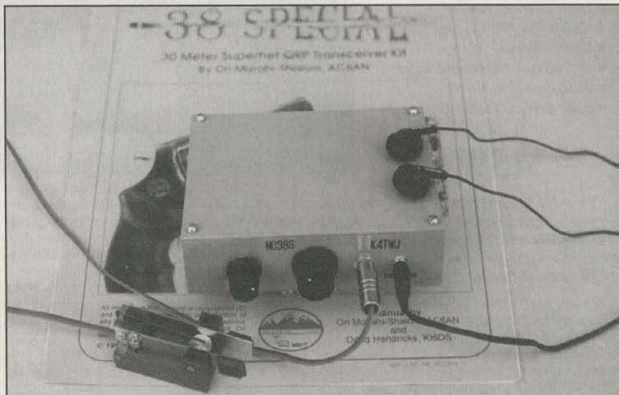
Photo 1— Amateur radio at its best! My NorCal 38 Special measures 1.2"H x 4.2"W x 3.2"D, slips right into a coat pocket, and pumps out a solid 5 watt signal. The little gem worked 5 countries during its first 5 minutes on the air. Details on the rig, plus the new 1" x 1.75" "Paddlette" beside it are in the text.
