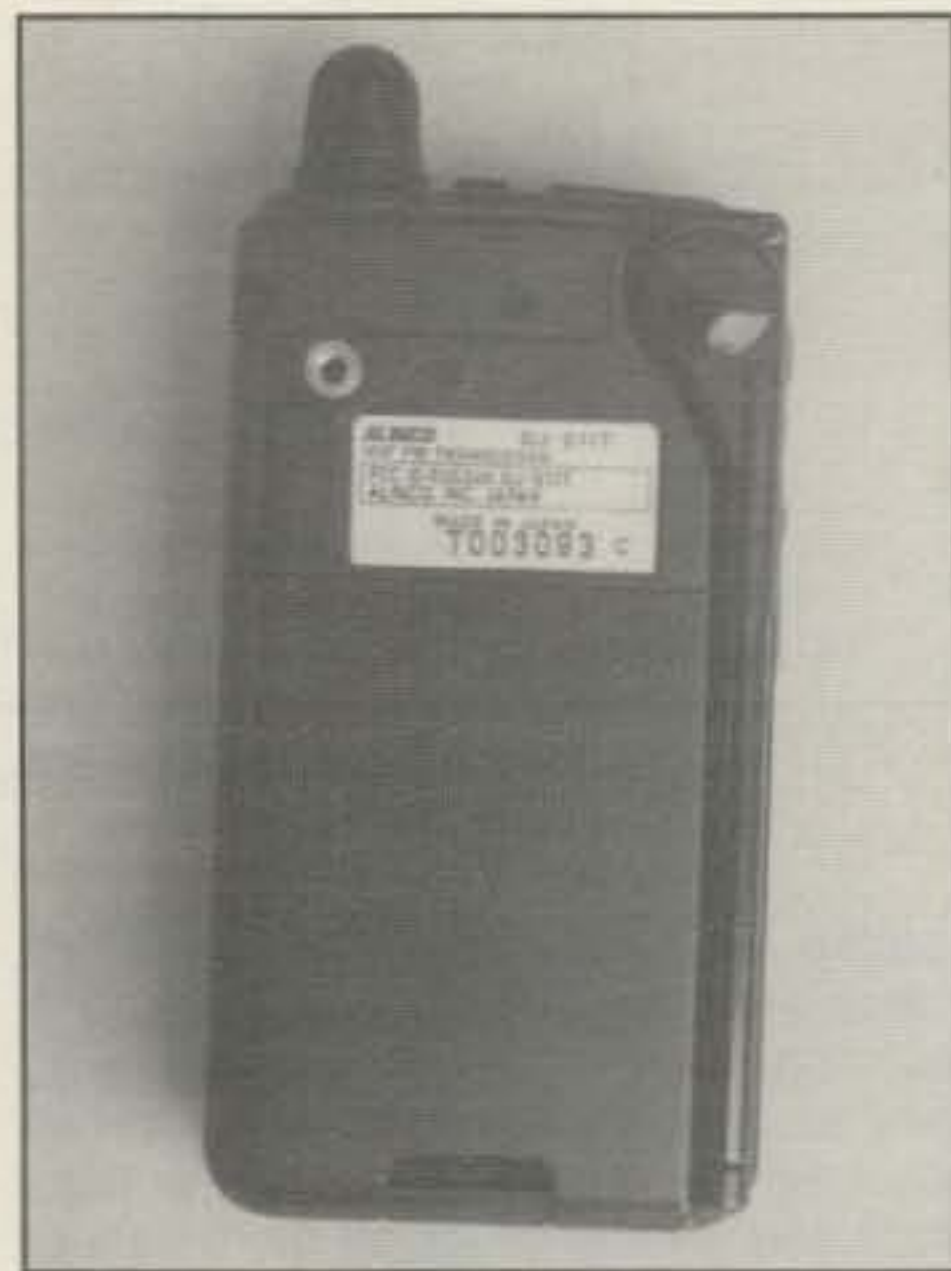
Rear view of the DJ-S11T showing the swivel-up antenna nestled into the groove on the case back. One grab and you have a ready-for-action handheld.
