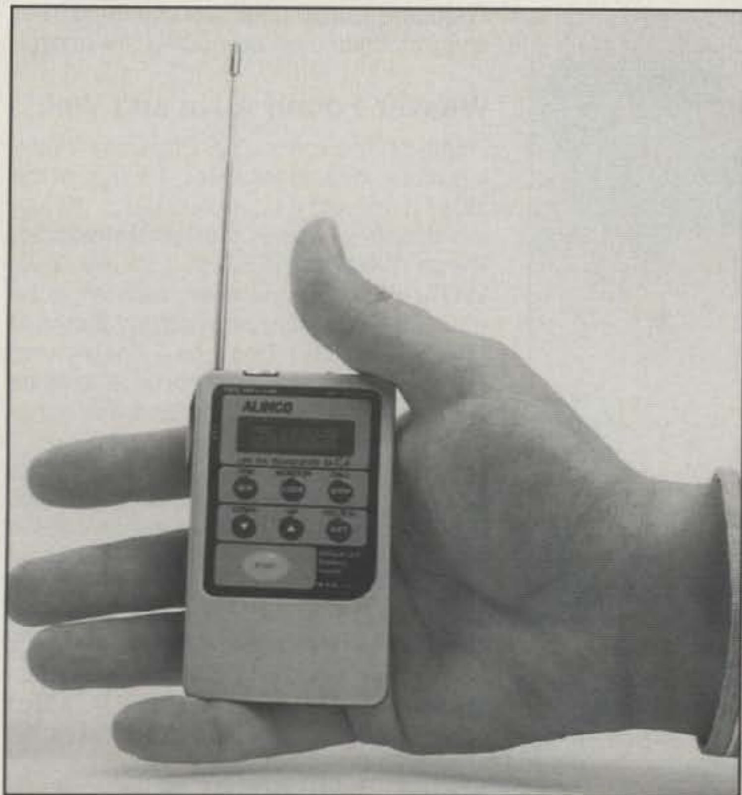
Photo D—Alinco's new micro-miniature, QRP-priced DJ-C1 two meter FM handheld. Unit is only three charge cards thick!
