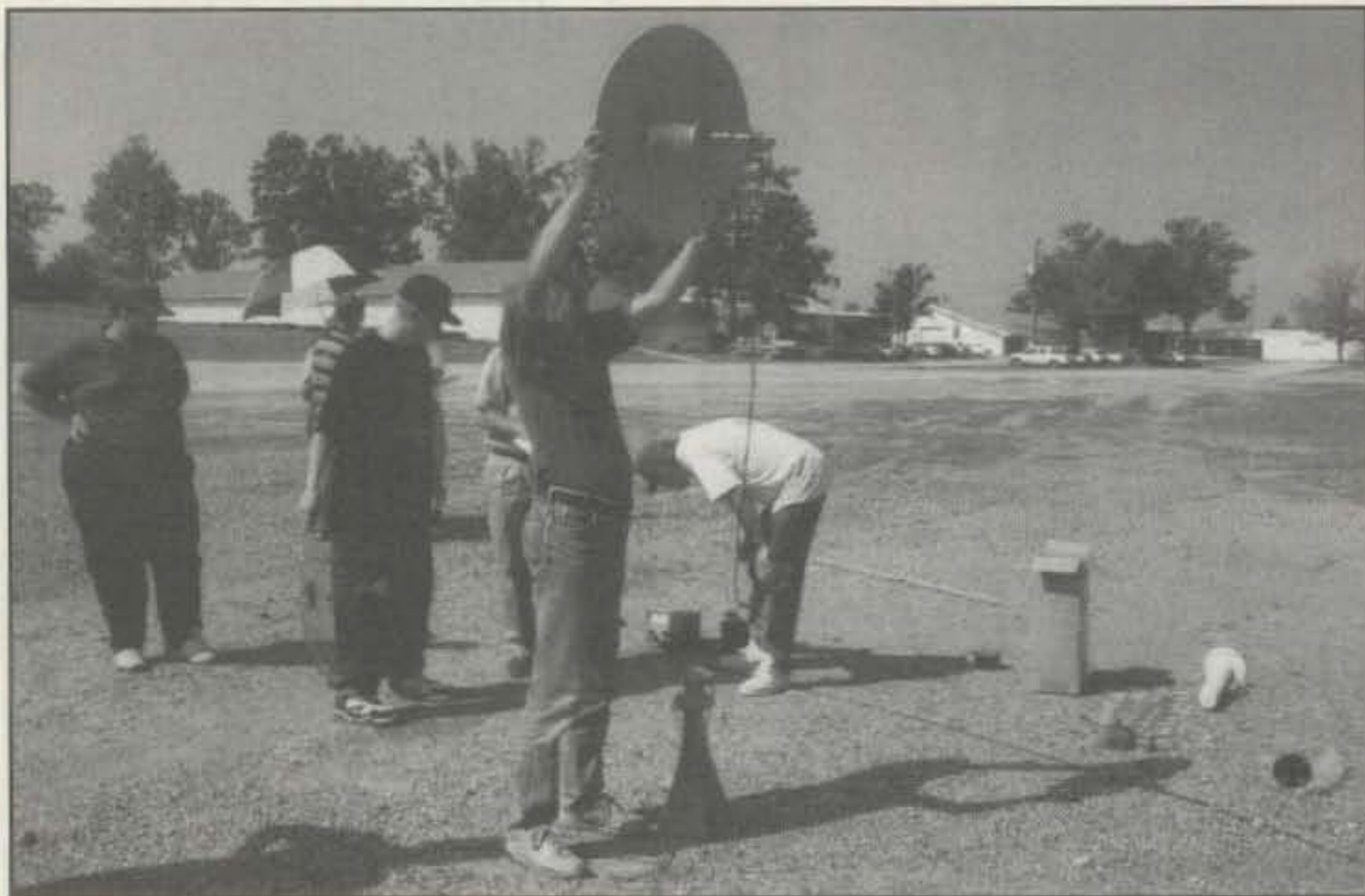
John Cress, KØGCJ, holds up a 2.3 GHz dish at the Central States antenna range, while Kent Britain, WA5VJB, bends over to read the gain measurement — +20 dBd.
