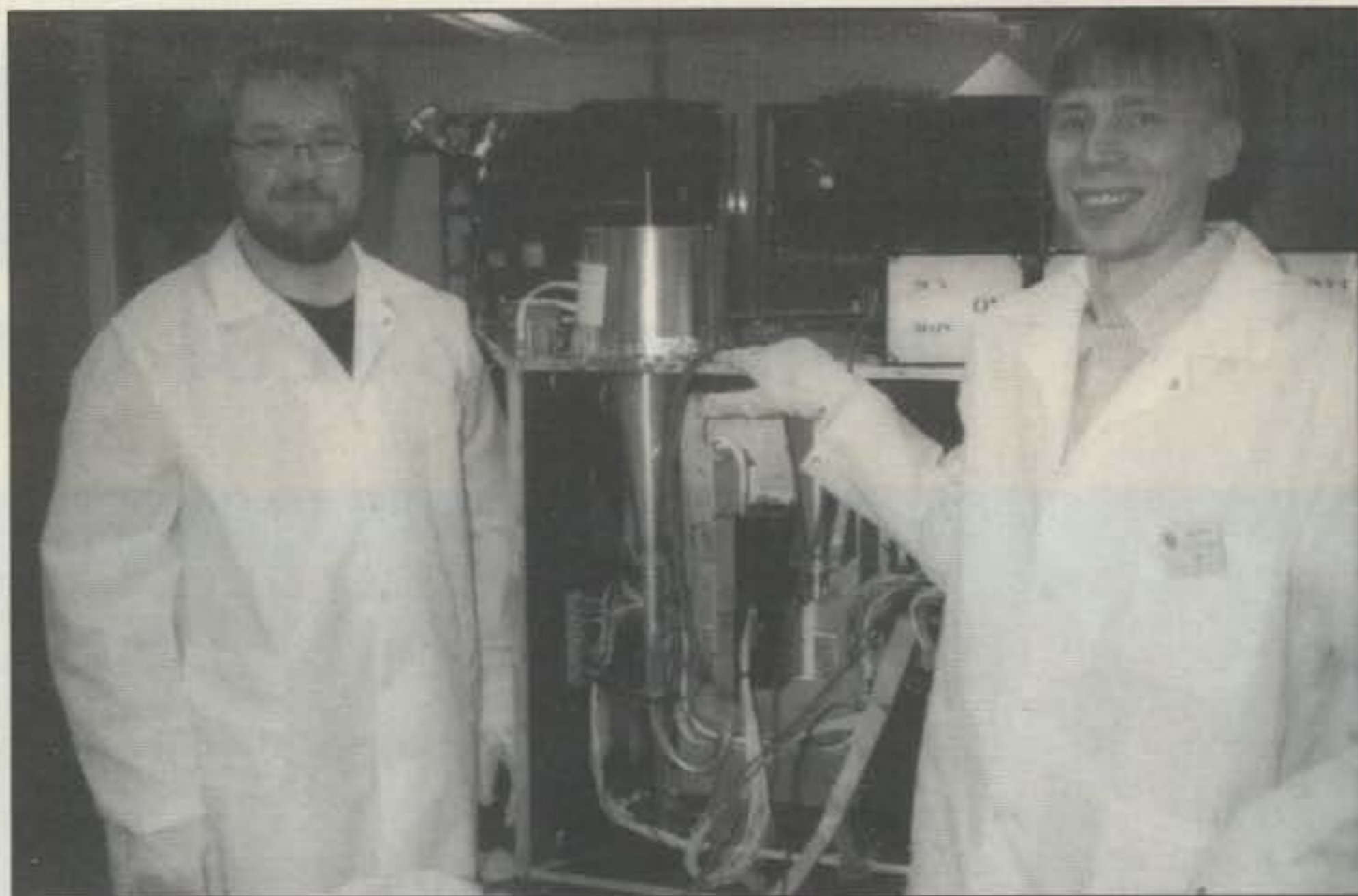
"Proud parents" Michael Fletcher, OH2AUE (left), and Harri Leskinen, OH2JMS (right), pause during testing of their AMSAT Phase 3D 10 GHz transmitter and traveling wave tube (TWT) amplifier at the P3D lab in Orlando, Florida. The TWT, procured by AMSAT-DL for the project, delivered a clean 60 watts output while installed in the spacecraft. AMSAT-NA Executive Vice President Keith Baker, KB1SF, adds that the "paint bucket" dummy load atop the 10 GHz feed horn worked well. He notes there's a block of carbon-impregnated concrete inside and stuck down into the horn's throat. The result was no leakage whatsoever, once they sealed the bottom with copper foil tape, providing a perfect match for testing. (AMSAT-NA photos courtesy Keith Baker, KB1SF)
