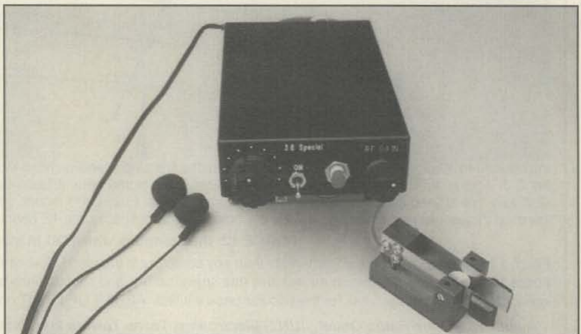
Photo B— Check out this collection of goodies, gang. The 38 Special transceiver kit, San Luis custom enclosure, internal Tick keyer, and miniature Paddlette yield a complete QRP station for less than $100. Even Monte Hall would appreciate a deal like that one!
