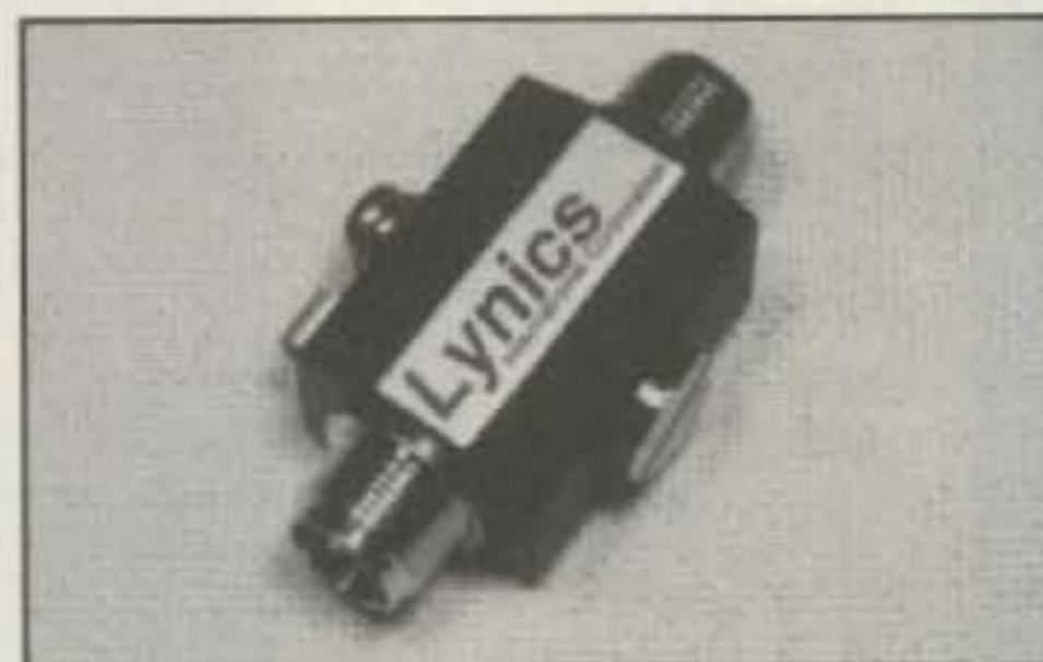
Lynics International offers commercial grade, UL-listed lightning protectors that incorporate an easily replaceable, tube-type arrester element. The devices are available four types. These include models in male/female (indoor) and female/female (outdoor) configurations, with either UHF or N connectors. Shown here is the No. 20206 female/female protector which uses N connectors. (Photo courtesy Lynics International, Inc.)
