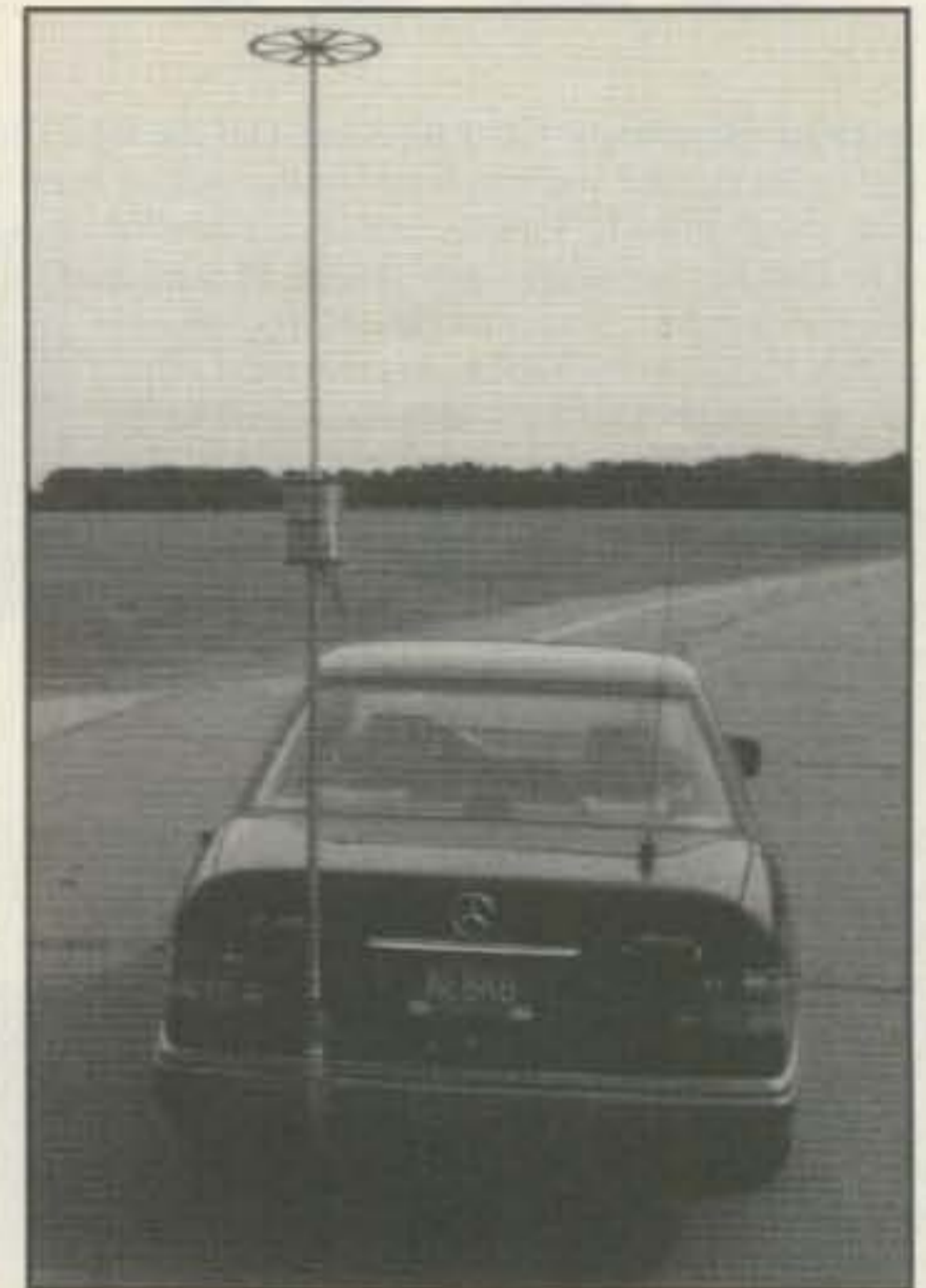
Fig. 2—Here is a trucker's-eye-view of the all-silver coiled, capacity-hatted Stealth antenna arrangement of Bill Becks, KE8KB. The setup pumps out a hefty signal and won first place in the 1997 Wisconsin Mobile Shootout.
