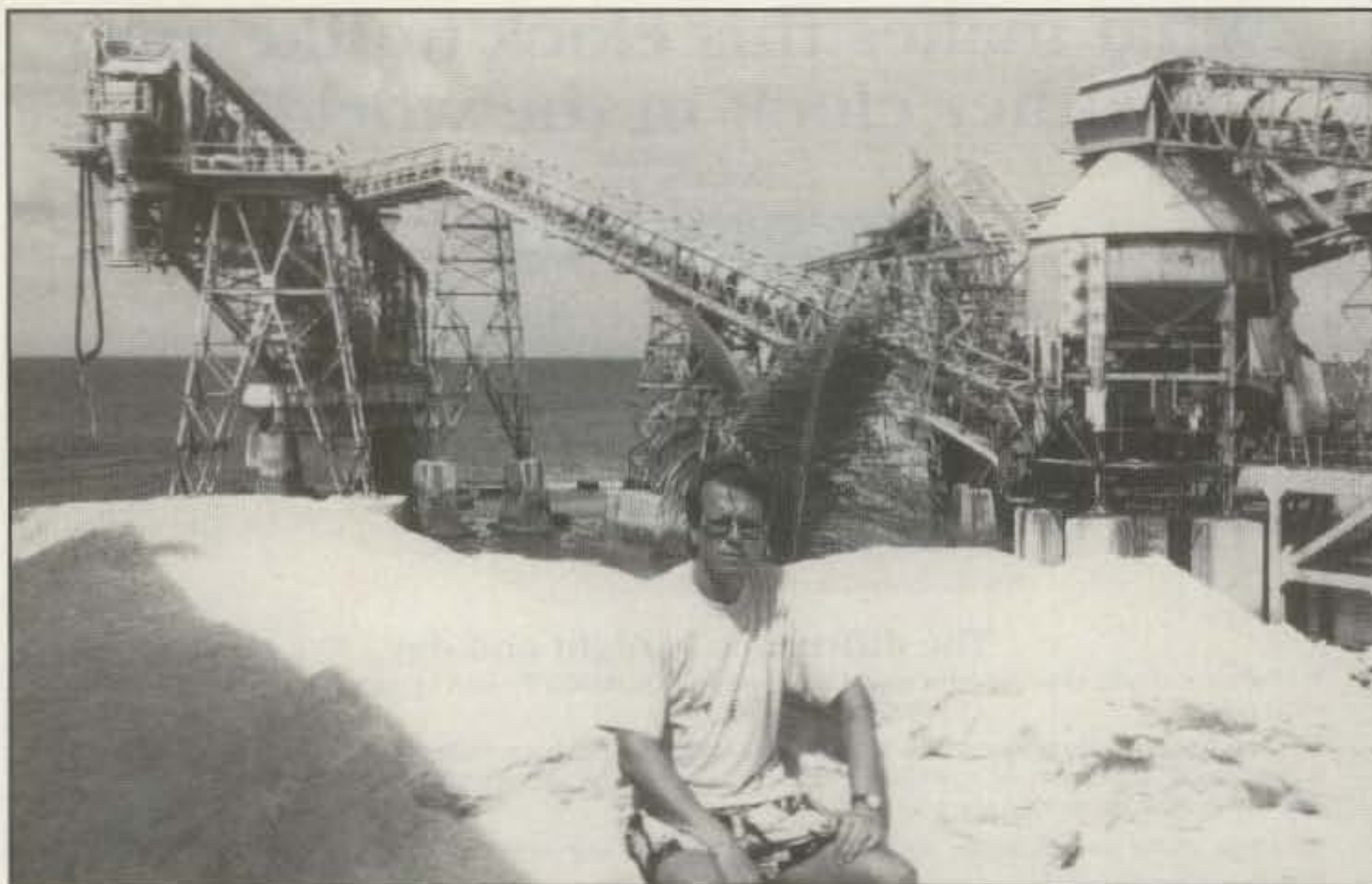
Pekka, OH1RY, at the loading dock. These conveyor belts are used to fill the freighters with crushed phosphate.
