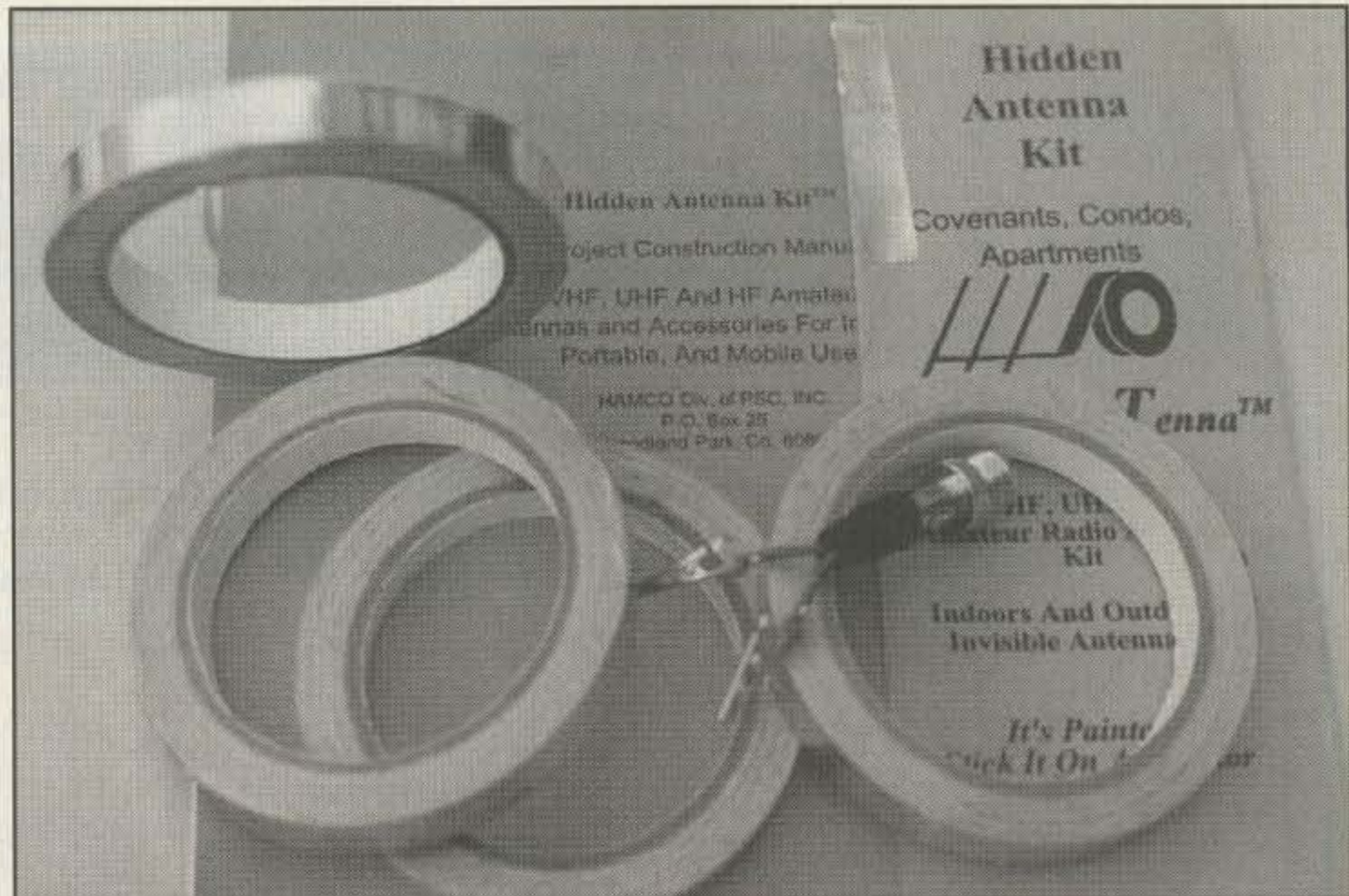
Fig. 4—The Tape Tenna made by Hamco makes an invisible stick-on antenna for low-profile hamming. Its adhesive copper strips also work great as a ground plane for modern composite-body cars as discussed in the text.
