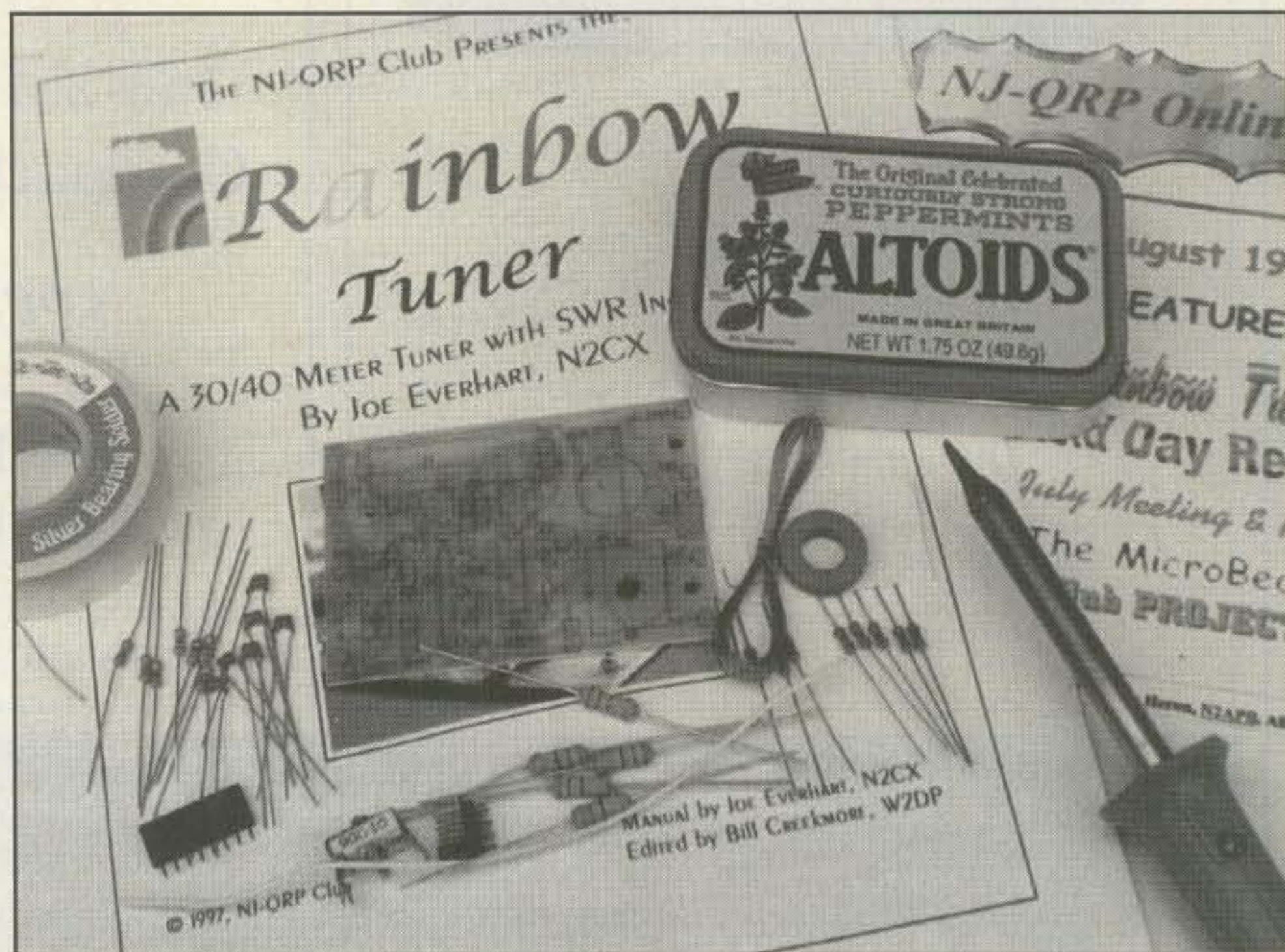
Fig. 5—The Rainbow Tuner kit as received and laid out ready for construction. The manual's step-by-step instructions plus silk-screened component layout on the board make assembly a snap.
