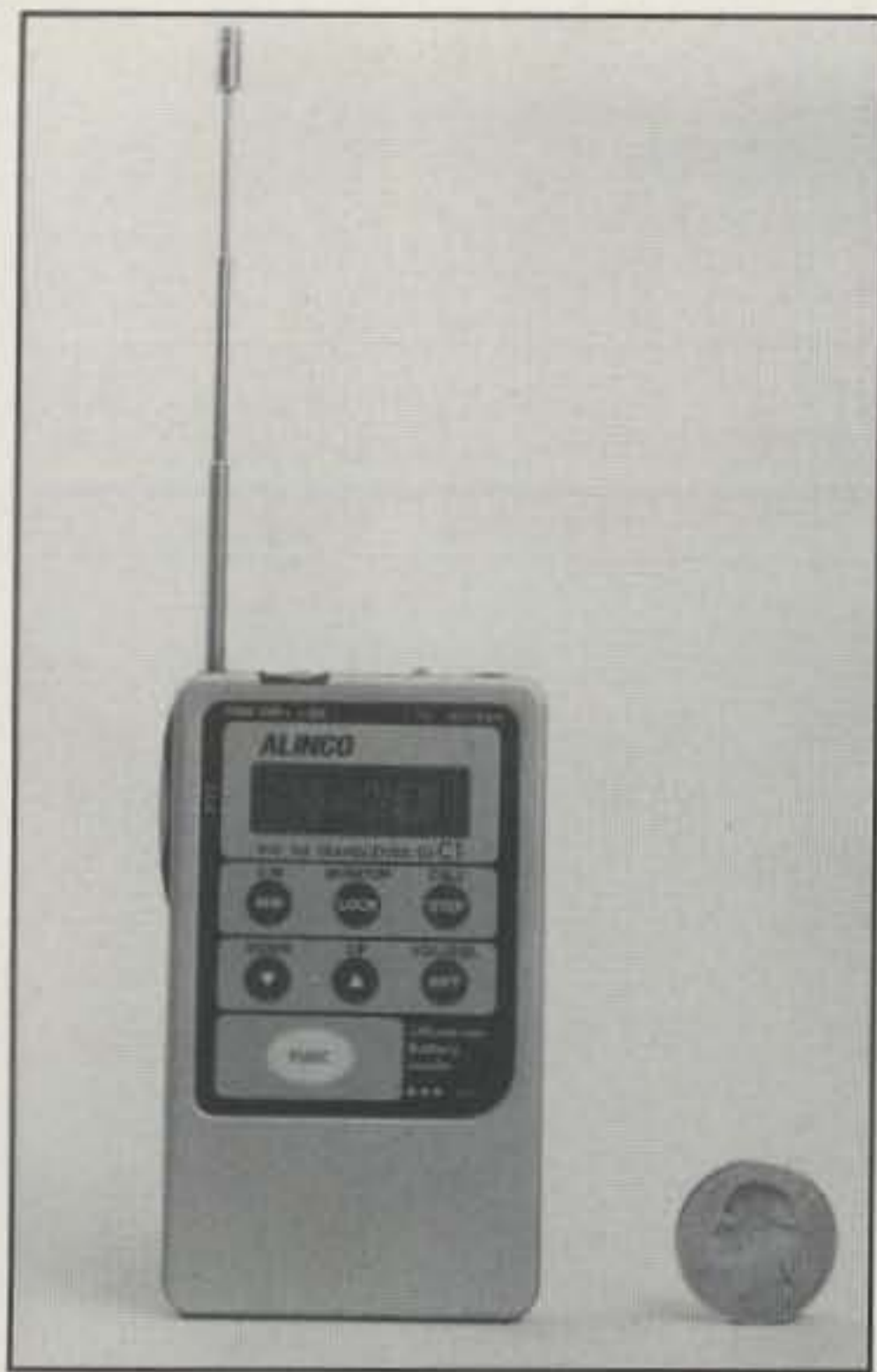
Photo 9—Possibly the hottest item of the year is Alinco's DJ-C1 microminiature 2 meter FM handheld transceiver. This talkie measures only 3.6"H x 2"W x .3"D. Even James Bond would envy this gem!
