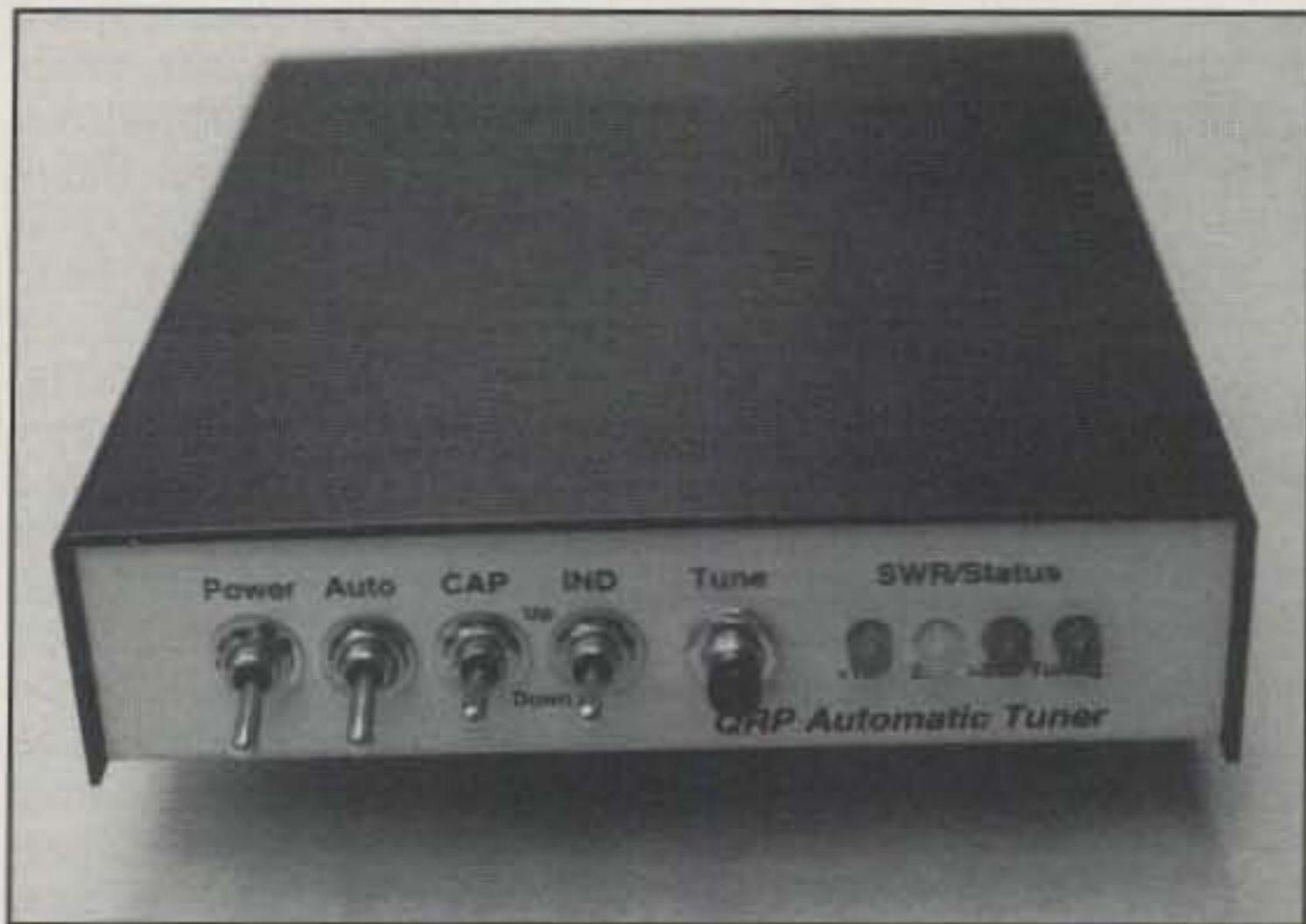
Photo 3— This ultra-compact Automatic Antenna Tuner from LDG Electronics is available in kit or preassembled form and in QRP or 100 watt versions. The tuner uses a switched "L" network, has a built-in SWR bridge, and is ideal for home, portable, and/or mobile operation.
