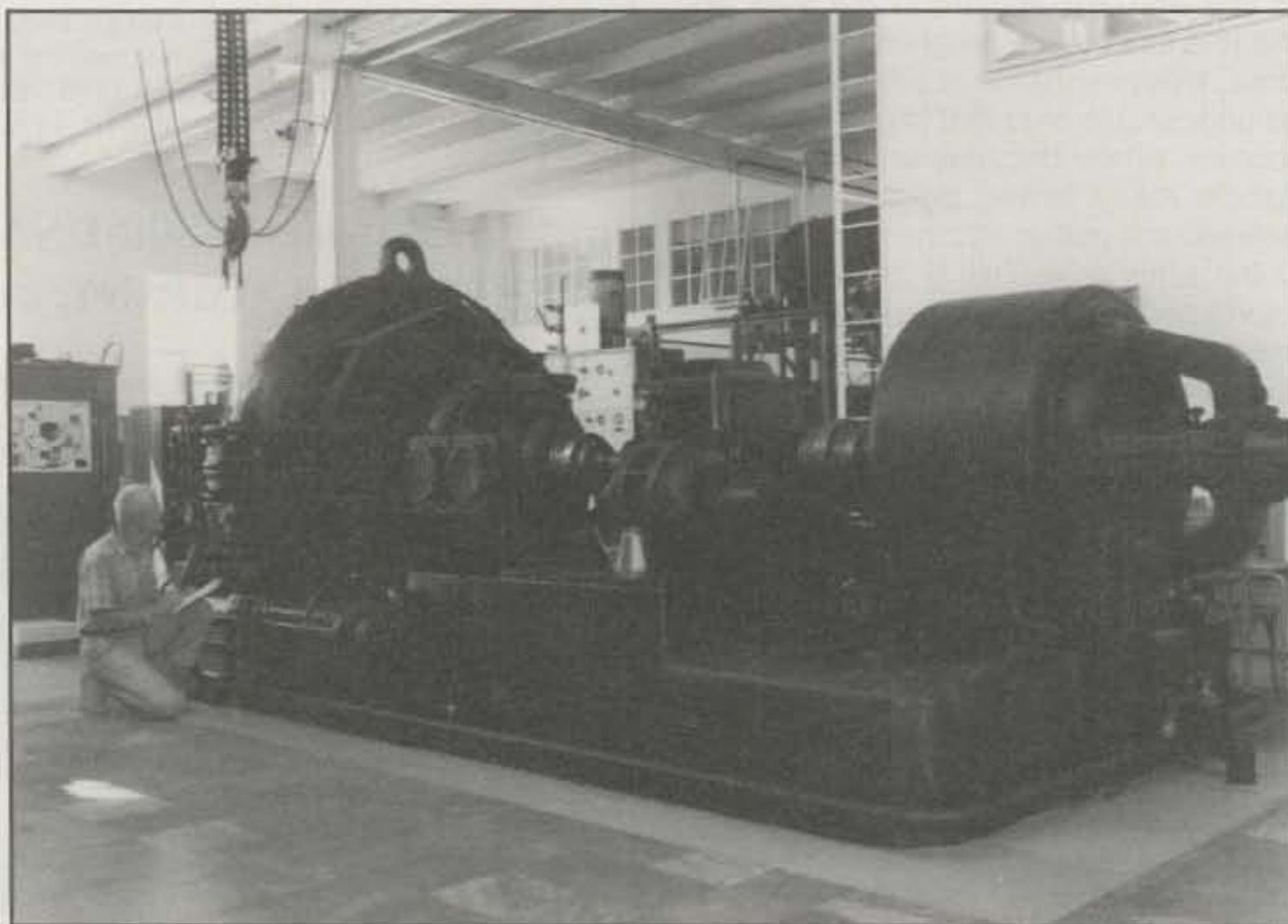
Alexanderson alternators were built by General Electric and RCA in the 1920s; only one is left. The device is a large, electromechanical high-frequency alternator with a high-speed rotor connected directly to an antenna. The only working station, at Grimeton, Sweden (shown here) broadcasts on ceremonial occasions on 17.2 kHz. (Photo courtesy Telia AB, Sweden)
