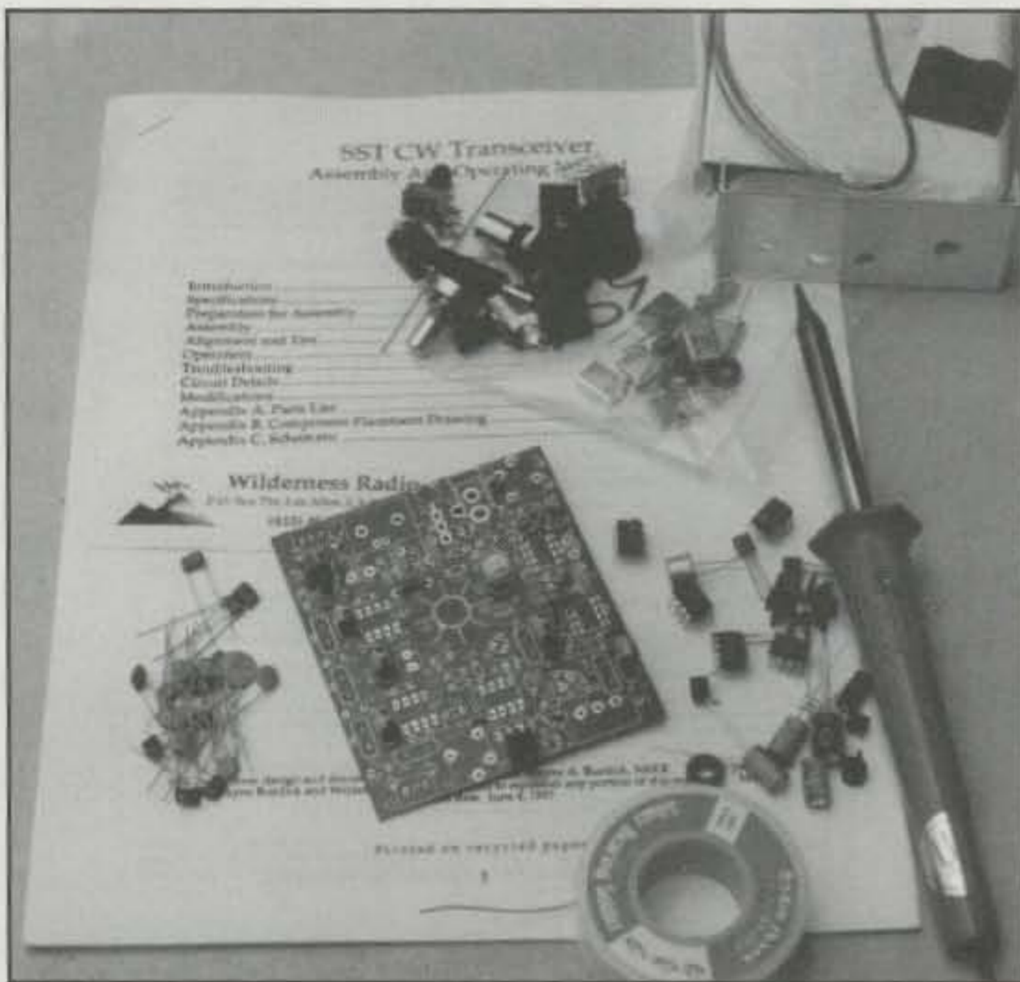
Photo 3— The SST kit as received and ready for assembly. Truthfully, I was over-enthusiastic and almost forgot to shoot this “45 minutes into construction” photo. Disc capacitors are at the 7 o'clock position; connectors, controls, crystals, and components for a selected band are at 12 noon; solid-state devices are at 3 o'clock; and electrolytics are at 5 o'clock.
