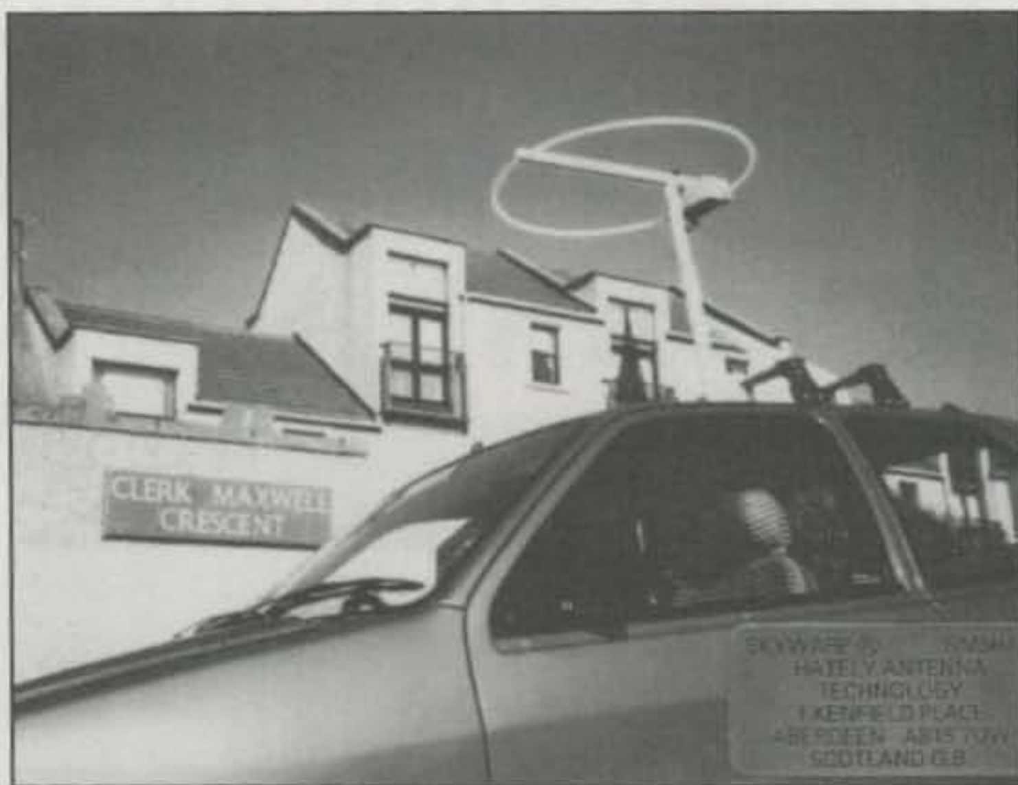
The same compact Hately CFL 1 Crossed Field Loop antenna can be used as a mobile (shown here) or maritime station antenna where compactness is highly desirable. (Photo courtesy Hately Antenna Technology)
