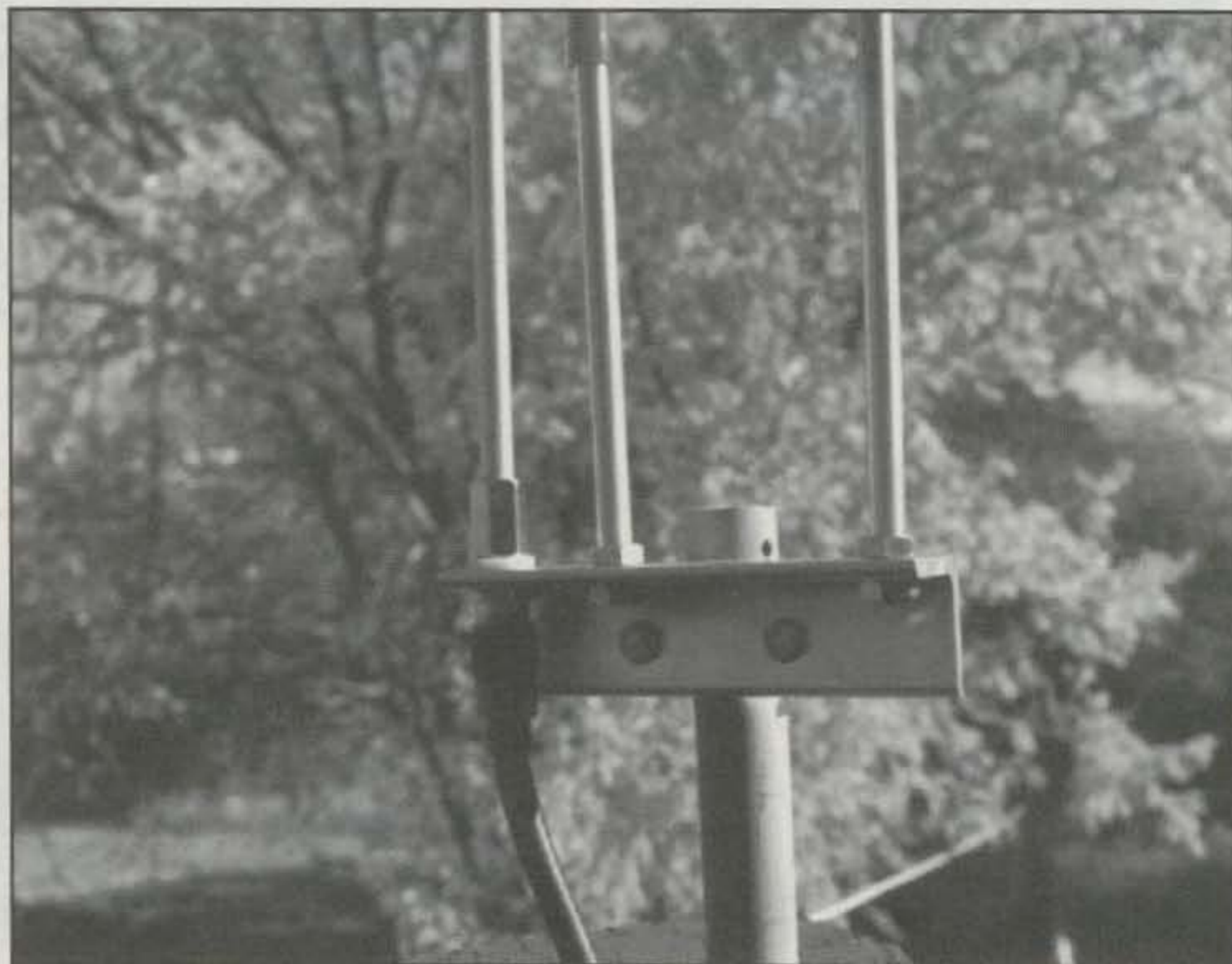
This is a close-up of the base mounting of the Arrow J pole. The feed goes to the section on the left. The base design is really outstanding. Standing wave checks showed that my Bird wattmeter never left 1.2 to 1 across the entire 2 meter and 450 MHz bands. This is a very fine performing antenna.
