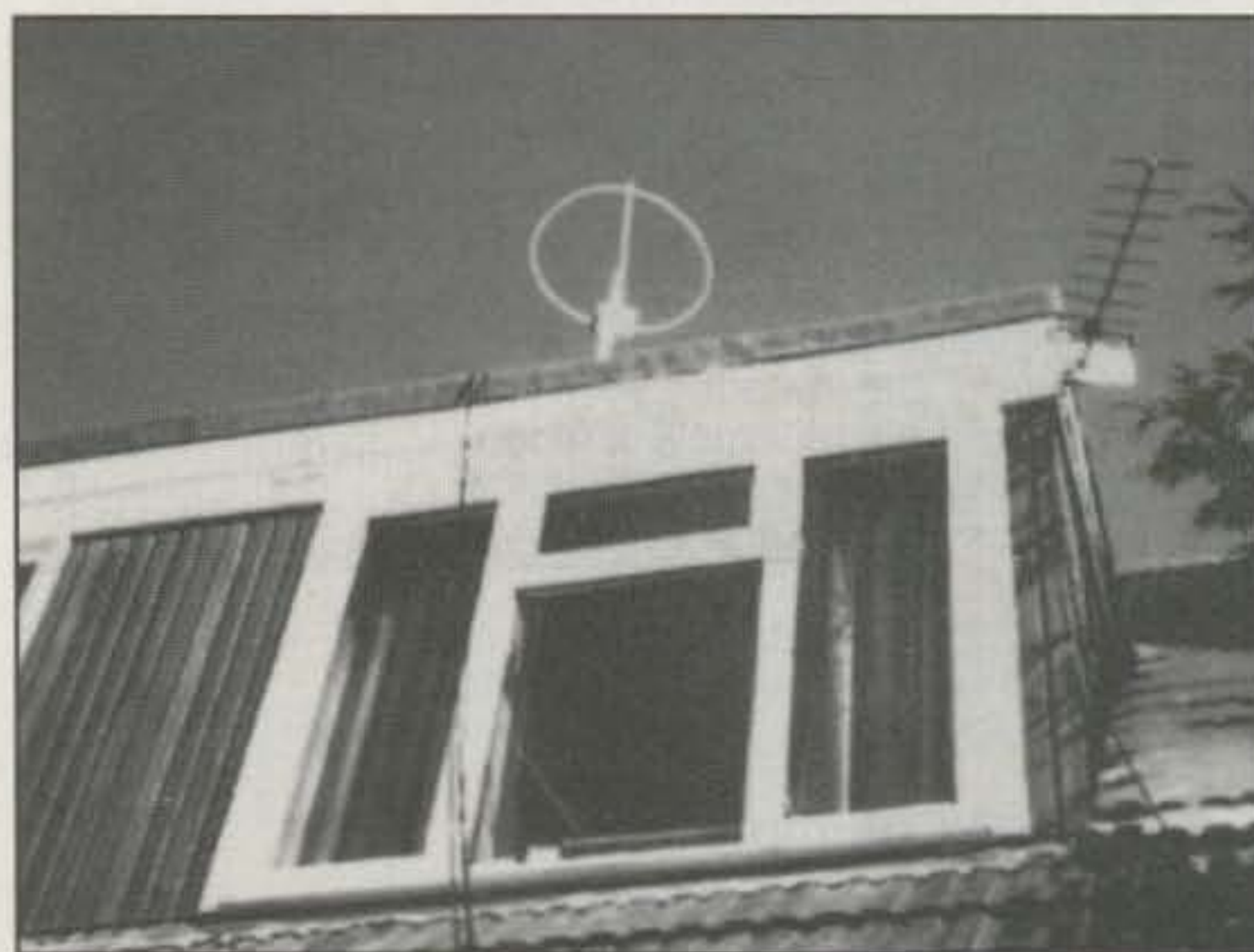
The Hately CFL 1 Crossed Field Loop Antenna is a compact antenna designed specifically for use at restricted sites or on vehicles or boats. The antenna depends on the principle of "Pointing Vector Synthesis," a complex, patented process explained in detail in the Hately product literature. The broadband CFL 1 system, which covers 160 through 10 meters, is described in the text of this month's column. The antenna is shown here in a typical fixed-station installation. (Photo courtesy Hately Antenna Technology)
