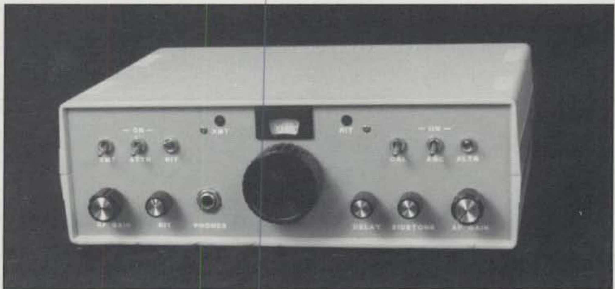
The finished project—the QRP 30 Plus compact 30 meter transceiver.
