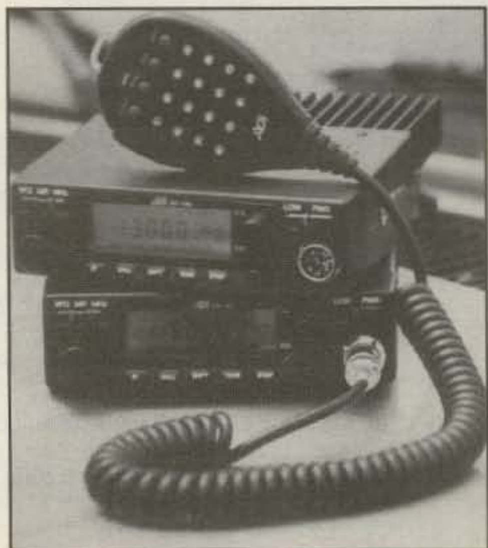
The AR-146 (bottom) and the AR-446 (top). All you need is an antenna and 12+ volts of power.
