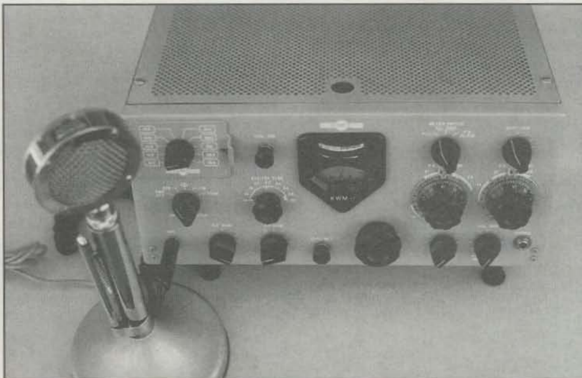
Photo 3— Reliability during the most unusual situations is another important factor in survival communications, and the stoutheartedness of older vacuum-tube gear may prove beneficial for withstanding indirect effects of EMP radiation.
