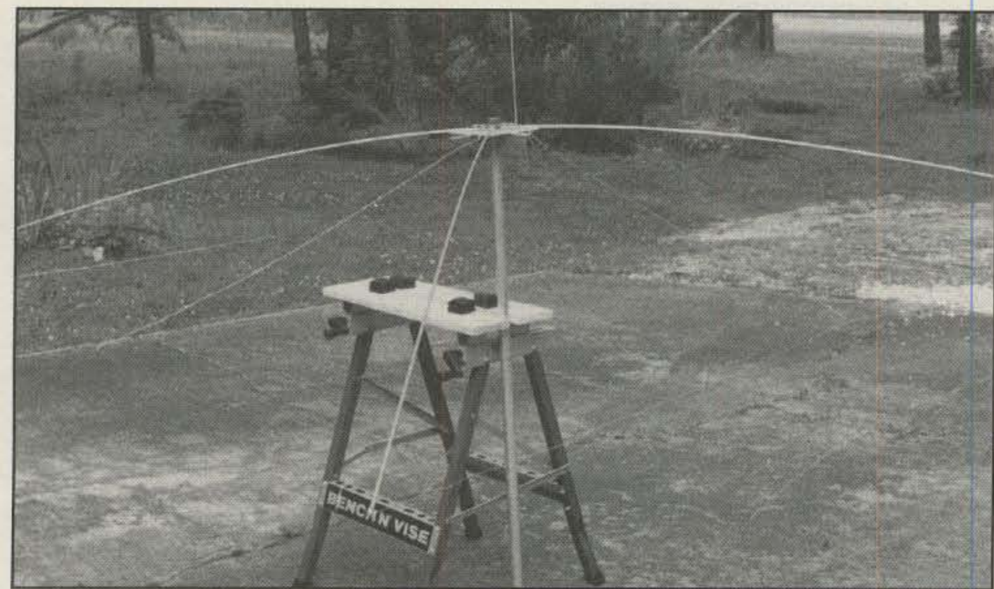
Having a test jig, such as shown, makes assembly easier.
