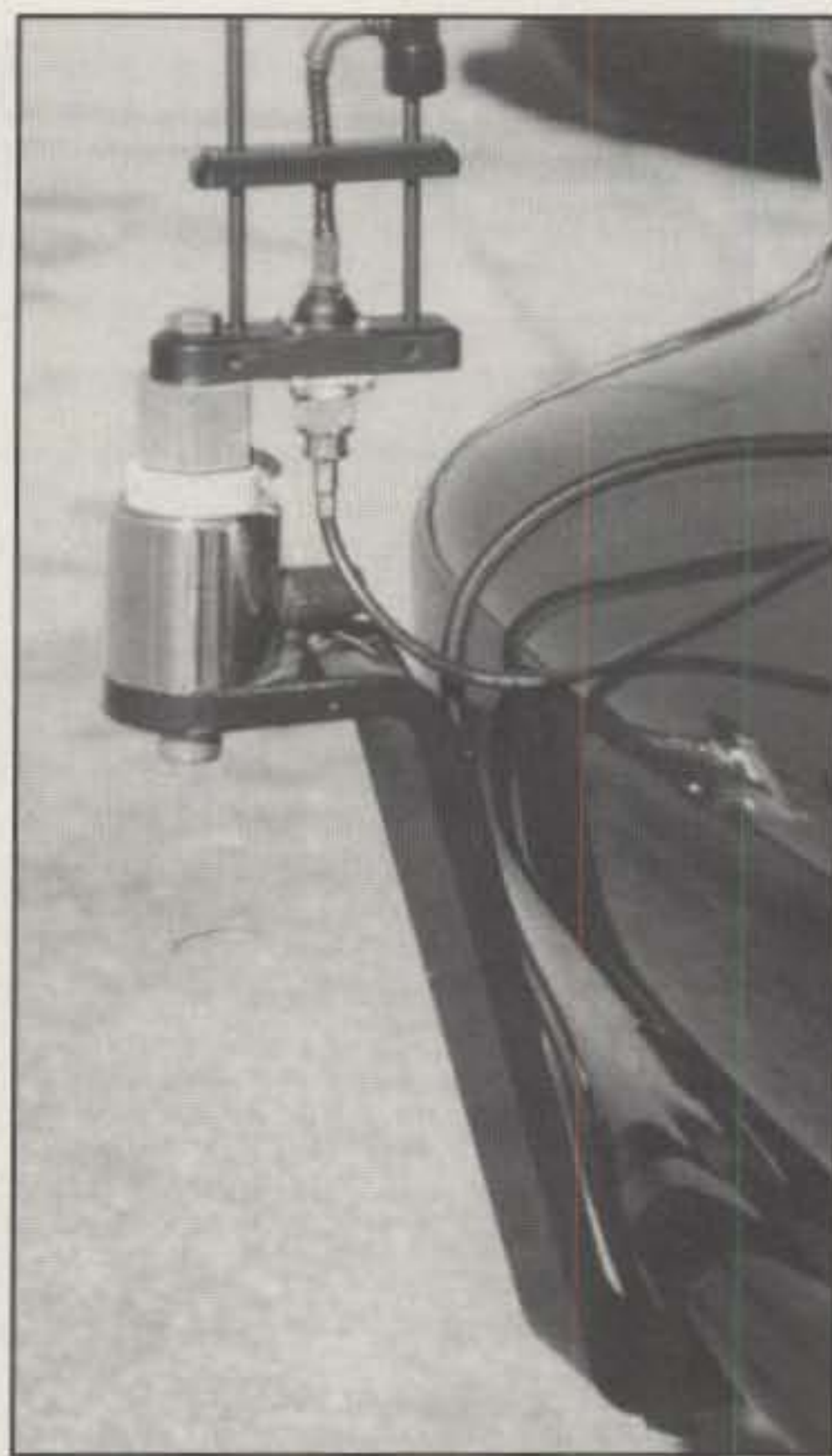
Photo 6— Close-up view of the base-mounting assembly and coax-connection method on the Rocky Mountain JP-2M antenna. Bolts for fitting the antenna into the mount are supplied.
