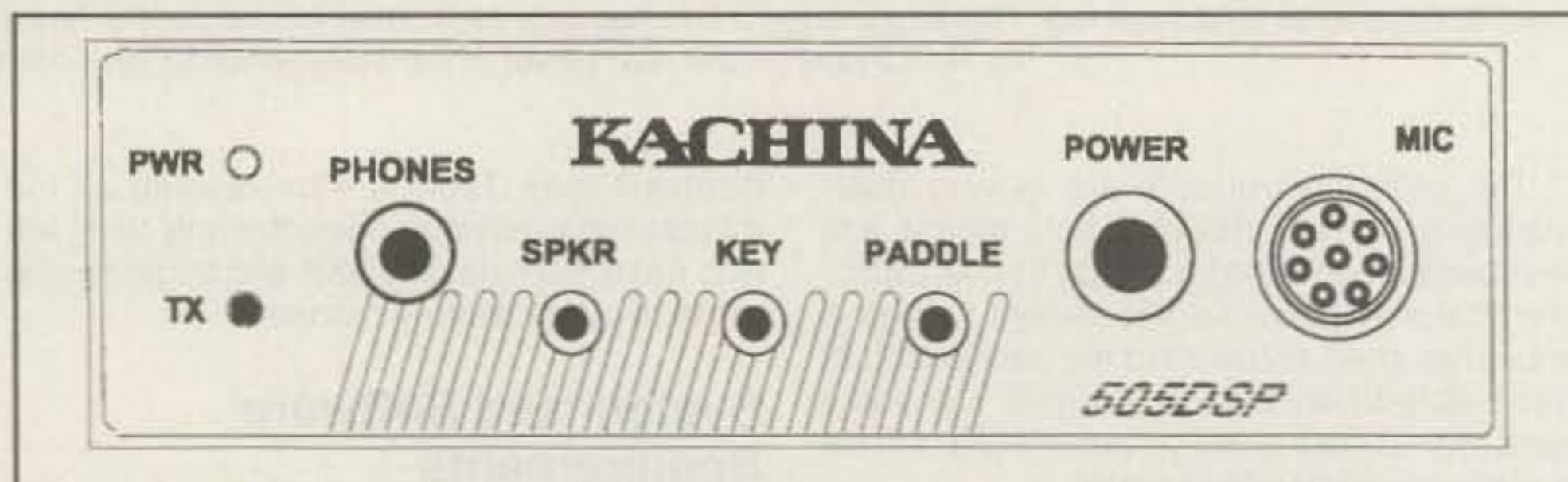
Fig. 4—The ON/OFF switch is the only moving part you'll be concerned with. Control is via the mouse and the onscreen menu. If you prefer, keyboard entry/control is an immediate option. The 505DSP is supplied with a control head containing the main power switch and microphone, speaker, Morse key, and phone jacks.
