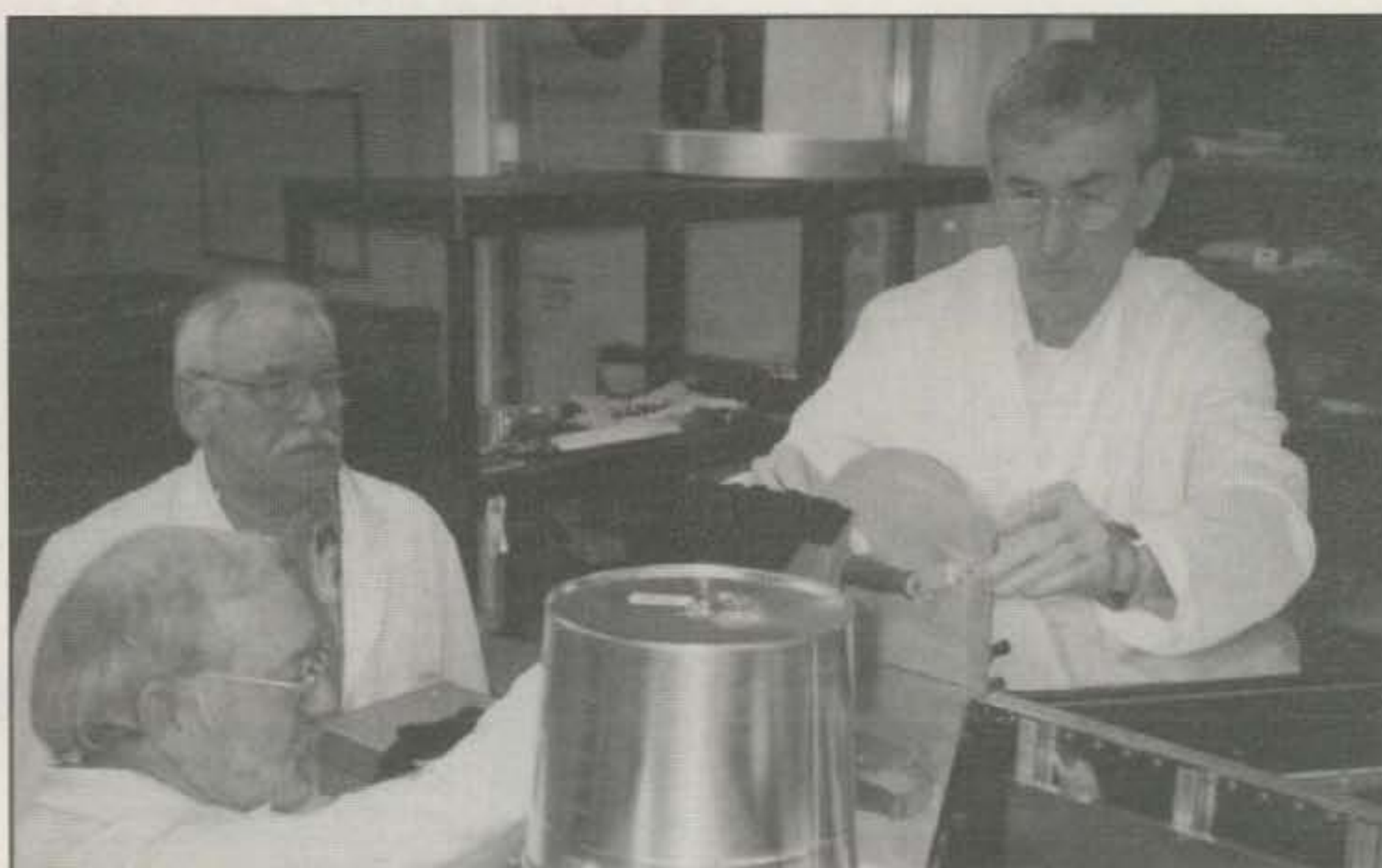
AMSAT-NA's VP of Engineering, Stan Wood, WA4NFY (right), uses a machinist's level to precisely balance the Phase 3-D spacecraft in its construction cradle while Lou McFadin, W5DID, P3-D Integration Laboratory Manager (far left) and Konrad Mueller, DG7FDQ, AMSAT-DL's Structural Specialist, assist. The "upside down paint bucket" on the top of the spacecraft is a dummy load that covers the opening on one of Phase 3-D's 10 GHz horn antennas during testing.
