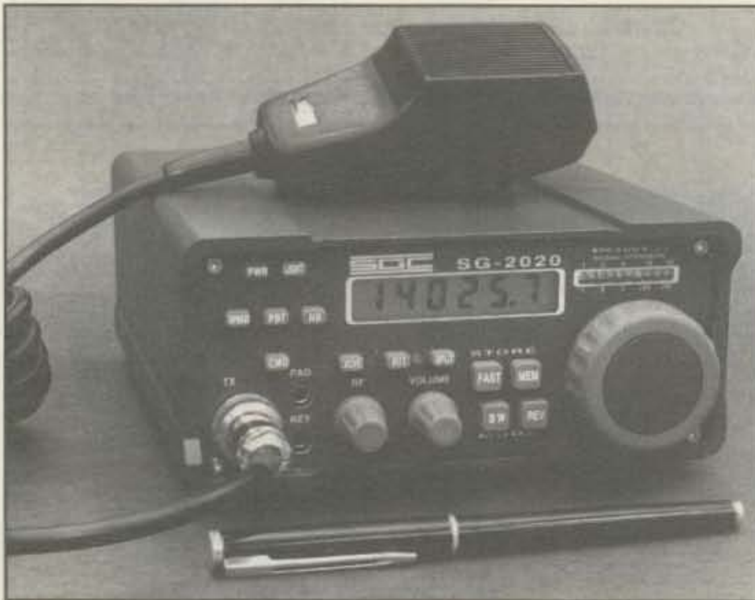
Photo 1— (Top Left) The new SGC SG-2020 HF transceiver. Unit is quite small, remarkably similar to the QRP Plus in design and operation, and packs a hefty punch on both CW and SSB. (Photo courtesy SGC, Inc.)
