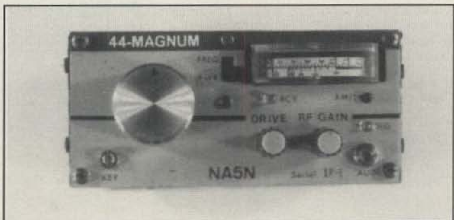
Photo 5— (Below) Although an enclosure is not included in the basic 44 Magnum kit, this front view of the NA5N prototype unit gives us a good idea of how a completed transceiver might look. (Photo courtesy NA5N)
