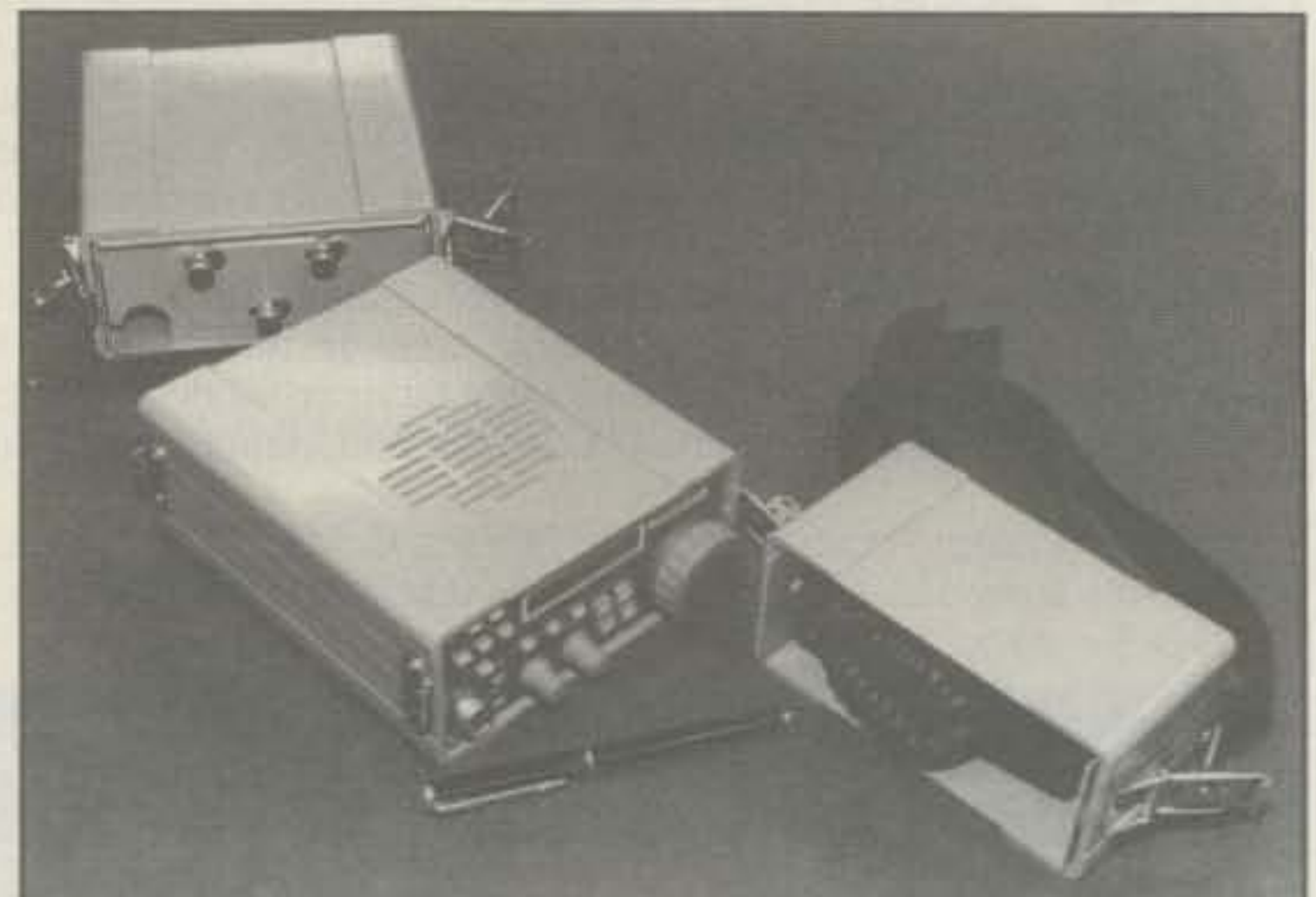
Photo 1— (Top Left) The new SGC SG-2020 HF transceiver. Unit is quite small, remarkably similar to the QRP Plus in design and operation, and packs a hefty punch on both CW and SSB. (Photo courtesy SGC, Inc.)
