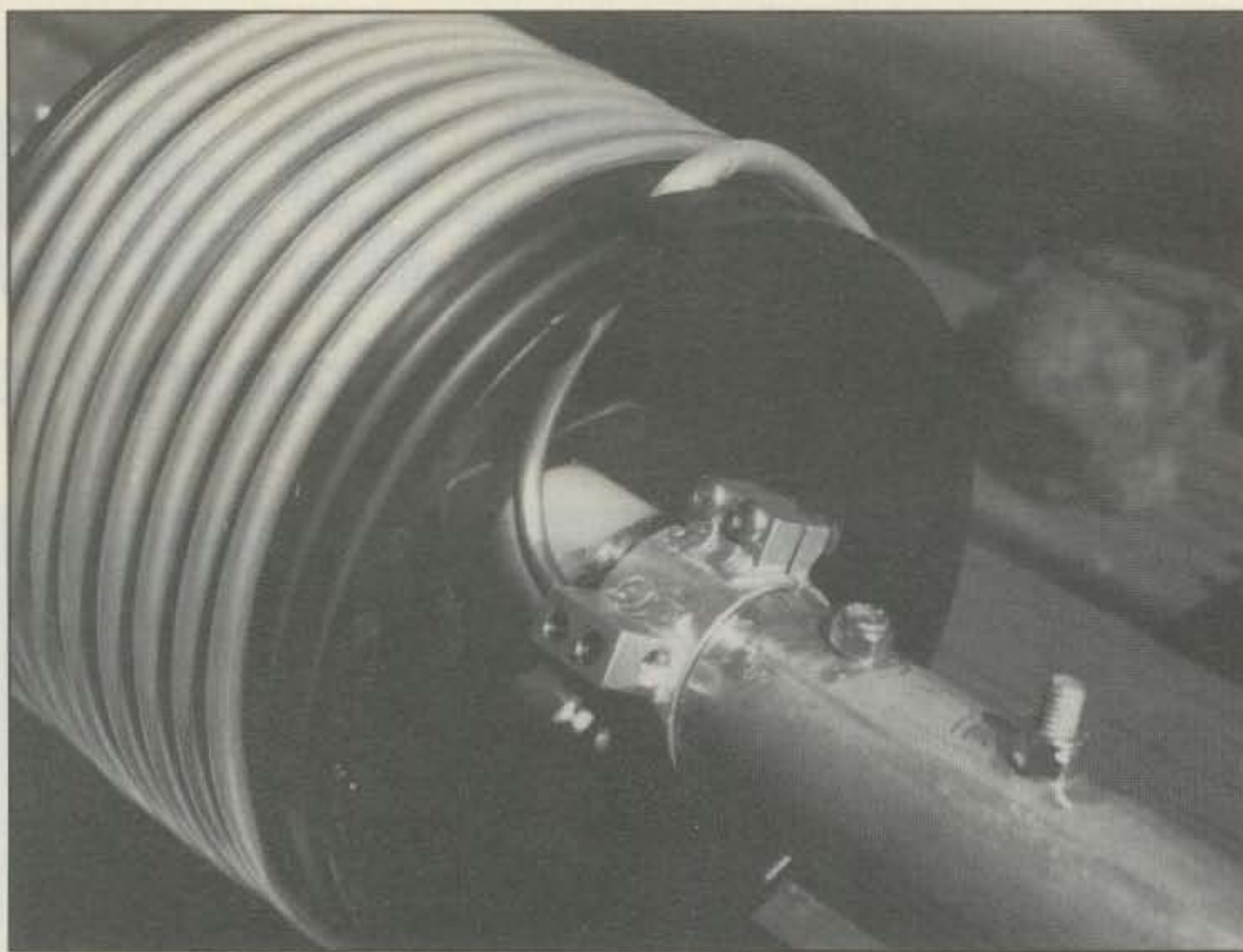
Close-up detail of the coil and mounting hardware.
