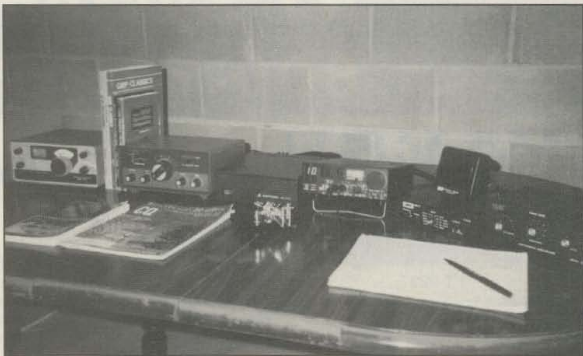
Photo 8— All QRP and proud of it! This neat setup of John Peregord, Jr., KB8UMD, sports a classic Heath HW-8 and HW-9 plus Ten-Tec QRP Scout, DSP, and antenna tuner. Now who could resist sitting down to a station like this! (Photo courtesy KB8UMD)
