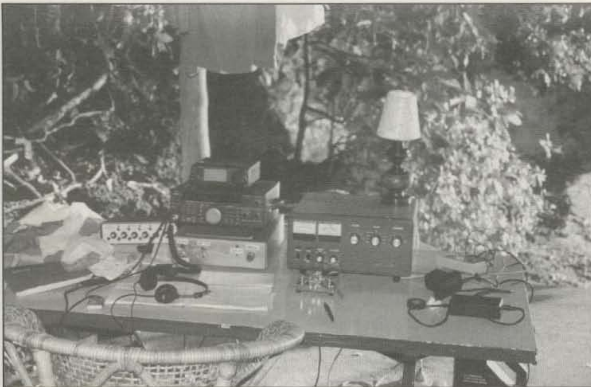
The H40AB station: TS-690S, IC-706 MKII, FL-2100Z, MFJ keyer, etc.
