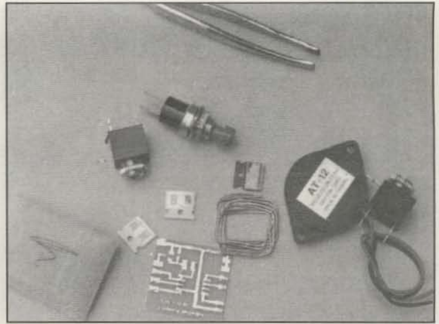
Photo 5— The Embedded Research Tick Keyer ready for assembly. Notice the PC board is barely larger than a pushbutton or paddle socket. The component in the wrapper on the left is the Tick IC. (Double capacitors, resistors, and transistors (above PC board) are included for soldering practice or as quick replacements if one is dropped and lost. (Discussion in text.)
