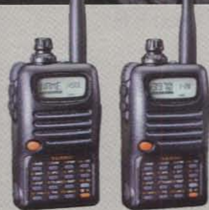
FT-10/40R Ultra Compact Handhelds VHF or UHF. Similar to FT-50RD including MIL-STD 810, and other exclusive features.
