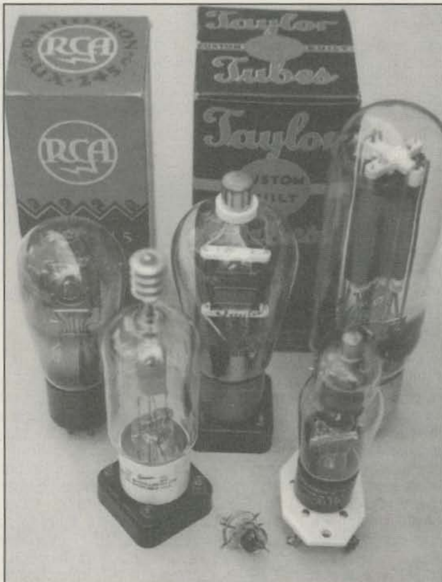
Fig. 1—Starting your own mini-collection of classic vacuum tubes is easy, fun, and most heartwarming. Further, special tubes in a well-planned collection can occasionally be used in past-era gear for an extra treat. Tubes shown here are a tall 211A "50 watter," famous Taylor T-20, RCA 245, Western Electric 311B, Eimac 3ST, and a tiny 956 "acorn tube." (Details in text.)
