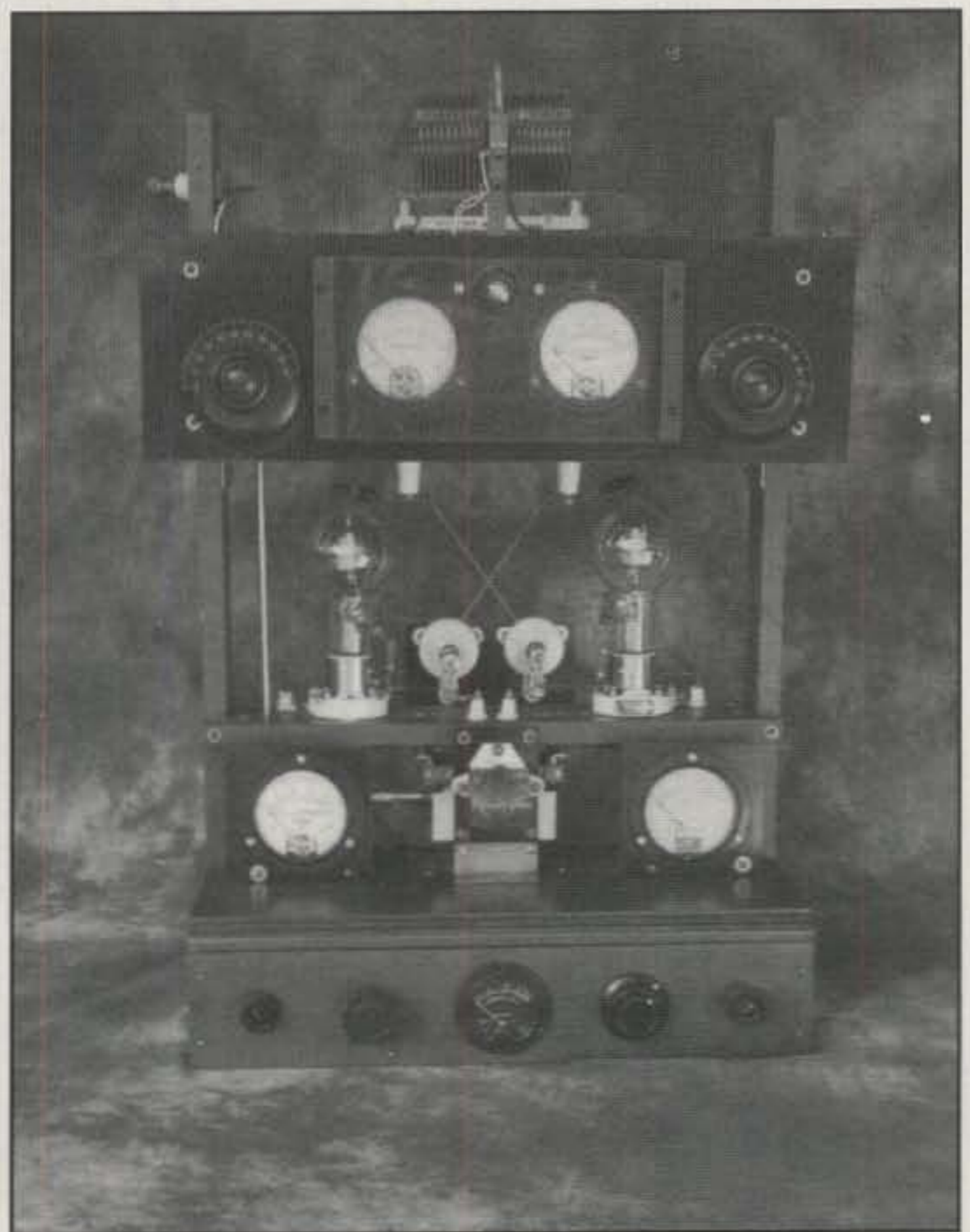
Fig. 5— My own 35T replica transmitter during assembly. I should have used a larger baseboard, but this one was beautifully finished and gave it a sort of "busy look" like a classic Bike Racer bug. Antenna loading capacitor and wattmeter for tuning are external to transmitter. Now this critter really looks like a rig!
