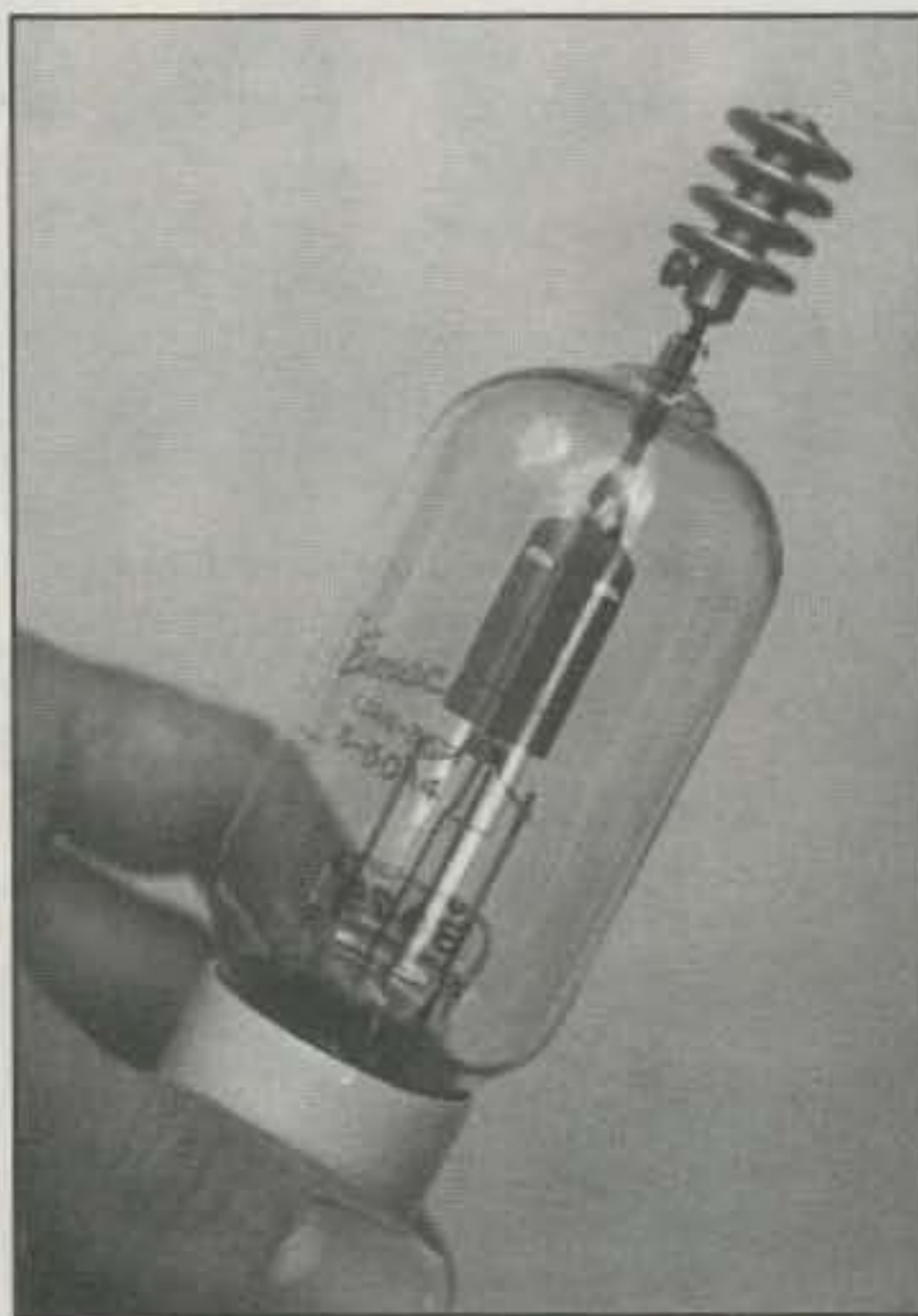
Fig. 1—The eye-catching and attention-grabbing Eimac 35T tube. This little gem stands 4.7 inches tall, is 1.7 inches in diameter, and has a 4-pin base the size of a UX-210 or 245. The tube is also double numbered as 3-50A4. (See profile of this classic in text.)
