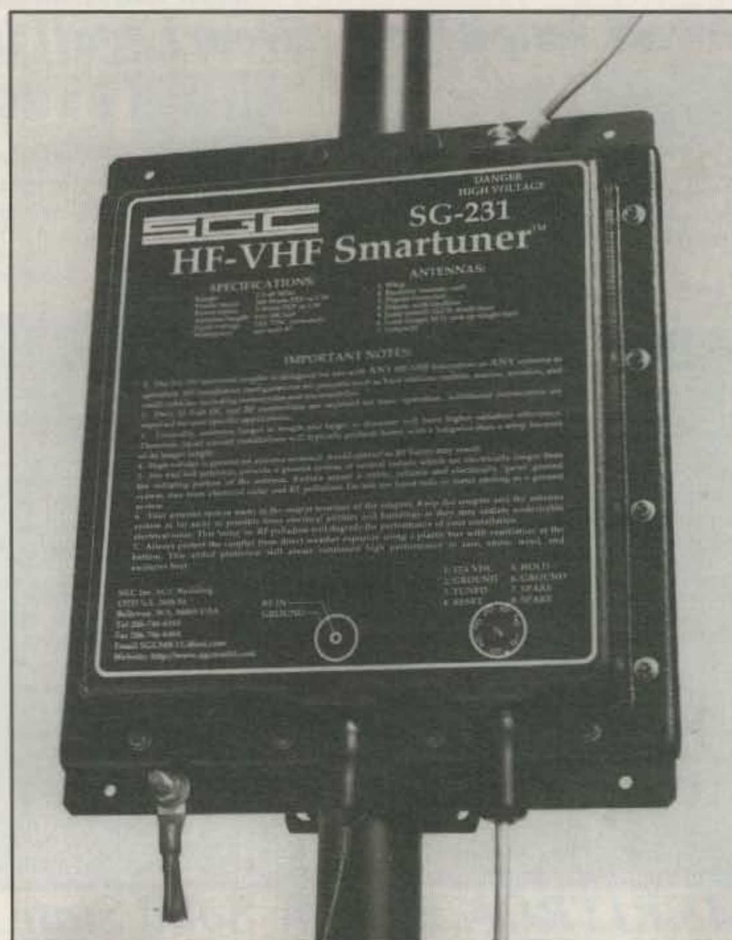
The SGC-231 Smartuner, a microprocessor-controlled automatic antenna coupler.
