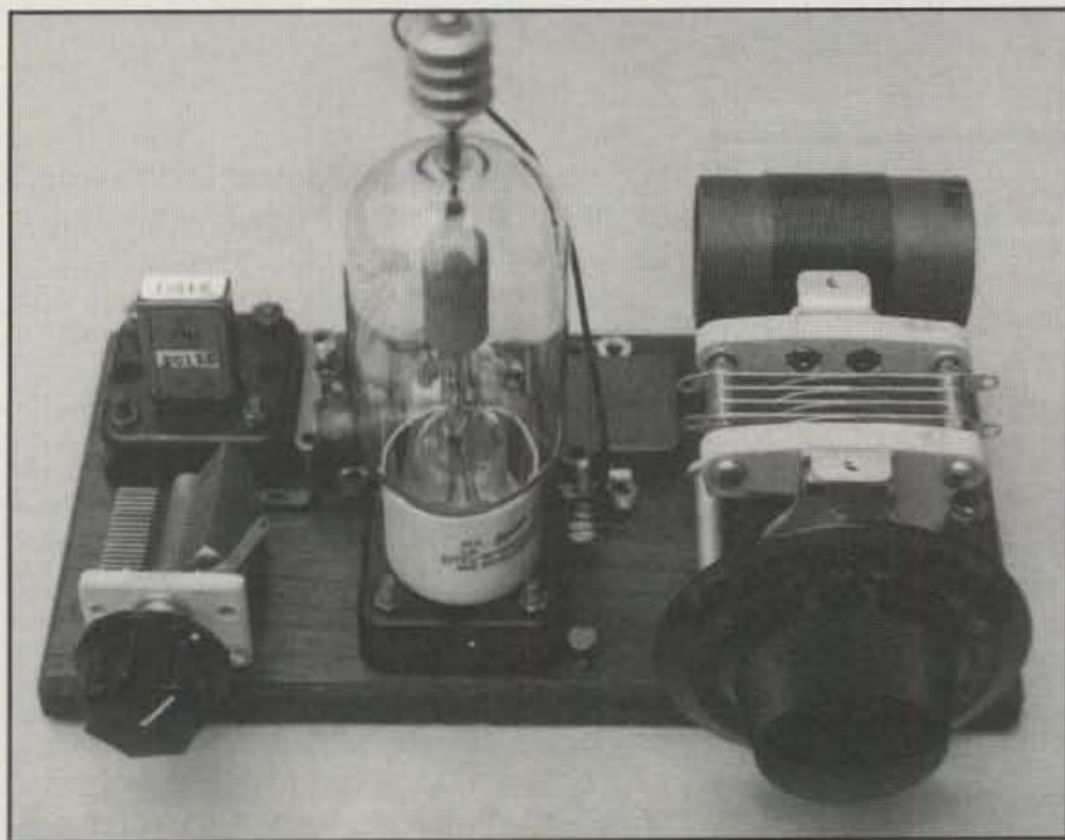
Fig. 5— My own 35T replica transmitter during assembly. I should have used a larger baseboard, but this one was beautifully finished and gave it a sort of "busy look" like a classic Bike Racer bug. Antenna loading capacitor and wattmeter for tuning are external to transmitter. Now this critter really looks like a rig!
