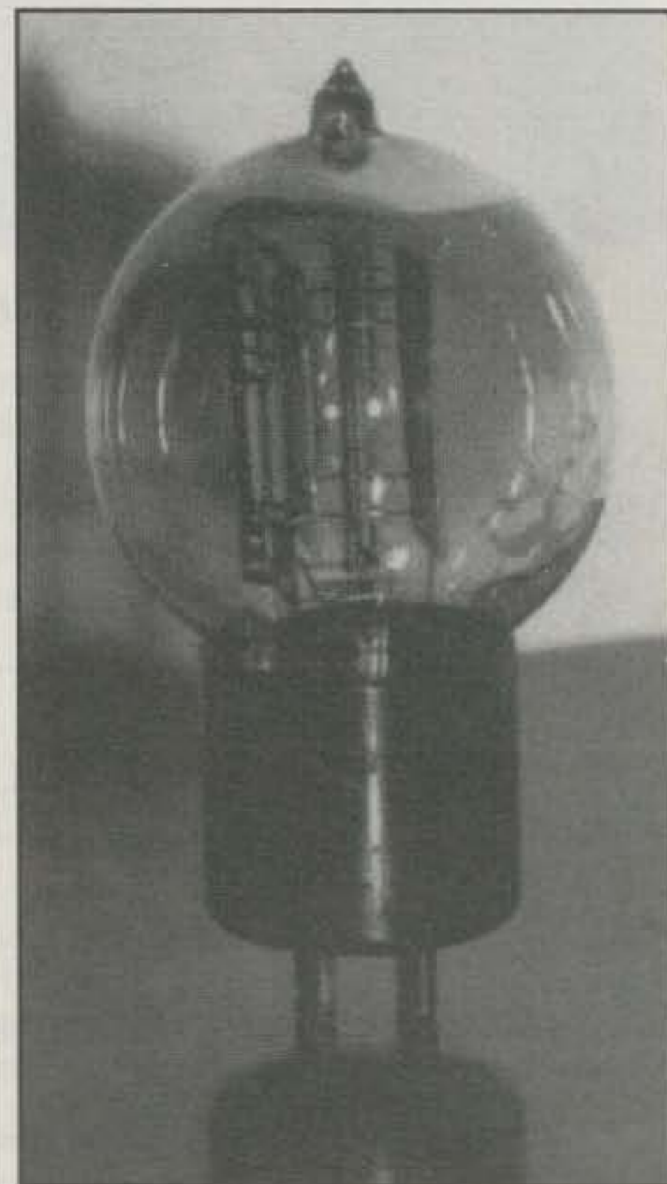
Fig. 10— Okay, friends and fans of QRP, check out this low-power dream triode of yesteryear. It is a unique WE-205D "tennis ball" tube, and it makes a neat "switch hitter" for UX-199s or 210s in old-style Hartleys or TNTs. Magnificent!
