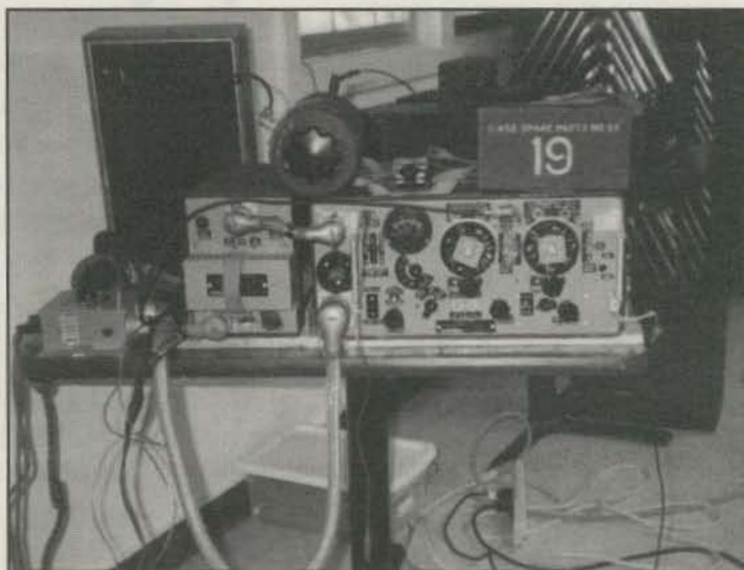
A complete WS-19 operating on 12 VDC ready to go.
