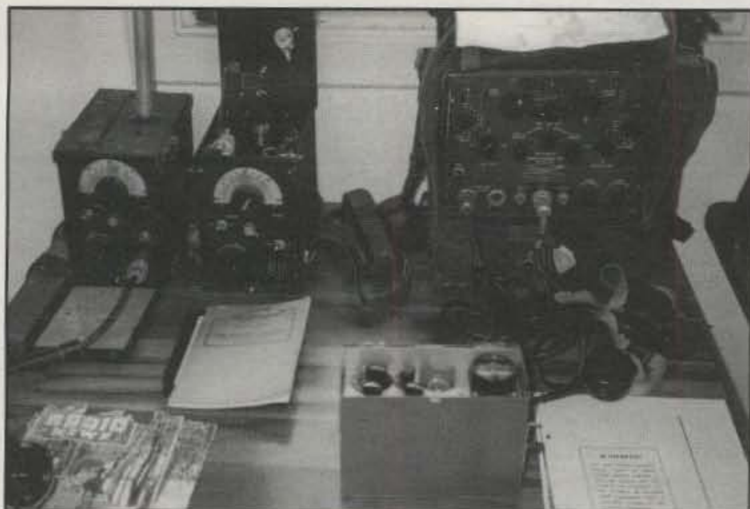
Shown in the upper left is a pair of TBX-5 transceivers with a TBY to the right. In front of them is a Japanese 30-40 MHz field set.
