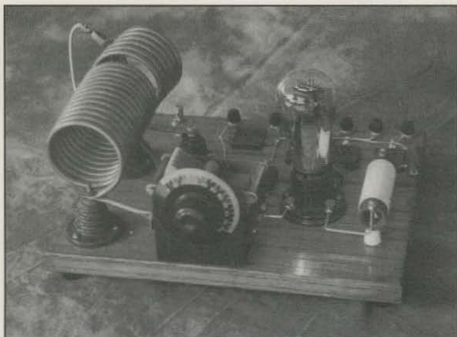
Fig. 8— 1998 replica of famous 1930-style TNT transmitter as built by Robert Root, WD6DPU. Look closely at this open-air marvel and you will see a special warmth, beauty, and personality that are noticeably lacking in modern closed-cabinet and digitally-tuned rigs.
