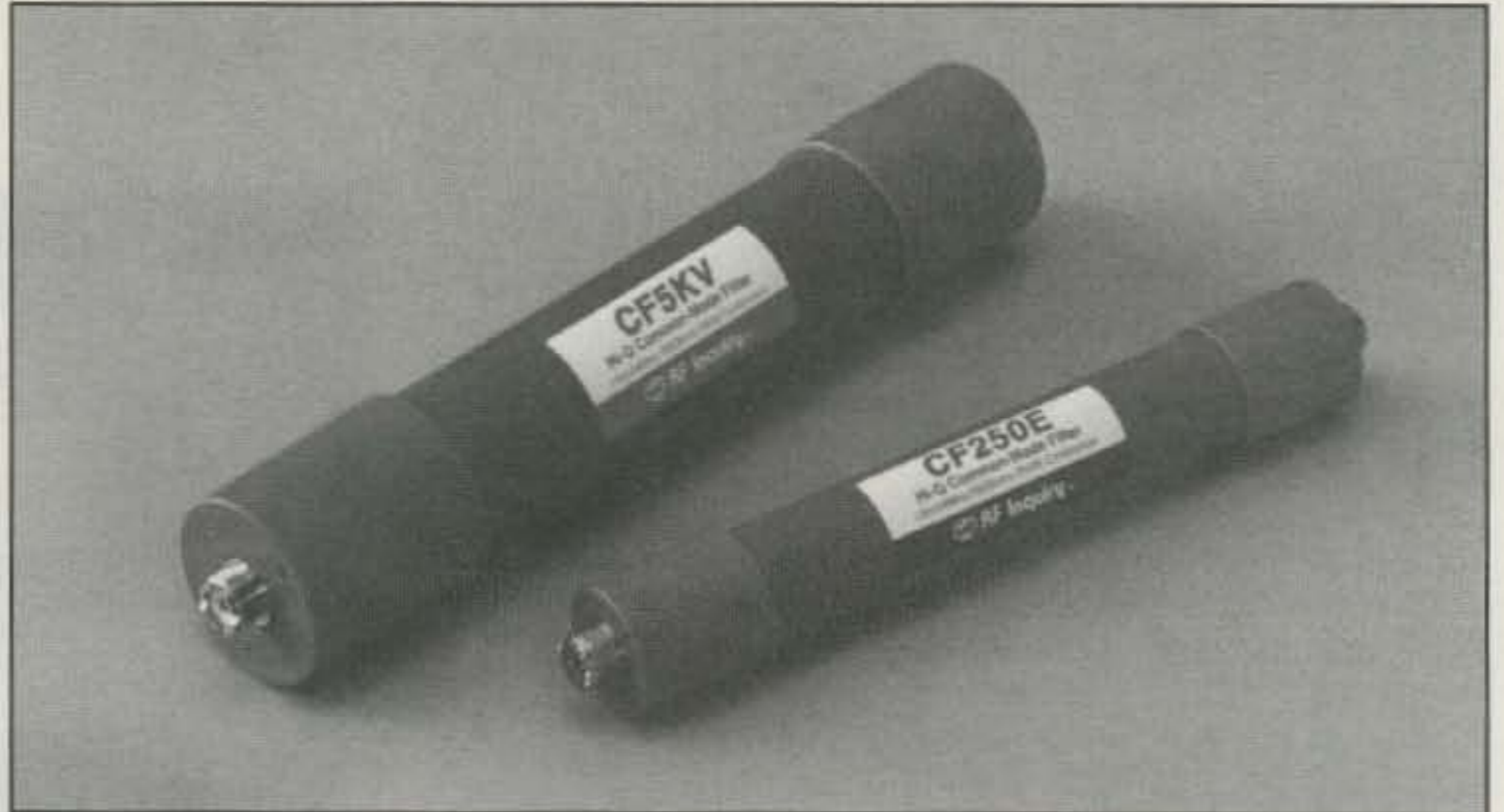
The CF Series Hi-Q Common-Mode Filters are designed to eliminate Common-Mode noise, operating over the range 1.8 MHz to 70 MHz. They also may be used in tandem with conventional lowpass filters to reduce or eliminate RFI. OB Communications offers the Model CF250E/CF5KV filters in four configurations, with power capacity ranging from 250 watts to 5 kW, and with a choice of UHF or N connectors. (Photo courtesy OB Communications)
