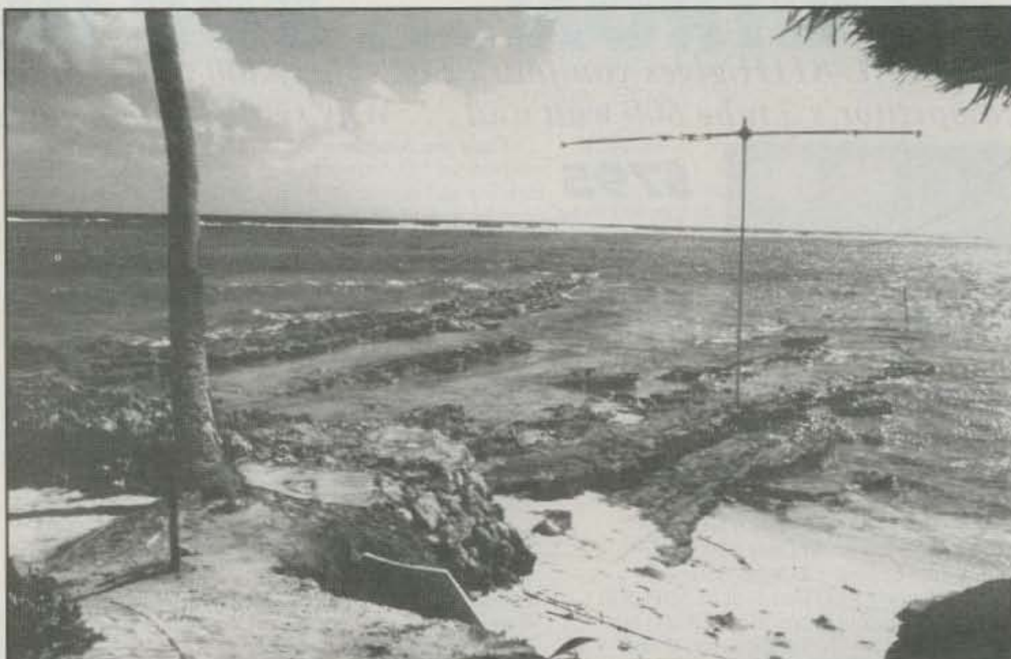
One of the two Force-12 C-3 multiband Yagis used in the 8Q7AA DXpedition.
