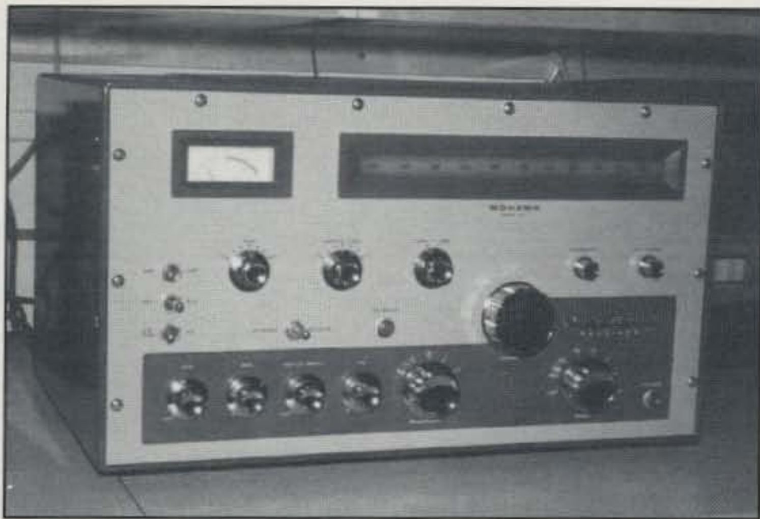
Definitely in the "lovable boat anchor" category, the Heath Mohawk RX-1 receiver was a massive, $274.95 tube-type kit that Heath sold from 1958 through 1963. The double-conversion set covered seven HF amateur bands, from 160 through 10 meters. Many amateurs used it in conjunction with its transmitter counterpart, the TX-1 Apache. (Photo by Tom Bonomo, K6AD, via Barry Wiseman, N6CSW/Ø, Editor and Publisher, Electric Radio magazine.)
