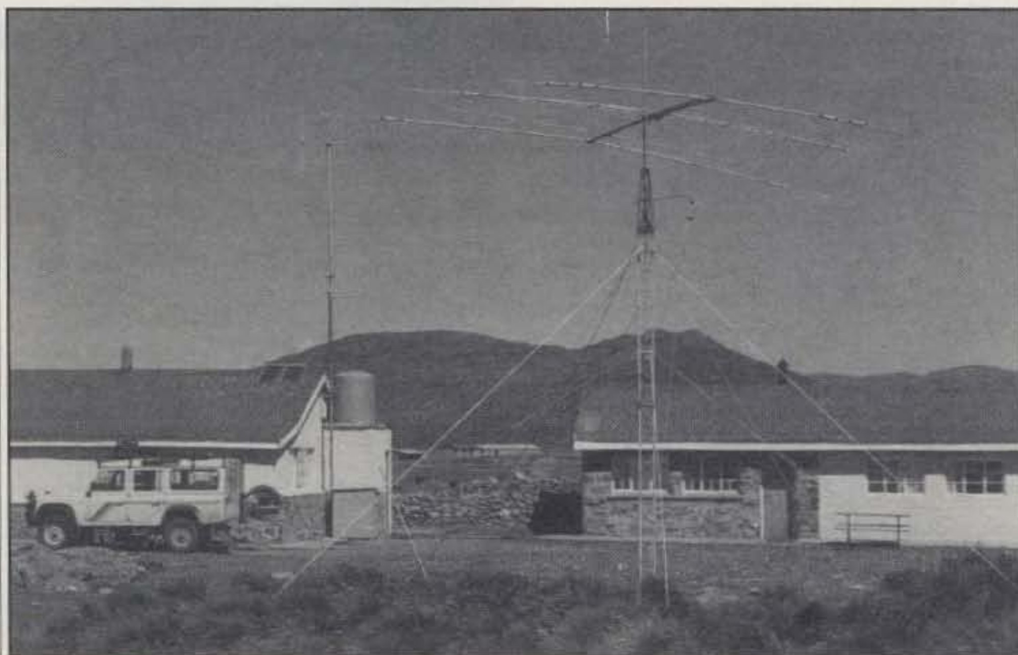
View of our Explorer-14 antenna for 10, 15, and 20 meters, with Dick's Land Rover on the left the Sani Top Chalets in the background. Notice the commercial VHF antennas to the right of our HF beam. They are the only link to the rest of the world when Sani is snow-bound for weeks on end.
