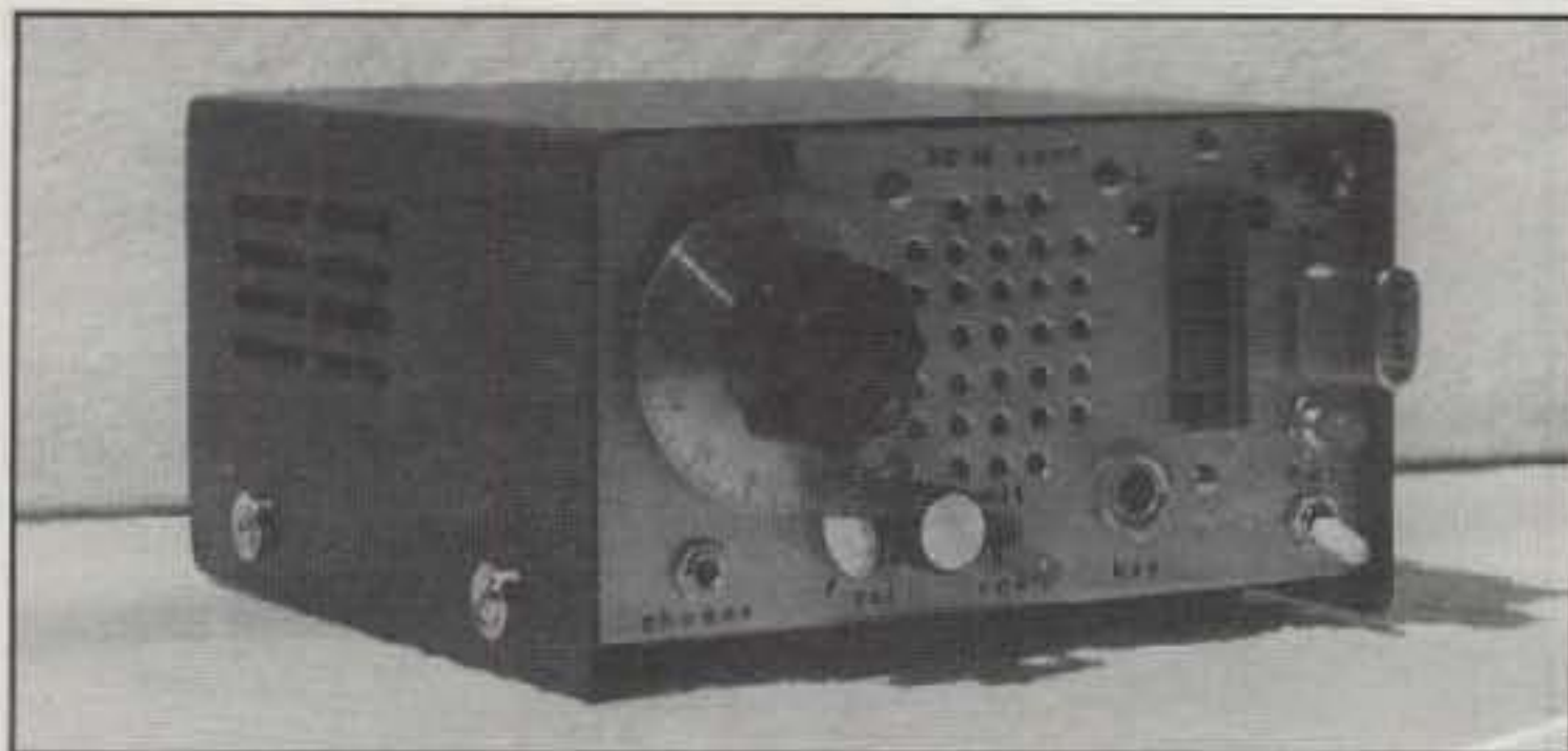
Photo 4— Front view of the neat homebrewed 30 meter QRP trans-receiver made from scratch by Stan, W3TFA. Transmitter is crystal controlled with sidetone and front-panel output meter. Receiver is three-IC design with VXO tuning and produces sufficient audio to drive the front-mounted speaker. Battery pack is included, so Stan just plugs in an antenna and key to operate. Size is 3 by 5 by 5 inches. (Photo by Stan Brigham, W3TFA)
