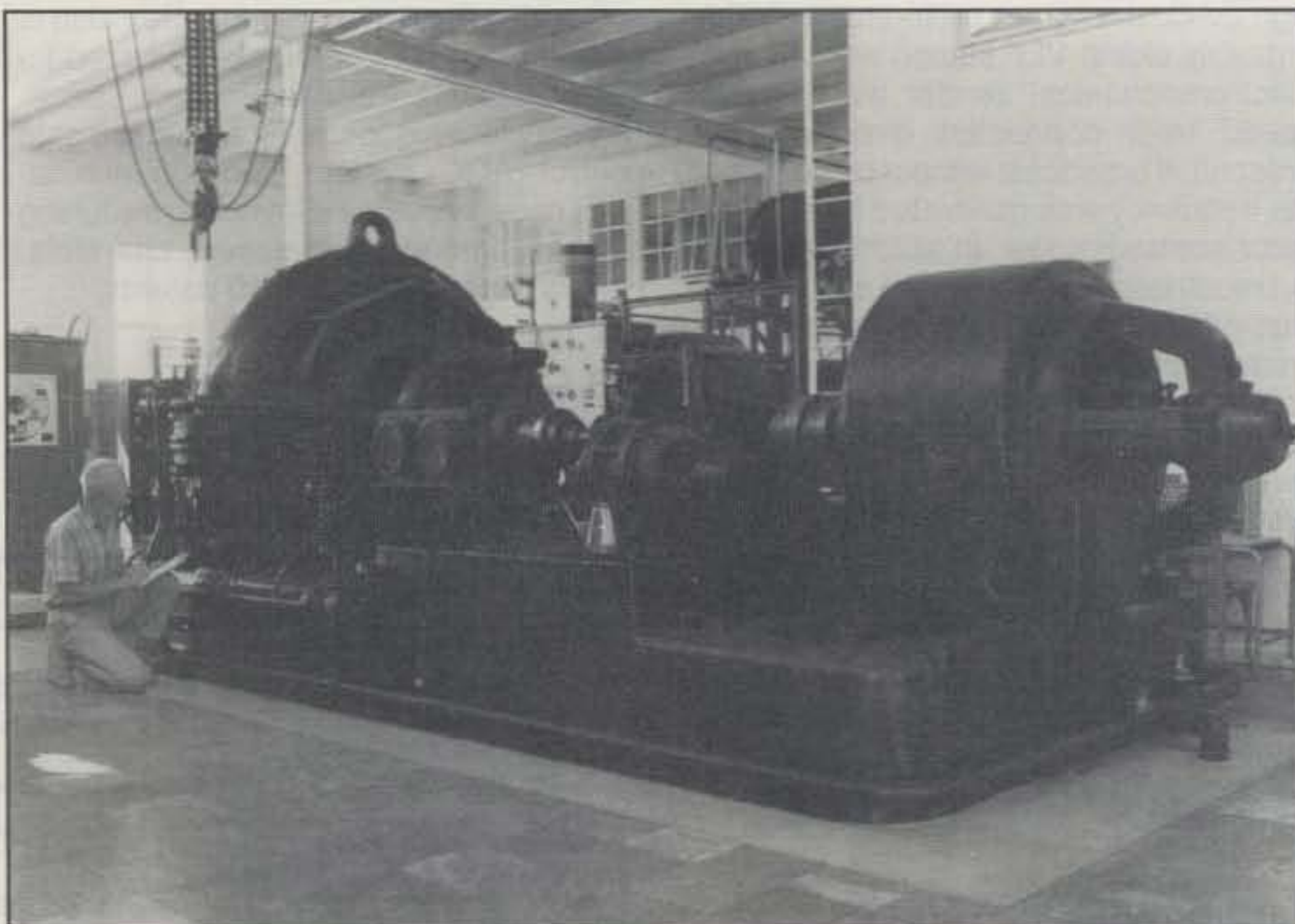
The Alexanderson Alternators, designed by Sweden's Dr. Ernst F. W. Alexanderson, were intended for worldwide communications; only one is left. The device is a large, electromechanical high-frequency alternator with a high-speed rotor connected directly to an antenna. Today Grimeton Station broadcasts on ceremonial occasions on 17.2 kHz. (Photo courtesy Telia AB, Sweden)
