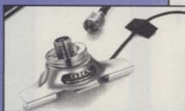
GR-5M Deluxe trunk lip mount. Rubber coated base protects the vehicle's paint. All stainless steel, includes the CK-3M5 deluxe cable assembly to avoid water leaks/cable damage when shutting the trunk. Four large set screws hold it securely in place. Two offset washers adjust the antenna to vertical. Gold-plated SO-239/PL-259 connectors.
