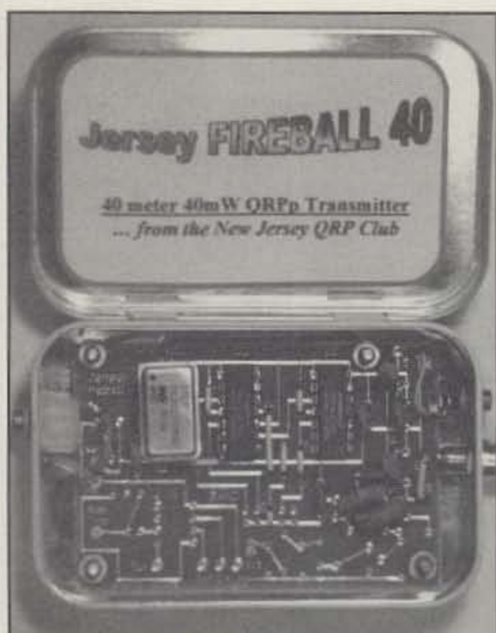
Fig. 4— You know this critter is QRP because it's in an Altoids tin! This is a completed and ready for action JF40. Optional Tick keyer, T/R switch, and RF amplifier have yet to be added, but it is still a gem. (JF40 photos courtesy George Heron, N2APB.)
