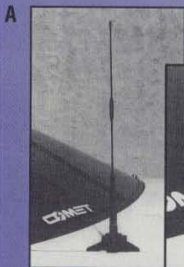
GR-5M Deluxe trunk lip mount. Rubber coated base protects the vehicle's paint. All stainless steel, includes the CK-3M5 deluxe cable assembly to avoid water leaks/cable damage when shutting the trunk. Four large set screws hold it securely in place. Two offset washers adjust the antenna to vertical. Gold-plated SO-239/PL-259 connectors.
