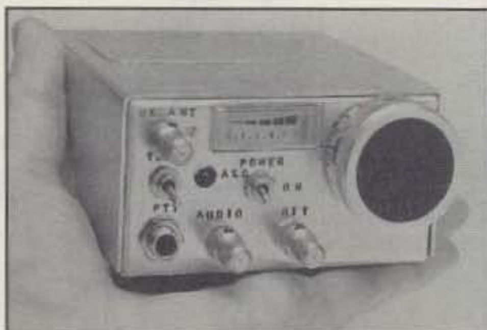
Fig. 7— The amazing palm-size 75 meter SSB transceiver homebrewed by Stein Torp, LA7MI, in Norway. Imagine carrying a tiny talker like this with you on a weekend getaway. Ham heaven for sure! (Photo courtesy Stein, LA7MI.)
