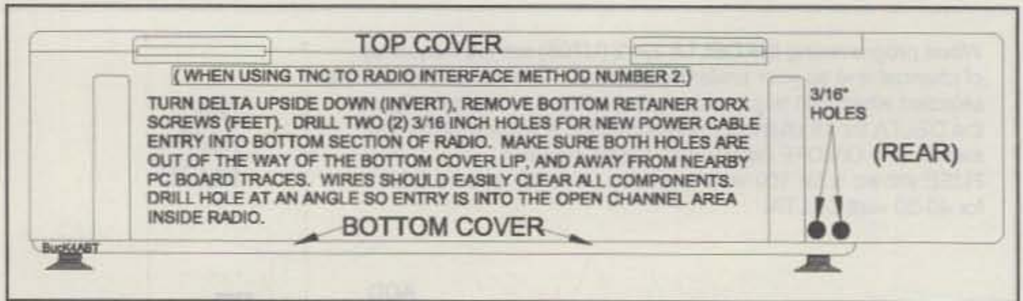
Fig. 4— Now for the preparation "R" as we carefully drill the two 3/16 inch holes in the "rear end" of our Delta. These two holes are for the DC power leads into the 110 watt Delta. See fuse information in fig. 1 or fig. 2.
