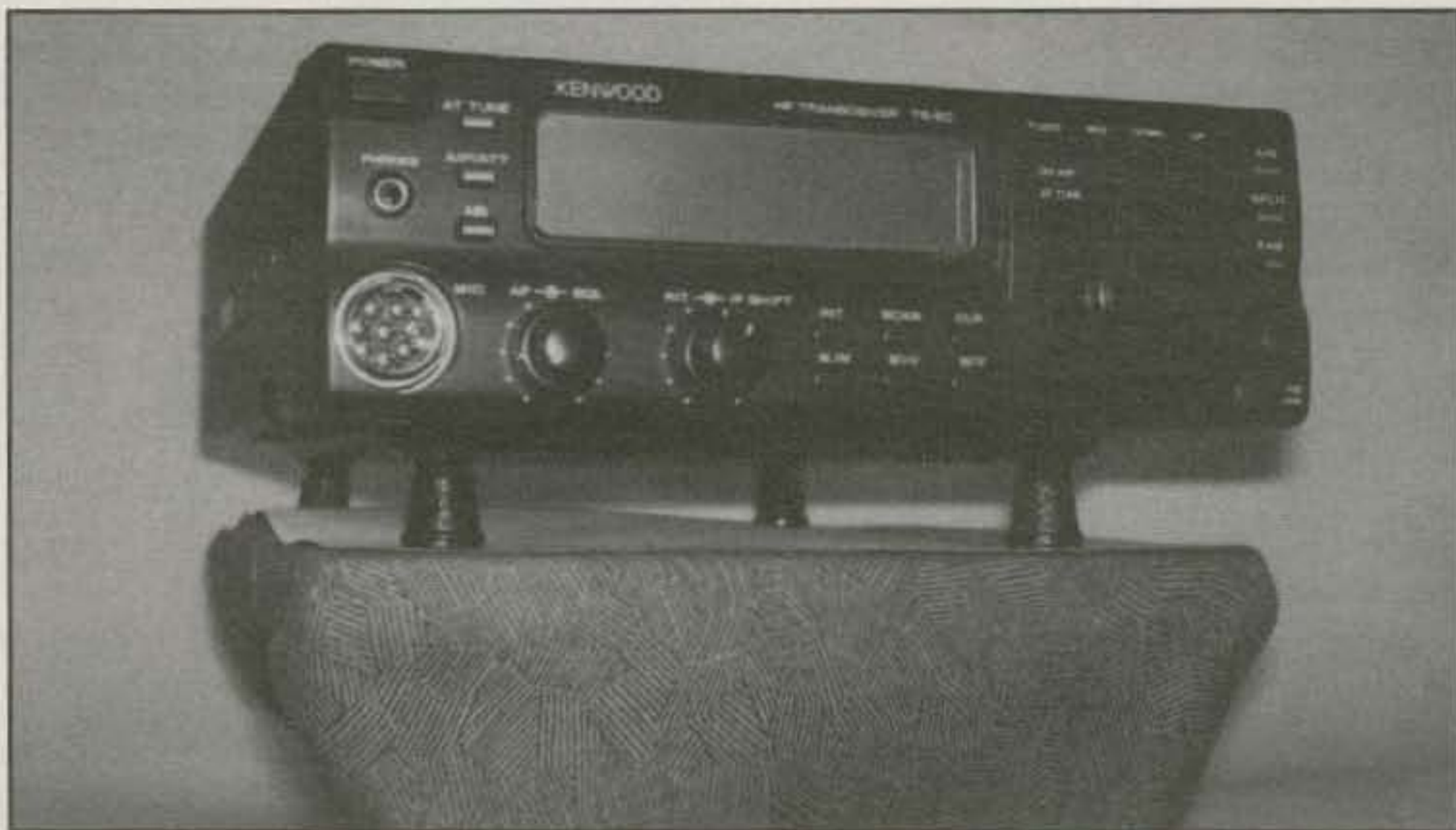
Photo 1— This homebrew shelf/mount was removed from our car for clear-view photographing in sunlight. It illustrates an important point in how a transceiver should be supported by its feet rather than its case. (Discussion in text.)
