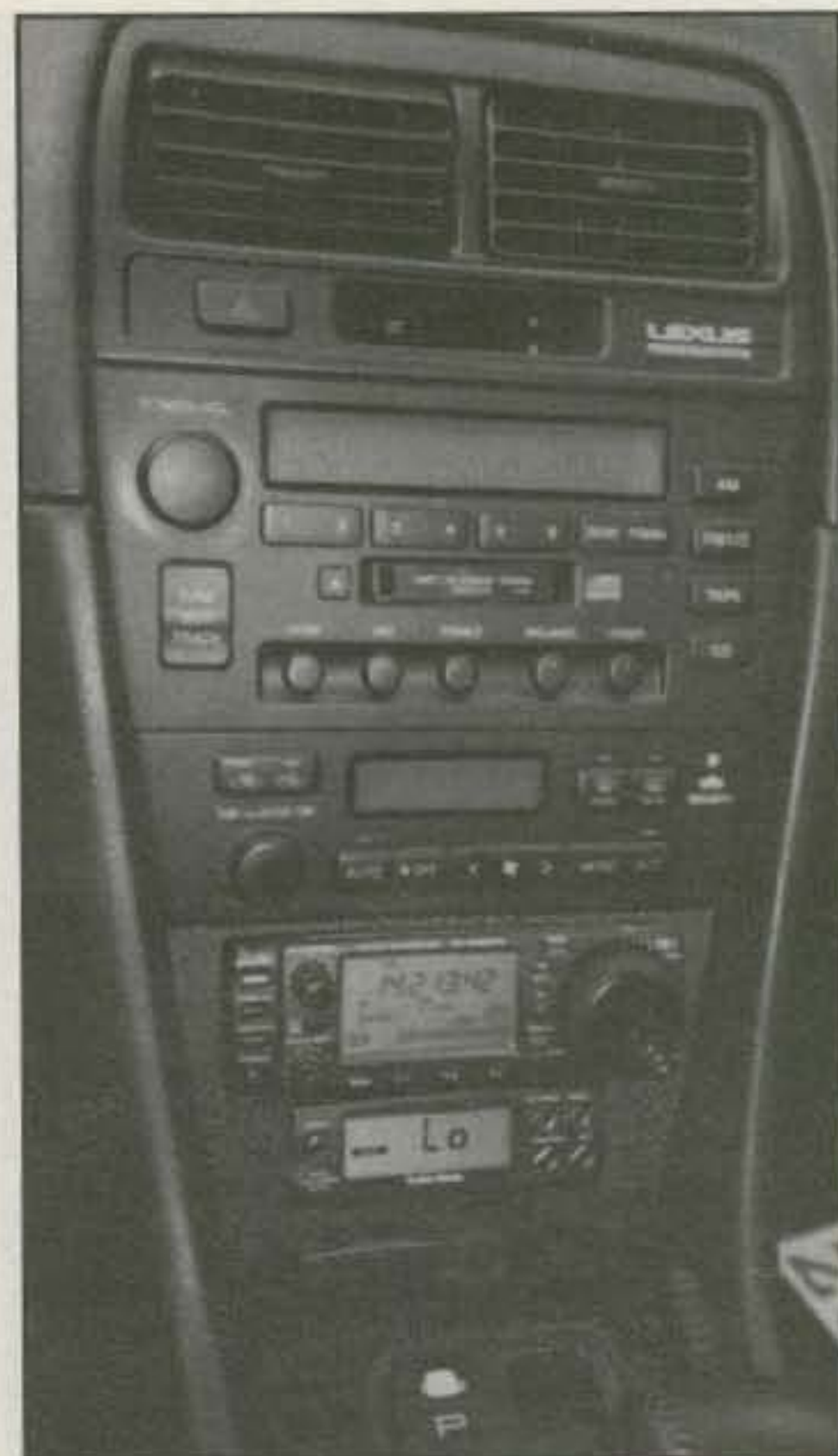
Photo 6— Center console view of the K2QBV custom mobile setup. Below the radio and heater are an ICOM 706 front control panel and digital SWR meter. Both fit into a homebrewed shelf that replaces the ashtray. A front template adds the perfect finishing touch. (Photo courtesy Joel Kornreich, K2QBV)
