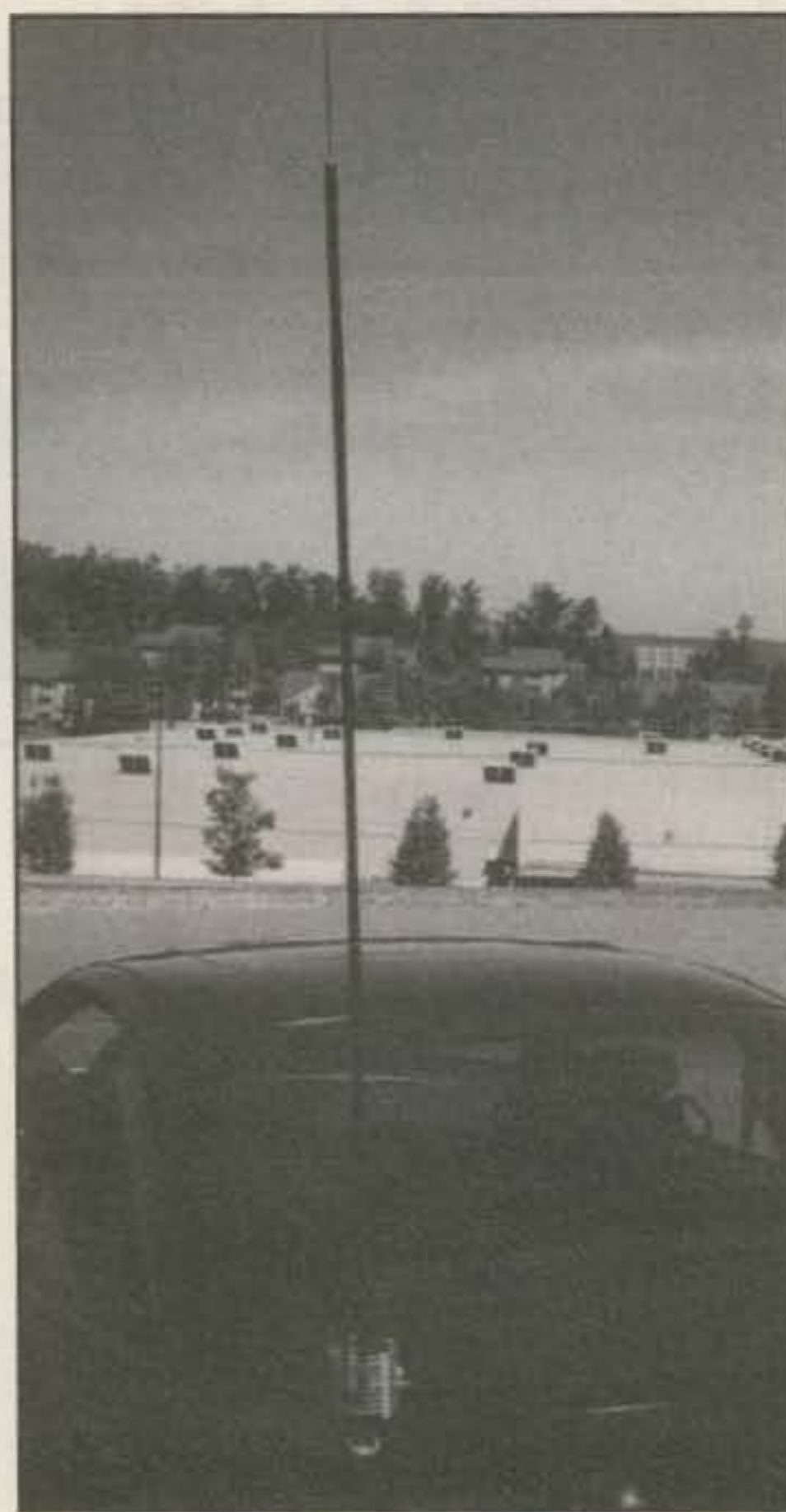
Photo 4— The Hamstick shortened to 4 foot height and modified for "one band up" operation as described in the text. The whip is lightweight and short enough to go almost anywhere. Note the short top stinger and base matching coil. The location? A park down the hill a few blocks from my house. Those black blobs are air conditioners atop a Wal-Mart.
