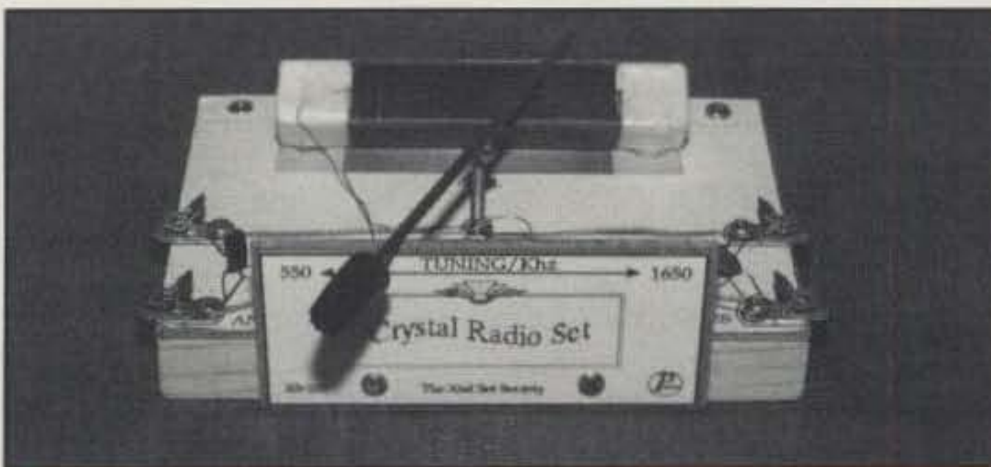
Photo 6— An assembled XS102 looks as good as it works. Decorative front panel and parts layout guide are included in the instructions and glue to boards for a nice finishing touch.
