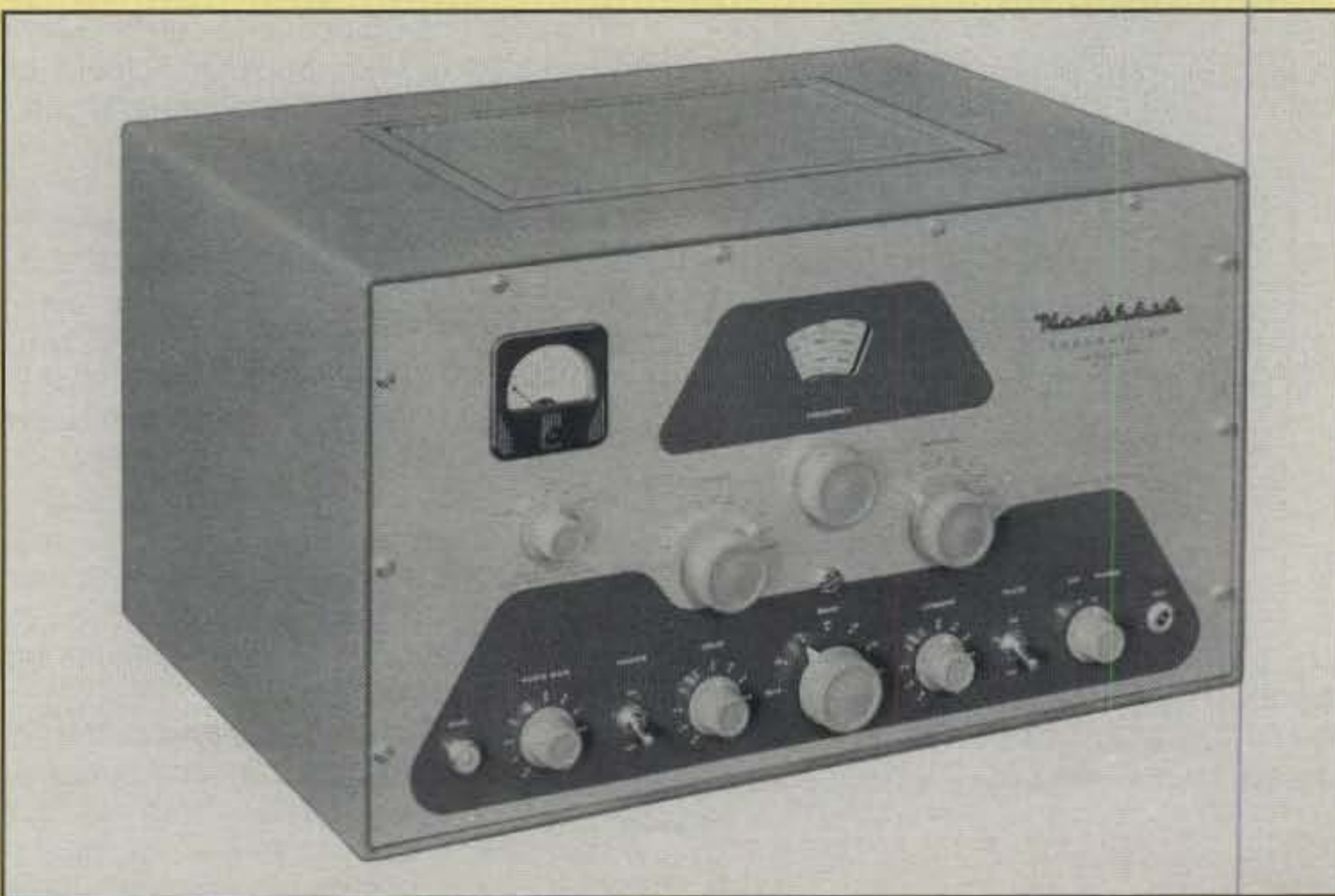
The Heath Company once was the world's largest manufacturer of electronic kits. A popular amateur kit was the 180 watt DX-100 (and later DX-100B) AM/CW transmitter. An angled front view of an assembled DX-100B is shown here. (Photo courtesy Terry Perdue, K8TP)
