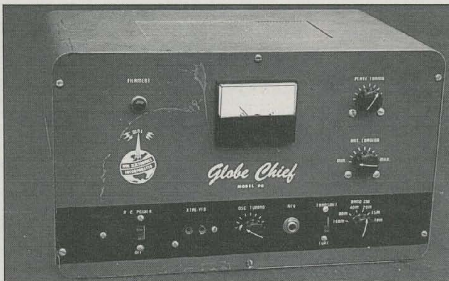
World Radio Laboratories (WRL) was known for big, heavy gear, which included the massive Globe Champion and Globe King series. The relatively lightweight, 90 watt Model 90 Globe Chief, circa 1956–1957, is shown here. (Photo by Jim Hanlon, W8KGI, via Electric Radio magazine)
