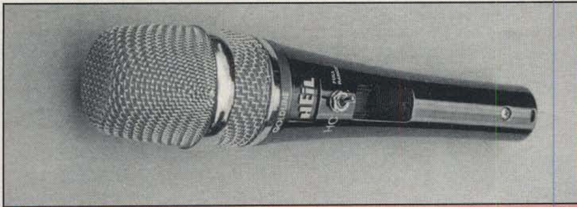
Photo 4— Heil Sound's new goldline microphone helps any transceiver stand above the crowd with full-bodied, studio-quality audio that sounds marvelous. Flip its "HC" switch, and a second element in the mic changes response to more "talk power" for DXing and contesting.
