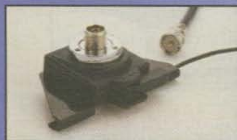
CQ-5M Deluxe "Quick-Disconnect" trunk lip mount with CK-3M5 cable included. With a flip of a lever, the antenna and coax are easily removed and stored in the trunk for car washes, theft prevention or any reason.
