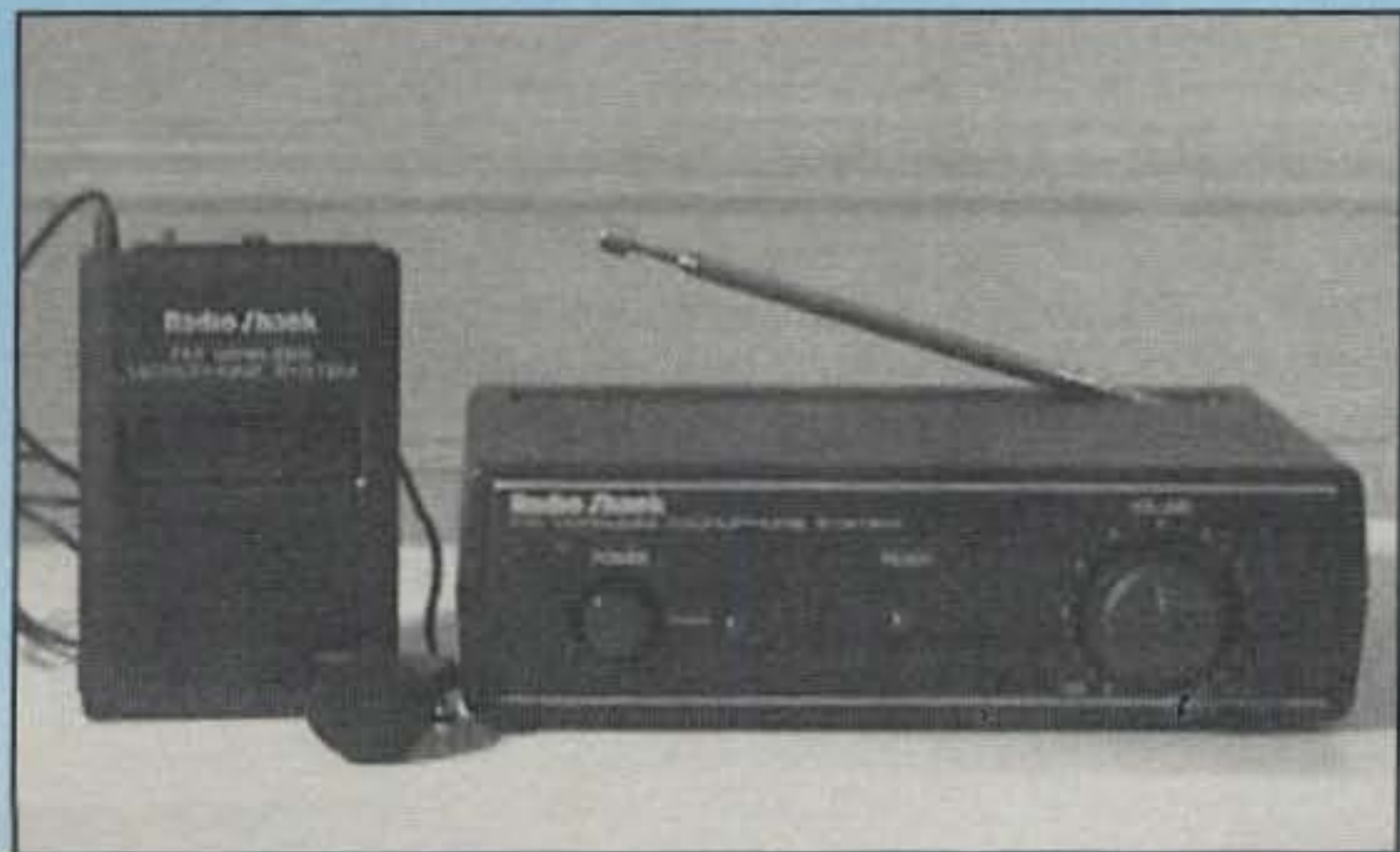
Watch for sales on wireless microphones. They let you move around while talking without being "off-mic." If you get more than one, make sure they're on different frequencies.
