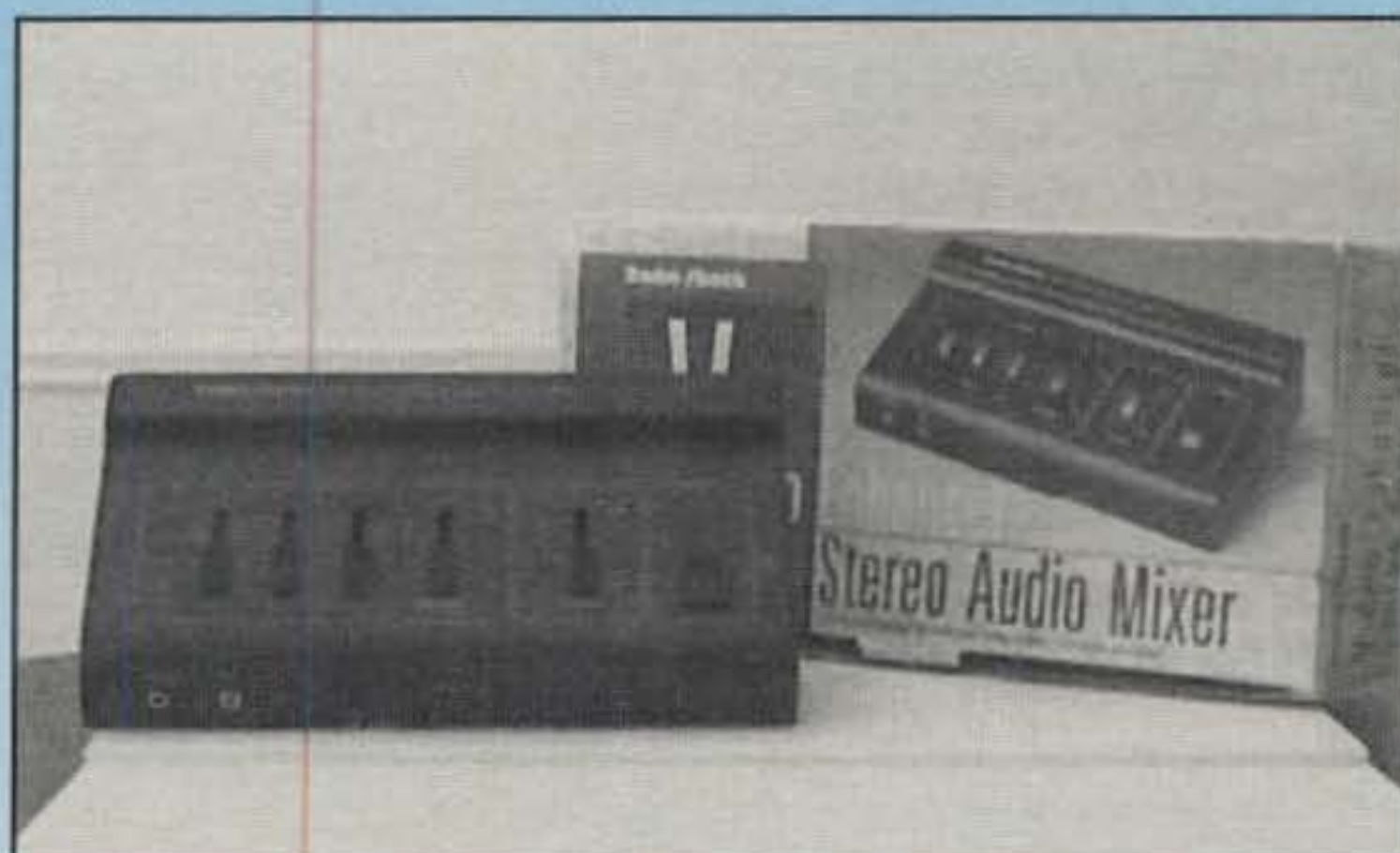
An audio mixer will let you control multiple microphones and other sound sources. Look for one with both mic-level and line-level inputs.
