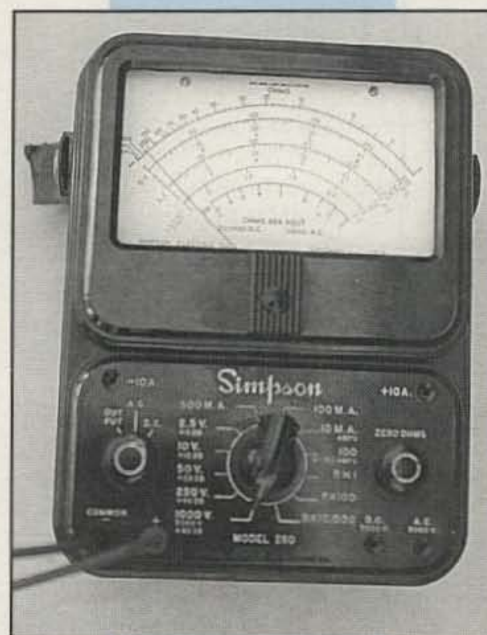
Photo B— An example of a traditional analog-scale volt/ohm meter (VOM) is the famous Simpson model 260. Center switch selects/connects various internal multiplier and shunt resistors required to read different voltage and current ranges. This particular VOM is special, as it was "handed down" to me from my father. He designed the original burnout-proof 260, and this was his prototype.
