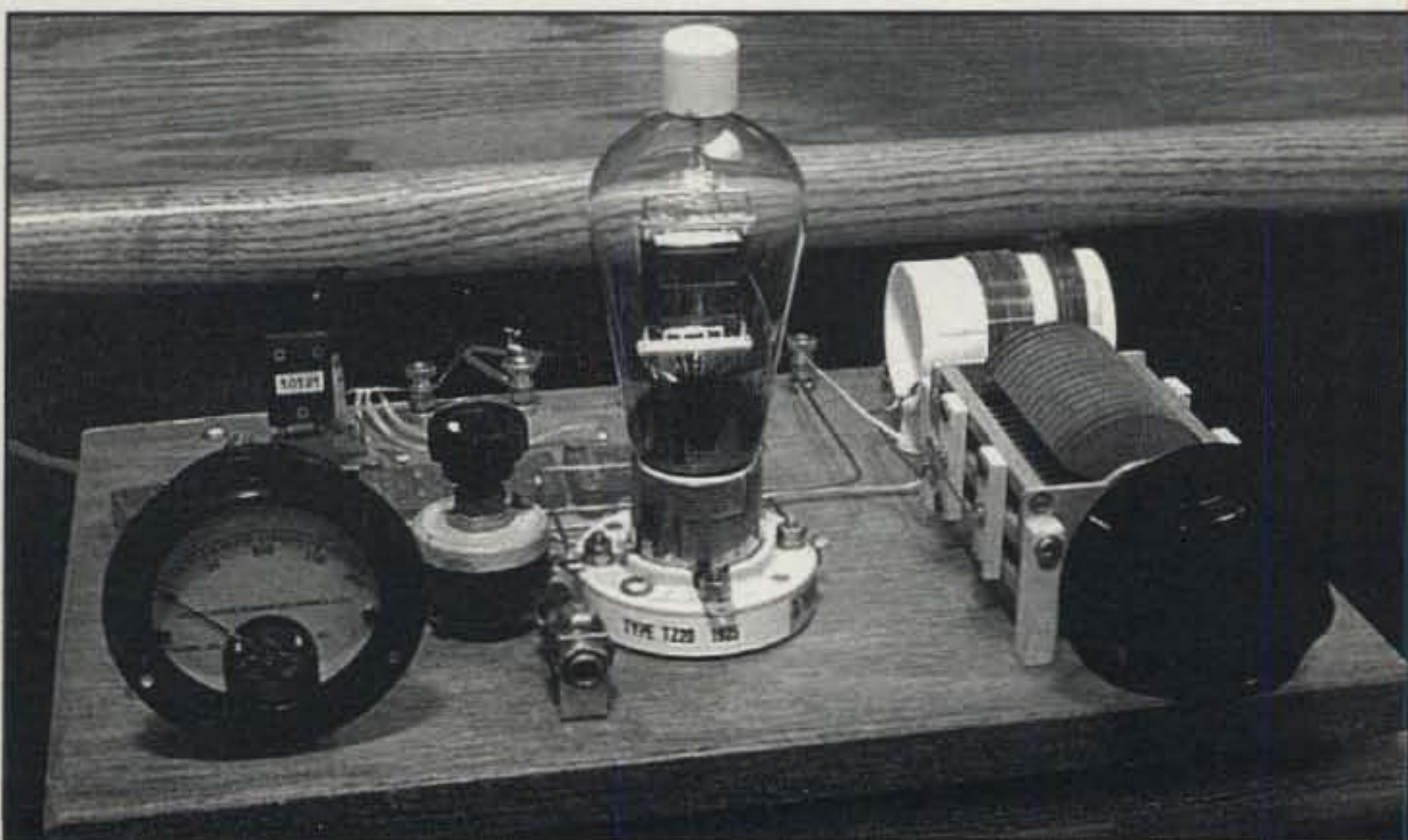
Photo D— This 1935 replica transmitter was made by Quent, K5TVC, after he read about it in our November 1998 column. The rig uses a Taylor TZ20 tube, Johnson ceramic socket, and Weston meter. Beautiful, isn't it? (Photo via K5TVC)
