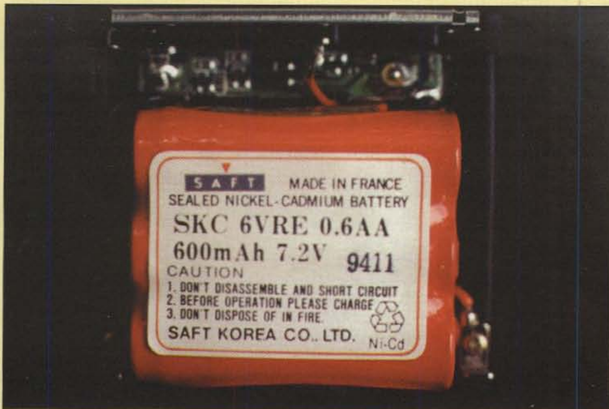
Photo 3— Original HTX battery compartment.
