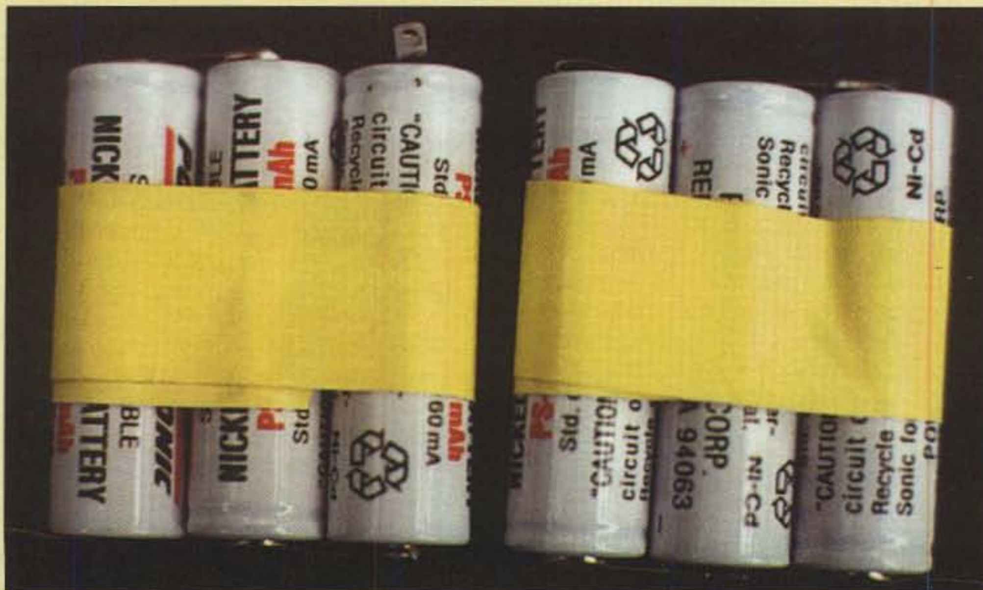
Photo 4— Align the new NiCad batteries, alternating plus and minus, into two sets of three batteries each and wrap with electrical tape.
