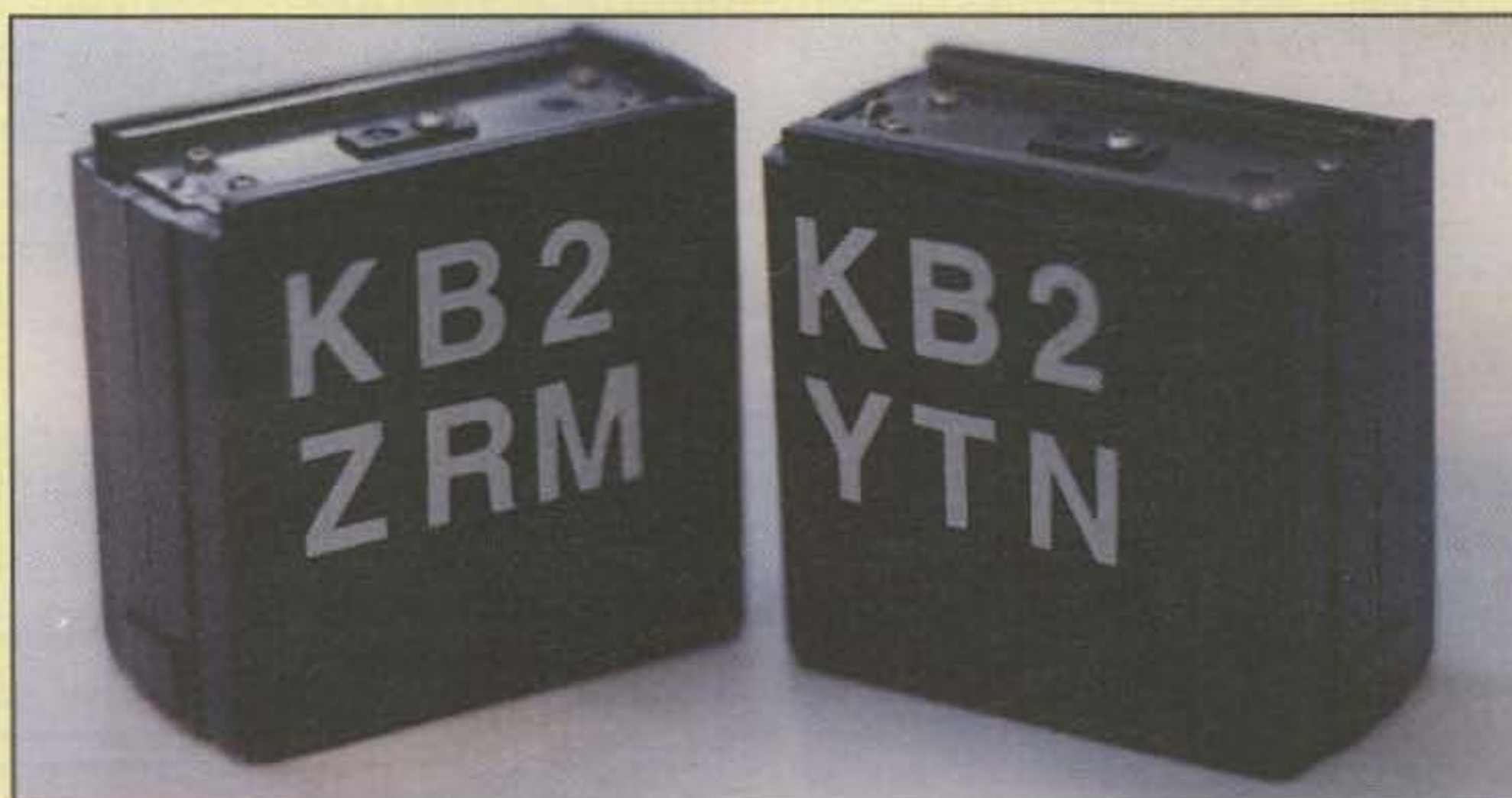
Photo 1—Two completed HTX battery packs.
