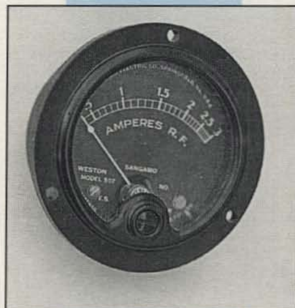
Photo A— Classic analog-type panel meter such as would be mounted on a high-power linear amplifier, SWR bridge, etc. This particular meter measures RF amps. By connecting it between a transmitter or amplifier's output and an antenna, and applying the formula of antenna current squared times resistance of antenna, it will indicate output power from one watt to approximately 450 watts.
