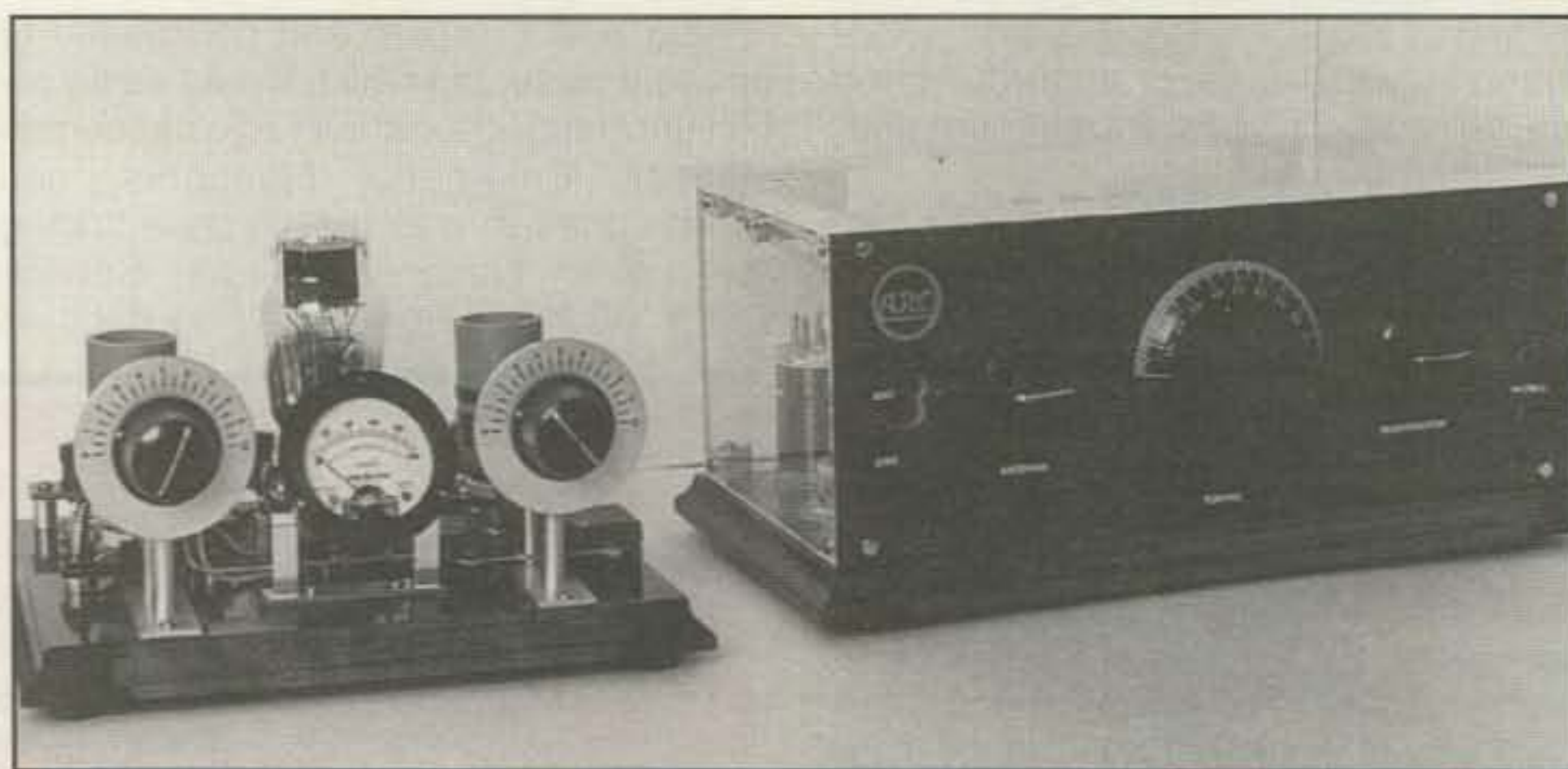
Photo A— This smart-looking Tri-Tet transmitter (left) and its mating receiver (right) were made by Arnold Sayre, W8WVM, and both units are absolute showpieces. The transmitter's tuning capacitors are mounted on metal spacers and graced with homebrew dials behind vintage knobs. The meter in the center adds symmetrical balance to the layout. (Photo courtesy W8WVM)
