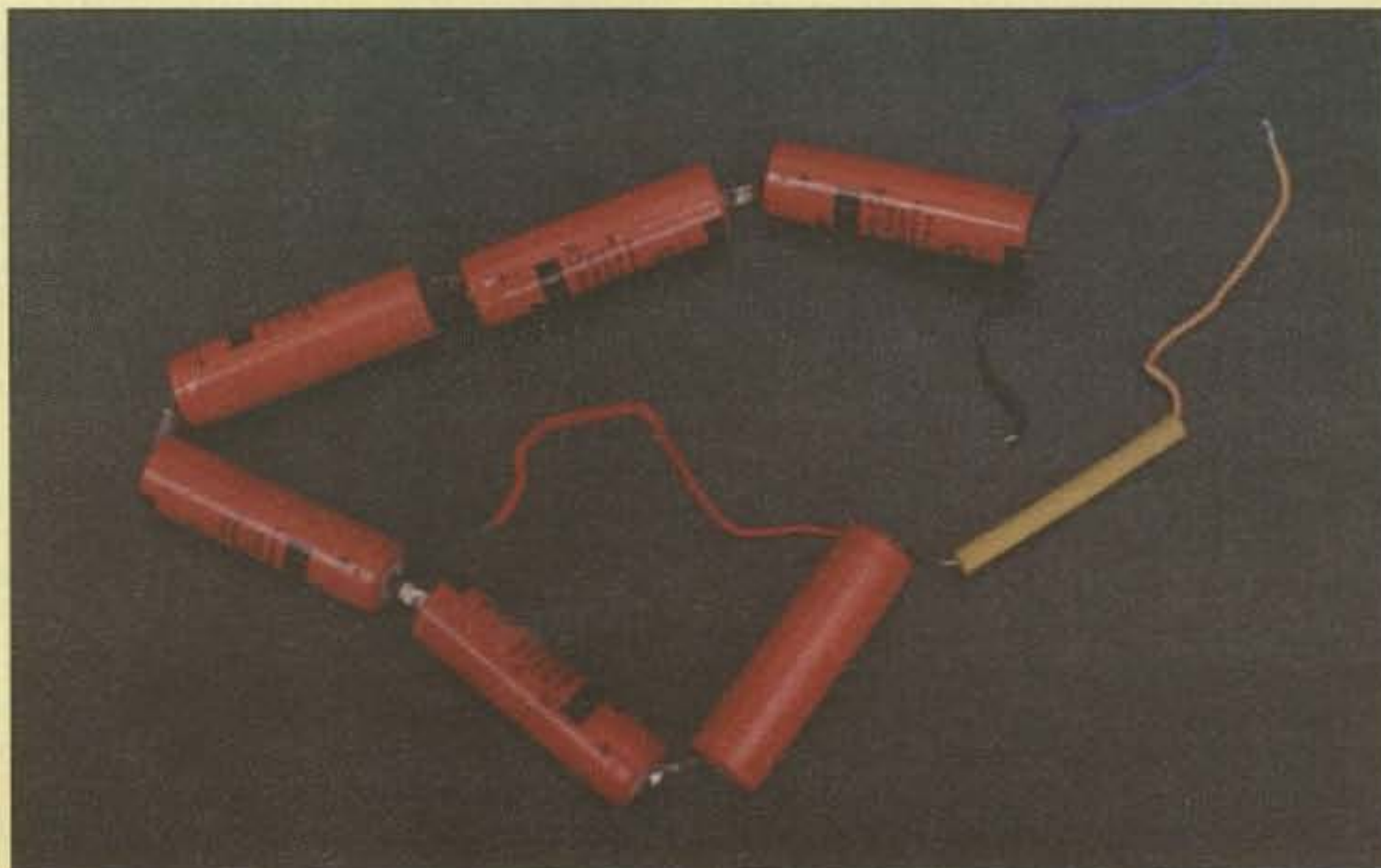
Photo 2—Six original 1.2 volt NiCad batteries in series with wires attached.
