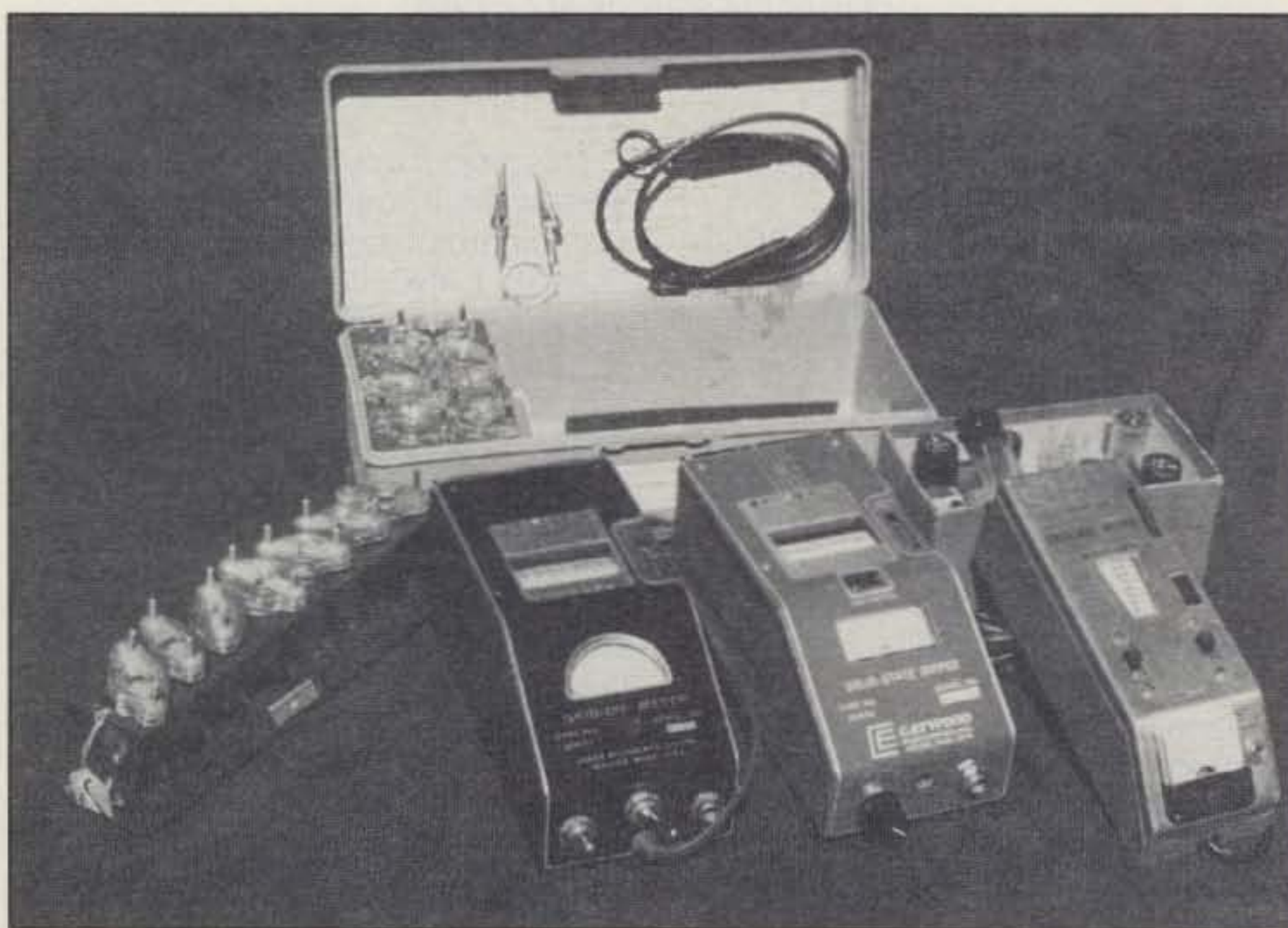
A trio of dippers: (left) Millen 90651 with coil rack, (center) Millen/Caywood 90652 with sniffer cable and universal clip-wire, and (right) Eico 710 with coils.
