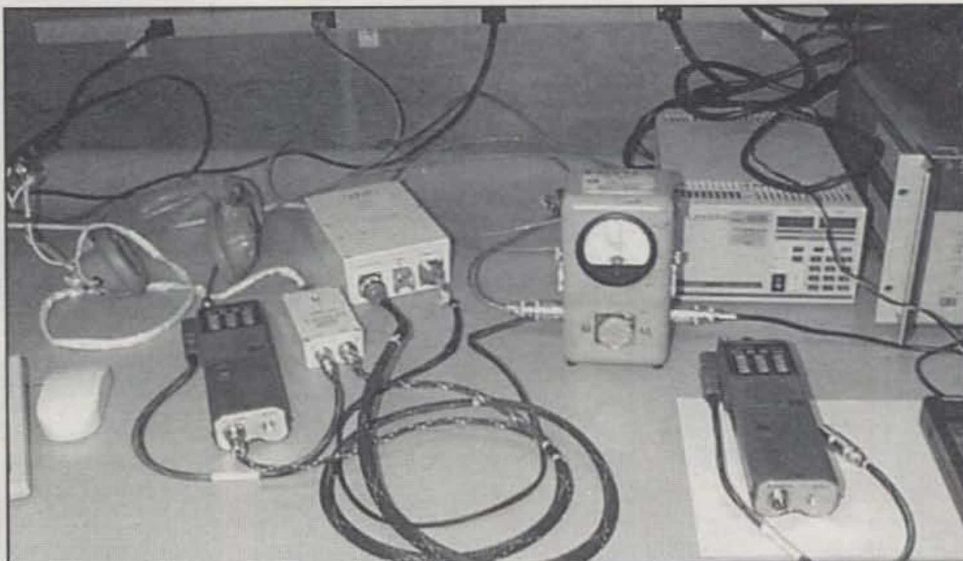
A photo of the handheld transceivers, headset, and packet module which will be the initial amateur radio equipment on the International Space Station.
