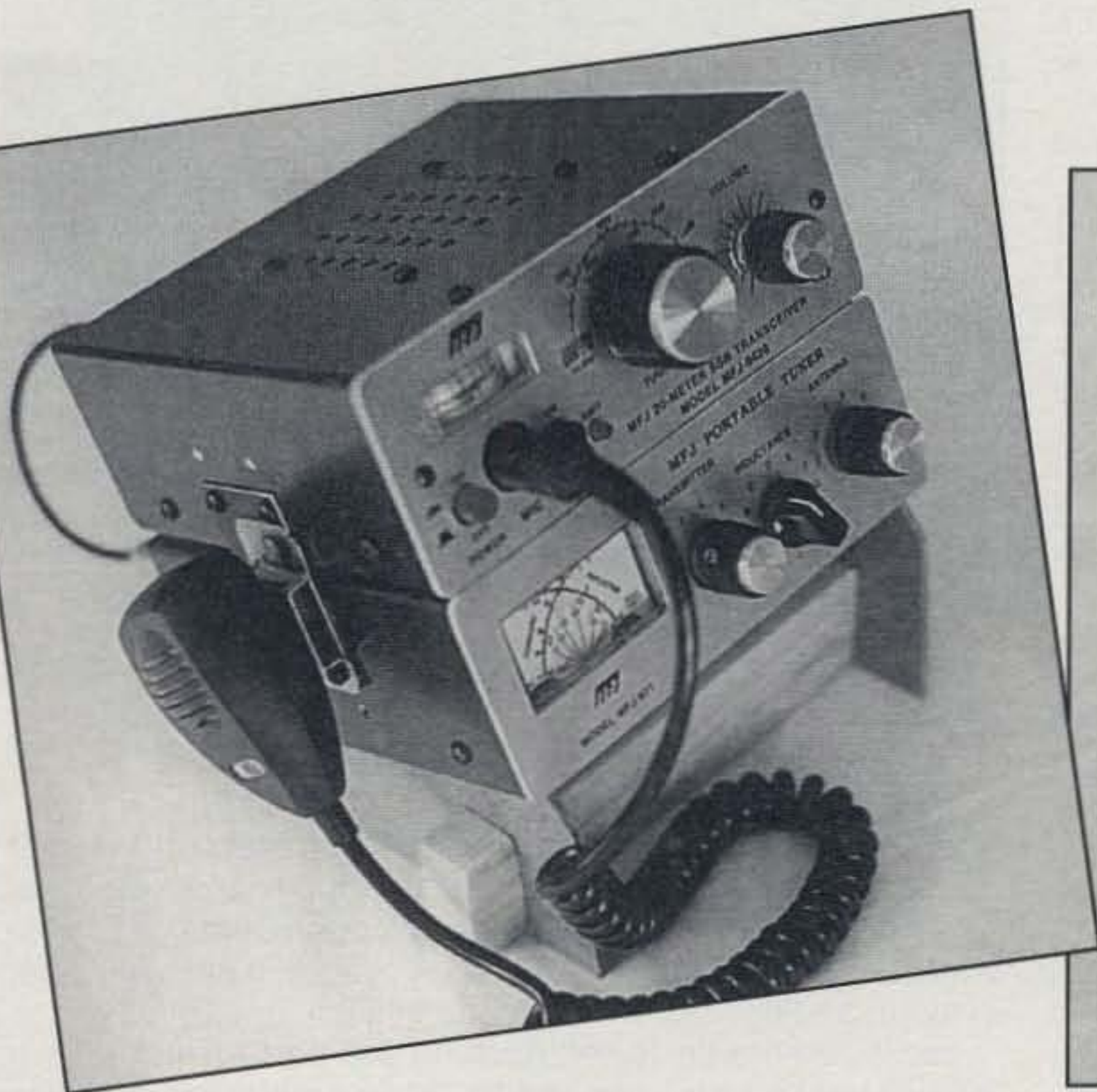
Photo 3— This smart-looking, functional QRP rig stand made by Thomas Hart, AD1B, tilts gear for easy viewing of dials and meters and snaps apart for traveling. Rather than including a bottom platform, gear is supported by fiber-board side rails. (Photo courtesy AD1B)
