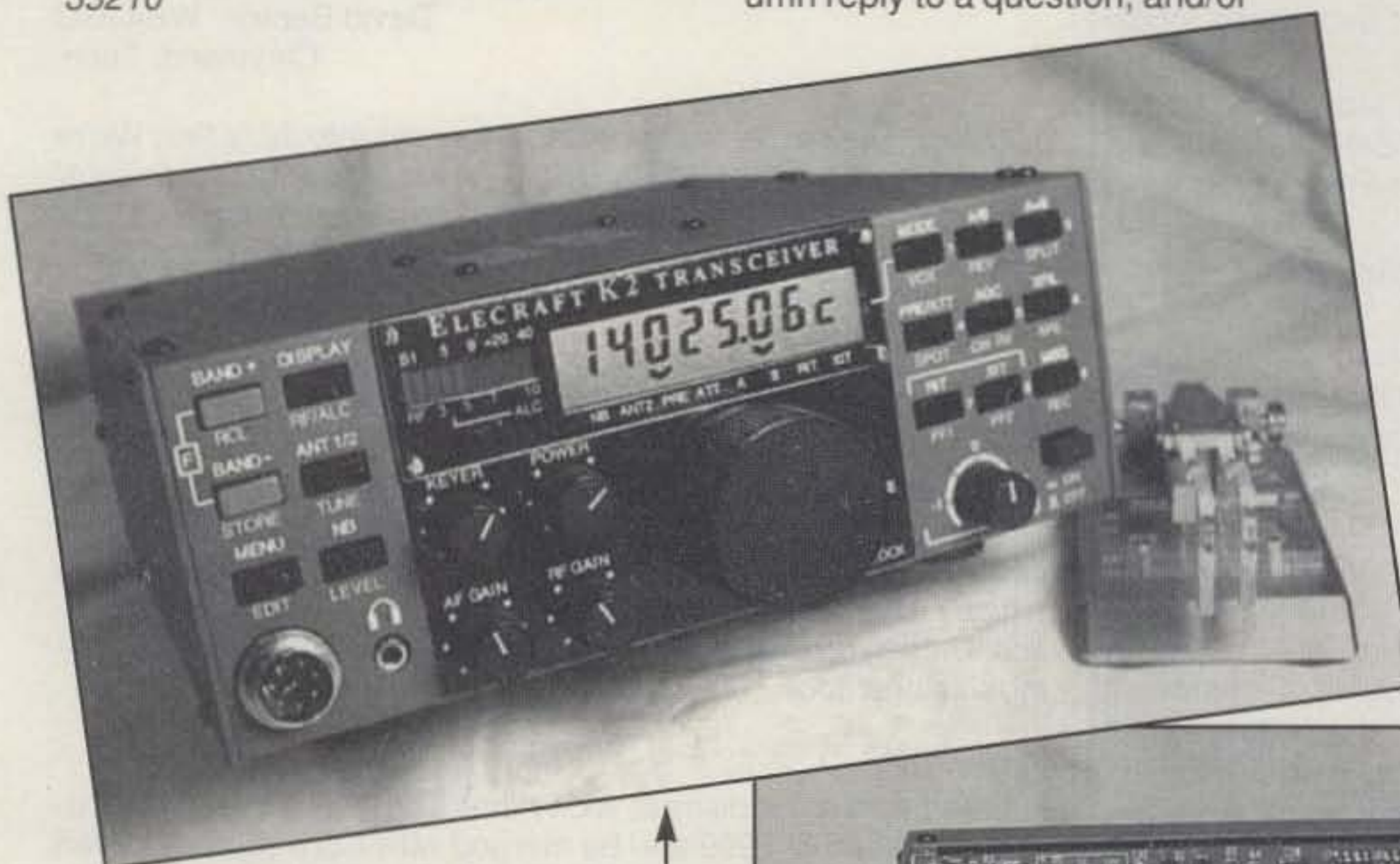
Photo 1— Front view of the new Elecraft K2 kit transceiver. The unit was designed by Wayne Burdick, N6KR, of NorCal QRP fame and measures 3"H x 8"W x 8"D. The transceiver operates CW with 10 watts output, and you can add options such as SSB, 160 meters, noise blanker, extra filters, auto antenna tuner, etc., to produce a custom unit. (Photo courtesy Elecraft Co.)
