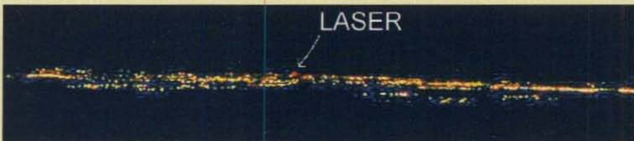
Fig. 1— At a distance of over 40 miles a 5 mw laser is still just about the brightest object in view. This is what a laser looks like from such a distance compared to city lights.
