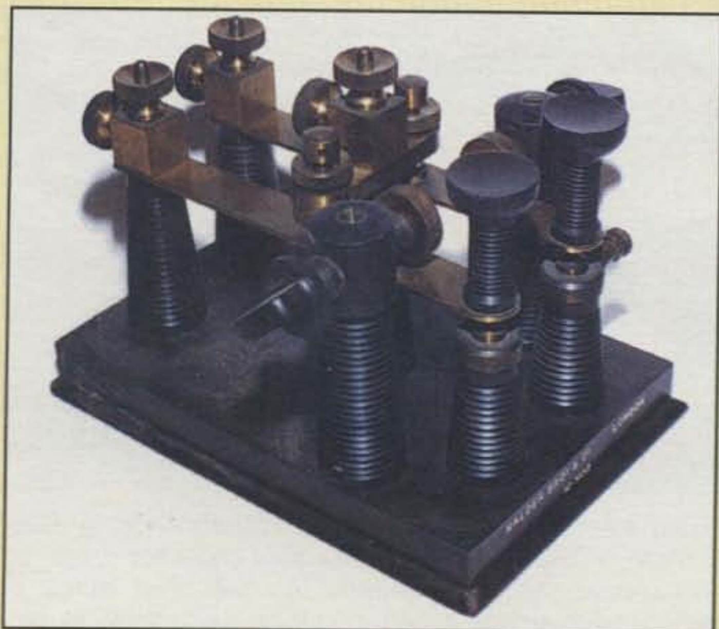
Photo 7— You are looking at a genuine London Cable Key made by Nalder Brothers and Co. of England. It was one of the very first Cricket keys. That's right—a Cricket key. You use your index and middle fingers to send dots and dashes "tabletop drummer style" with the little tyke. Hmm... separate wires could be connected to those two levers for interfacing with a modern electronic keyer. Now that really would make a killer paddle! (Thanks again to K9WDY)
