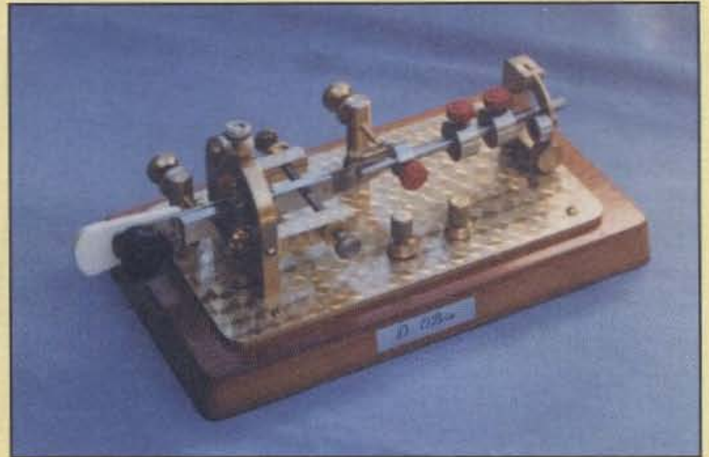
Photo 12— This snazzy bug was homebrewed by Des O'Brien, ZL2UOB, from an unusual collection of parts and pieces. Most notable is the fact Des made it without ever seeing a commercially made bug! (Photo courtesy ZL2UOB)
