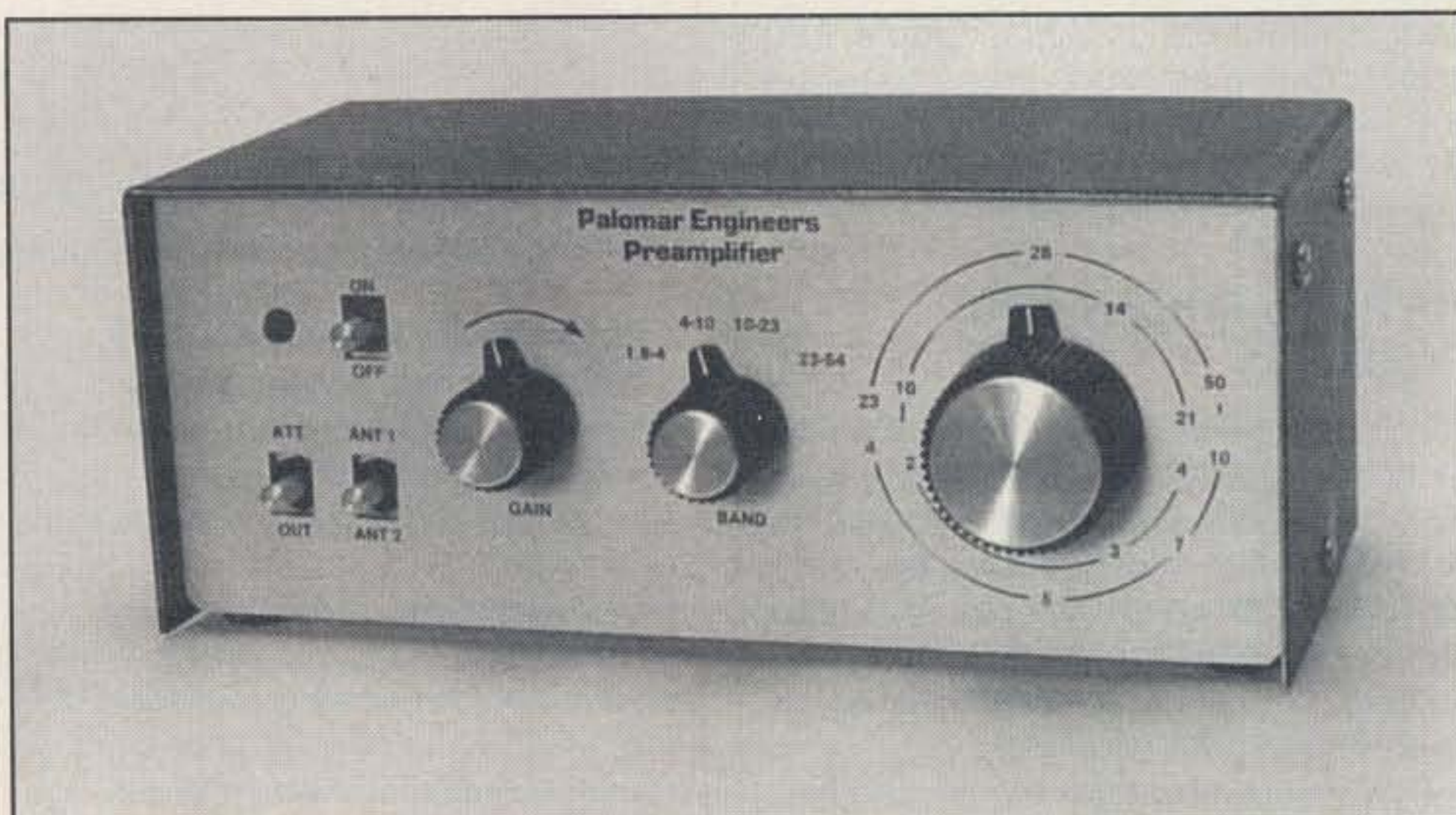
This now-discontinued Palomar Engineers P-405/P-408 receiver preamplifier is representative of units that helps enable weak-signal reception, especially with shortwave receivers that are not as sensitive as they might be. Many older radios, especially tube-types and portables, could use a signal boost. (Photo courtesy Palomar Engineers)
