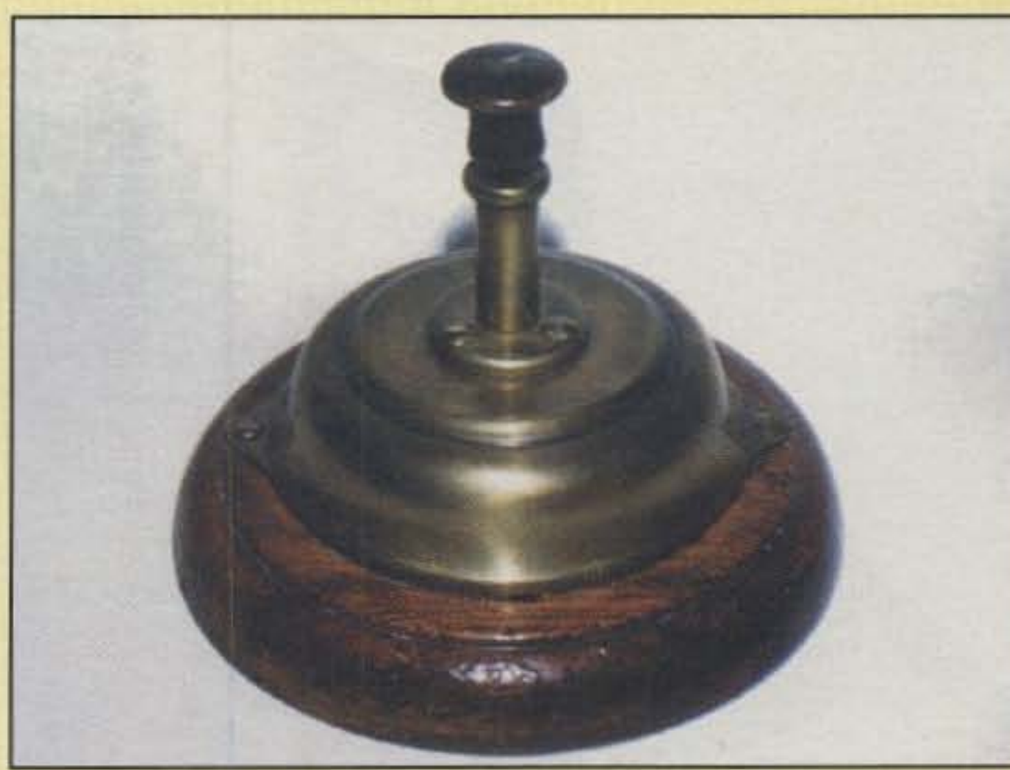
Photo 4—What's this? A bellboy's key? A waitress's key? No, it's a Plunger key, and it has a full-blown hand-key mechanism under that top cover. Unbelievable but true! (Photo courtesy K9WDY)
