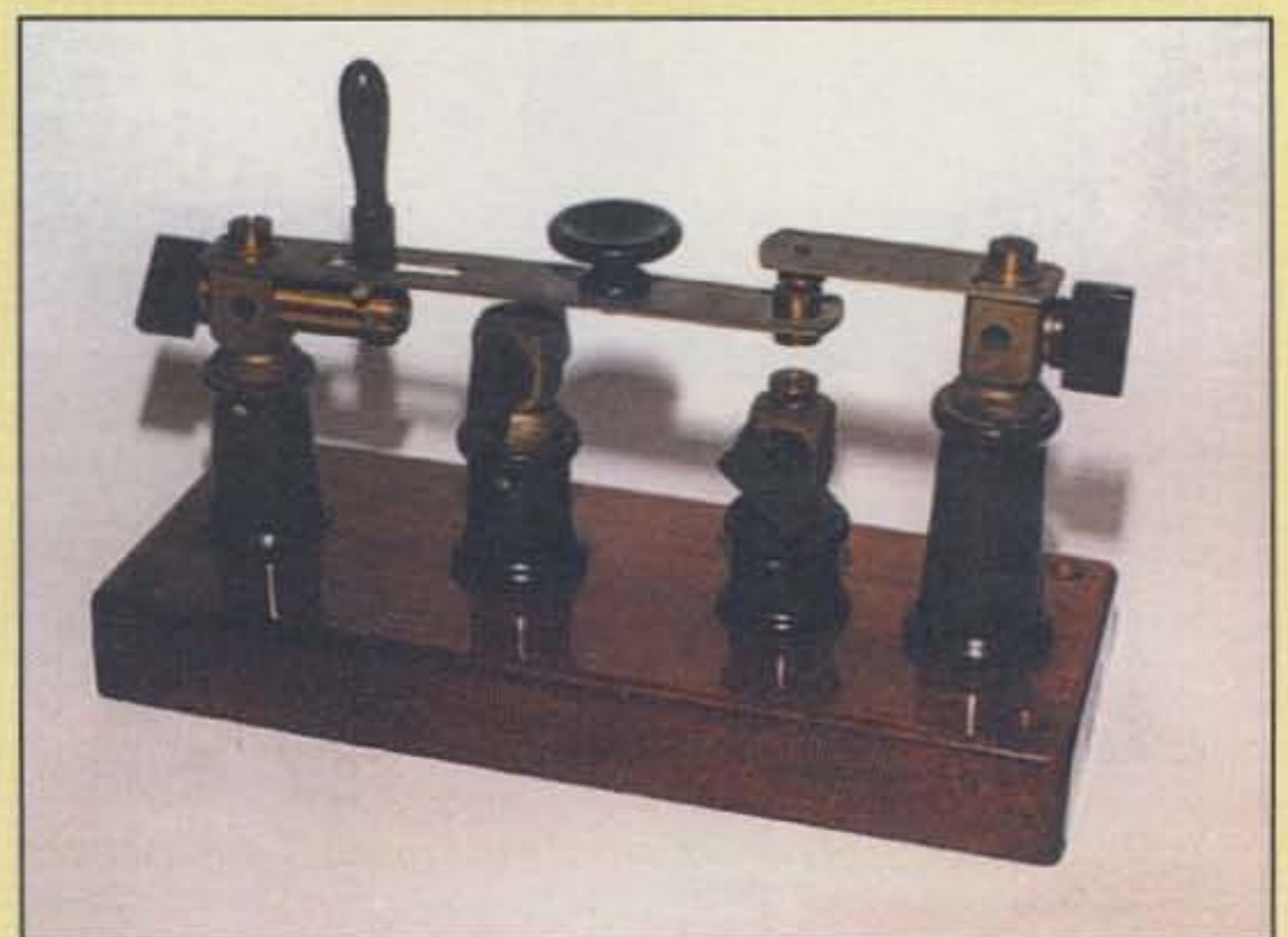
Photo 6— This unusual item is a Frankfurt Cable Key made by the Hartmann and Braun Co. It was designed for use with dual-polarity cable systems of the 1930s. The knob actuates the horizontal arm which "breaks" one circuit while "making" another circuit. (Photo courtesy K9WDY)
