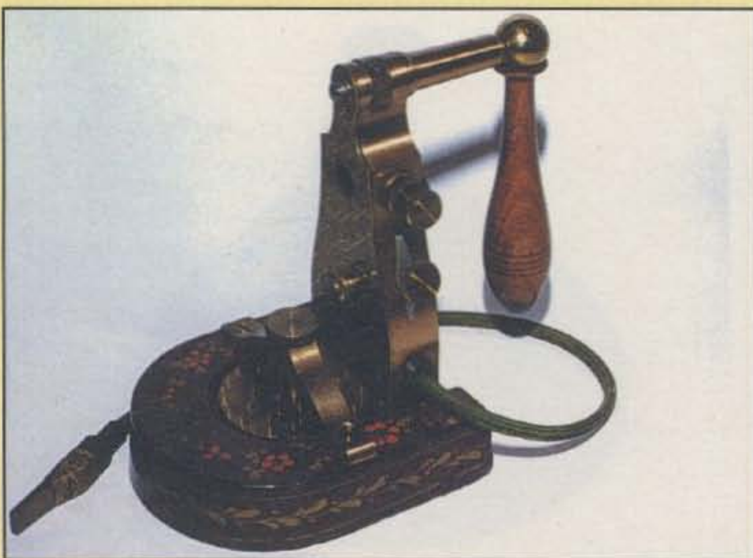
Photo 5— We nicknamed this delight a farm-boy's key or a milkmaid's key for obvious reasons. Rather than pushing down on a knob, you pull down on a lever to make dots and dashes. Every ham needs one of these pumpers for Straight Key Night! (Photo courtesy K9WDY)
