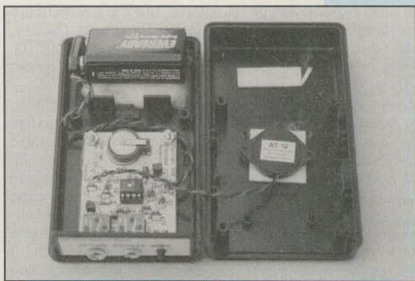
Photo 7— Interior view of new Tick EMB keyer and enclosure. Unit was assembled in only a few minutes (see text).
