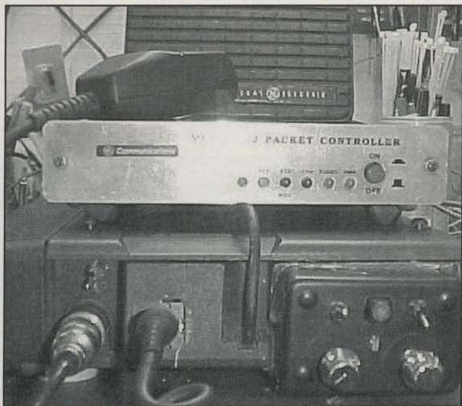
Photo M— The finished product is now a 32-channel/frequency, 6 meter transceiver capable of operating FM voice, 1200 baud AFSK, and 9600 baud DFSK packet. If you wish to acquire some of the hard-to-find parts and components for these mods, on the internet check < www.PacketRadio.com/parts.html >.
