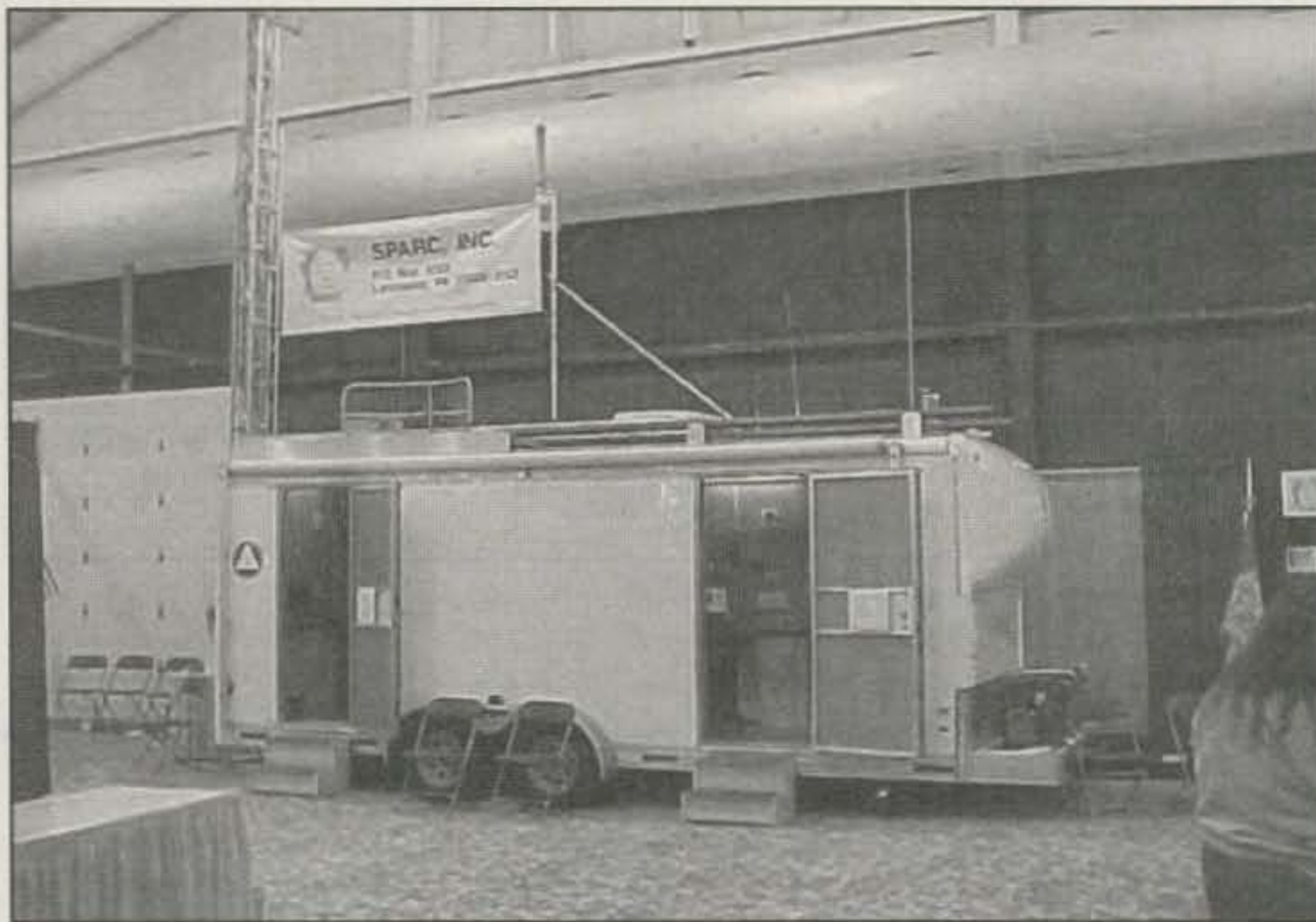
SPARC's Field Service Van was completed in just over two years. It has an attached tower and two generators for power. (Photo courtesy KA3UQA)
