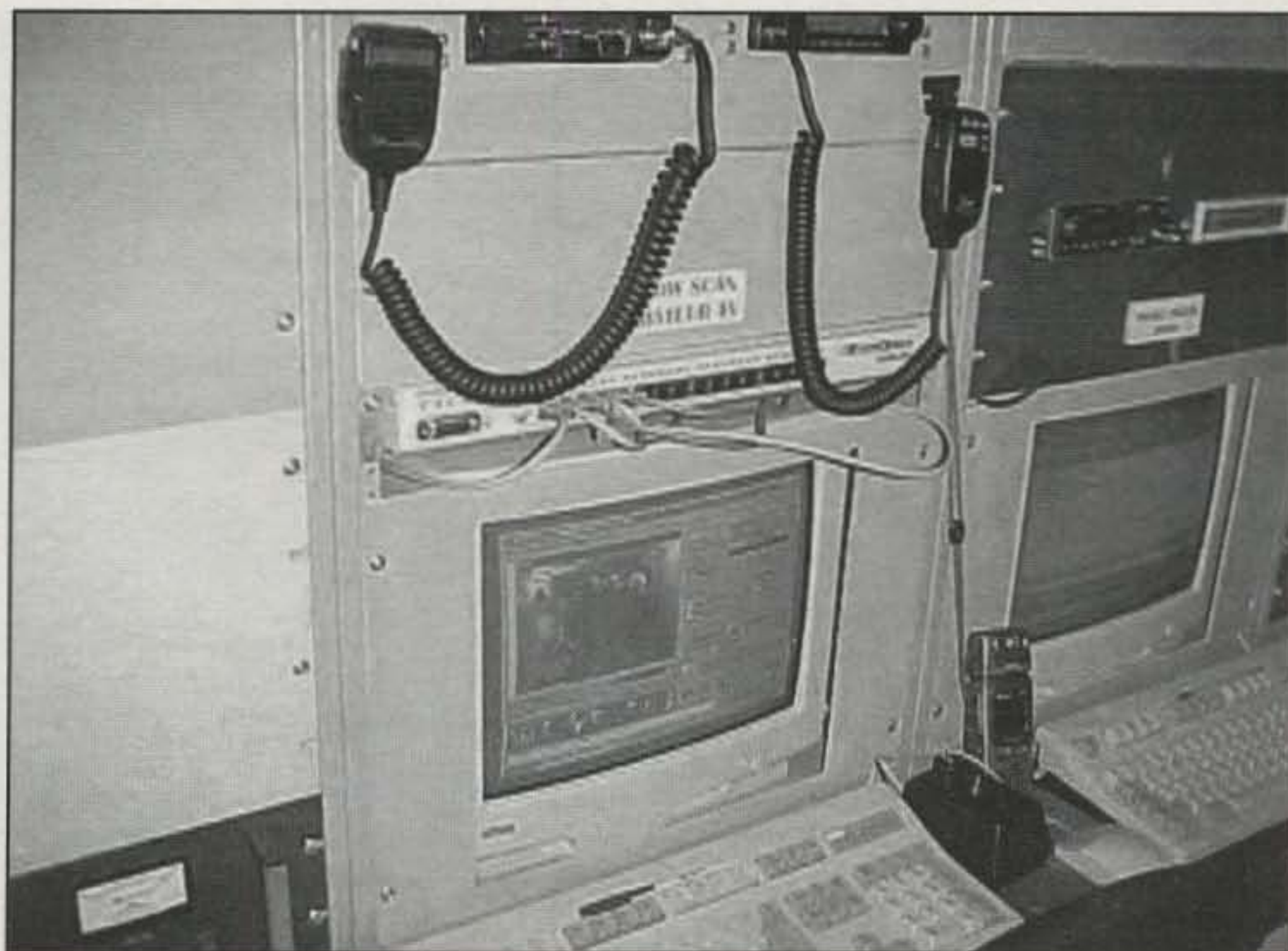
A closer look at the Slow Scan TV unit with miniature SSTV camera-modem/transceiver. (Photo by KI6NJ)
