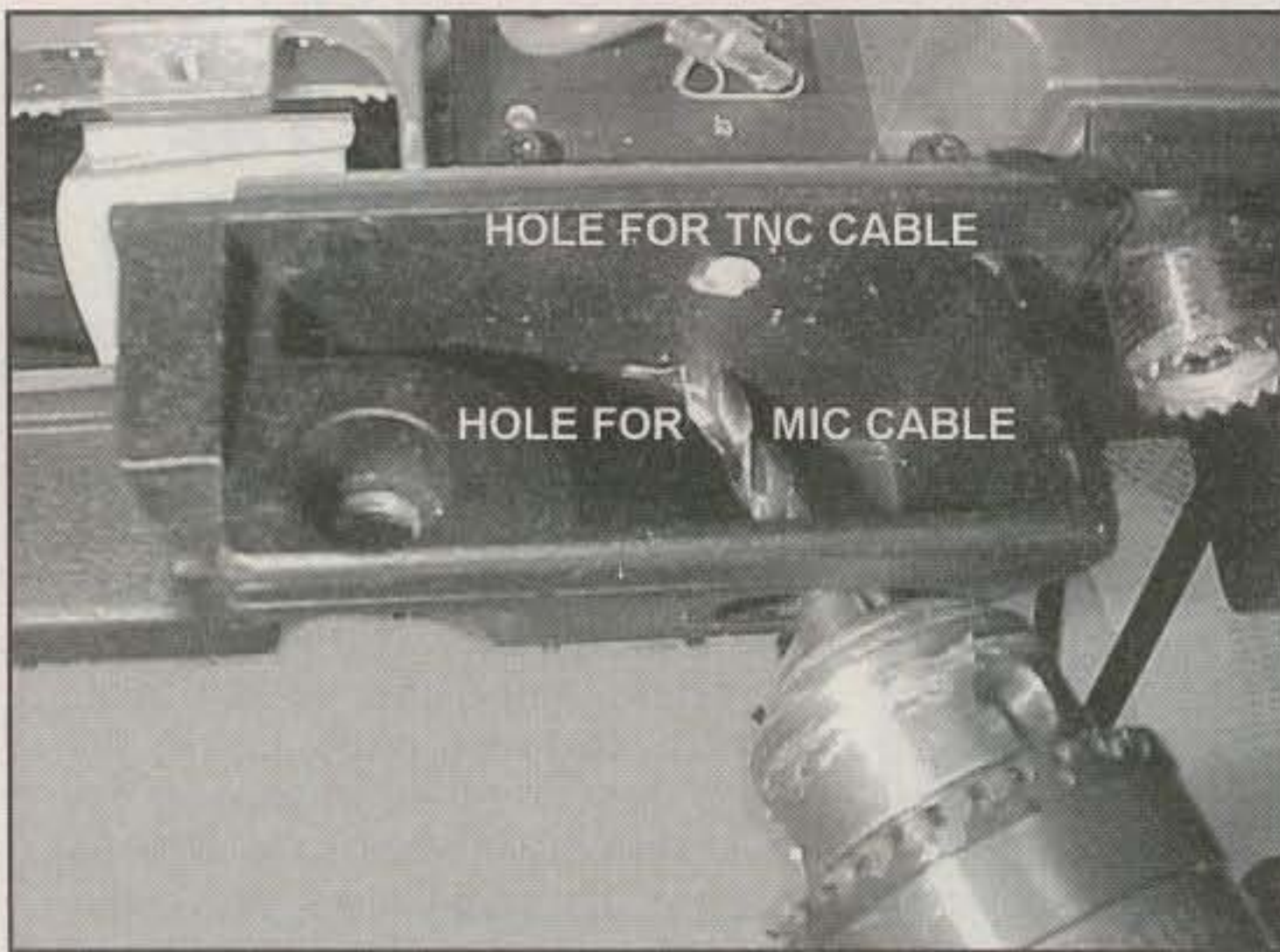
Photo A— A couple of holes up front for the microphone and TNC I/O cables. Your application may vary if you plan to use a MIC jack instead of hardwiring the mic to the RANGR.
