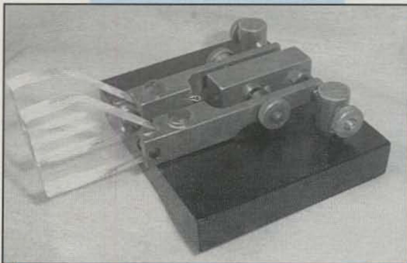
Photo 5— No springs and miniature to boot! This recently announced Vibroplex mini paddle is called the "Code Warrior Junior," and it is a commercial version of the NorCal-introduced K8FF QRP paddle. It responds to a fairly light touch and handles very well.
