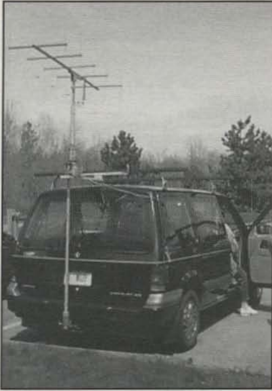
Photo 2—Fred Miller, WO2P, and Judy Stonehill, N2KXS, went transmitter hunting in style during last year's NFW with a quad and rotor on the back of their van. Jon Dickason, N2JAC, reported from the Xerox Amateur Radio Club in Fairport, New York.
