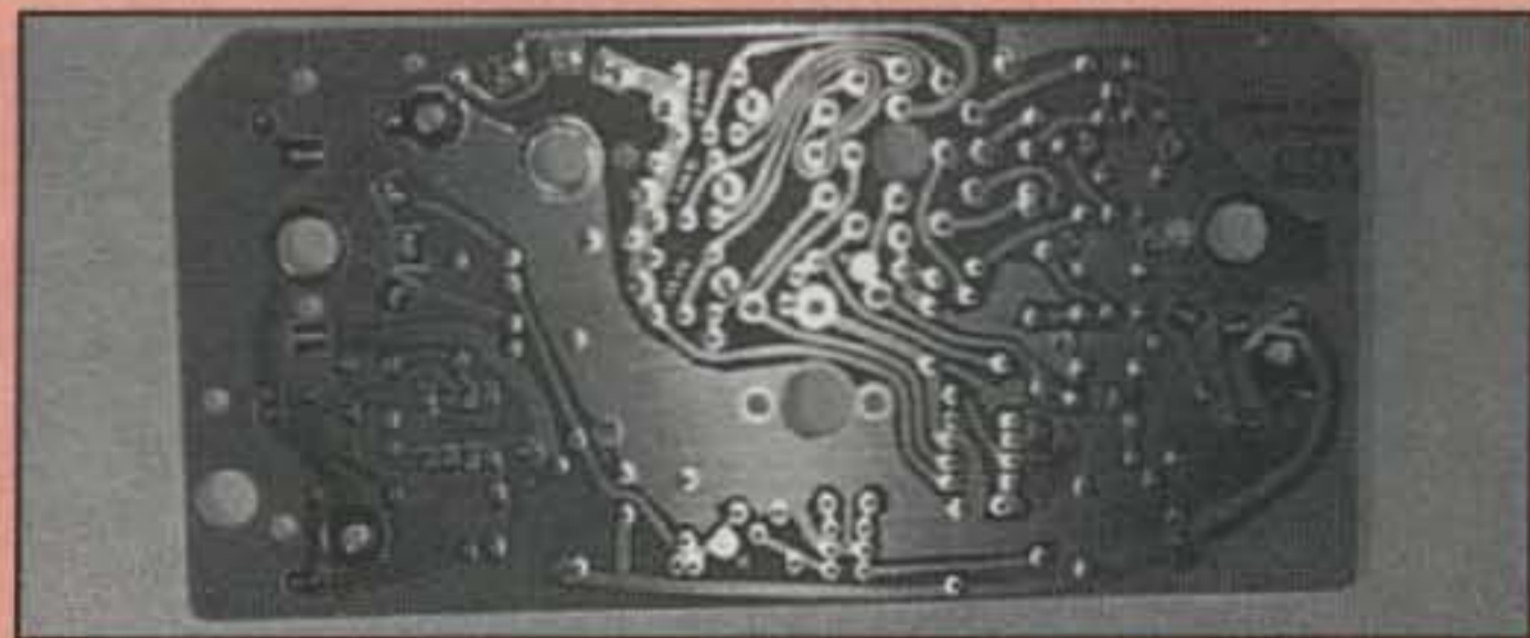
Photo C— SK205 PC board lead side showing solder resist coating.
