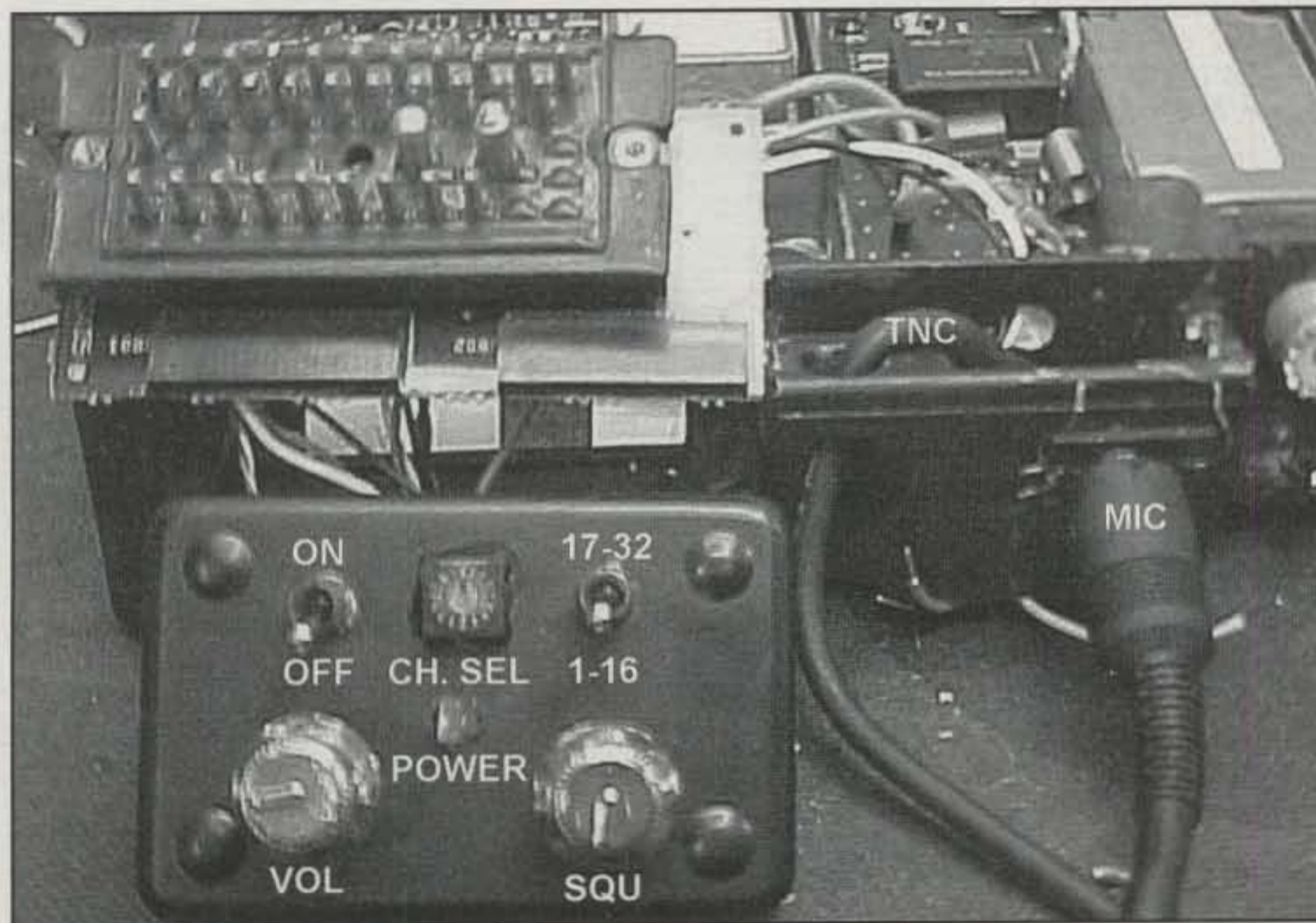
Photo E— This is a view of the condensed (mini) control head built according to the drawing at fig. 2. The mini-control head is housed in a plastic RadioShack project enclosure, P/N 270-1801.
