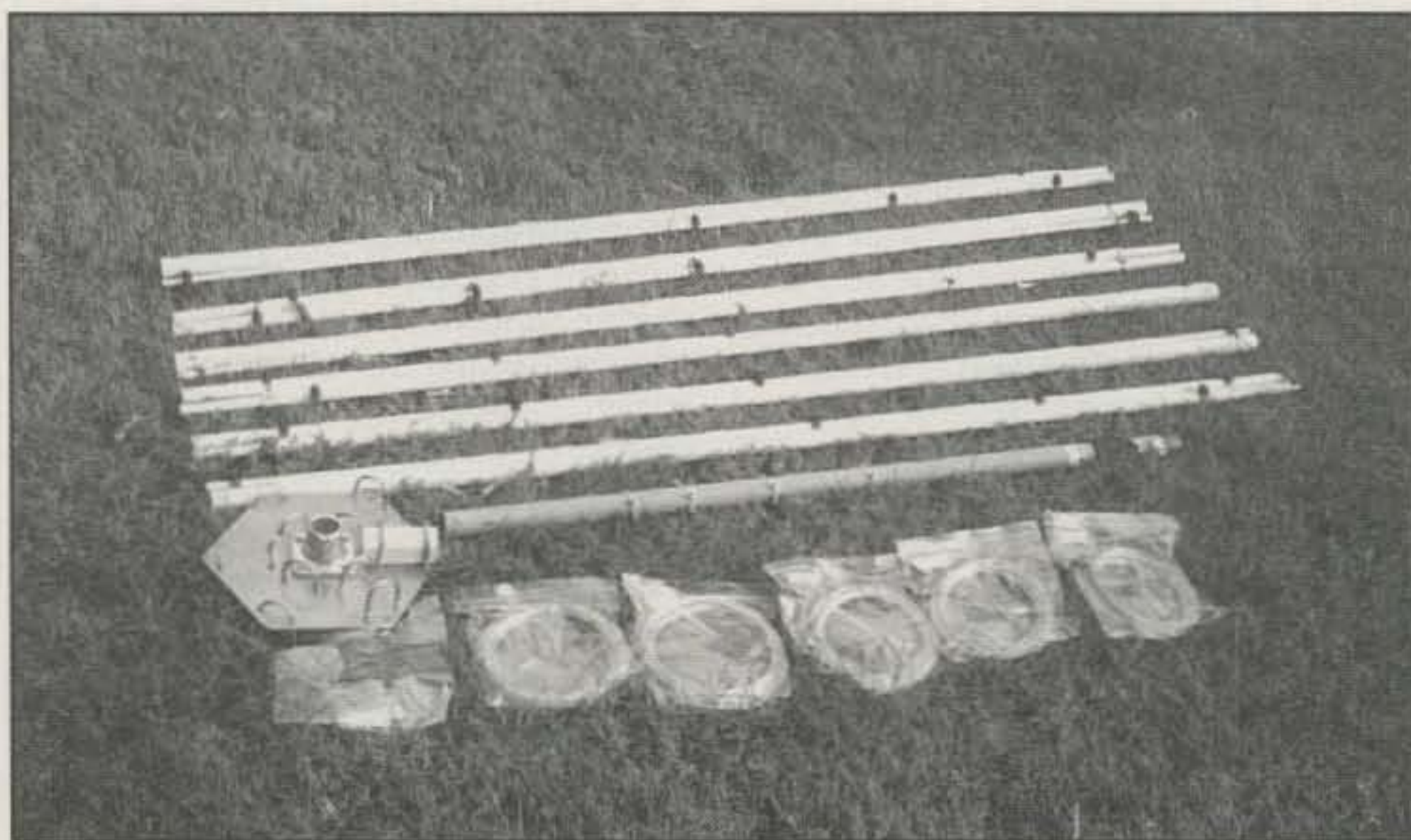
Here are the parts of the five-band HEX beam. The poly rods are of space-age technology material and are very strong. The hub, which supports the antenna, is at the bottom left.
