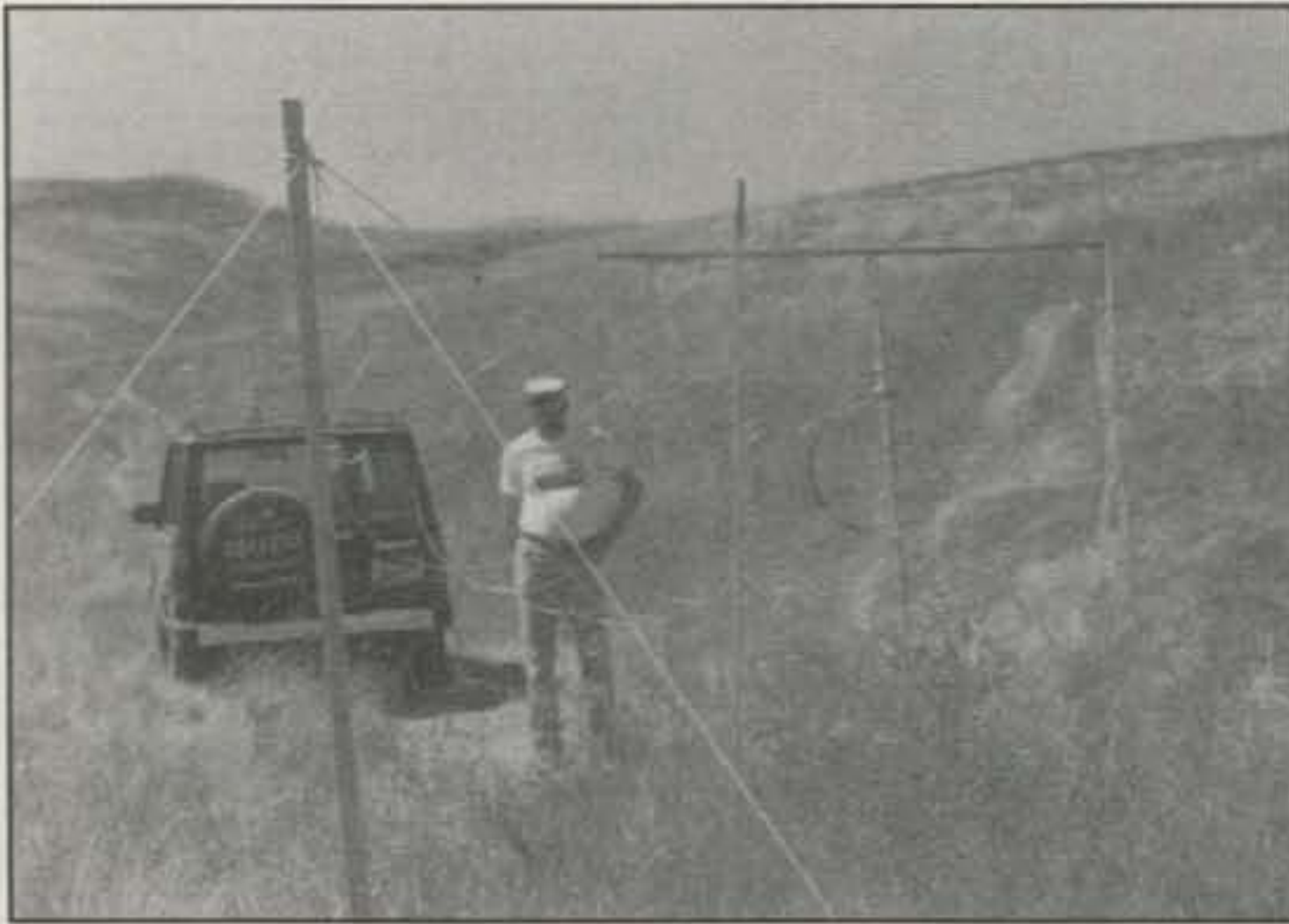
Photo 3— Gary Holoubek, WB6GCT (pictured), and Tony Levand (now AA9CC) assembled this 16-foot-long circularly polarized beam with 6 × 6 foot screen reflector in a wilderness area for a Fullerton Radio Club T-hunt a few years ago. Just as they hoped, it put lots of RF at the far end of the canyon into which it was aimed, but there was very little signal at the road just behind it. (Photo by Joe Moell, KØOV)
