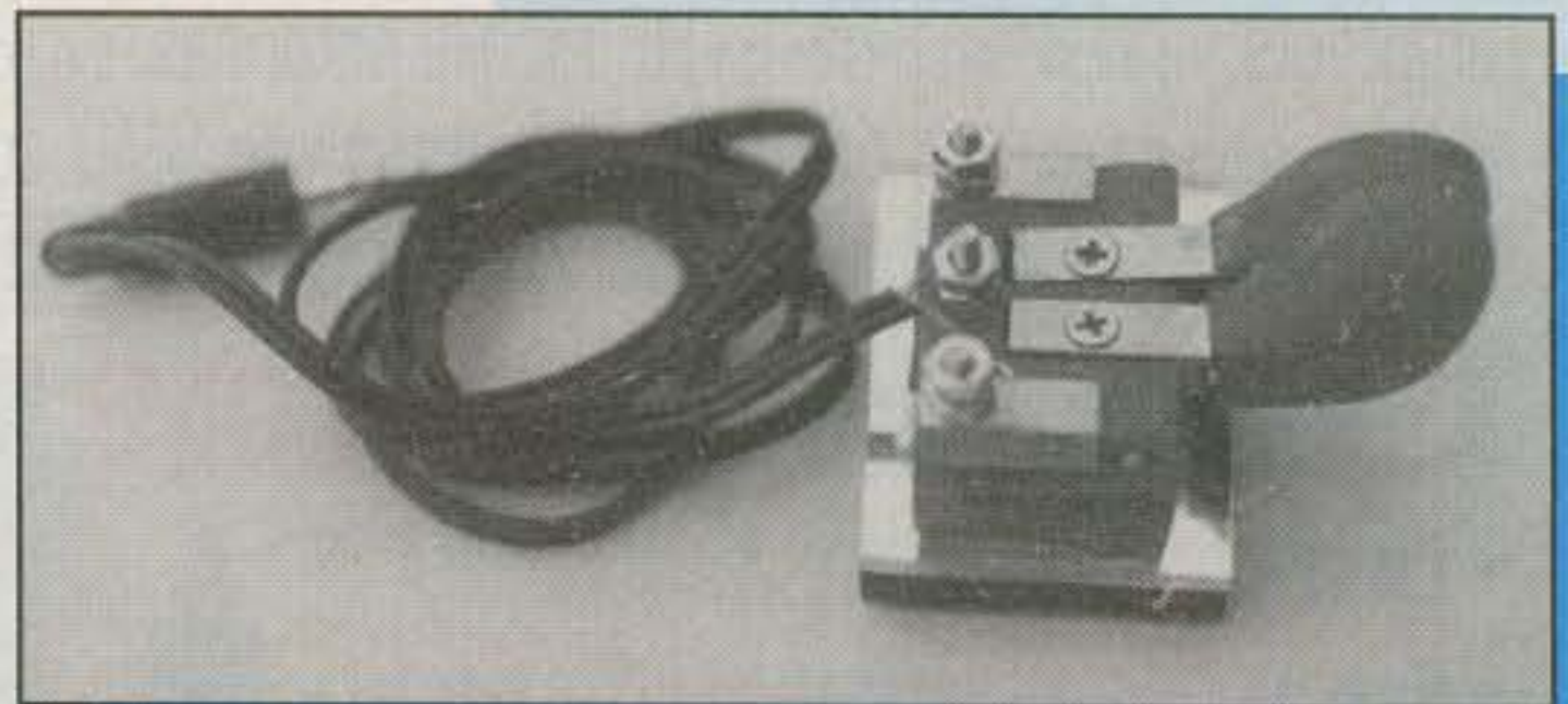
Photo 2— This good-looking brass and red-plastic paddle is made by Gil Kost, W3MKE, and is popular among QRPers nationwide. It measures 2" x 1.5" and has a medium to slightly heavy feel and a hearty "use anywhere" personality.
