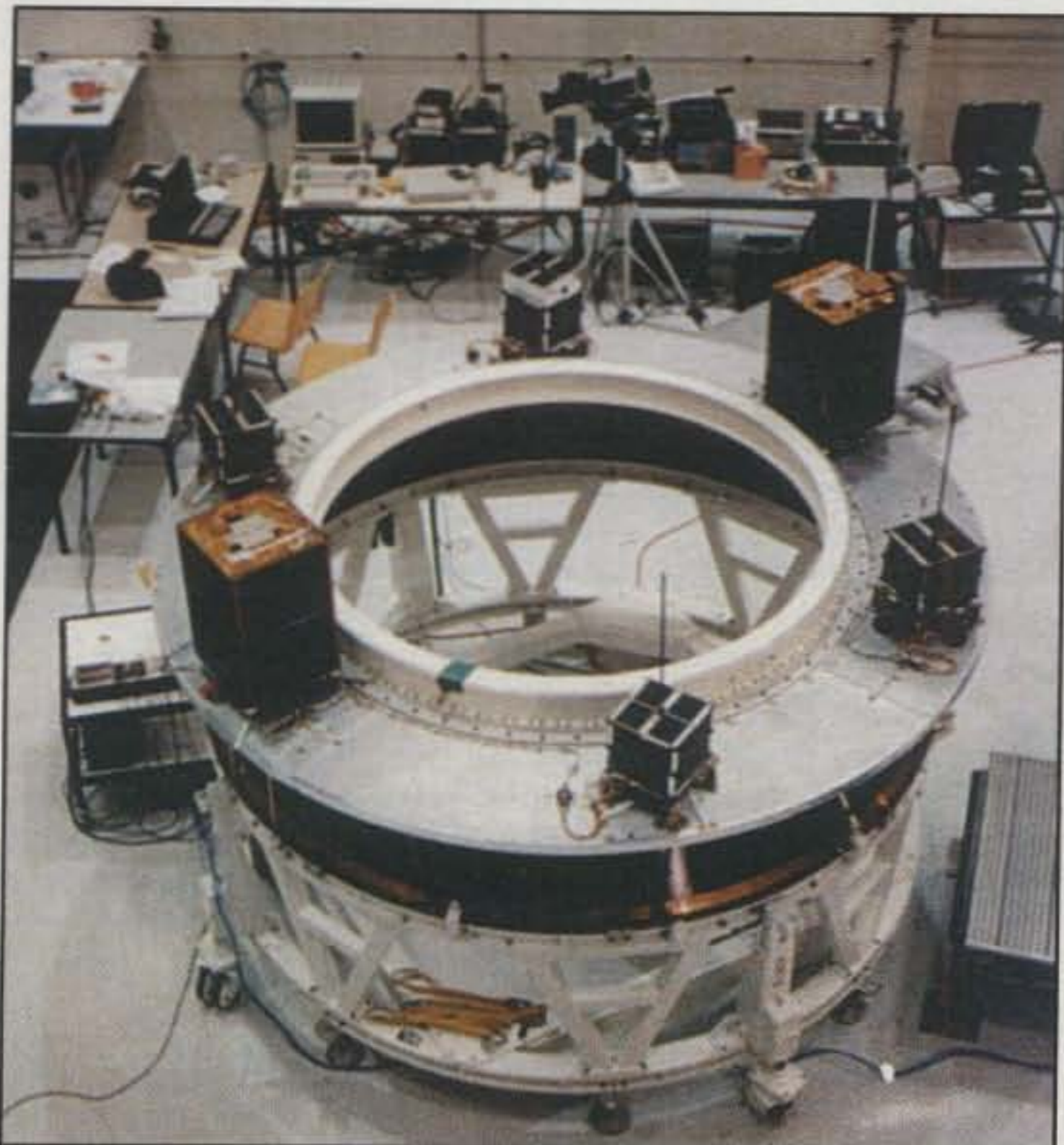
Two University of Surrey satellites, UO-14 and UO-15, and the four microsats—AO-16, DO-17, WO-18, and LO-19—on their Ariane Structure for Auxiliary Payloads (ASAP) before mating with the primary payload. (Courtesy Arianespace)
