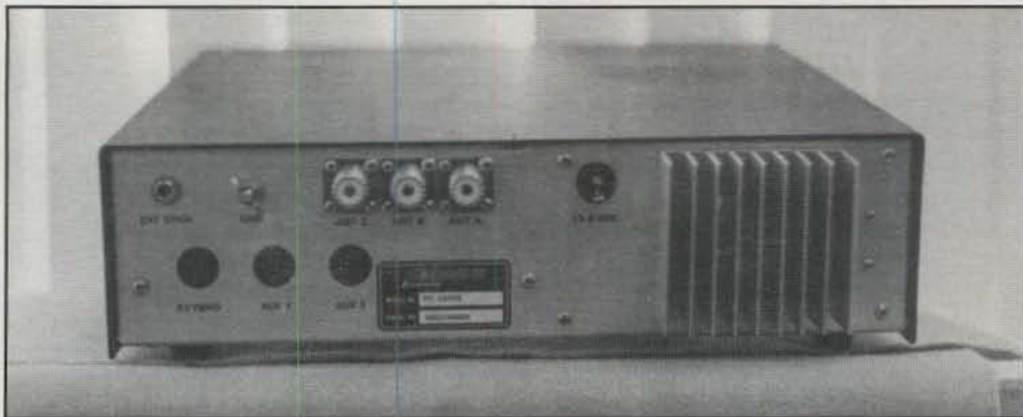
Rear view of the unit shows a nice, simple layout along with a decent-size heat sink. There are no fans on this unit, and it doesn't need any. Note the three antenna inputs, which are selectable from the front panel. The cable for the supplied keyboard plugs into the jack shown on the far left in the photo.
