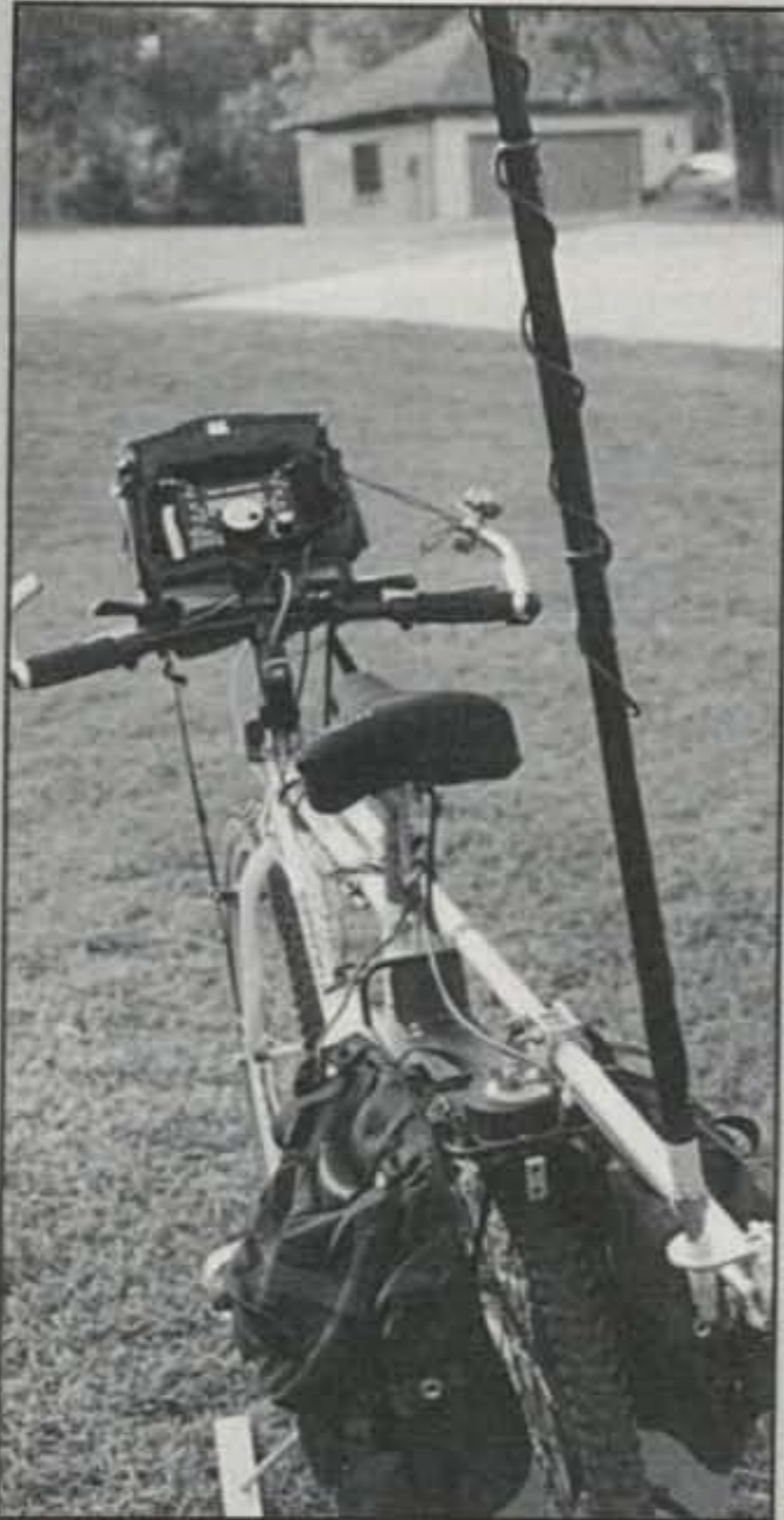
Photo 3— This rear view shows the Outbacker, its mount, and the extension tube from another angle. Notice the PL259 at the antenna's base for quick removal. Look carefully, and you can see the antenna and battery cables secured to the frame.
