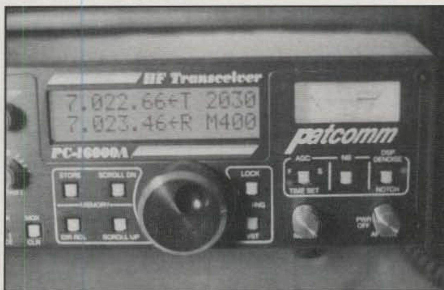
The two-line display on the PC-16000A is larger than on the original PC-16000. In "split" operation, the display shows transmit frequency on the top line and receive frequency below. Decoded CW and RTTY signals also scroll across this screen.
