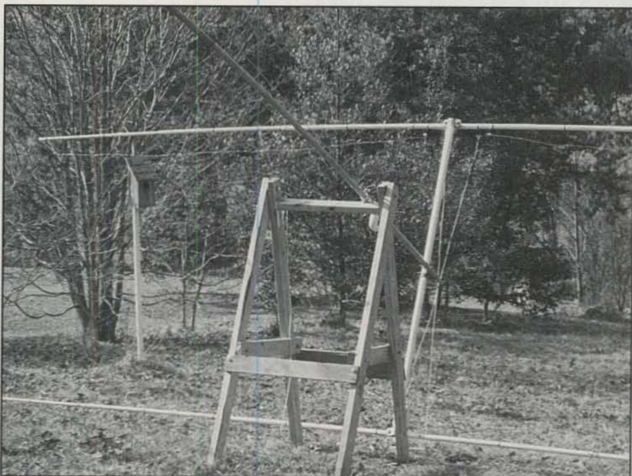
Photo C— The D2T mounted to the test mast prior to raising for tests.
