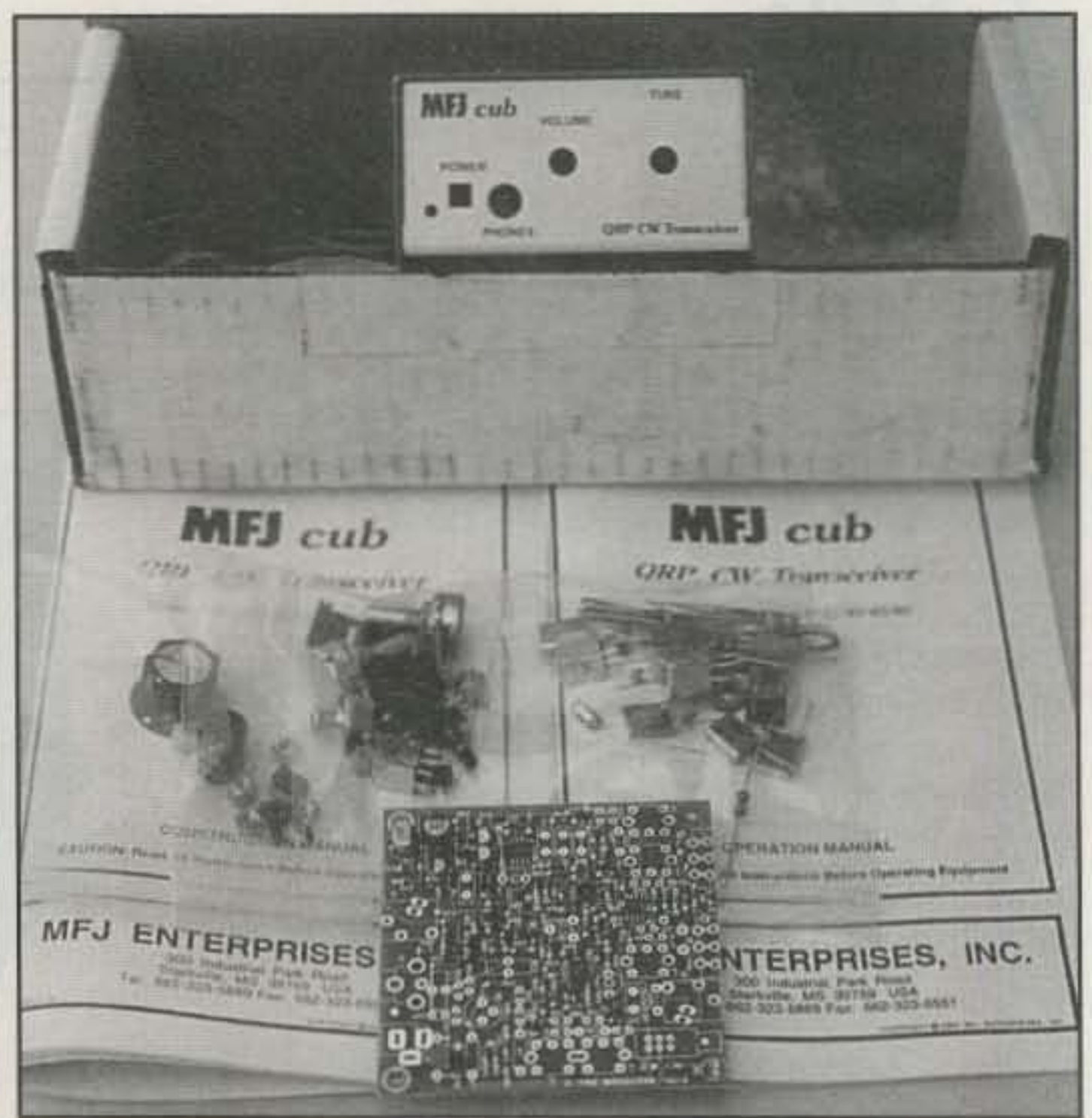
Photo 3— Here you see the Cub as received and laid out for assembly. The kit's parts are contained in three clear bags: knobs and mounting hardware, controls and connectors, and band-related components. The manual shown on the left explains assembly, while the one on the right describes operation.
