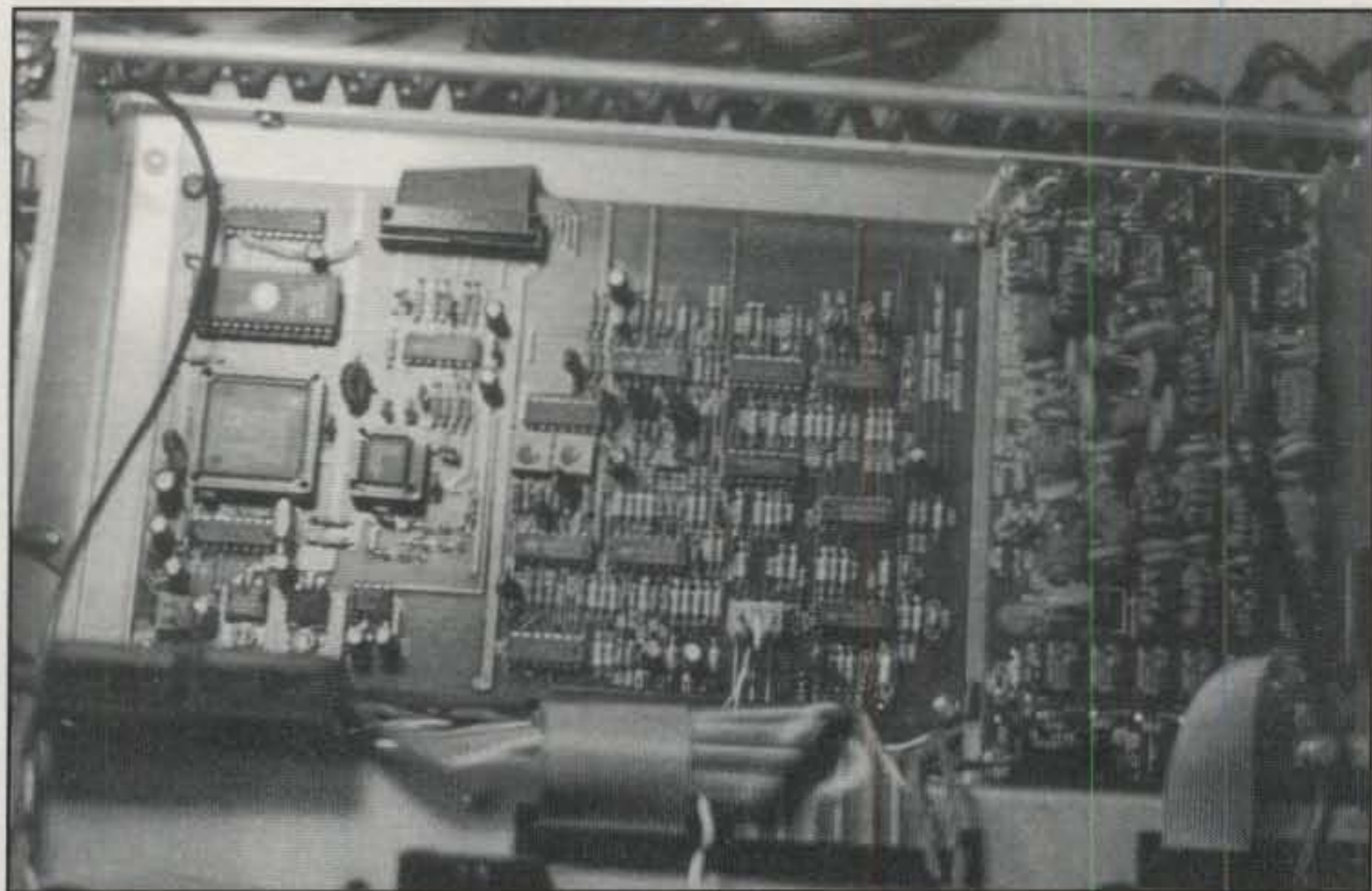
The inside of the unit shows surface-mount technology and a neatly arranged layout. Patcomm prides itself on its quality control.
