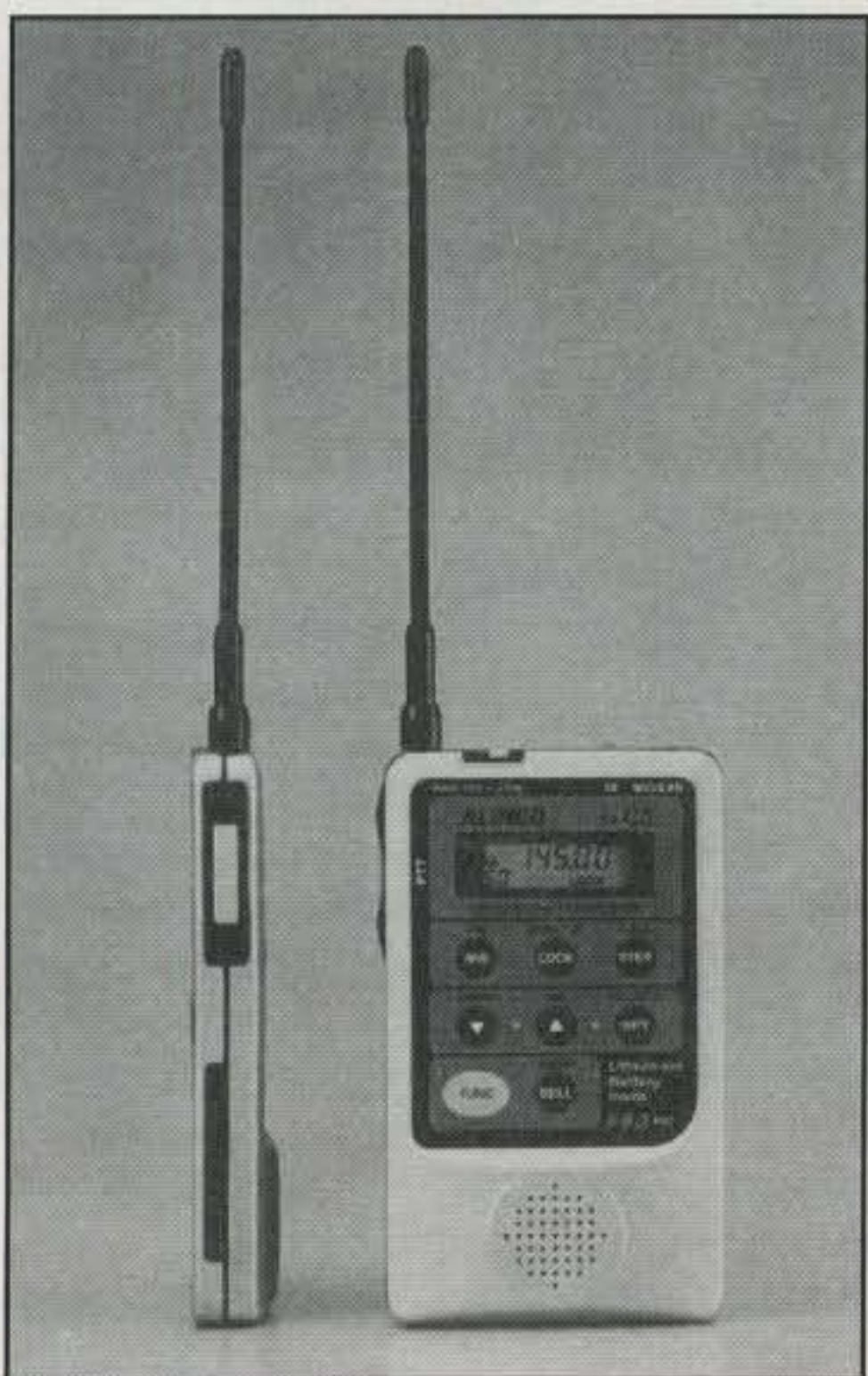
They don't get much cuter than the Alinco DJ-C5, a nearly credit-card-sized two-band handheld. It does have a fixed antenna, and only puts out a half watt, but it has broad receive coverage and 50 memories. Not bad for something that will slip into your purse or shirt pocket. (Courtesy Alinco USA)
