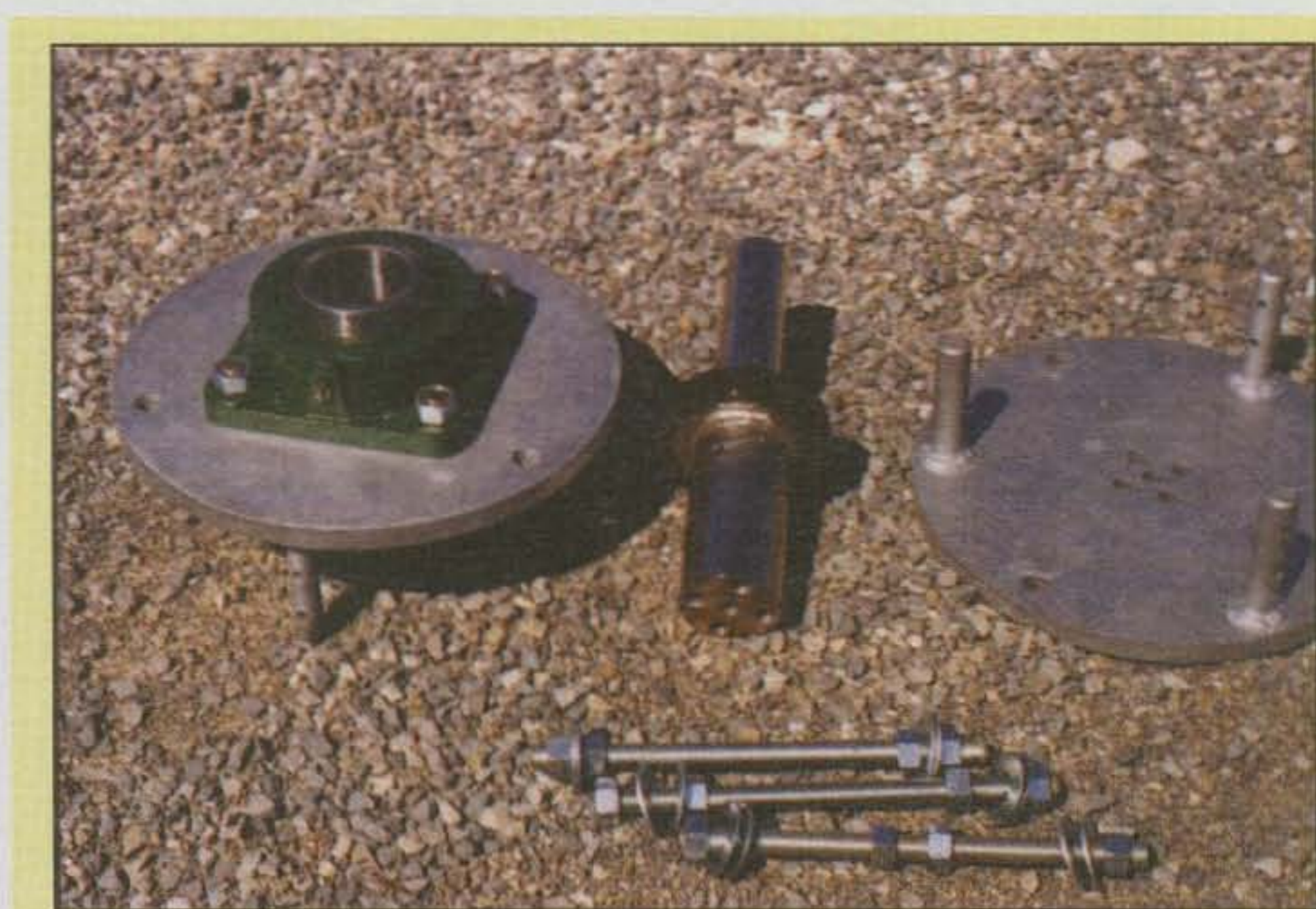
Photo 1—Components of the main rotating bearing assembly of the Rotating Tower System (RTS) designed by Dick Weber, K5IU. (Photos by the author)
