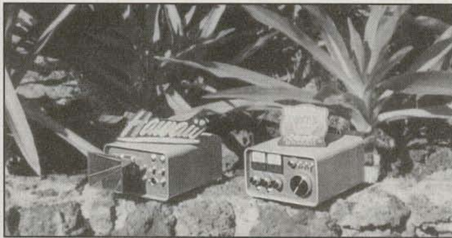
10 GHz Gunn-Plexers ready to go, in pursuit of volcanic-ash-scatter contacts from Hawaii. (Photos courtesy of the author)
