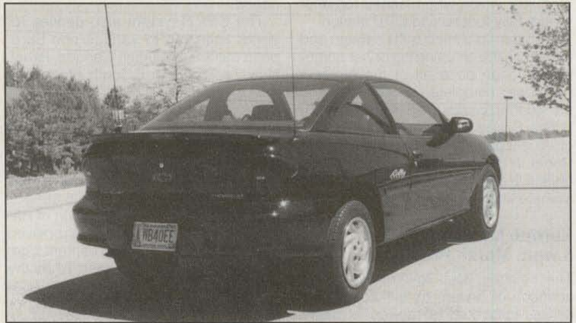
Photo A— HF mobiling with a small, clean-looking antenna system gives you the ability to work the world while maintaining a mild-mannered appearance. The setup shown here is a 4 foot tall mini-Hustler on a trunk mount. The antenna is painted to match the car, resulting in a "natural looking" setup with worldwide range.
