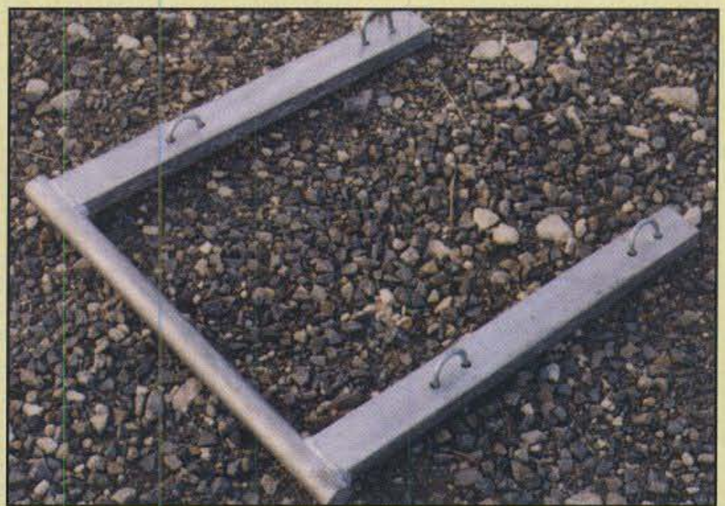
Photo 4— Gin-pole adapter designed to permit you to work around the guy ring. Photo 5 shows it in use on the tower.
