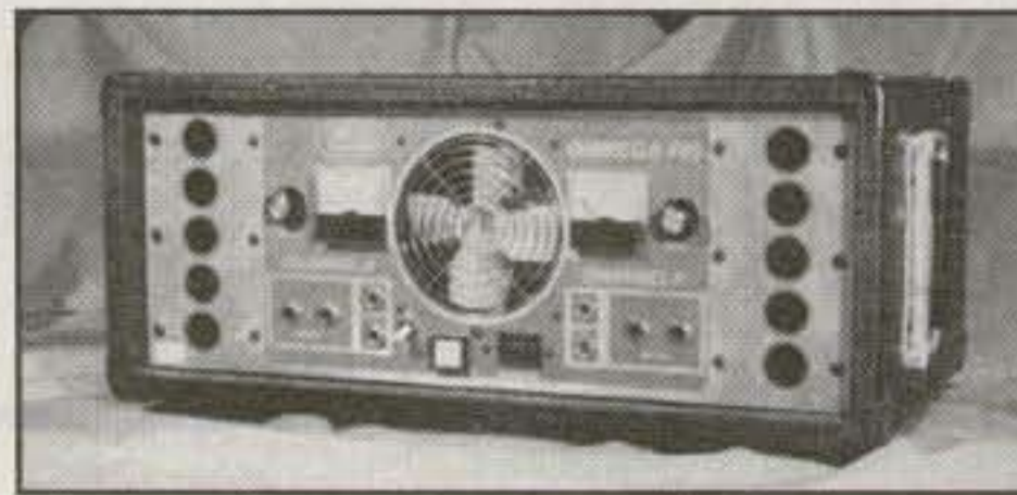
Photo A— Most stand-alone audio amplifiers are designed to boost microphone levels to room-filling volume. This famous Heil sound amplifier serves that purpose in high style. It is a 400 watt, full-range unit made by Bob Heil, K9EID, and used by several top bands during the early days of rock 'n roll. It also launched Bob's career in top-grade sound equipment. (Photo courtesy K9EID)
