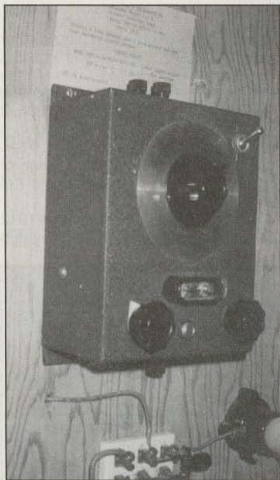
Photo D— This Mackay Radio and Telegraph Co. model 123 crystal set was designed for emergency ship-board use during eras past and tunes the international distress frequency range of 350 to 550 kHz. Proud owner Henry Johnson, K4IP, restored it to like-new condition and mounted it on his ham shack wall, where it captures every visitor’s attention. (Photo courtesy K4IPY)
