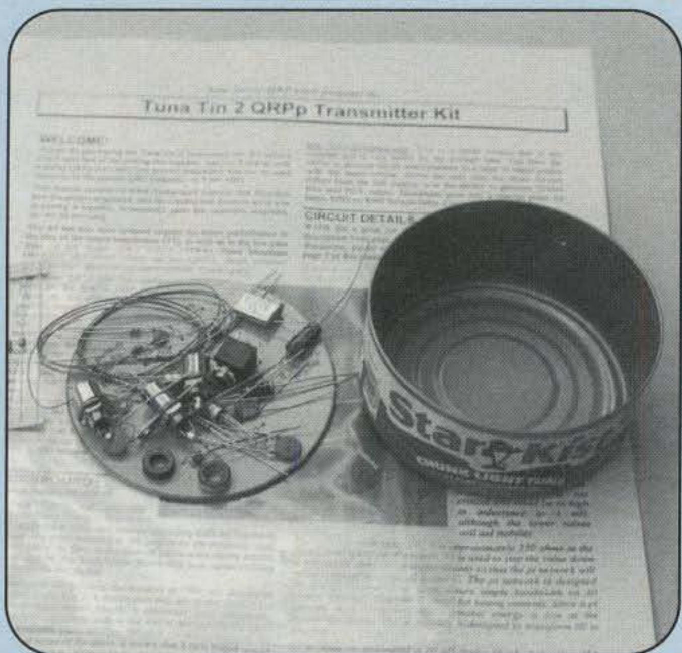
Photo C— It's back! This "25 years later" version of the legendary W1FB Tuna Tin 2 Transmitter is updated with toroid coils, supplied with a 7040 kHz crystal, and pumps out a healthy 400 milliwatt signal. It mounts on a tuna-can chassis (not supplied) and is available as a quick-brew kit from the New Jersey QRP Club for $12.
