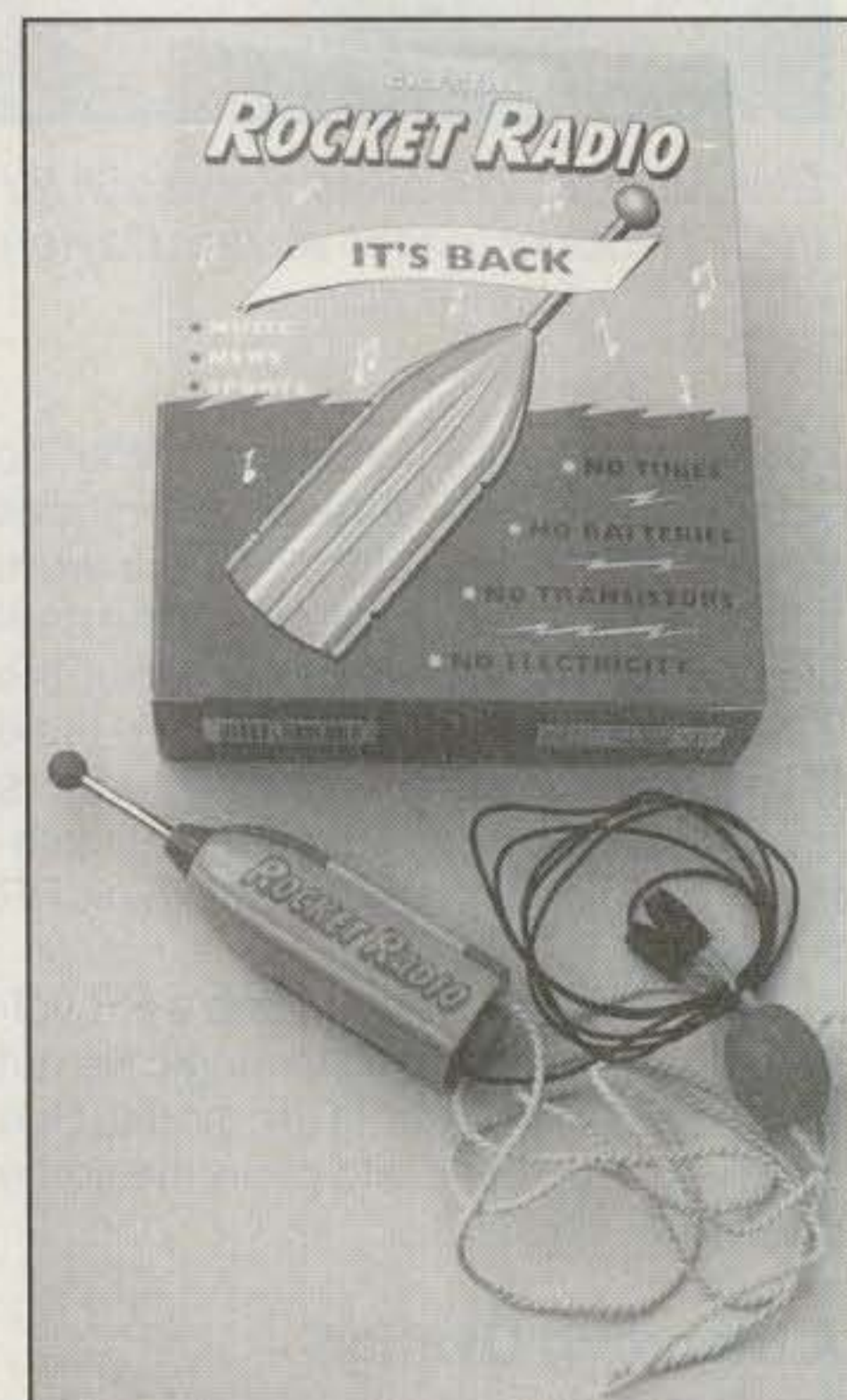
Photo A—One of the most popular crystal sets of all times is the famous Rocket Radio of the 1950s. This pocket-size wonder worked great with almost any makeshift antenna and no ground. The sliding "Space Probe" on nose cone was used for tuning. Exact reproductions of the Rocket Radio are available from Restoration Hardware stores.
