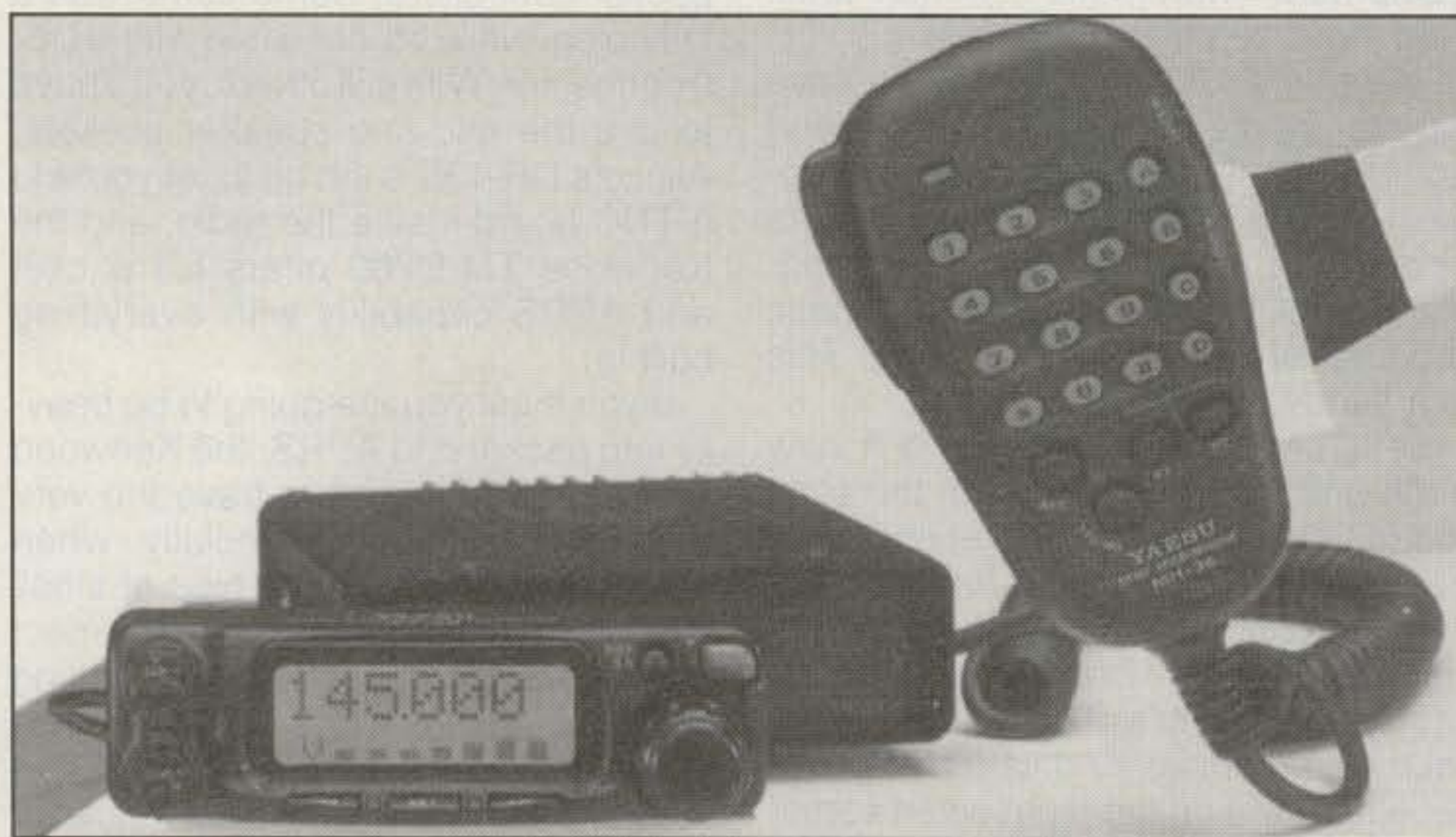
The Yaesu FT-90R two-band transceiver offers two bands, but only one at a time may be operated. With only one band showing at a time, you know exactly what you're doing at a glance when zipping down the highway.
