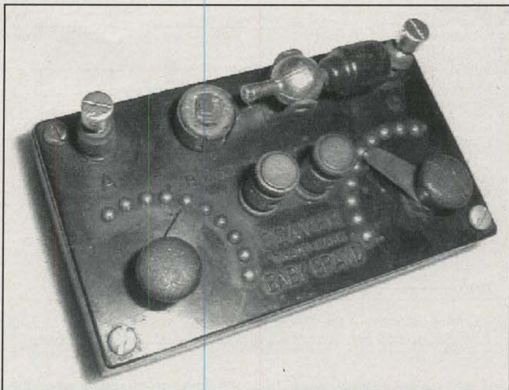
Photo B—Roaring back from the 1920s is this original Beaver Baby Grand crystal set made by the B M & T Co. of California. It sports a multi-tap coil for tuning and matching various antennas and a galena-and-catwhisker detector. This particular set has seen extensive use over the years but still works. (Photo courtesy owner W6BNB)
