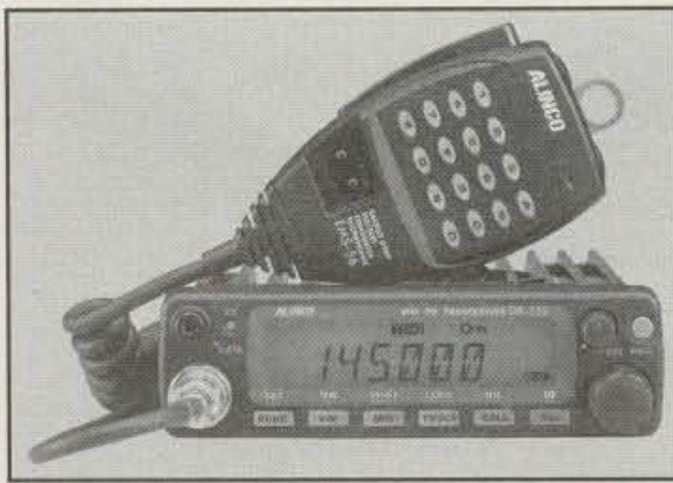
Alinco's DR-135 is set up to let you add a TNC board inside the radio.
