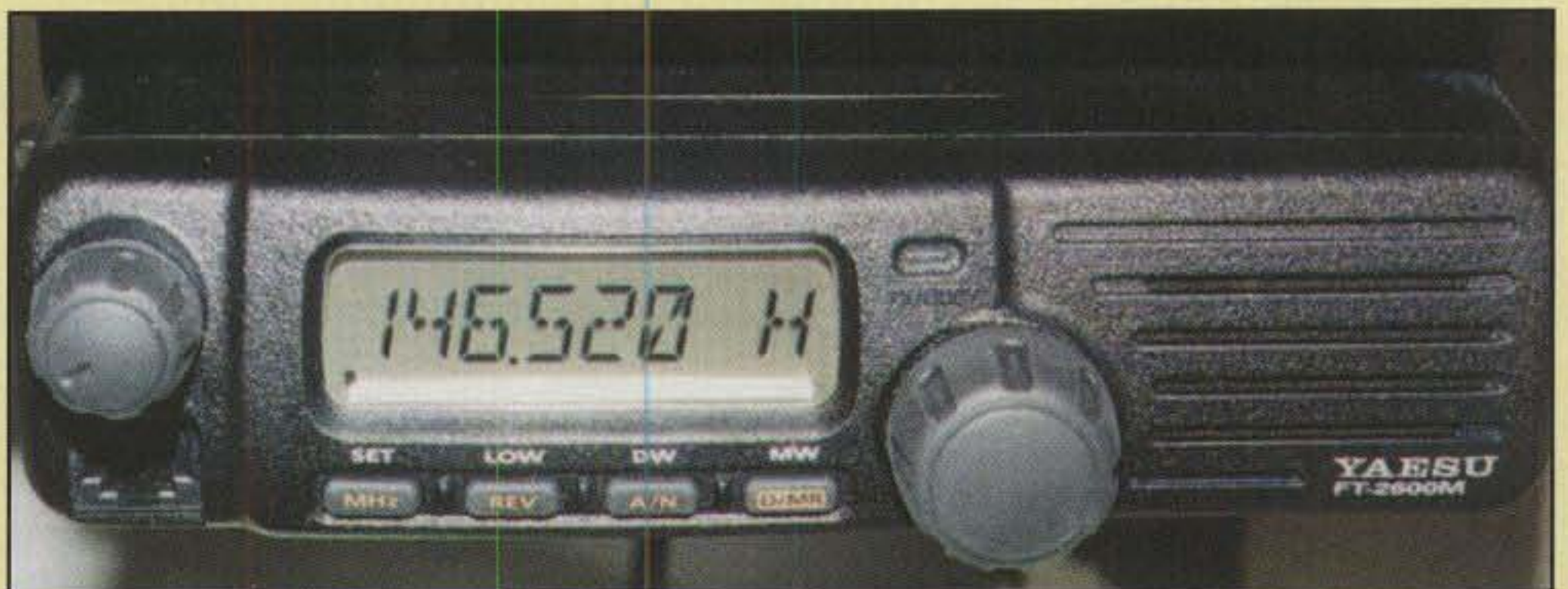
The heavy-duty Yaesu FT-2600M has a speaker that comes right out the front. Although it's a single-bander, it's built like the Yaesu land-mobile line and works well.
