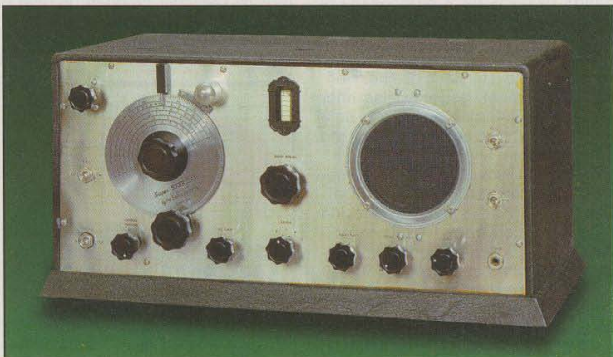
The Hallicrafters SX-9 receiver pictured here is a prototype. It differs slightly in appearance from those made in both early and late production runs. (Photos by Joe Veras, N4QB)
