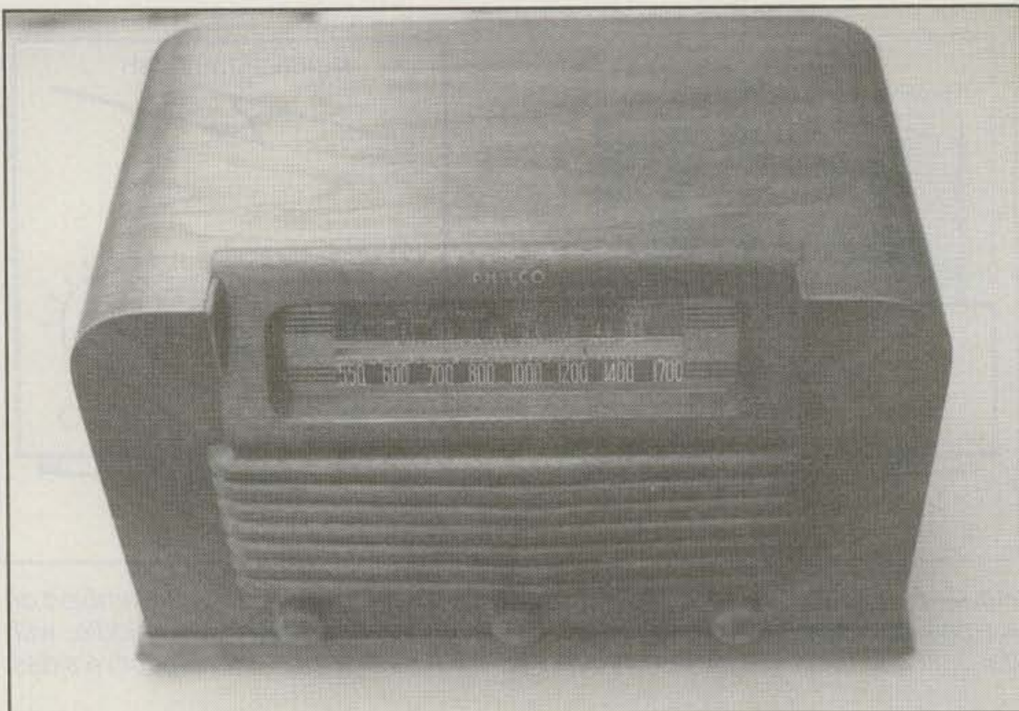
Photo B— Looking for a novel idea? Assemble the Minnie rush-rush on a defunct AM radio's chassis, include extra audio and RF amplifier stages, and you have a ham rig that looks like—a radio!
