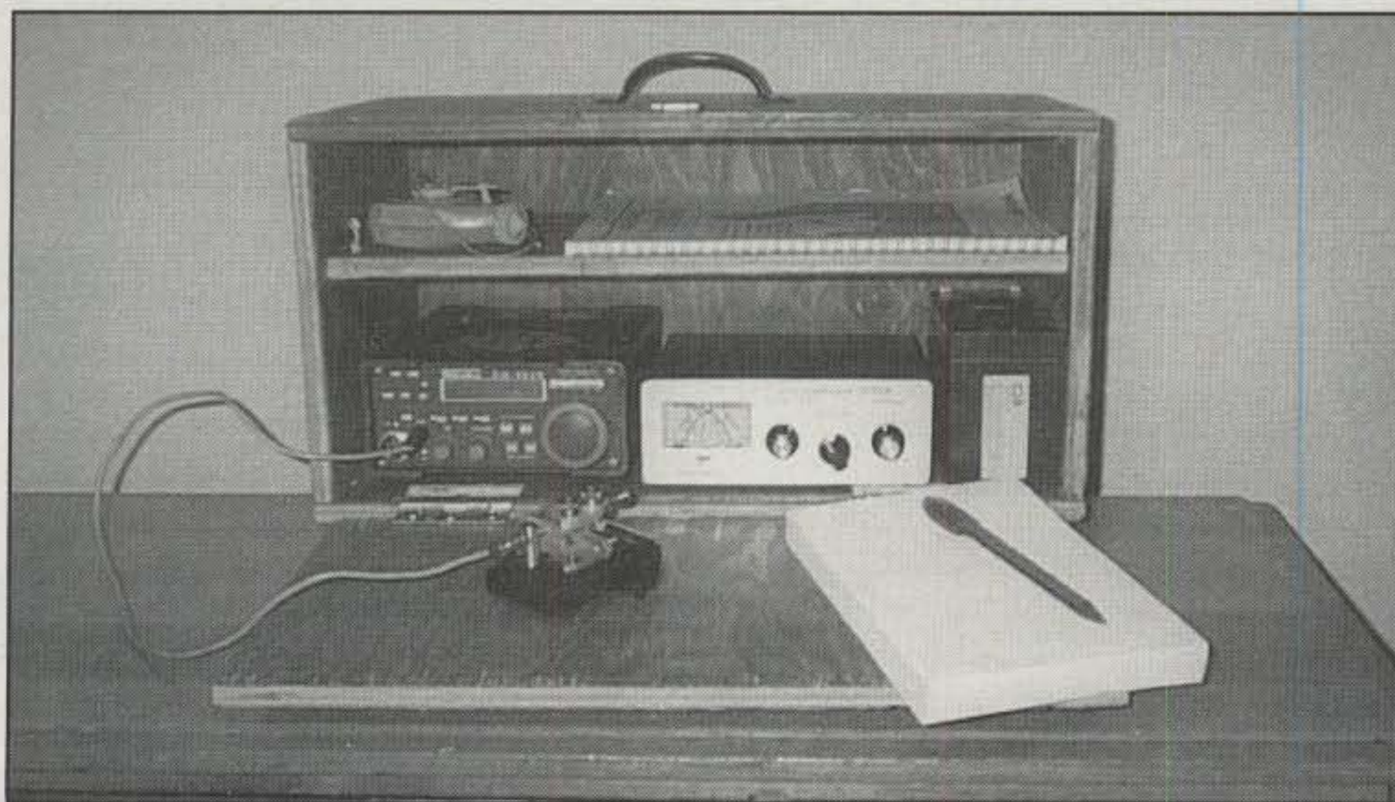
Photo 3— Have QRP, will travel! This go-anywhere mini-rig cabinet was made by Dick Swanson, KØRDS, and it turns any tabletop or campsite into an instant ready-to-operate QRP station. The cabinet is a scant 9 inches high by 17 inches wide and has a swing-down front cover plus slip on/off base support section.
