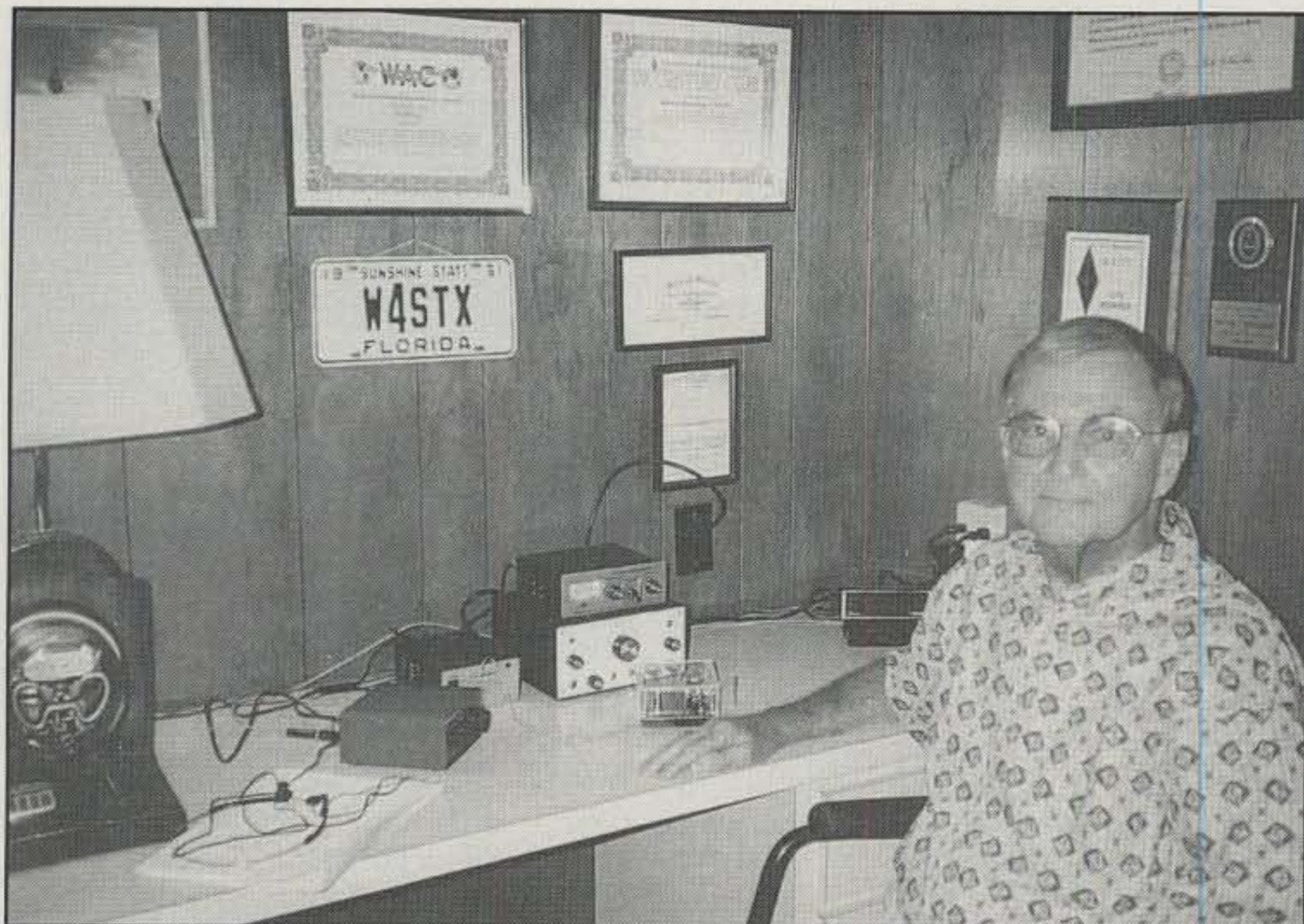
Photo 2— How do you spot a big-time QRP station? By its lack of large transceivers, naturally! Here, for example, Bill Penhallegon, W4STX, shows us his prescription for QRP happiness with a white-faced Oak Hills Research transceiver, MFJ antenna tuner, small AC power supply, and (between the Oak Hill Research transceiver and desk lamp) a new red-case, Red Hot Radio, 20 meter mini-transceiver. As discussed in the text, Bill's setup gives a good account of itself on the air.
