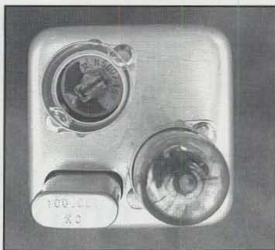
Overhead view shows the trimmer capacitor does line up inside the unused tube socket hole, and the crystal is securely held in the new opening.
