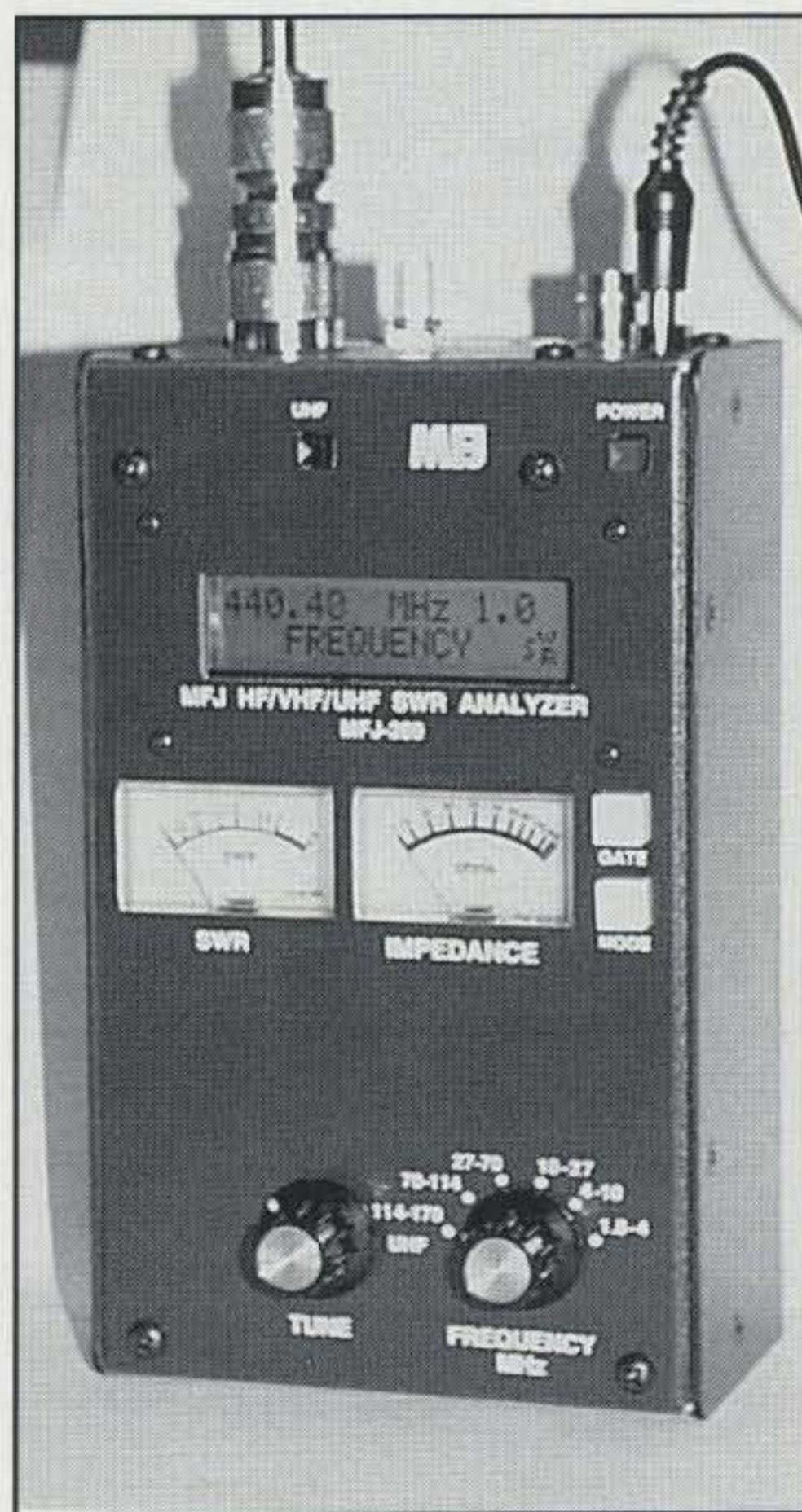
MFJ's fully portable HF/VHF plus UHF MFJ-269 SWR analyzer covers 1.8–170 MHz and 415–470 MHz and includes all of the features of the popular MFJ-259B. (Photo courtesy MFJ Enterprises, Inc.)
