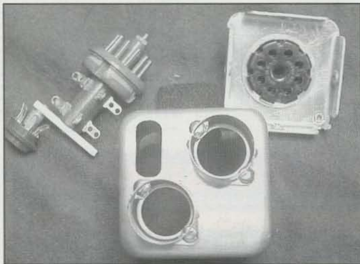
"Major" components of the Cali-Kit: The original turret with one tube socket removed. The base has a new 8-pin octal plug installed. The top case has the two original tube socket holes, and a new crystal clearance hole.
