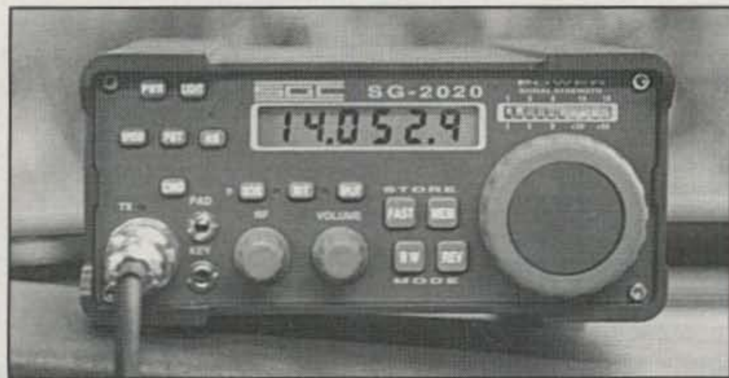
Photo 1—The SGC-2020 is a neat little transceiver for multiband SSB QRP'n. It is small, rugged, energy efficient, and loaded with deluxe operating features. (Photo courtesy SGC Corp.)
