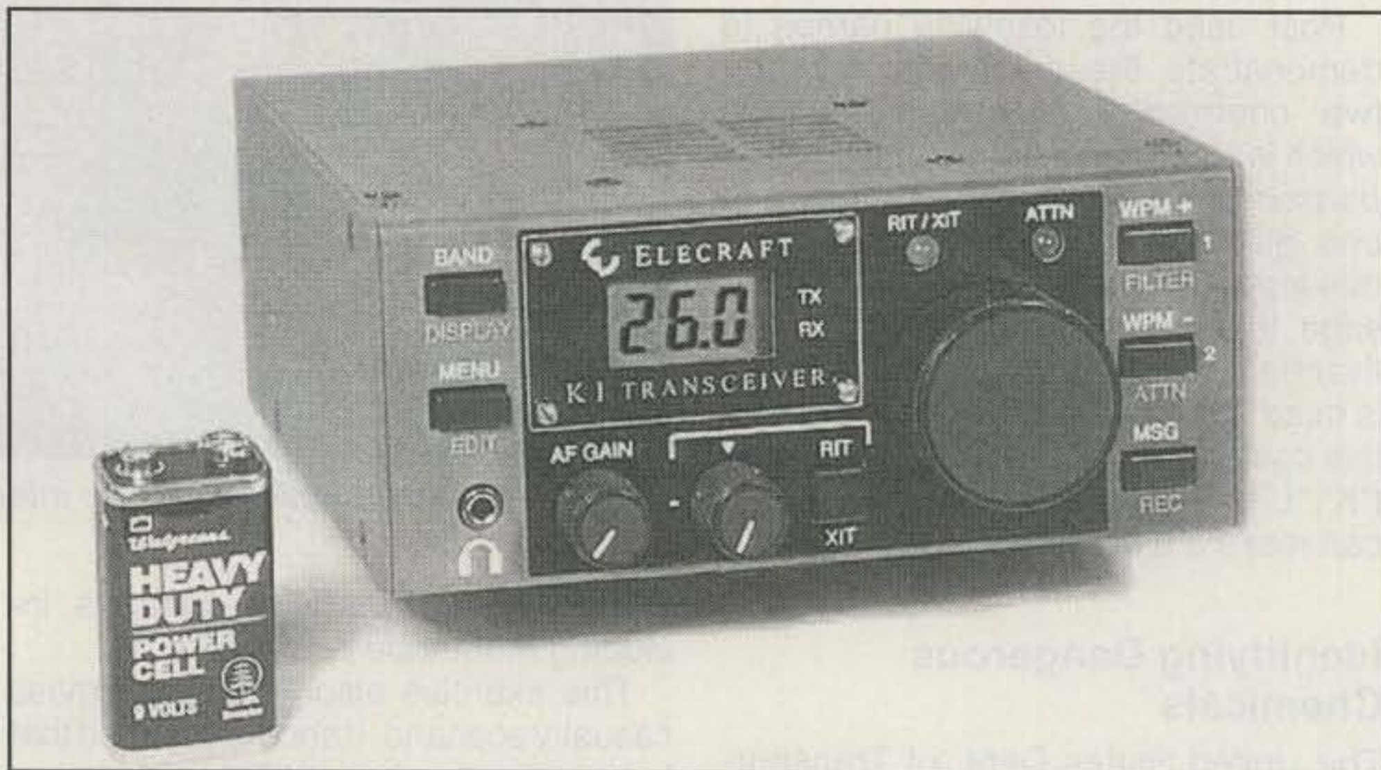
Photo A— Elecraft has followed the launch of its popular K2 transceiver with the K1, a compact, dual-band HF transceiver. As small as a traditional QRP monobander, but packing many of the features of the K2, the new radio runs up to 5 watts CW on two user-selected bands. The new rig is said to take small, backpack-friendly QRP transceivers to a new level. (Photo courtesy Elecraft LLC)
