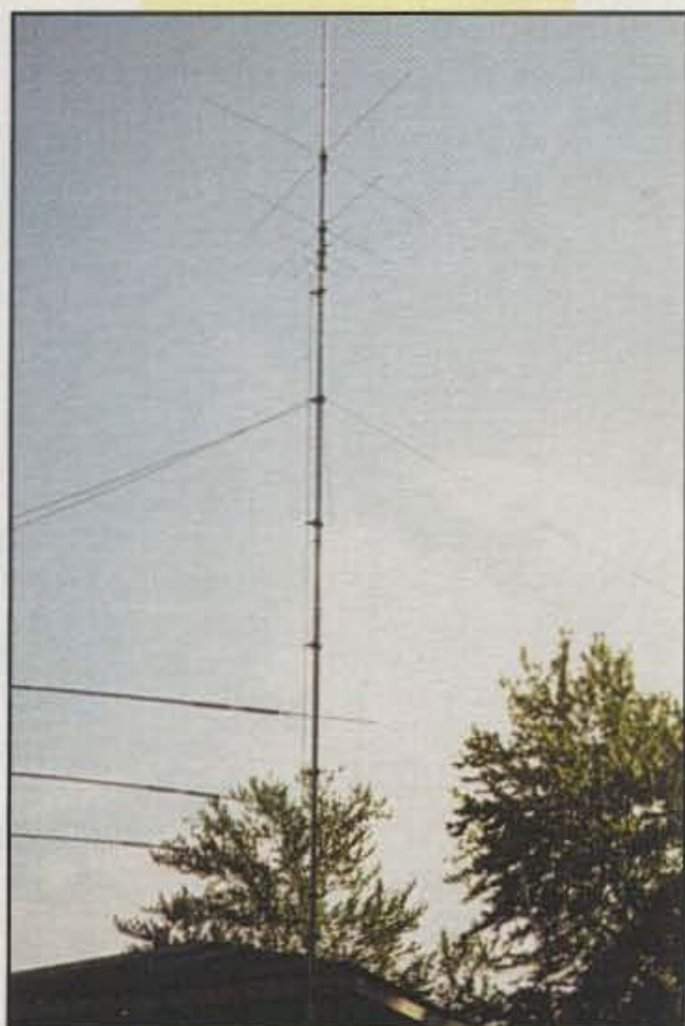
Photo 4— Thinking about an easy-up antenna that will give your station big signal clout? Hy-Gain's new 3/8 -wave and ground-independent AV-640 gets our vote. The vertical covers 40 through 6 meters with low SWR and exceptionally wide bandwidth and "works out" like a champ.
