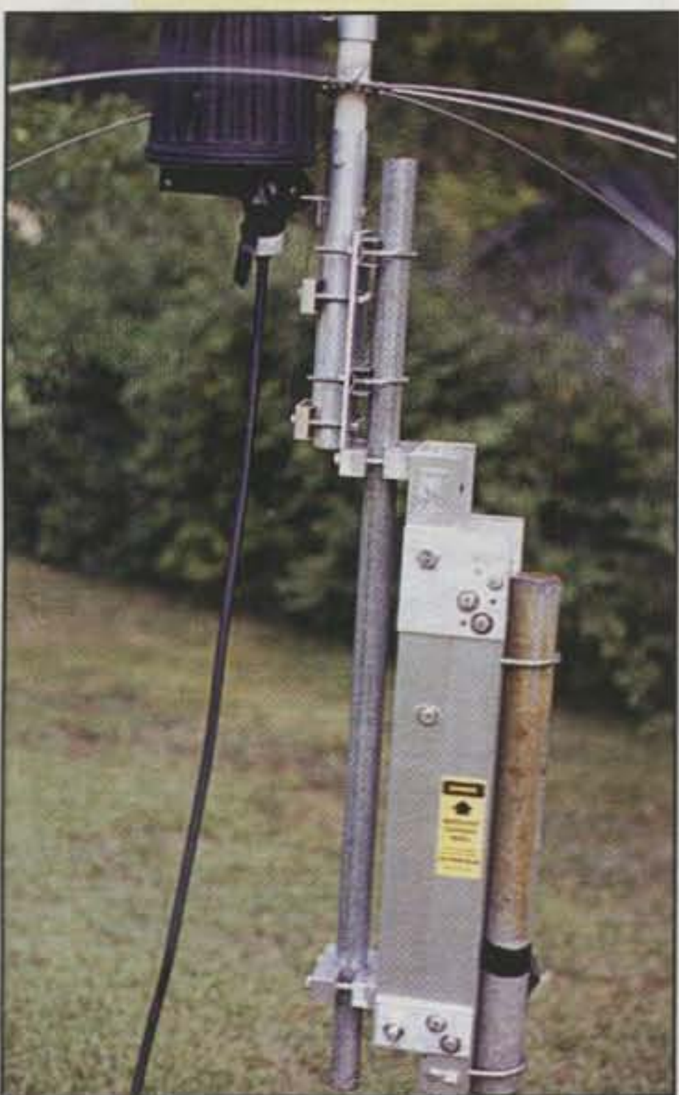
Photo 5— Surely the most useful vertical-antenna mounting accessory ever devised is this clever pneumatically-dampened tilt-over mount from Alpha Delta Communications. It allows one person to raise or lower a vertical up to 29 feet tall in less than a minute—a real back saver!
