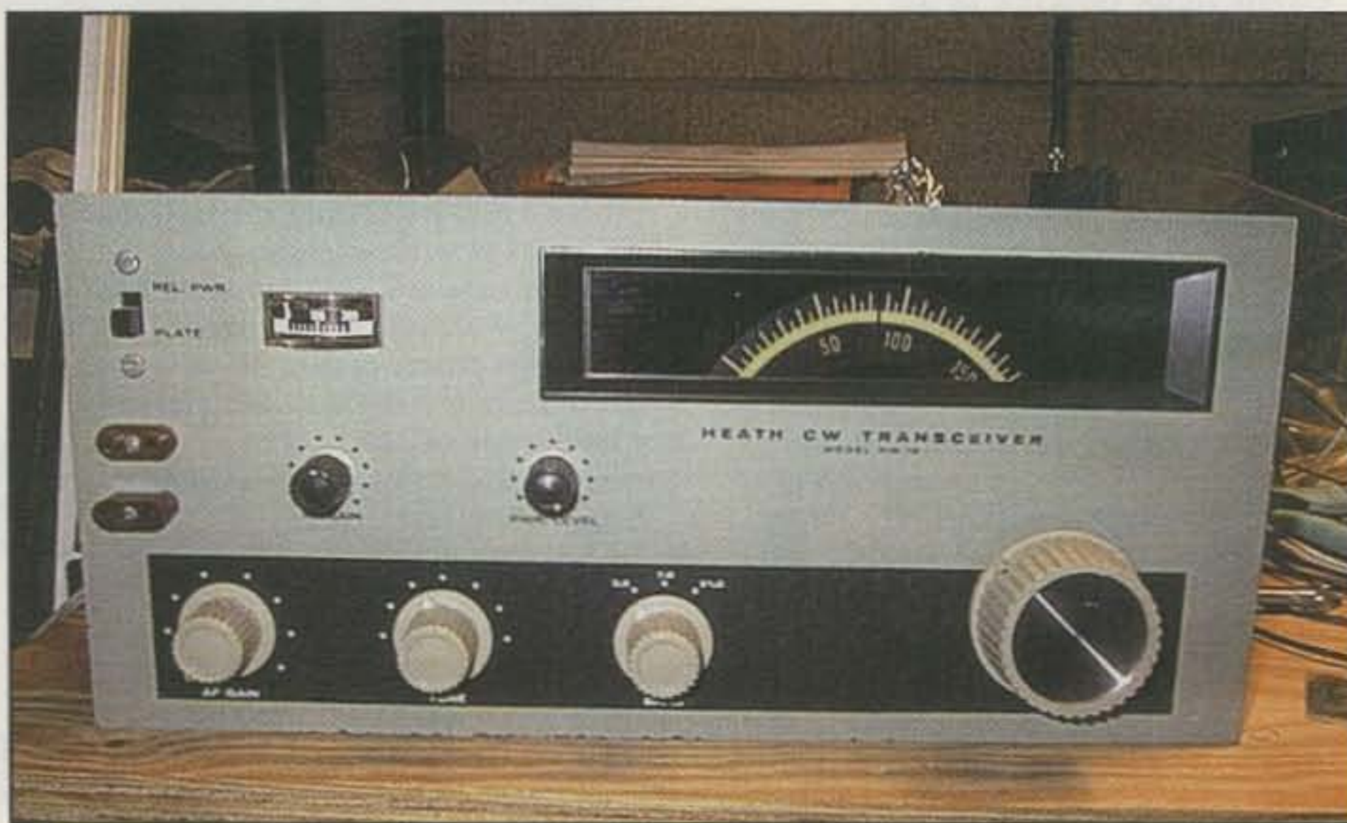
Front panel of the classic Heathkit HW-16 Novice transceiver. The tuning dial at right is for receive only, as FCC rules at the time required Novices to use crystal-controlled transmitters. Note the two crystal sockets at the far left. (Photos by the author)
