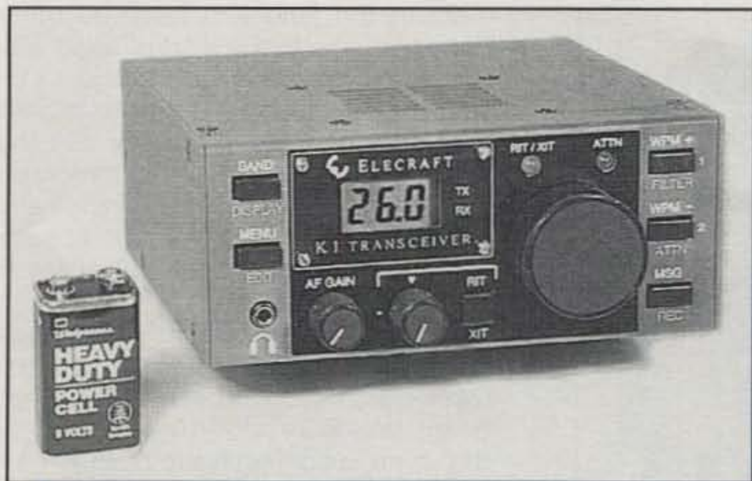
The new Elecraft K1 kit is a dual-band HF transceiver that runs 5 watts and measures only 2" x 5" x 5 1/2".
