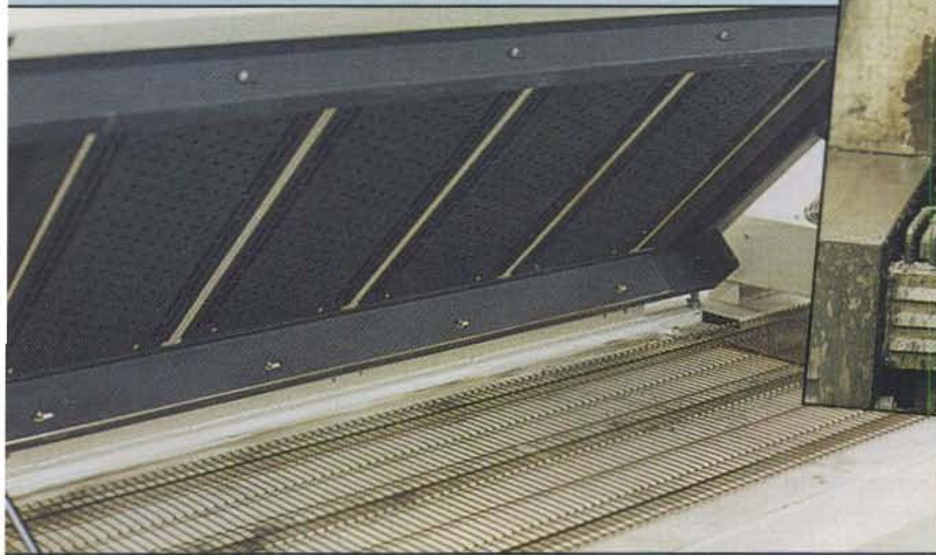
Photo 8— The surface-mount "pizza oven." Boards containing components placed on solder paste move slowly through this four-zone oven, where the solder melts and mounts the surface-mount parts to the surface of the circuit board.
