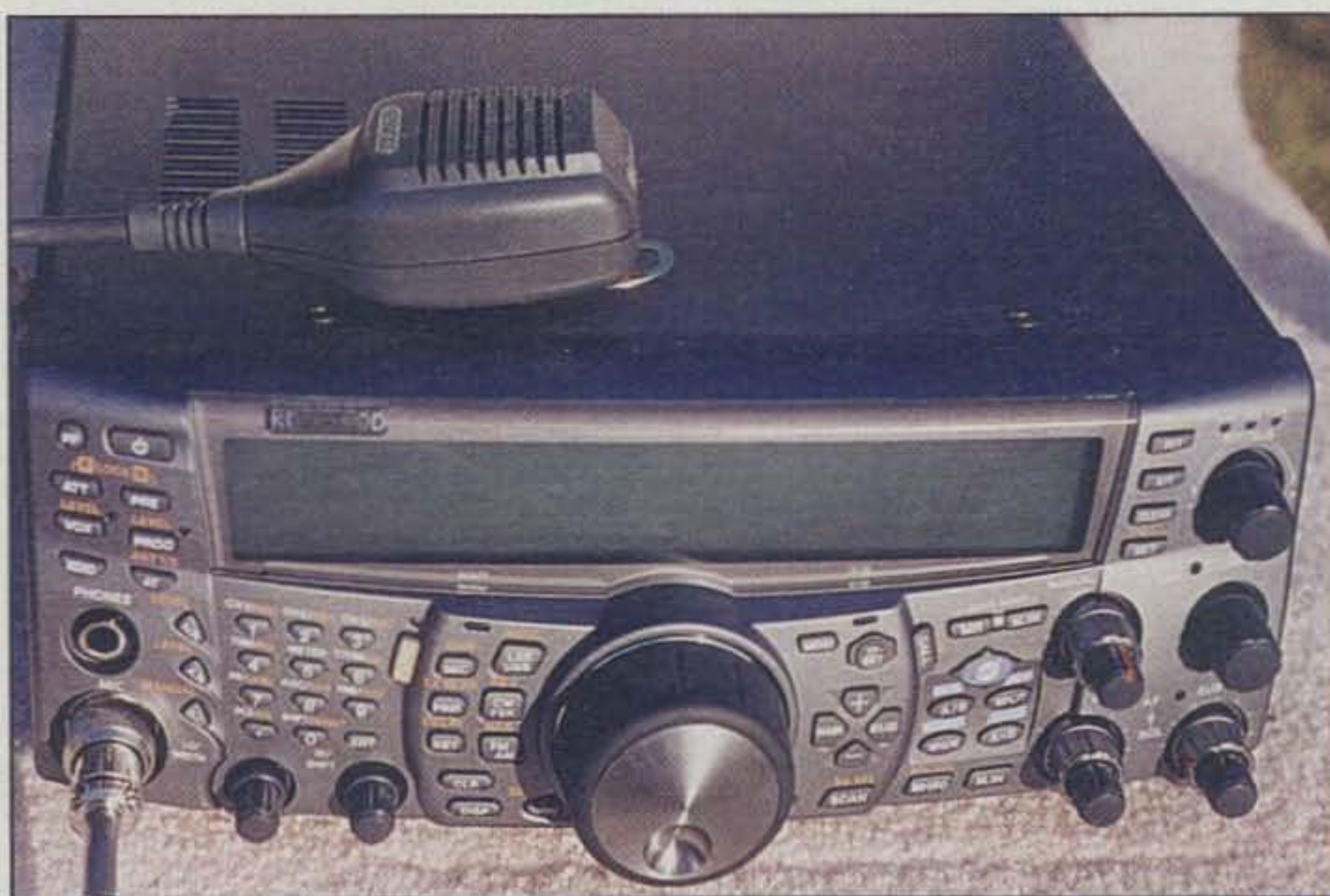
The new Kenwood TS-2000 offers HF, 6 meters, 2 meters, and 440, all multimode, with an optional 1200 MHz band unit that fits on the inside. It is also a full-blown satellite rig.
