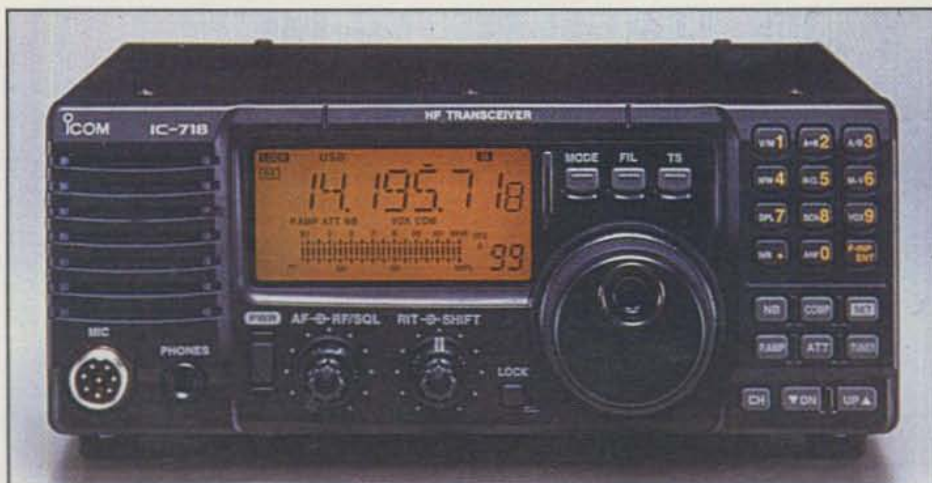
The ICOM IC-718 is not necessarily a small box, nor does it do 6 meters, but it does offer 100 watts output on HF, 101 memory channels, and a very large LCD display.
