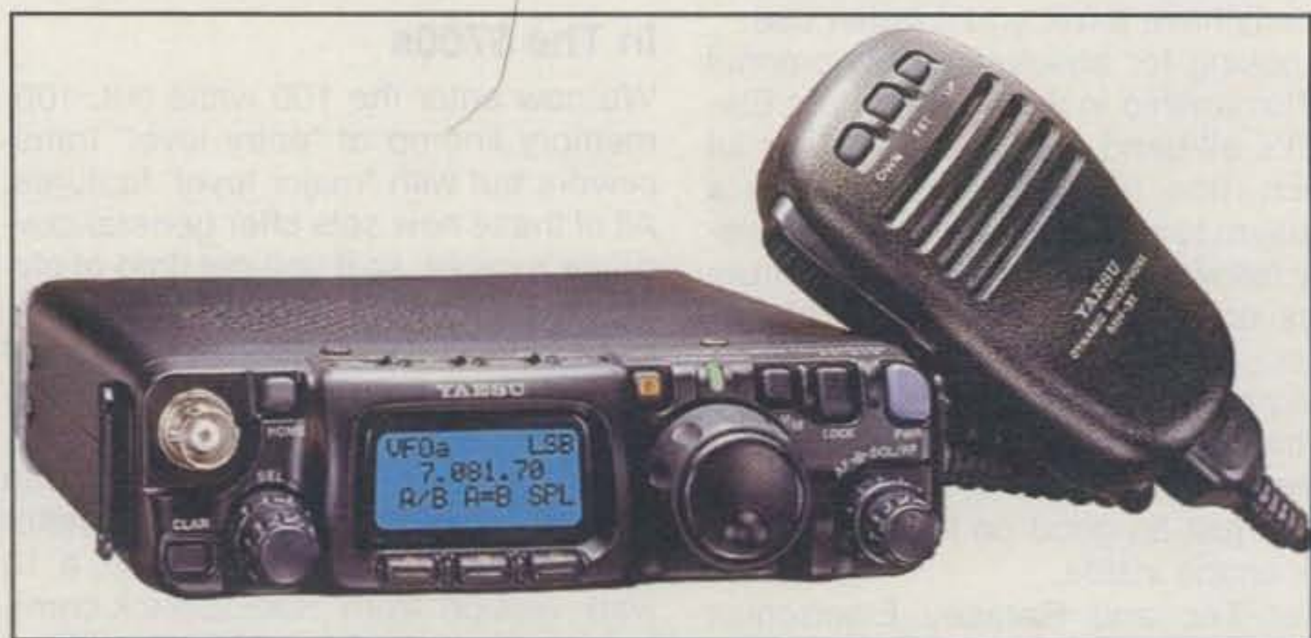
Yaesu's FT-817 is one of the hottest new rigs on the market today. Designed as a backpacking-QRP radio to operate from anywhere, the rig puts out 5 watts on all HF ham bands plus 6 meters, 2 meters, and 70 cm, in CW, SSB, FM, and AFSK for digital modes.
