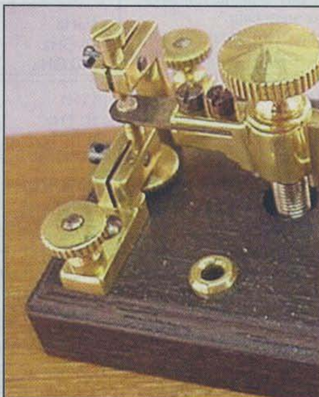
Photo 3— Close-up view of Swedish Key's rear contact assembly and related adjustments. Note tiny parts and intricate components of mechanism. Very nice!
