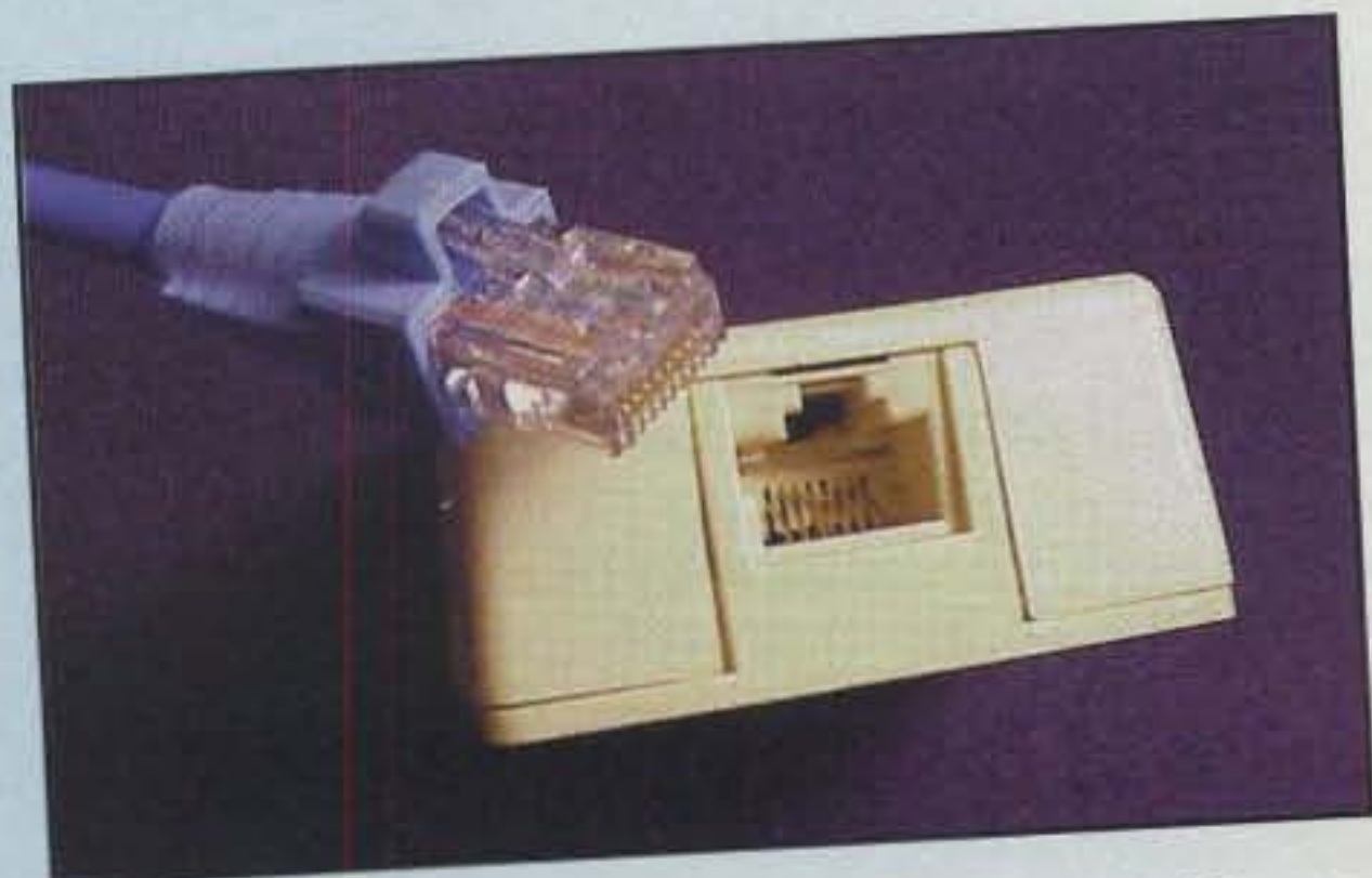
Fig. 1—A male (left) and female (right) RJ-45 connector. This is the same connector as used in many newer radios for the microphone connection. Note the "snagless" boot on the male connector, which prevents the release tab from snagging on objects as you pull the wire through walls. For computer networking be sure to use wire, connectors, and accessories certified to meet the Category 5 standard.
