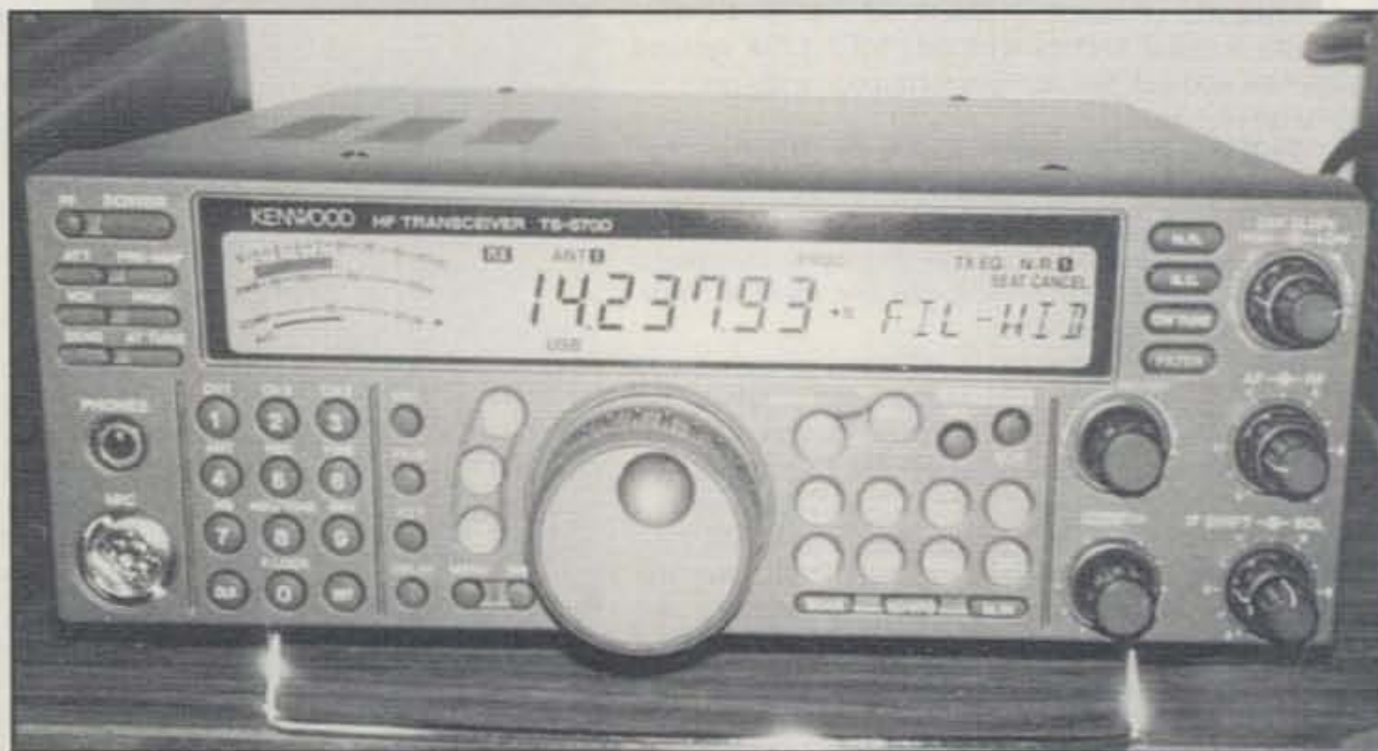
Photo A—DSP capabilities are built in or optional features in an increasing number of modern transceivers. They are used to reduce band noise (NR), cancel beat tones (BC), and dodge QRM by varying the slope of a passband's skirts (DSP slope). Some DSP systems operate at the IF level, while some operate at the AF level. They all work great!
