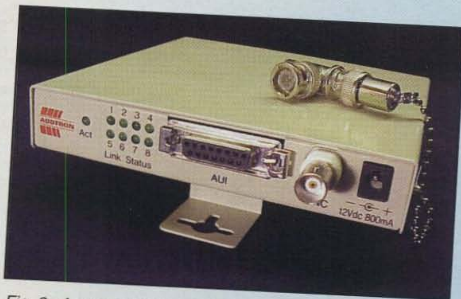
Fig. 2—An 8-port 10BaseT hub used by the author. This hub cost only $55 and has been in use for three years. At the rear there are eight RJ-45 jacks. On the front panel, shown, there is a BNC connector for ThinNet and a 15-pin Sub-D AUI connector. These two extra connectors allow older networking equipment to connect into the hub. Also note the eight "Link Status" LEDs, one for each port, and the power jack.
