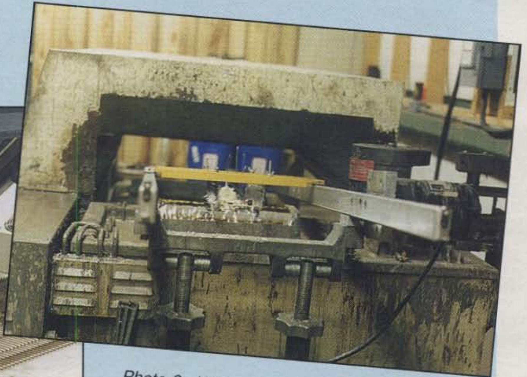
Photo 9— Wave soldering machine lays down a thin layer of solder on boards that are not suitable for surface-mount construction.
