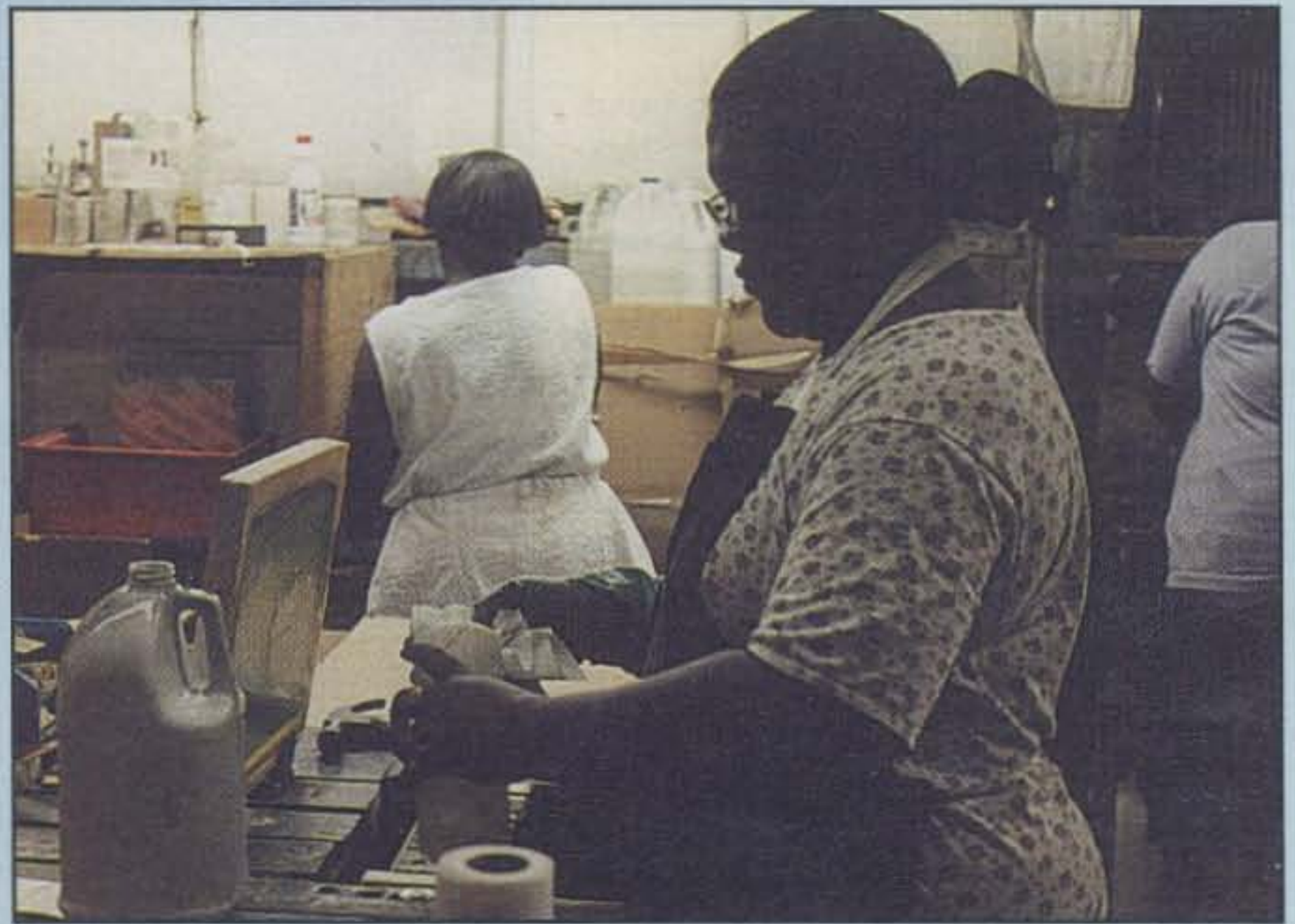
Photo 5—MFJ worker Azzie Weaver prepares a silk screen for printing labels onto newly cut, bent, and painted equipment enclosures.
