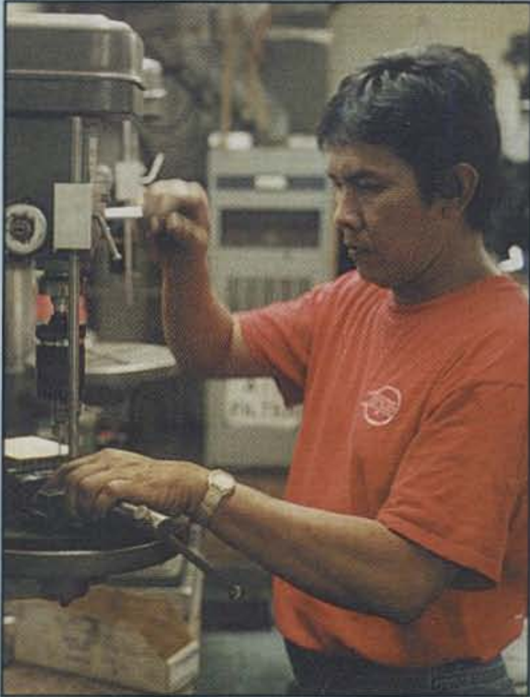
Photo 6— Hartono Agustus uses a drill press in the metal shop to tap threads into a block of metal that will be cut into rectangular pieces and used to hold screws that secure circuit boards inside a case.
