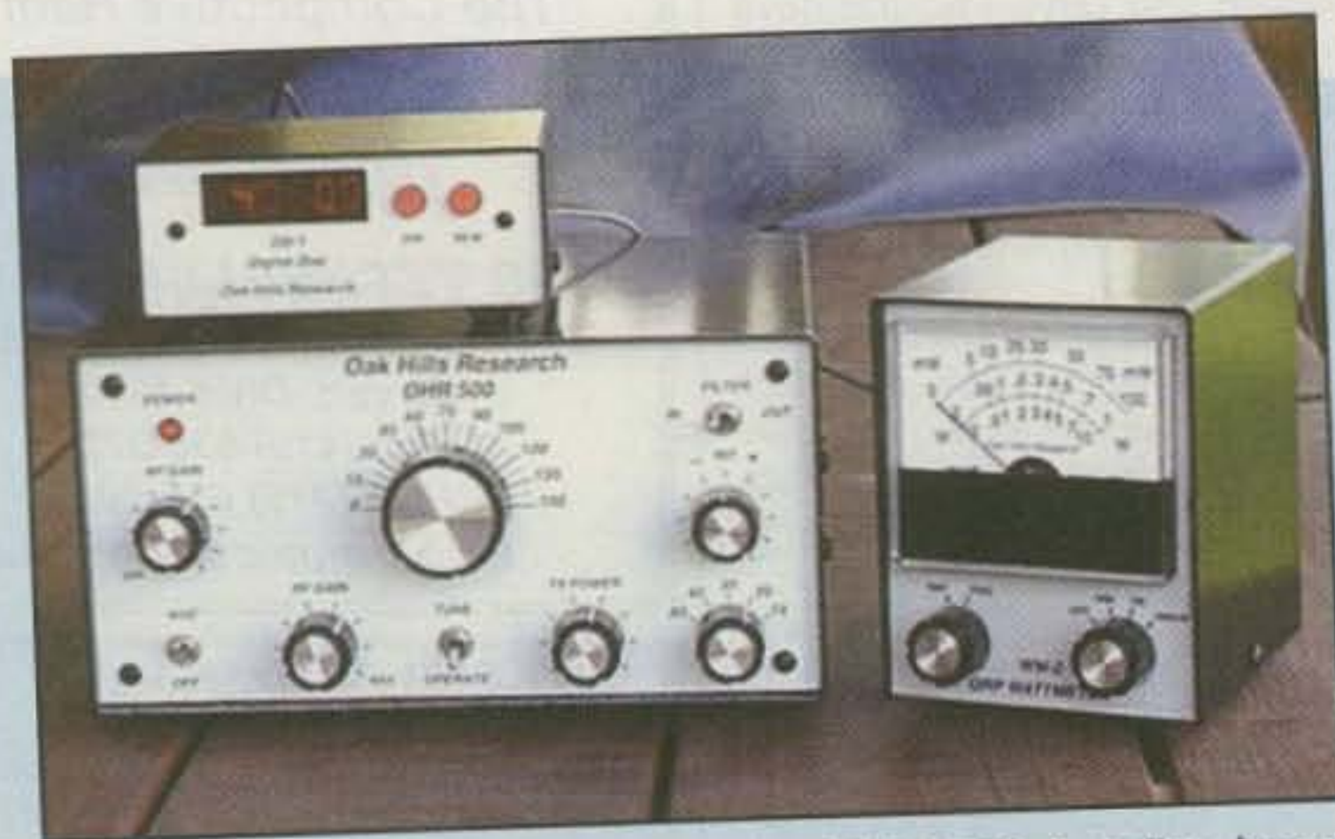
Photo B— The Oak Hills Research OHR 500 is a five-band CW transceiver that covers 150 kHz of the 80, 40, 30, 20 and 15 meter bands; it's shown here with the DD-1 Digital Display and WM-2 QRP Wattmeter. You'll find details in the text of this month's column.
