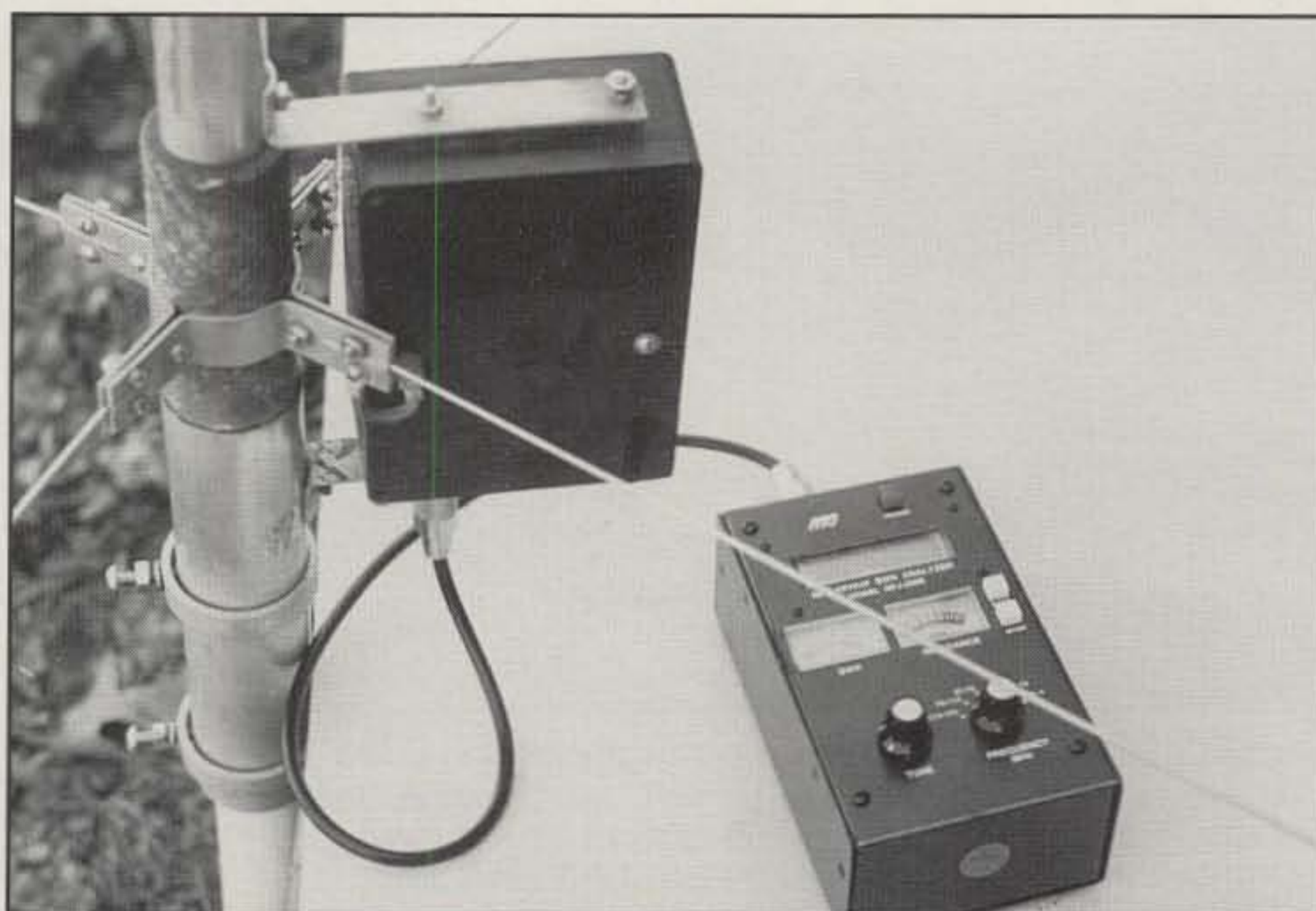
Photo B— To facilitate easy, on-the-spot tuning and checking, I compare the antenna's at-base SWR with its in-shack-measured SWR. Due to feedline interaction, all SWR measurements are shifted up-frequency by 80 to 100 kHz. The SWR is now 1.4:1 at 14.218 MHz.
