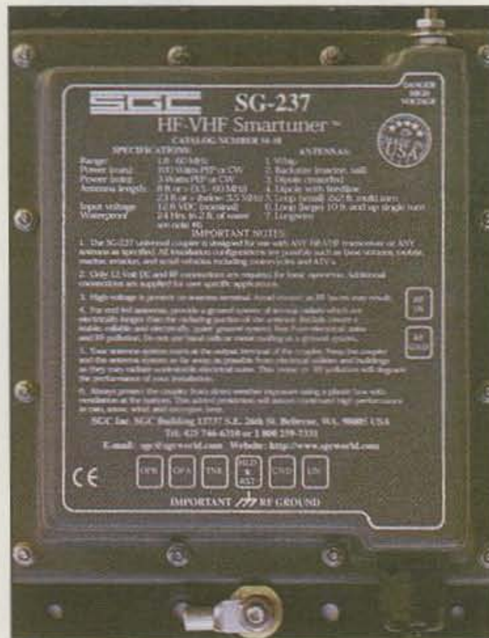
Photo A— This new SG-237 automatic tuning antenna coupler from SGC lets you operate 160 through 6 meters in a quite effective and hands-free manner. The little unit measures only 1.8"H x 7"W x 9"D and works with a 7 or 9 foot whip for mobiling, or with numerous wire antennas for home use.
