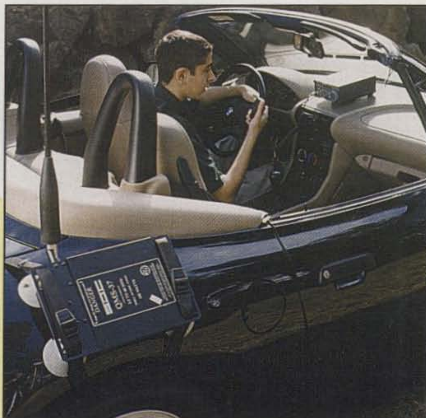
Photo B—As illustrated in this BMW setup, the complete SG-237/QMS-37/SG-307 automatic antenna system can be installed quickly on almost any vehicle without holes, screws, or marring the finish. (Photo courtesy SGC)
