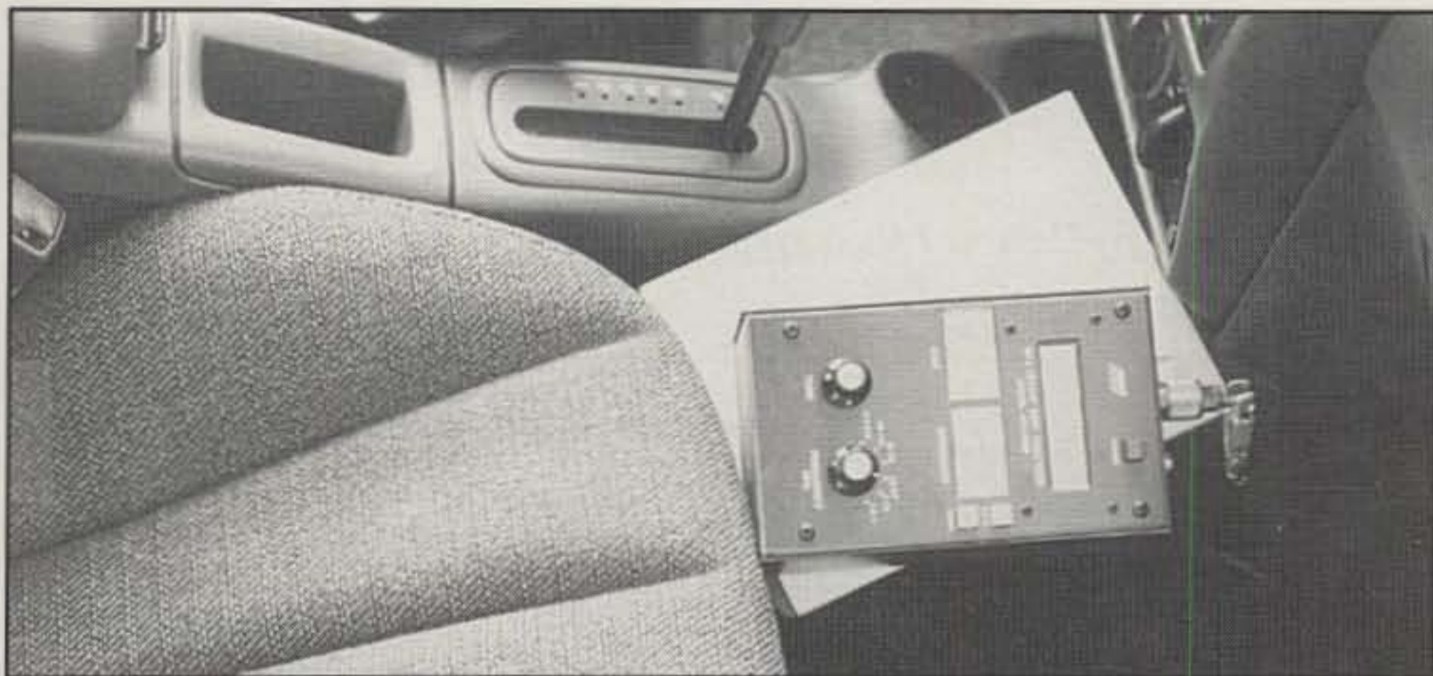
Photo E— The MFJ259B also works great for setting frequencies and adjusting impedance matching coils on mobile antennas—and you need not even put your transceiver in the vehicle until the antenna is perfectly set.
