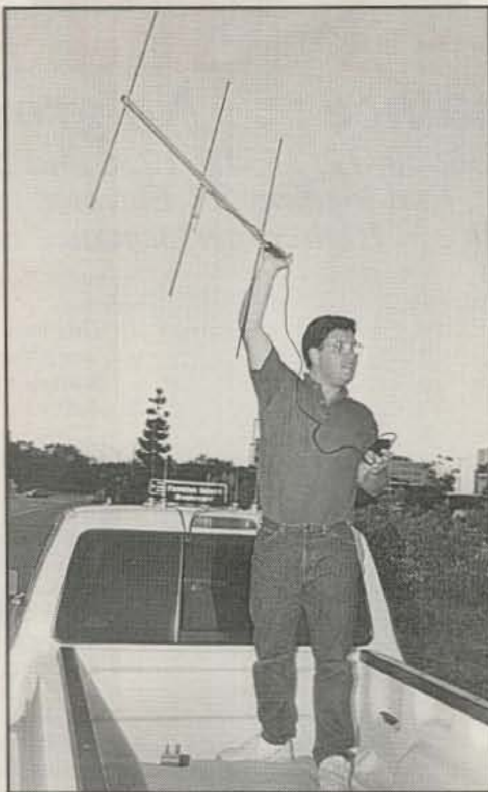
Photo B- When Paul Shinn's Doppler RDF set can't hear the fox's signal, he gets up in the back of his pickup and uses a handheld beam antenna to get bearings. (Photo by Joe Moell, K0OV)
