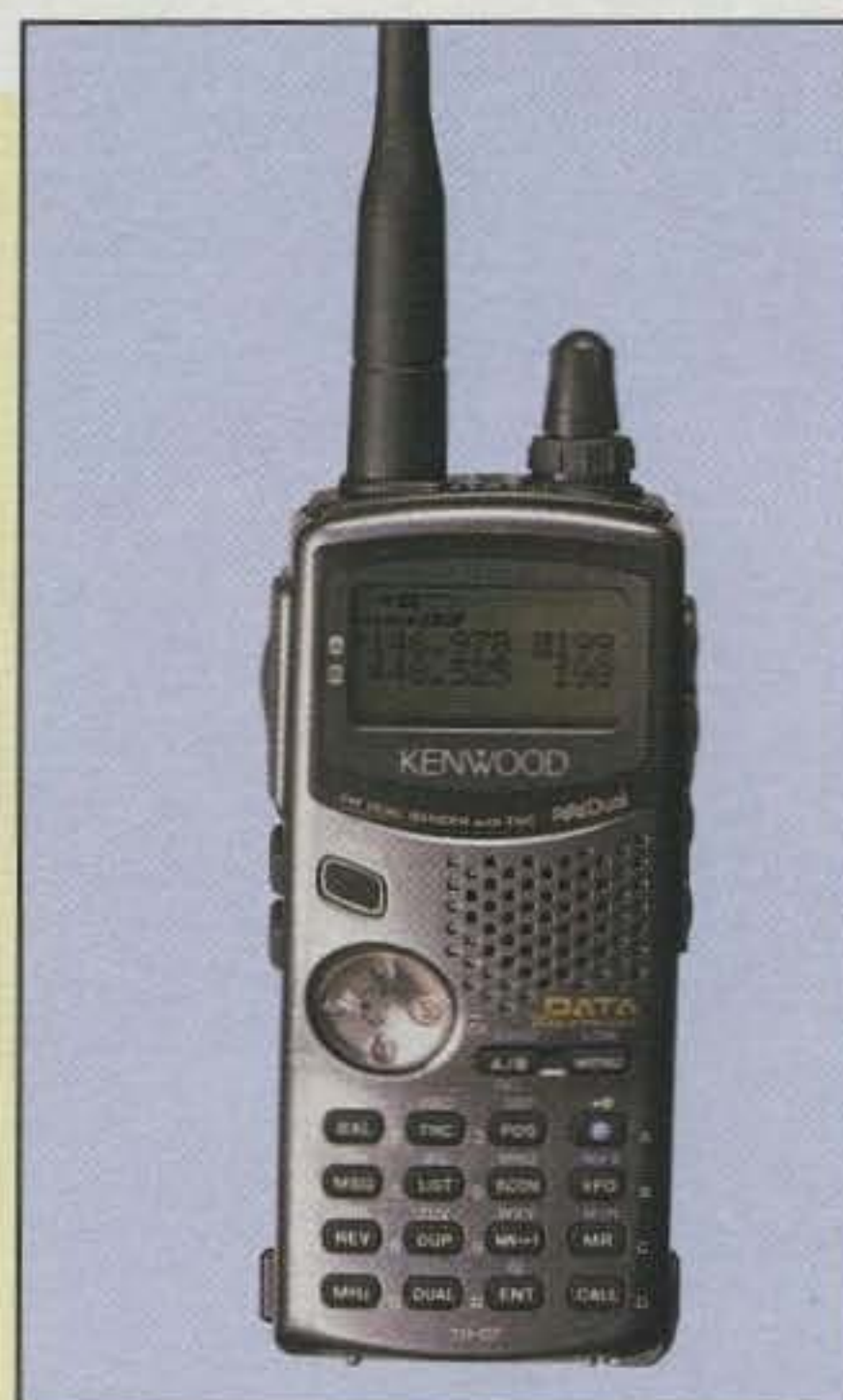
A built-in packet controller and software for APRS are the big features of Kenwood's TH-D7A. You can read short packet messages right on the screen, including downlinks from some amateur satellites. Hook up a GPS receiver and transmit your location wherever you are.
