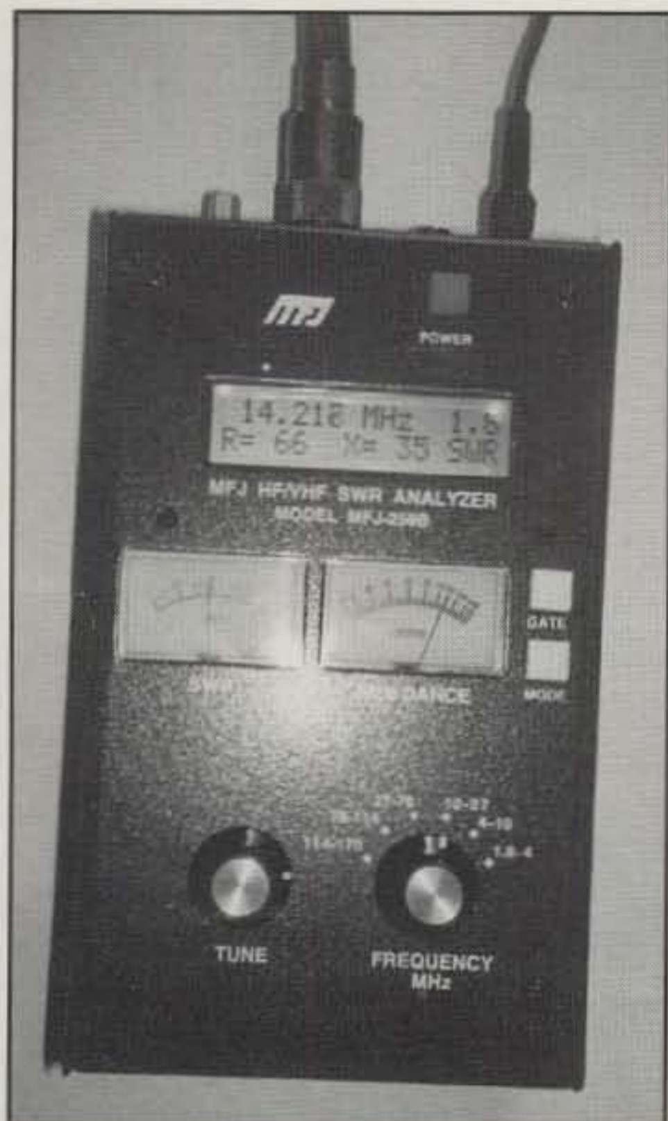
Photo A— The MFJ 259B Antenna Analyzer is an easy-to-use, self-contained unit that is ideal for checking SWRs, bandwidths, and coax cables; presetting a manual tuner's controls; and much more. Here it is checking the in-shack or "rig end of coax" SWR of a five-band vertical antenna as discussed in the text. Prior to adjusting the antenna's top length, SWR is 1.8:1 at 14.218 MHz.
