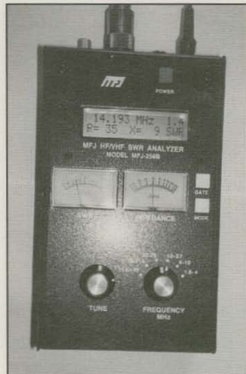
Photo D— Confidently returning to the shack, I recheck the antenna's "rig end of coax" SWR. It now shows 1.4:1 at 14.193 MHz. (Sorry—I did not aim for 14.218 exactly before taking the photo. Also, pardon the flash reflection from the camera.) The retuning was a rollicking success!
