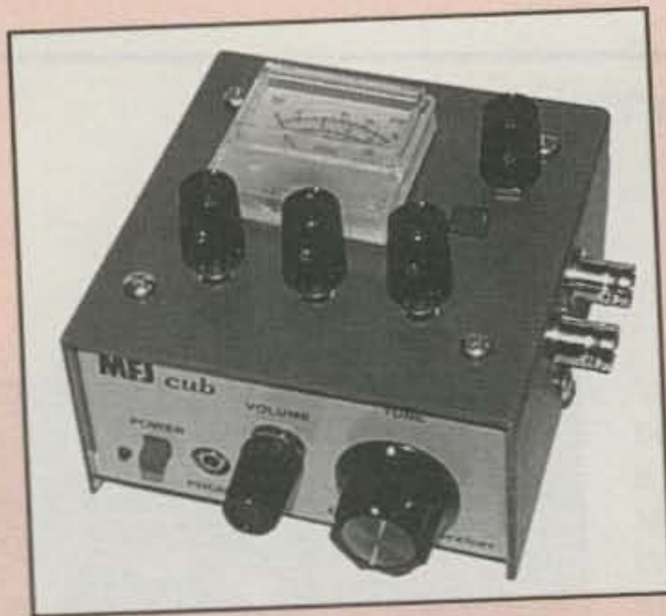
Photo C— MFJ's ever-popular '90 series CW QRP transceivers exhibit good sensitivity and selectivity and a solid 5 watt output signal. Units sport adjustable QSK and RIT top-mounted speaker and are well on their way to being classic. (Photo courtesy KC5NSZ and MFJ) →
