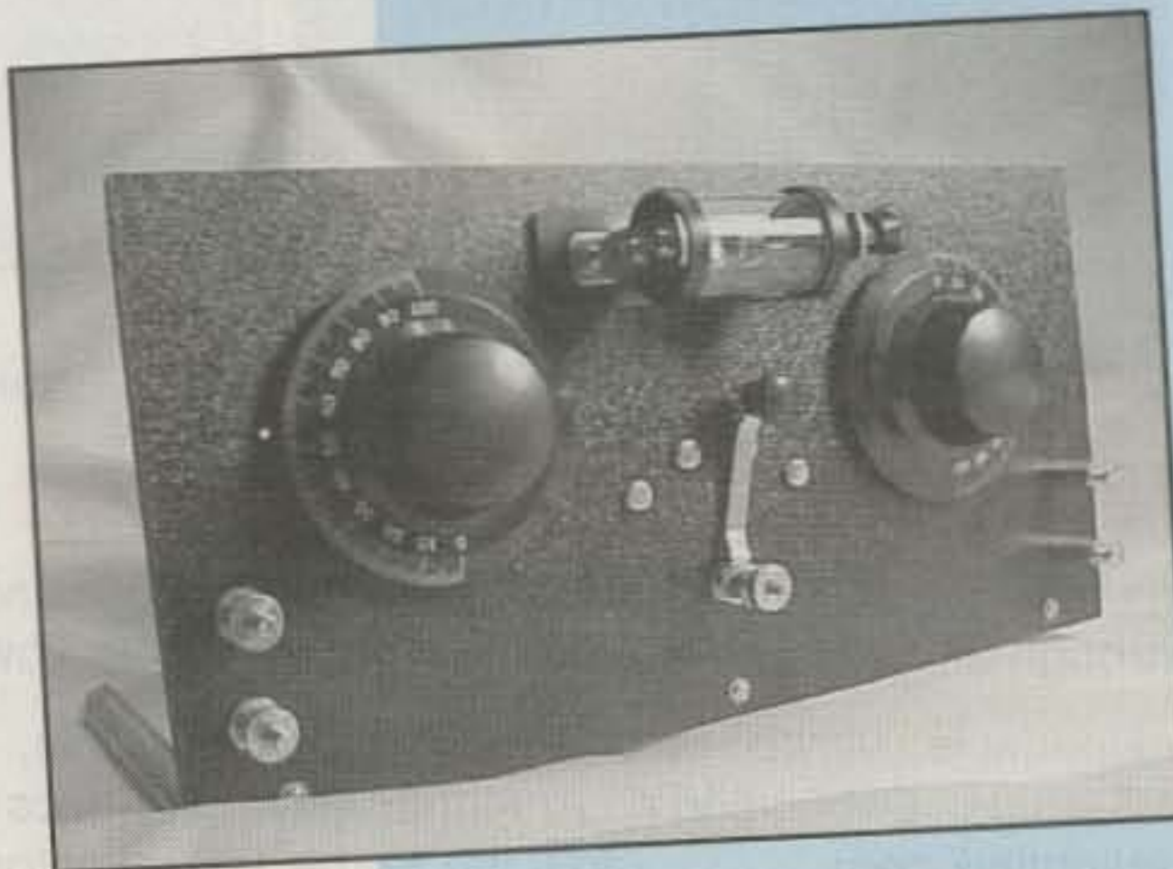
Photo B— This attractive reproduction of a vintage Levinson Radio Crystal Set from Australia was made by Dan Petersen, WA6OIL, and its authentic-era glamour is remarkable. Unit sports classic National "Velvet Vernier" knobs, cartridge-type crystal, and assembled-from-scratch antenna switch. Our special thanks to Dan, WA6OIL, and Rebecca Hewes of The Crystal Set Society for permission to highlight their "Levinson Repro Info" here in CQ.
