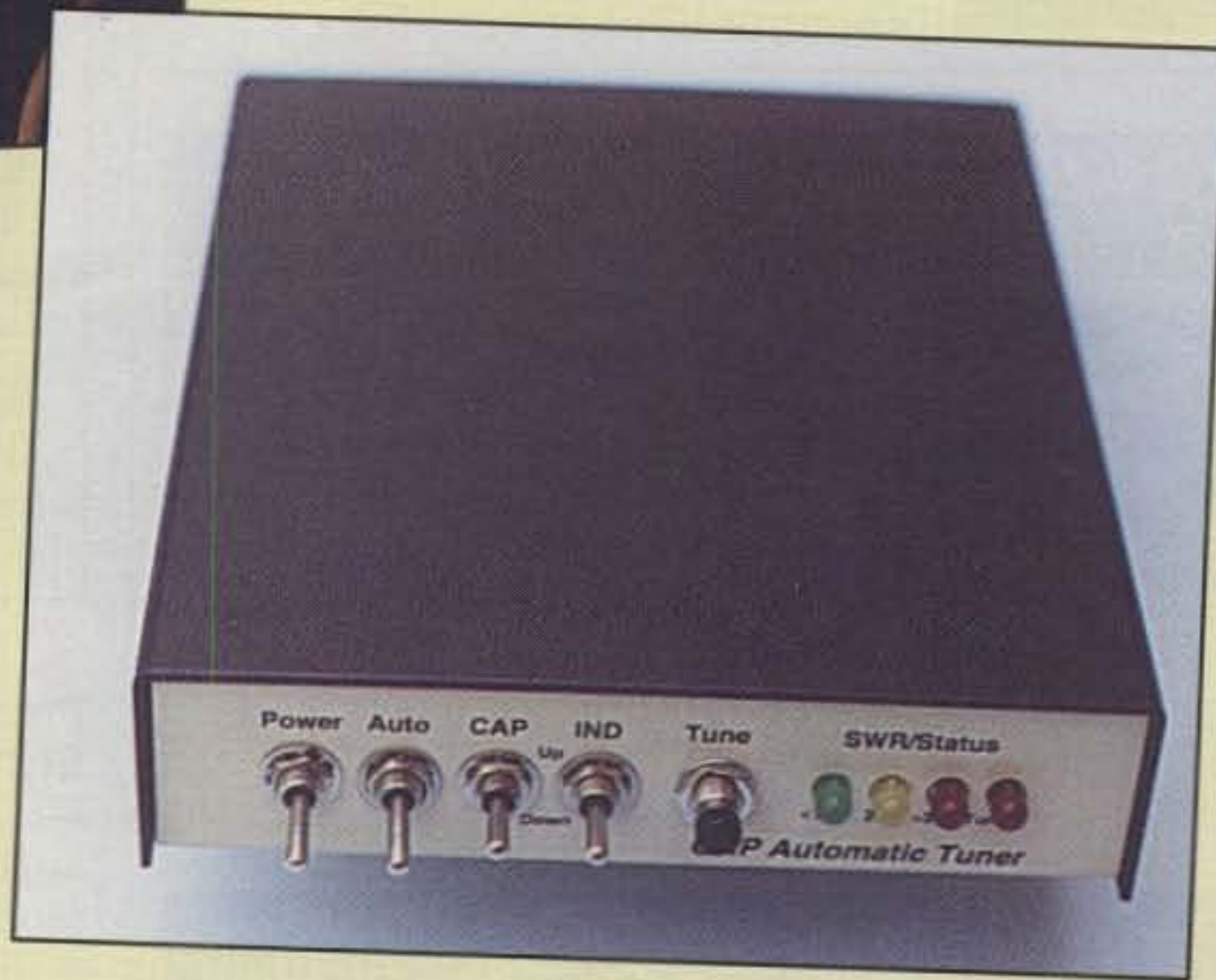
Photo D— This LDG stand-alone automatic antenna tuner is one of several units produced to work with all types of transceivers, and it makes "hands free" operation a cinch. This particular unit also includes a built-in SWR bridge for convenience.
