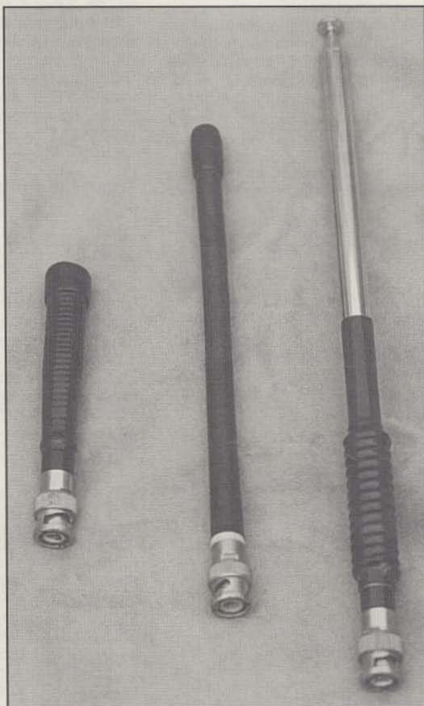
Antennas for handhelds come in all shapes and sizes, and very few are efficient. On the left here is a shortened duck antenna, which loses in effectiveness what it gains in convenience. In the center is a “standard” rubber-duck antenna, and at right is a telescoping half-wave antenna. (W2VU photos)
