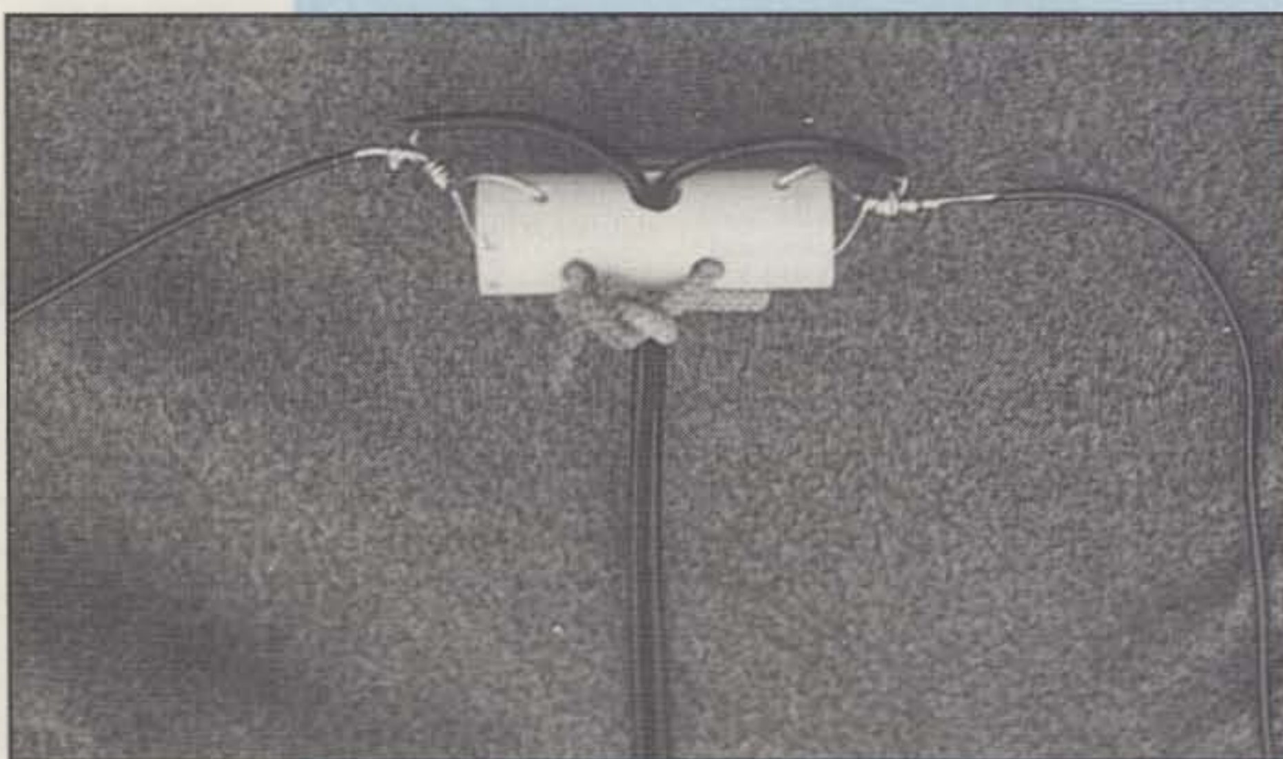
Insulator construction for the Lowe's dipole.
