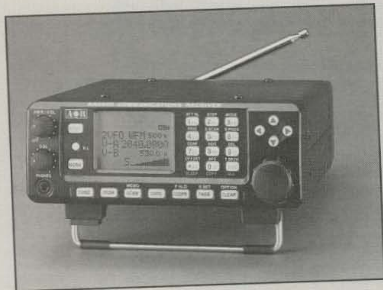
Photo A— Recently AOR USA introduced the AR8600 wide-range communications receiver. The unit's tuning range is 520 kHz to 2.040 GHz, with cellular ranges blocked. The receiver can accommodate optional cards that let you add extended features, and it accepts Collins mechanical filters for excellent selectivity. (Photo courtesy AOR USA)
