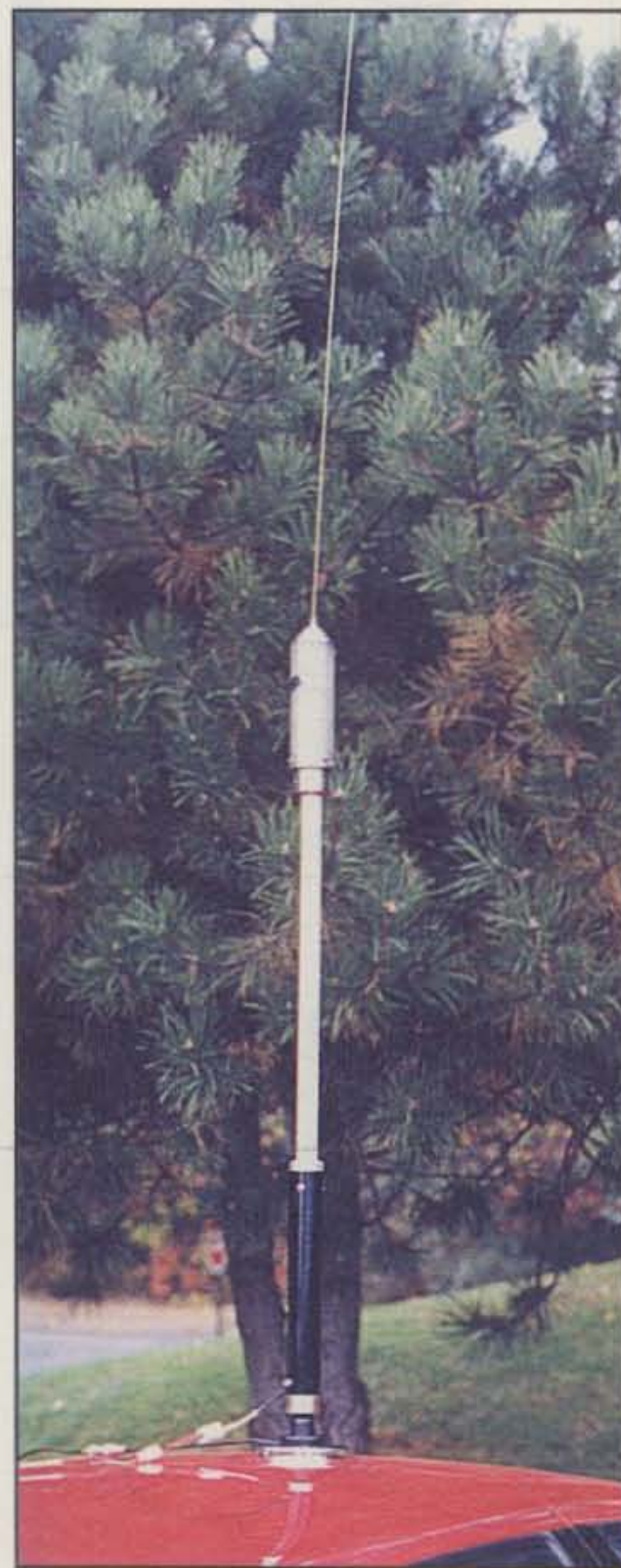
The Stealth II-2.5 antenna as attached to the author's car using a mag-mount configuration. Note that the setup shown here is for portable operation or testing only, as the antenna's weight cannot be supported by the magnet when the car is driven. The tuning coil is on top of the CNC-machined rod and a 6 meter whip is inserted into the top of the tuning coil assembly. (WB2AMU photo)
