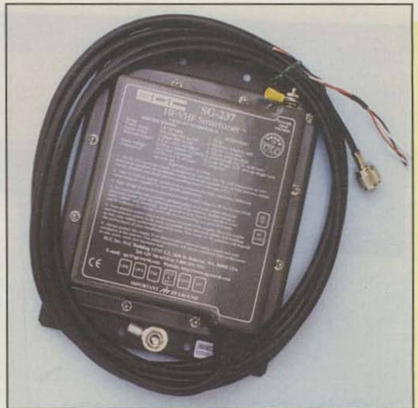
Photo E— Automatic antenna couplers such as this compact SGC Model 237 installed at the feedpoint or base of an antenna, match impedance and reduce SWR at the antenna’s base. The concept has the special advantage of minimizing radiation/signal pickup from coax cable and is often preferred for low-profile operations.
