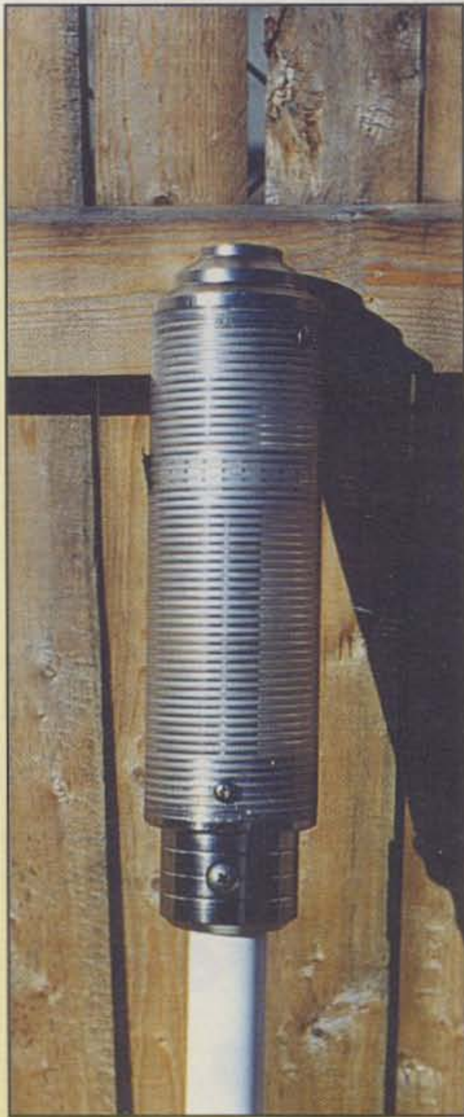
Close-up view of the tuning-coil assembly of the Stealth II-2.5 antenna. Note the excellent machining of the metal pieces that are located on the top and bottom parts of the tuner. You can see the tuning platform inside the coil itself. (WB2AMU photo)
