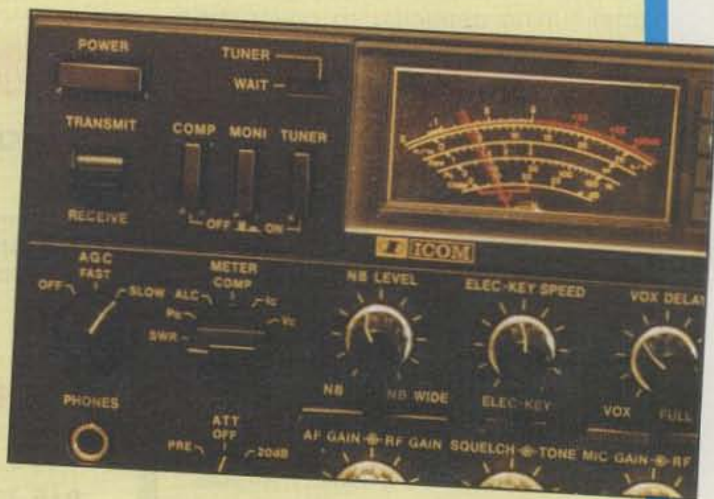
Photo B—ICOM's in-rig and automatic antenna tuners are analog-based with motors adjusting variable capacitors. They work like champs.
