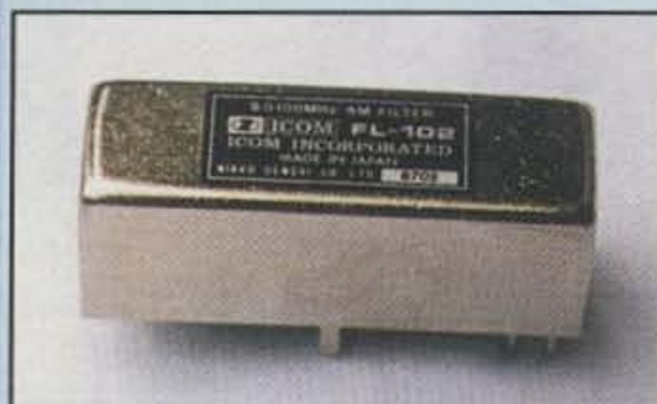
Photo B- This is an optional plug-in crystal ladder filter used for full-bodied AM reception with an ICOM transceiver. It operates at approximately 9 MHz and has a bandwidth of 6 kHz. Most optional SSB and/or CW filters look similar, but have more narrow bandwidths.
