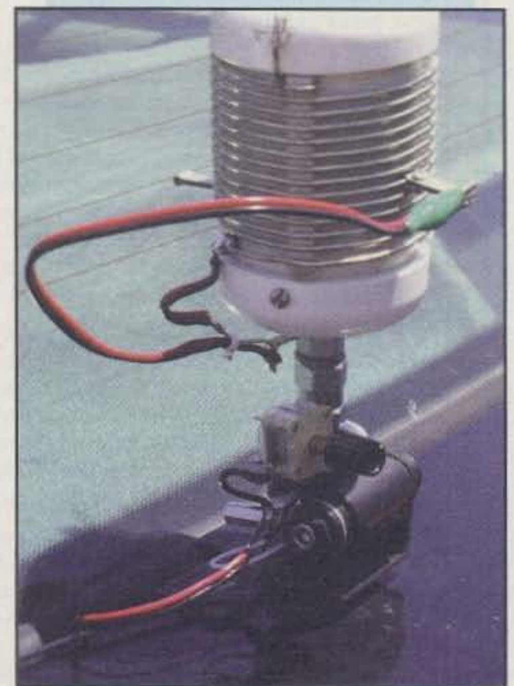
Photo F— "Business end" of the K5FLU base-loaded mini-mobile antenna showing B & W coil on PVC support, band clips/taps, miniature tuning capacitor, etc. A kit of parts to build this gem is available from MFJ Enterprises (details in text). (Photo courtesy Richard Stubbs and MFJ)
