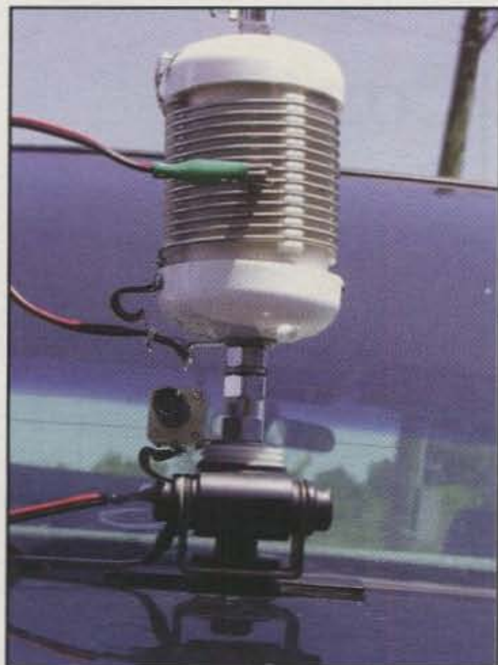
Photo G— Another view of the K5FLU mini-mobile 'tenna with miniature tuning capacitor near bottom of coil and set screw securing whip to screwstock at top of coil. End caps on top and bottom of coil support/form were cut down for custom appearance. (Photo courtesy Richard Stubbs and MFJ)
