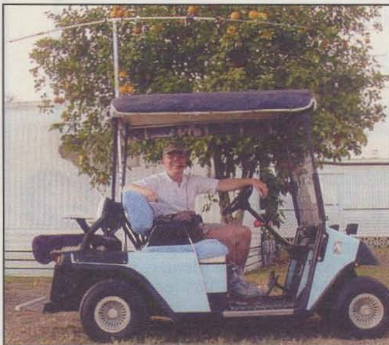
Photo D— An unusual operation for sure! Budd Drummond, W3FF, put together this golf-cart mobile setup during his annual visit to Florida, and it proved to be a real attention grabber on the air and on the course. Station consists of a Kenwood TS-50 with cart batteries for power and a rotary dipole for a signal squirter. (Photo via W3FF)
